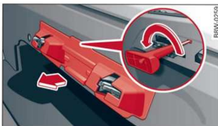
Fig. 47 Rear seat bench: Unlocking the storage box lid with the release tool
