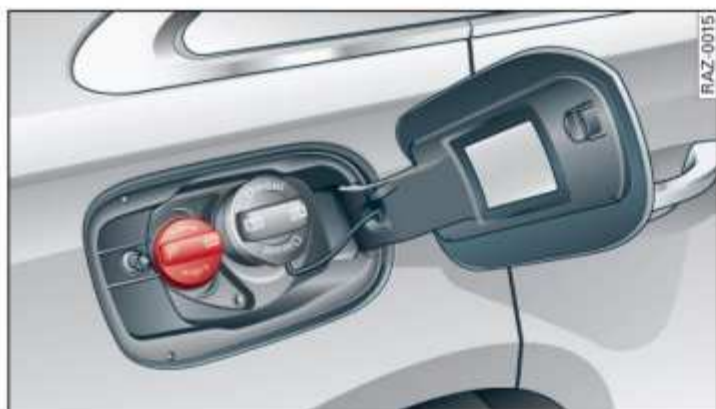
Fig. 185 Vehicle as seen from the rear right: Unscrewing the AdBlue cap
