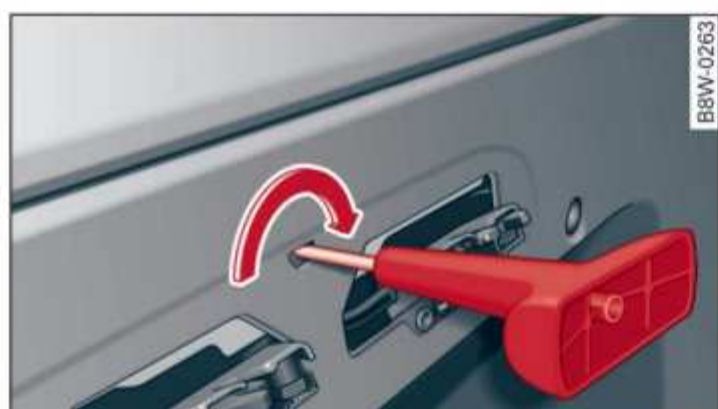
Fig. 52 Rear seat bench: Locking the storage box lid with the release tool
