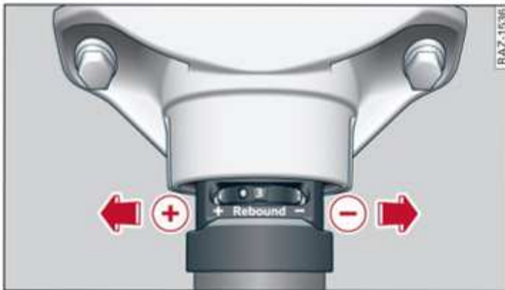
Fig. 117 Shock absorber piston rod: Adjuster wheel for rebound stage
