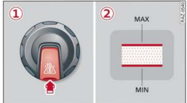
Fig. 193 Engine compartment – coolant expansion tank (example): ① Cap with release catch, ② Markings on coolant expansion tank (4-cylinder engine)
