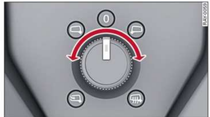
Fig. 59 Driver's door: Adjuster knob for exterior mirrors
