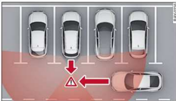
Fig. 158 Areas covered by sensors for rear cross-traffic assist
