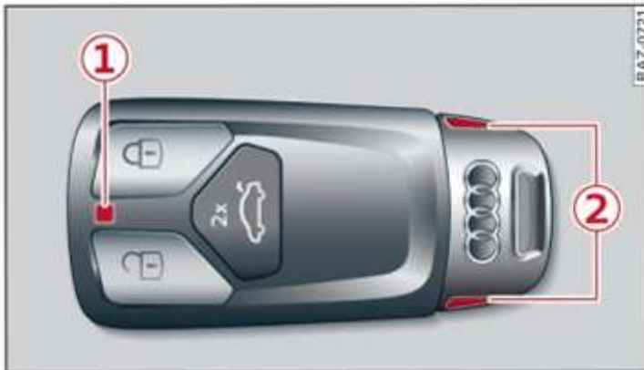
Fig. 29 Vehicle key: Removing battery holder
