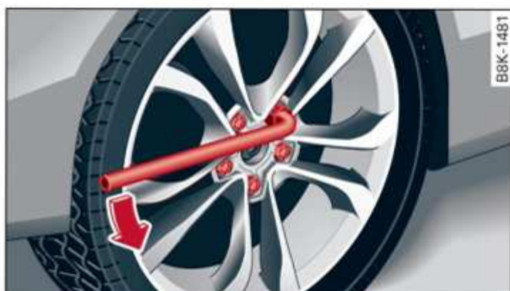
Fig. 208 Wheel: Loosening the wheel bolts
