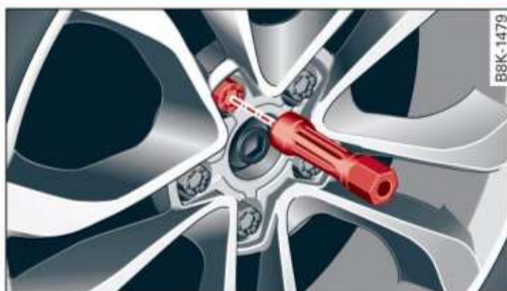
Fig. 211 Wheel: Hexagonal socket for turning wheel bolts
