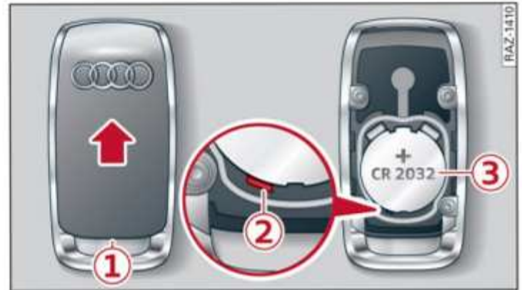
Fig. 108 Remote control: Changing battery
