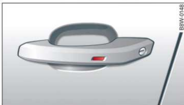
Fig. 28 Door handle: Sensor* for locking the vehicle
