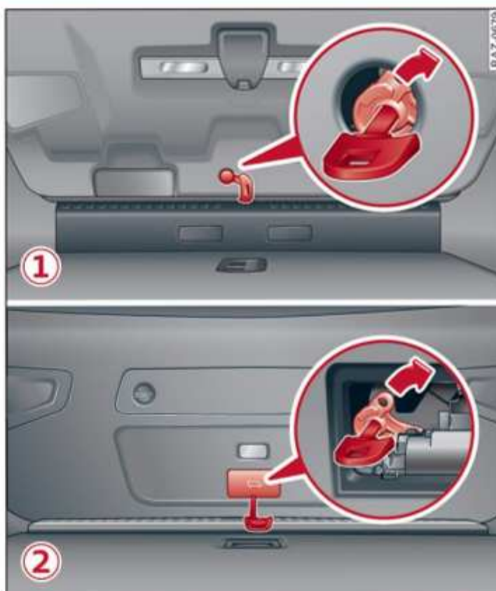
Fig. 35 Inside of boot lid: Access to manual release; ① Coupé, ② Sportback
