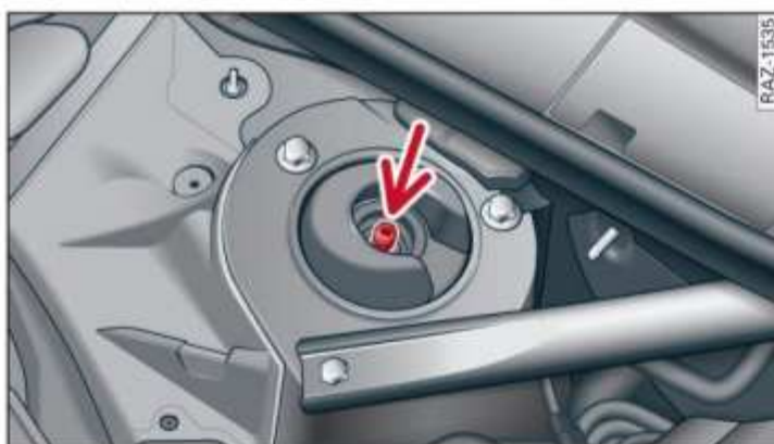
Fig. 116 Engine compartment: Hole for adjuster screw for setting rebound stage on front axle
