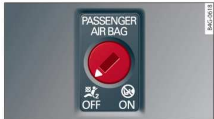
Fig. 81 Glove box: Key-operated switch for deactivating front passenger's airbag
