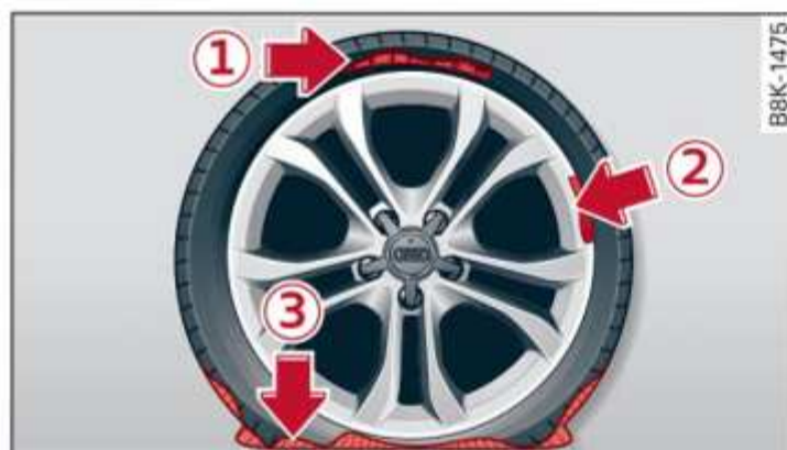
Fig. 203 Tyres: Irreparable tyre damage
