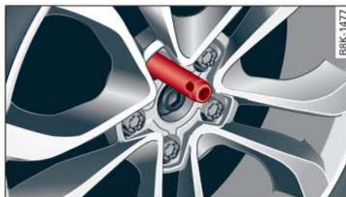
Fig. 212 Wheel: Mounting pin in wheel bolt hole nearest to the top
