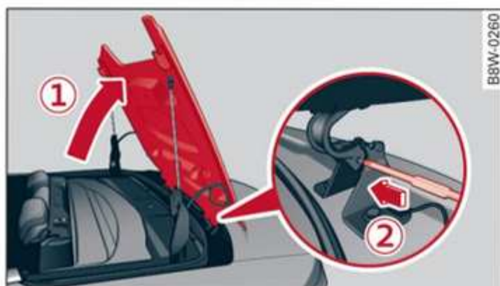
Fig. 48 Rear of vehicle: Lifting out and securing the storage box lid
