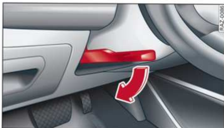
Fig. 69 Steering column: Lever for adjusting the steering wheel position
