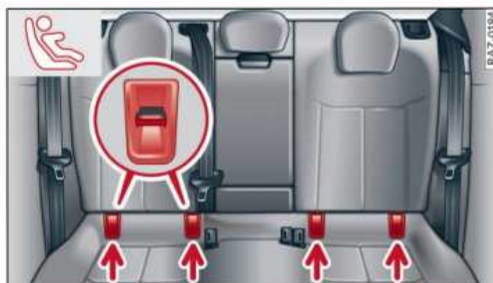
Fig. 84 Rear seat: Bottom ISOFIX anchorages
