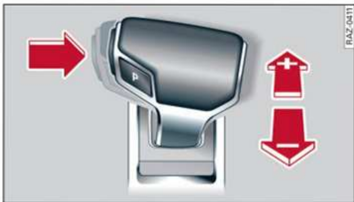
Fig. 111 Centre console: Manual gear selection using selector lever
