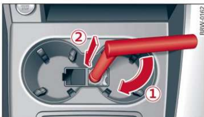
Fig. 114 Front cup holder: Releasing parking lock manually
