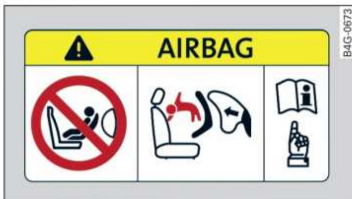
Fig. 83 Passenger's sun visor: Airbag sticker
