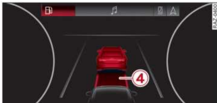
Fig. 145 Instrument cluster: Distance warning
