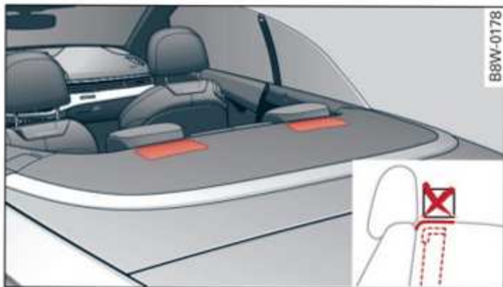
Fig. 87 Rear seats: Deployment area of rollover bars
