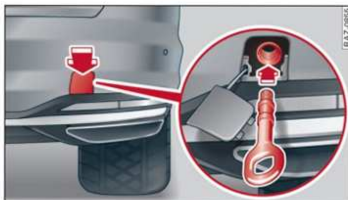
Fig. 216 Rear bumper: Fitting the towline anchorage
