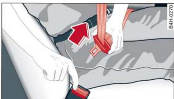
Fig. 77 The latch plate of the belt springs out of the buckle
