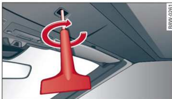
Fig. 50 Inside the front of the soft top: Locking the soft top with the release tool
