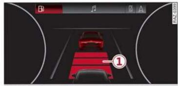
Fig. 91 Instrument cluster: brake intervention request
