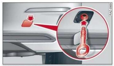
Fig. 162 Rear bumper: installing the towing loop (version 1)
