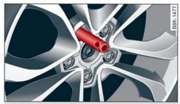
Fig. 158 Wheel: alignment pin in the top hole
