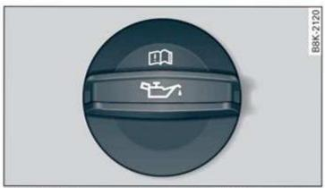
Fig. 138 Engine compartment: engine oil filling opening cover (example)
