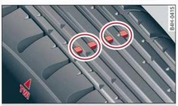
Fig. 145 Tire profile: treadwear indicator
