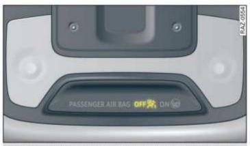
Fig. 61 Headliner: indicator light to display the status of the front passenger's airbag
