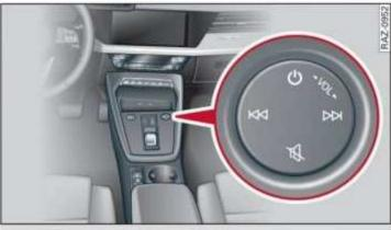
Fig. 21 Center console: MMI control pad
