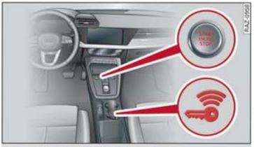
Fig. 73 Center console: starting the engine
