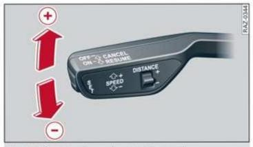
Fig. 89 Operating lever: changing the speed
