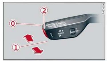
Fig. 94 Lever: using adaptive cruise assist
