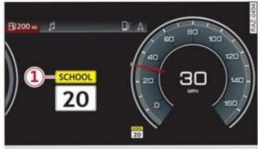
Fig. 81 Instrument cluster: traffic sign recognition
