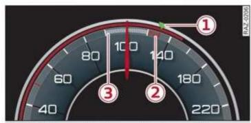
Fig. 92 Instrument cluster: speedometer: predictive control display
