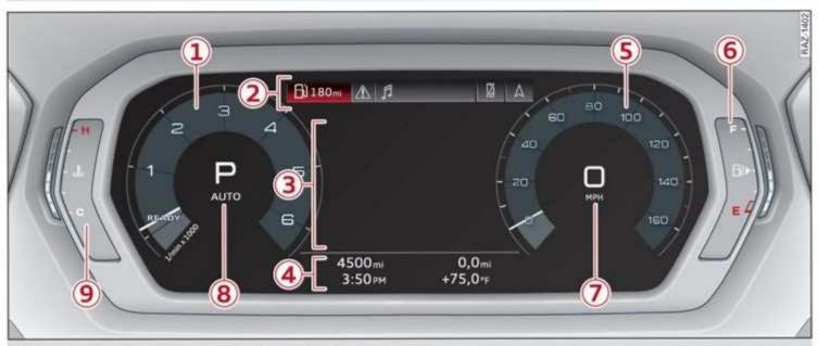
Fig. 4 Digital instrument cluster or Audi virtual cockpit overview
