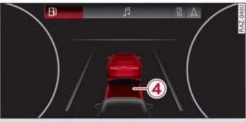
Fig. 97 Instrument cluster: distance warning
