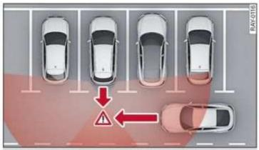
Fig. 107 Sensor detection range for rear cross-traffic assist
