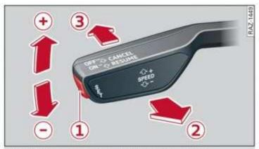
Fig. 83 Operating lever: switching the system on
