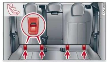
Fig. 62 Rear bench seat: lower LATCH anchors
