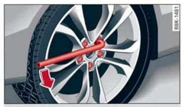
Fig. 154 Wheel: loosening the wheel bolts
