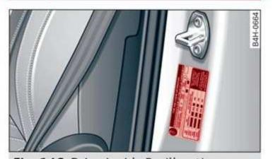
Fig. 146 Driver's side B-pillar: tire pressure label
