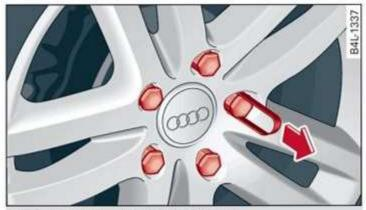
Fig. 152 Wheel: wheel bolts with caps
