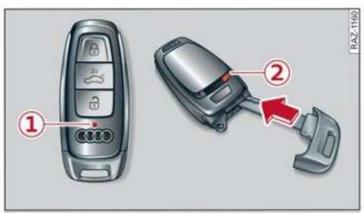
Fig. 27 Vehicle key: removing the battery cover
