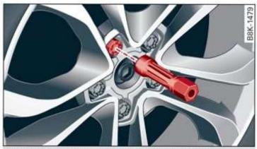
Fig. 157 Wheel: internal hex socket to turn the wheel holts
