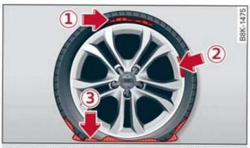
Fig. 149 Tire: tire damage that cannot be repaired
