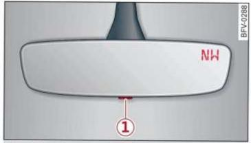
Fig. 47 Rearview mirror: digital compass is switched on
