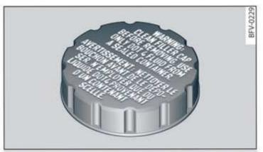
Fig. 140 Engine compartment: cap on brake fluid reservoir
