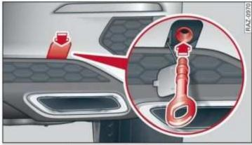
Fig. 163 Rear bumper: installing the towing loop (version 2)
