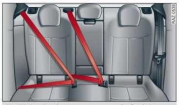
Fig. 65 Rear bench seat: securing unused safety belts
