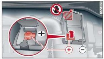
Fig. 141 Engine compartment: connections for the charging device or the jump start cable (vehicles with battery in the engine compartment)
