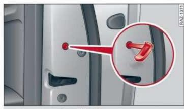
Fig. 24 Door: mechanically locking
