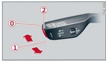
Fig. 88 Lever: using adaptive cruise assist
