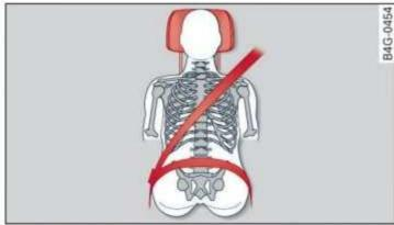
Fig. 52 Correctly-adjusted head restraint
