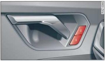
Fig. 22 Driver's door: central locking switch
