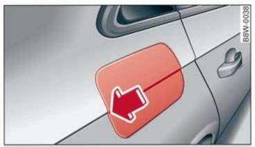
Fig. 131 Right rear side of the vehicle: opening the fuel filler door
