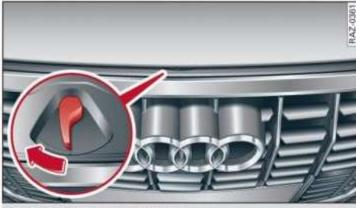
Fig. 134 Unlocked hood: lever
