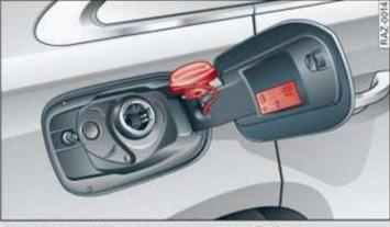
Fig. 132 Fuel filler door with attached fuel cap
