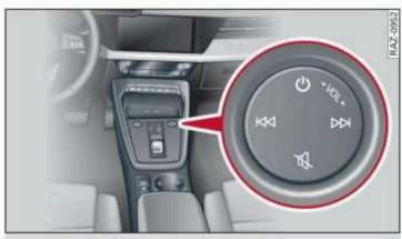
Fig. 20 Center console: MMI control pad
