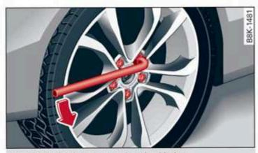
Fig. 152 Wheel: loosening the wheel bolts
