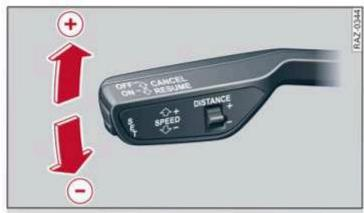
Fig. 87 Operating lever: changing the speed
