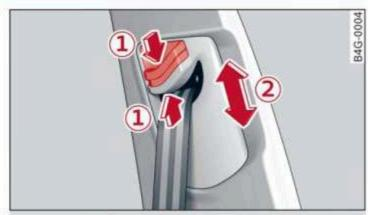
Fig. 58 Belt height adjustment for the front seats - safety belt relay
