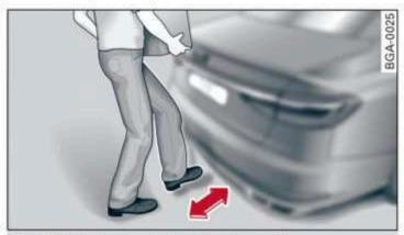
Fig. 30 Vehicle rear: foot motion (example)
