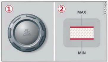
Fig. 137 Engine compartment - coolant expansion tank (diagram): 1 cover; 2 markings
