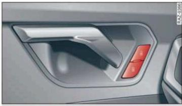
Fig. 21 Driver's door: central locking switch
