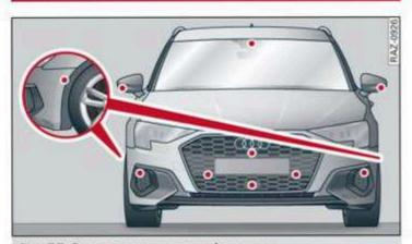
Fig. 77 Front area: sensors and cameras
