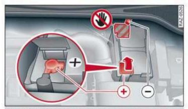
Fig. 139 Engine compartment: connections for the charging device or the jump start cable (vehicles with battery in the engine compartment)
