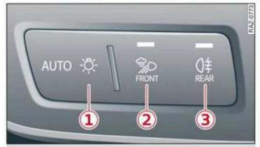
Fig. 37 Instrument panel: light button module
