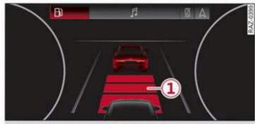
Fig. 93 Instrument cluster: request for driver intervention
