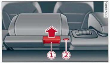
Fig. 67 Center backrest: release lever and latching indicator with red marking
