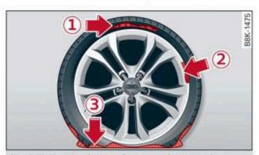
Fig. 147 Tire: tire damage that cannot be repaired
