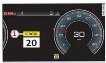
Fig. 79 Instrument cluster: traffic sign recognition
