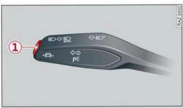
Fig. 96 Turn signal lever: button for lane departure warning and lane guidance for adaptive cruise assist\*
