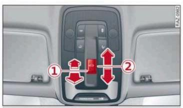
Fig. 36 Headliner: panoramic glass roof button
