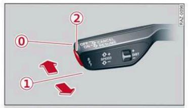
Fig. 91 Lever: overriding the control
