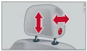
Fig. 52 Front seat: adjusting the head restraint
