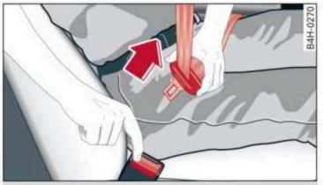
Fig. 57 Releasing the belt buckle from the belt latch
