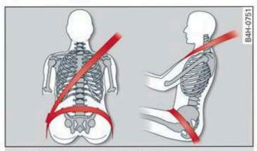
Fig. 54 Lap/shoulder belt positioning
