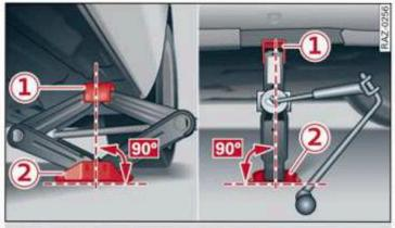
Fig. 154 Sill: positioning the vehicle jack
