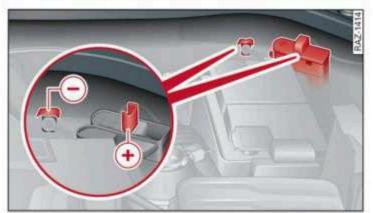
**Fig. 140** Engine compartment: connections for the charging device or the jump start cable (vehicles with jump start connection in the engine compartment)
