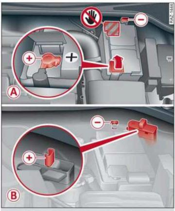
Fig. 157 Engine compartment: connections for a charger or a jump start cable: (A) vehicles with battery in the engine compartment, (B) vehicles with jump start connection (+) in the engine compartment
