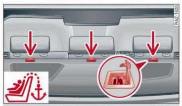
Fig. 62 Rear shelf: top tether anchors to secure a child safety seat with an upper belt
