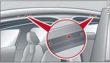
Fig. 70 Roof: mounting points
