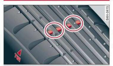
Fig. 143 Tire profile: treadwear indicator
