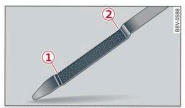
Fig. 135 Oil dipstick (example): checking the engine oil level
