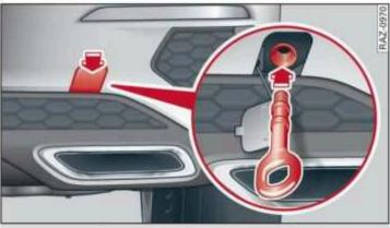
Fig. 161 Rear bumper: installing the towing loop (version 2)
