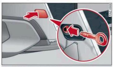
Fig. 159 Front bumper: installing the towing loop
