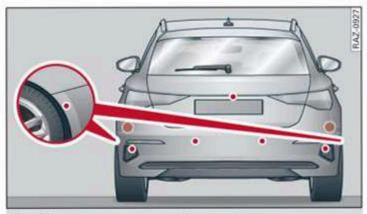
Fig. 78 Rear area: sensors and cameras
