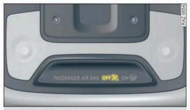
Fig. 60 Headliner: indicator light to display the status of the front passenger's airbag
