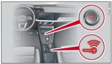
Fig. 72 Center console: starting the engine
