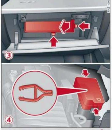
Fig. 163 Glove compartment (right-hand drive): cover (3); left side of engine compartment: cover (4)
