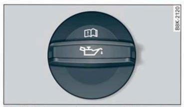
Fig. 136 Engine compartment: engine oil filling opening cover (example)
