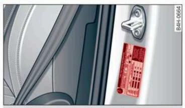
Fig. 144 Driver's side B-pillar: tire pressure label
