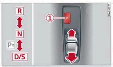
Fig. 73 Center console: selector lever
