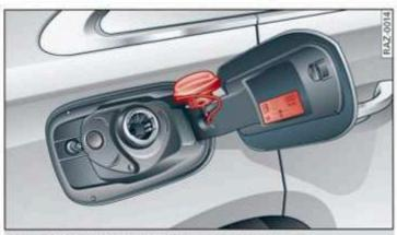
Fig. 130 Fuel filler door with attached fuel cap
