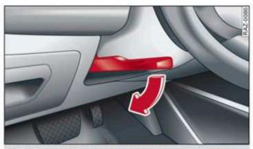
Fig. 50 Steering column: lever for adjusting the steering wheel position
