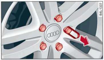
Fig. 150 Wheel: wheel bolts with caps
