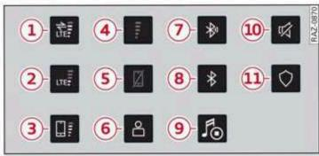
Fig. 15 Center display: frequently used symbols in the status bar
