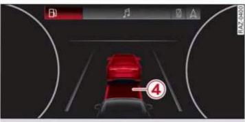
Fig. 95 Instrument cluster: distance warning
