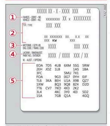
Fig. 167 Vehicle identification label
