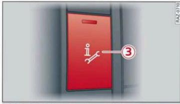
Fig. 114 Front headliner: online roadside assistance button
