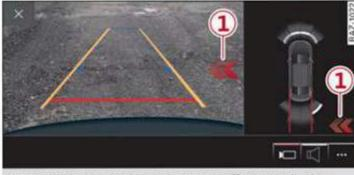
Fig. 106 Center display: rear cross-traffic assist display
