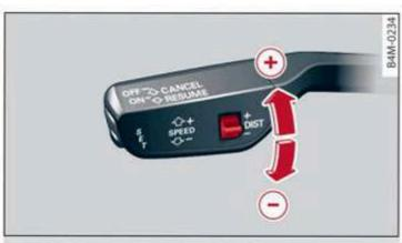
Fig. 90 Operating lever: setting the distance
