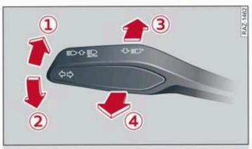
Fig. 38 Operating lever: switching the light functions on and off
