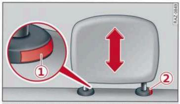
Fig. 53 Rear seat: adjusting or removing the head restraint
