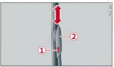
Fig. 45 Windshield wipers: changing the wiper blades
