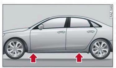
Fig. 153 Sill panels: markings
