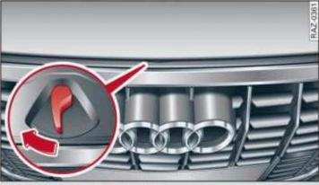
Fig. 132 Unlocked hood: lever
