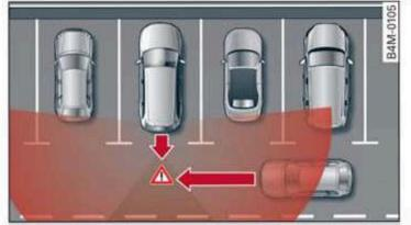
Fig. 105 Sensor detection range for rear cross-traffic assist
