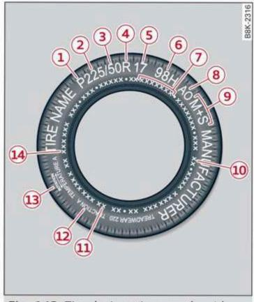
Fig. 142 Tire designations on the sidewall
