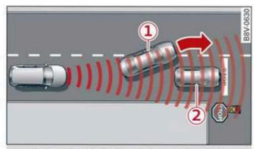
Fig. 82 Example: vehicle changing lanes and stationary vehicle
