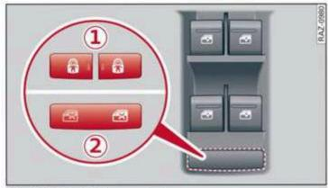
Fig. 33 Driver's door: controls
