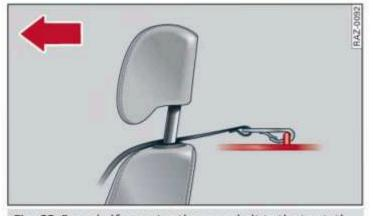
Fig. 63 Rear shelf: securing the upper belt to the top tether anchor
