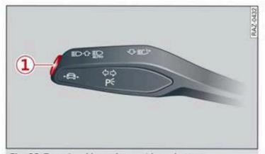
Fig. 88 Turn signal lever: lane guidance button
