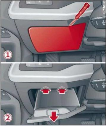
Fig. 162 Area of the steering column (left-hand drive): cover (1); storage compartment\* (2)
