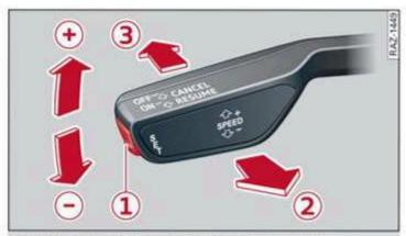
Fig. 81 Operating lever: switching the system on
