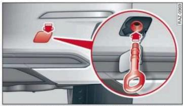
Fig. 160 Rear bumper: installing the towing loop (version 1)
