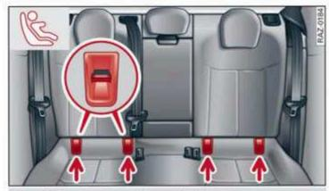
Fig. 61 Rear bench seat: lower LATCH anchors
