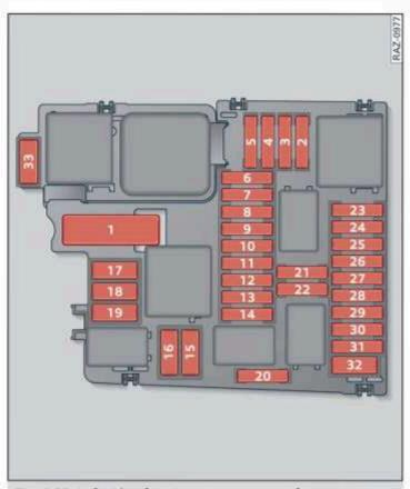
Fig. 165 Left side of engine compartment: fuse assignment
