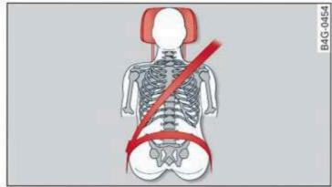
Fig. 51 Correctly-adjusted head restraint
