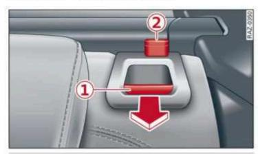
Fig. 66 Outer backrest: release lever and latching indicator with red marking
