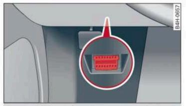
Fig. 166 Driver's side footwell: connection port for the On Board Diagnostic System (OBD)
