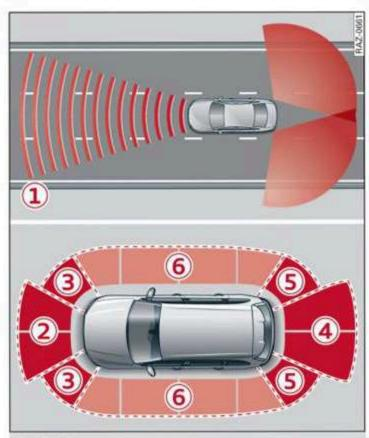
Fig. 75 Sensor detection ranges
