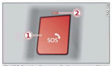
Fig. 113 Front headliner: cover for the emergency call button
