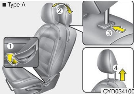
3. Press the headrest release button (3) while pulling the headrest up (4).
