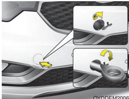
1. Remove the towing hook from the tool case.
