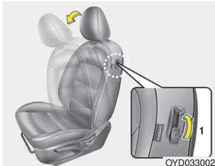
The driver and front passenger's seatback should be tilted to enter the rear seat.
