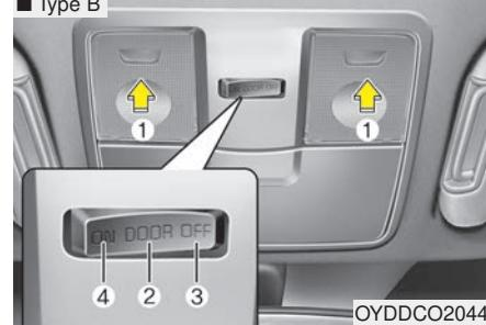
Push the lens (1) to turn the map lamp on or off. This light produces a spot beam for convenient use as a map lamp at night or as a personal lamp for the driver and front passenger.
