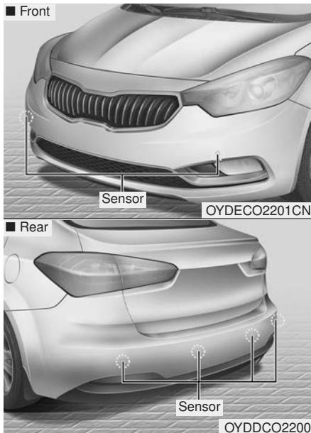
The parking assist system assists the driver during movement of the vehicle by chiming if any object is sensed within the distance of 60 cm (23.62 in) in front or 120 cm (47 in) behind the vehicle.
