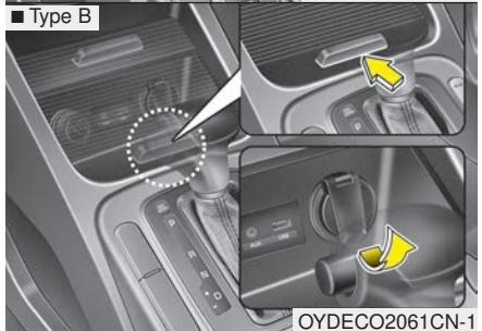
The power outlet is designed to provide power for mobile telephones or other devices designed to operate with vehicle electrical systems. The devices should draw less than 12V, 10A with the engine running.
