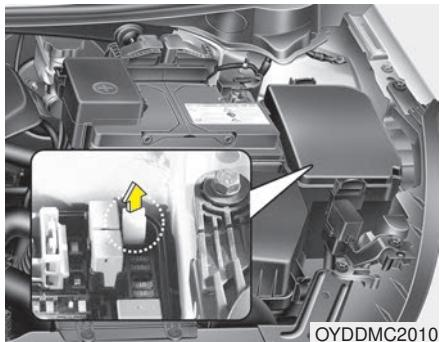
If the headlights or other electrical components do not work and the fuses are OK, check the fuse panel in the engine compartment. If a fuse is blown, it must be replaced.
