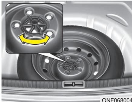
Turn the tire hold-down wing bolt counterclockwise.
