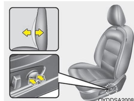
The lumbar support can be adjusted by pressing the lumbar support switch on the side of the driver's seat. Press the front portion of the switch to increase support, or the rear portion of the switch to decrease support.
