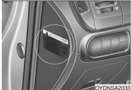
Air bag warning labels, some required by the Canada Motor Vehicle Safety Standards (CMVSS), are attached to the sunvisor to alert the driver and passengers of potential risks of the air bag system.
