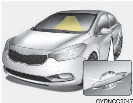
When the headlight (light switch in the headlight or AUTO position) is on and all doors (and trunk) are locked and closed, the headlight, position light and tail light will come on for 15 seconds if any of the below is performed.
