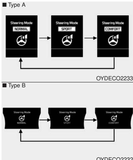
When the steering mode button is pressed, the selected steering mode will appear on the LCD display.
