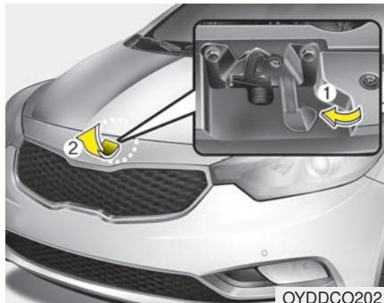
2. Go to the front of the vehicle, raise the hood slightly, push the secondary latch (1) left side and lift the hood (2).
