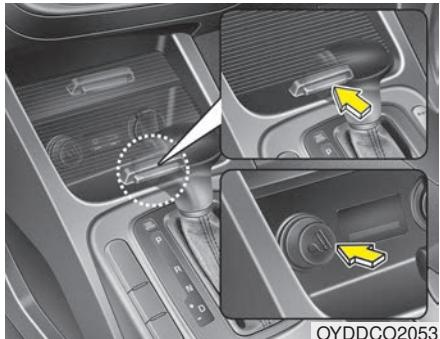
For the cigarette lighter to work, the ignition switch must be in the ACC or ON position.
