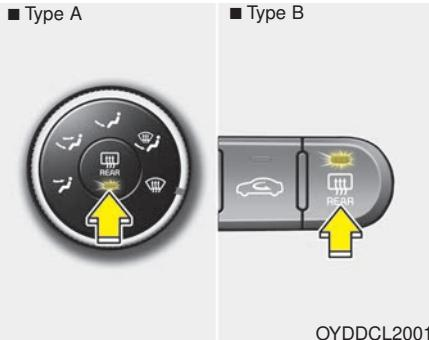
The rear window defroster automatically turns off after approximately 20 minutes or when the ignition switch is turned off. To turn off the defroster manually, press the rear window defroster button again.
