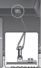
Child restraint hook holders are located on the package tray (4 Door, 2 Door) or the floor behind the rear seat (5 Door).
