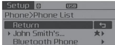
From the paired phone list, select the currently connected device and select [Disconnect] button.
