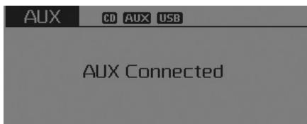
\*AUX mode cannot be started unless there is an external device connected to the AUX terminal.
