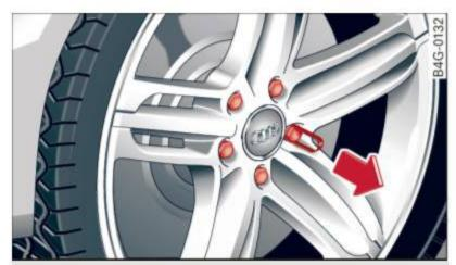
Fig. 168 Changing a wheel: removing the wheel bolt caps
