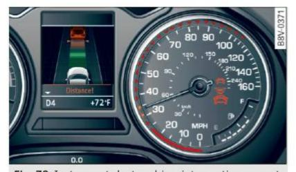
Fig. 79 Instrument cluster: driver intervention request
