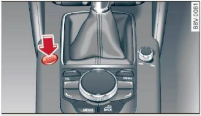
**Fig. 66** Center console: START ENGINE STOP button (with convenience key)
