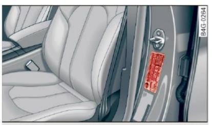
Fig. 156 Tire pressure label: located on driver's side Bpillar
