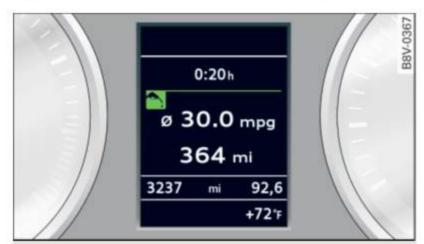
Fig. 13 Instrument cluster: efficiency program (example)
