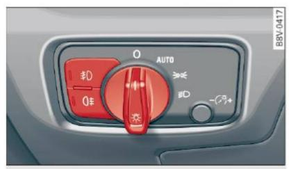
Fig. 29 Instrument panel: light switch
