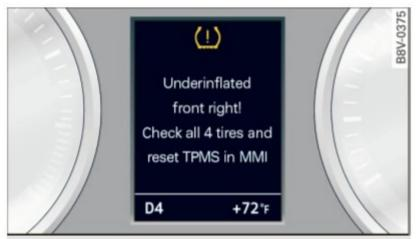
**Fig. 161** Instrument cluster: indicator light with message
