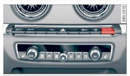
**Fig. 125** Center console: passenger airbag off warning light
