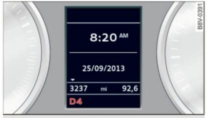
Fig. 91 Instrument cluster: selector lever positions
