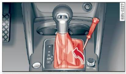
Fig. 96 Selector lever: removing the cover
