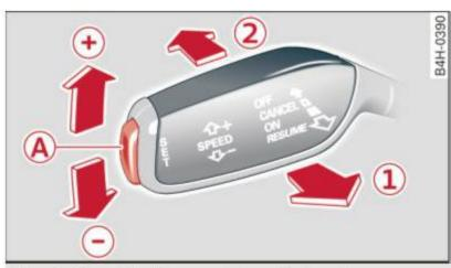
Fig. 69 Operating lever: cruise control system
