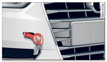
Fig. 181 Right front bumper: towing loop installed
