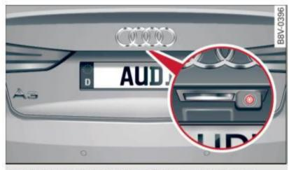
Fig. 104 Rear lid: Location of the rear-view camera
