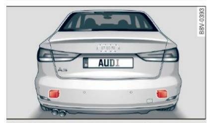
Fig. 88 Rear of the vehicle: sensor positions
