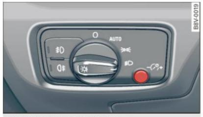
Fig. 34 Instrument illumination
