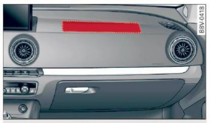
Fig. 123 Location of front passenger's airbag: in the instrument panel
