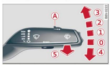
Fig. 36 Windshield wiper lever: operating the front washer system
