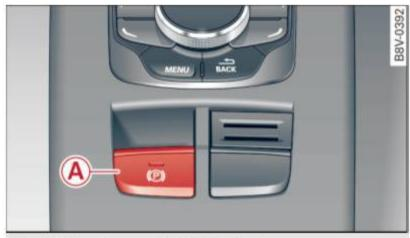
Fig. 68 Center console: Parking brake
