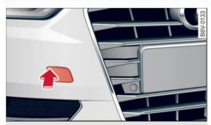
Fig. 180 Right front bumper: removing the cover
