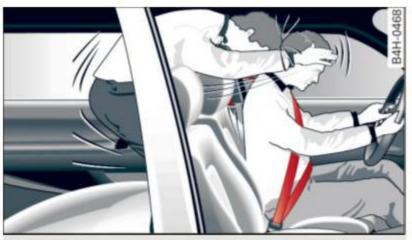
**Fig. 115** A rear passenger not wearing a safety belt will fly forward and strike the driver
