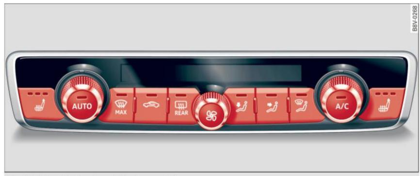
Fig. 61 Automatic climate control system: controls
