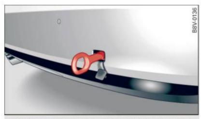
Fig. 183 Right rear towing loop: towing loop installed
