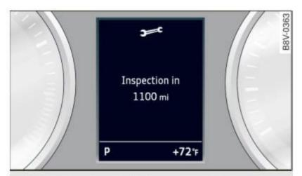
**Fig. 7** Instrument cluster: service interval display (example)
