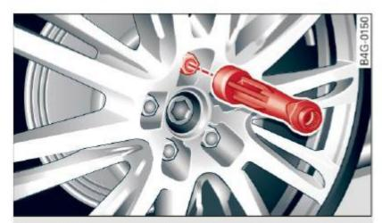
**Fig. 172** Changing a wheel: using the screwdriver handle (with the blade removed) to turn the bolts
