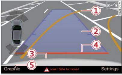
Fig. 105 MMI: aiming at a parking spot
