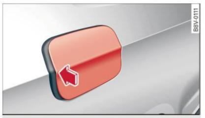
**Fig. 144** Right rear side of the vehicle: opening the fuel filler door
