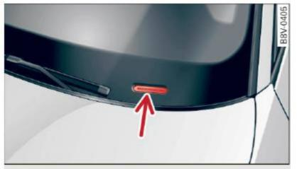
Fig. 187 Vehicle Identification Number (VIN) plate: location on driver's side dash panel
