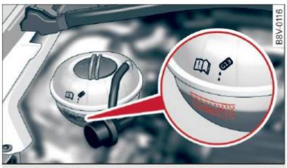
Fig. 152 Engine compartment: markings on the coolant expansion tank
