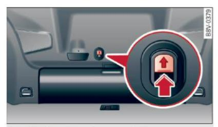
Fig. 162 Rear lid opening: access to the emergency release
