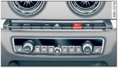
Fig. 143 Upper center console: ESC button
