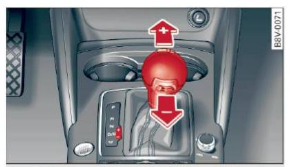
Fig. 94 Center console: manual shifting with the selector lever
