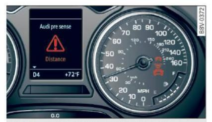
Fig. 80 Instrument cluster: approach warning
