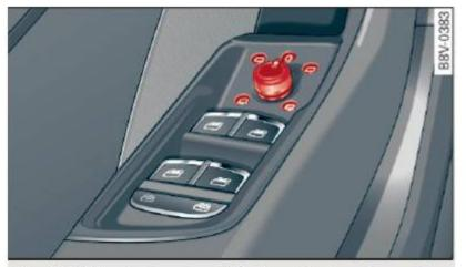
Fig. 38 Driver's door: knob for the exterior mirrors (example)
