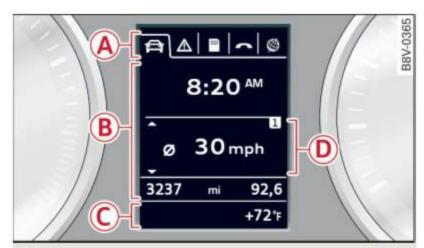
**Fig. 10** Instrument cluster: driver information system (example)
