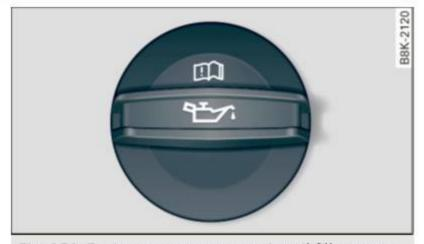
Fig. 151 Engine compartment: engine oil filler opening cover
