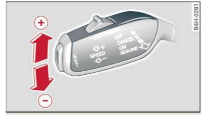
Fig. 76 Operating lever: changing the speed
