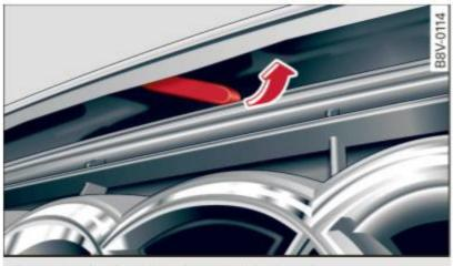
Fig. 148 Rocker switch under the hood
