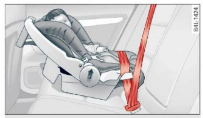
Fig. 133 Schematic overview: rearward-facing infant seat, properly installed on the rear seat
