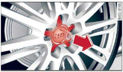
Fig. 167 Changing a wheel: Removing the wheel cover
