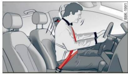
Fig. 116 Driver is correctly restrained in a sudden braking maneuver
