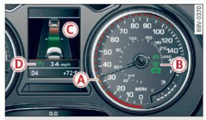
Fig. 75 Instrument cluster: adaptive cruise control
