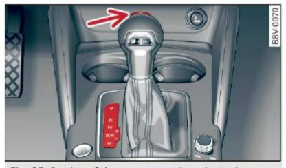
**Fig. 93** Section of the center console: selector lever with interlock button
