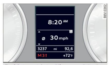
**Fig. 6** Instrument cluster: shift recommendations in tiptronic mode (automatic transmission)
