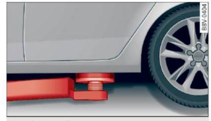
Fig. 186 Rear lifting point
