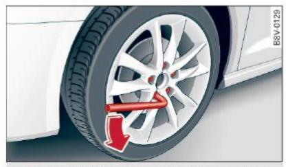
Fig. 169 Changing a wheel: loosening the wheel bolts
