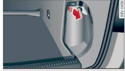
**Fig. 146** Right rear luggage compartment: emergency release
