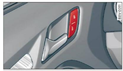
Fig. 22 Driver's door: central locking switch
