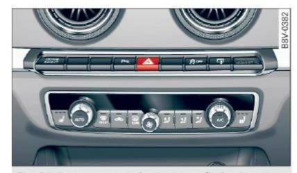
Fig. 30 Instrument panel: emergency flasher button
