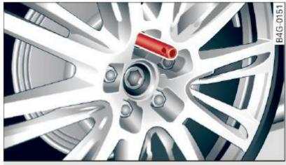
Fig. 173 Changing a wheel: alignment pin inside the top hole
