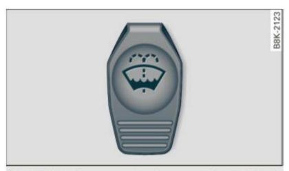
Fig. 155 Engine compartment: cover on the windshield and headlight\* washer fluid reservoir
