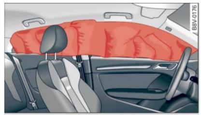
Fig. 131 Illustration of principle: Inflated side curtain airbags on the left side
