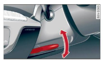
Fig. 64 Steering column: steering column adjustment lever
