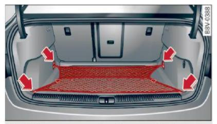
Fig. 57 Luggage compartment: cargo net\* unhooked
