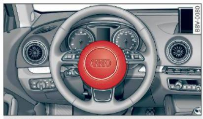
Fig. 122 Location of driver airbag: in steering wheel
