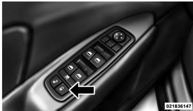
Power Door Lock Switch Location
