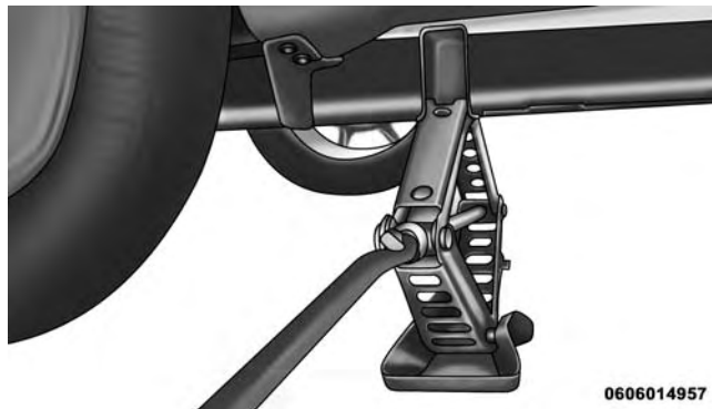
Rear Jack Engaged With Jack Handle
