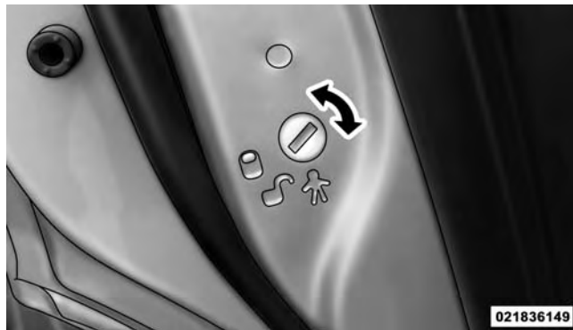
Child-Protection Door Lock Function
