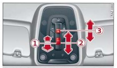
Fig. 36 Headliner: panoramic glass roof and sunshade\* buttons (shown on the Avant/allroad as an example)
