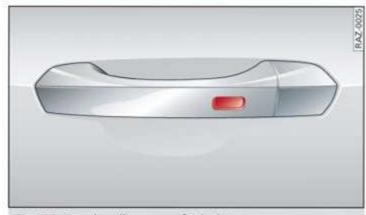
Fig. 25 Door handle: sensor for locking
