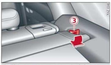
Fig. 72 Luggage compartment: removing the luggage compartment cover
