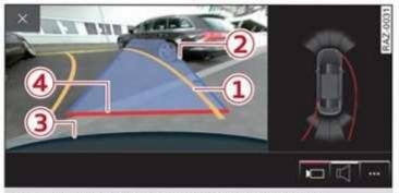
Fig. 129 Upper display: aiming at a parking space
