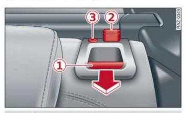
Fig. 73 Outer backrest: release lever, latching indicator with red marking and lock\*
