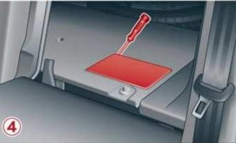
Fig. 192 Left side of cockpit: cover (3), luggage compartment floor: fuse panel cover (4)
