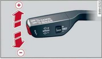
Fig. 105 Operating lever: changing the speed
