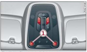
Fig. 41 Headliner: interior lighting
