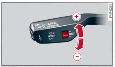
Fig. 110 Operating lever: setting the distance
