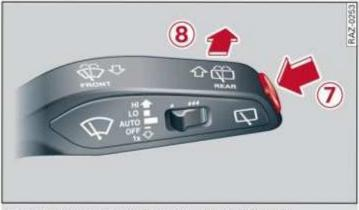
Fig. 47 Lever: rear window wiper (Avant/allroad)
