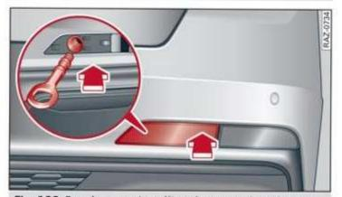
Fig. 190 Rear bumper: installing the towing loop (version 2)
