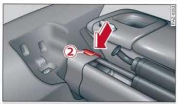
Fig. 78 Luggage compartment: removing the partition net
