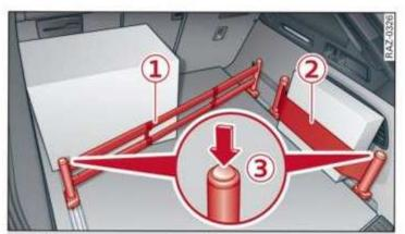
Fig. 80 Luggage compartment: securing attachments
