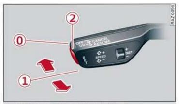
Fig. 104 Lever: using adaptive cruise assist
