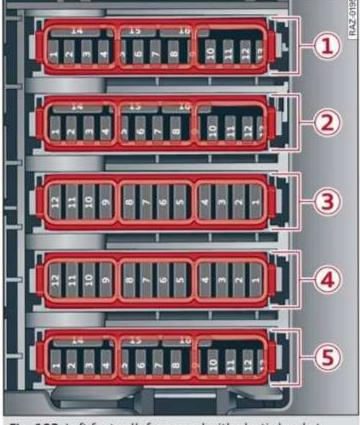
Fig. 193 Left footwell: fuse panel with plastic bracket
