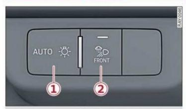
Fig. 37 Instrument panel: light button module
