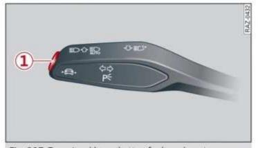
Fig. 117 Turn signal lever: button for lane departure warning and lane guidance for adaptive cruise assist\*
