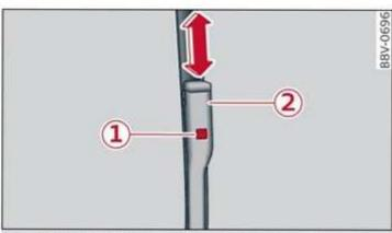
Fig. 48 Windshield wipers: changing the wiper blades
