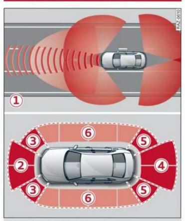
Fig. 91 Sensor coverage area
