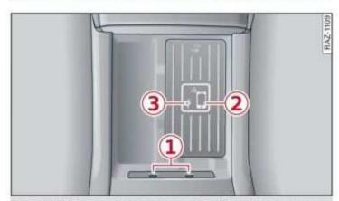
Fig. 140 Storage compartment under the center armrest: Audi phone box with connections
