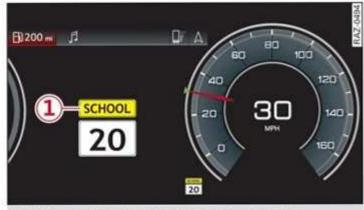
Fig. 97 Instrument cluster: traffic sign recognition
