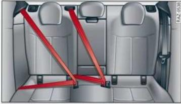
Fig. 68 Rear bench seat: securing unused safety belts
