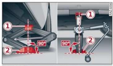
Fig. 183 Sill: positioning the vehicle jack
