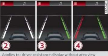
Applies to: driver assistance display without area view Fig. 118 Instrument cluster: lane departure warning
