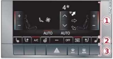
Fig. 84 Center console: lower display and switch panel
