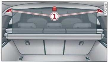
Fig. 77 Luggage compartment: installing the partition net
