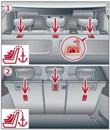
Fig. 66 Version 1 rear shelf / Version 2 rear backrest: top tether anchors for securing a child safety seat with an upper strap
