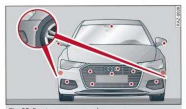
Fig. 93 Front area: sensors and cameras
