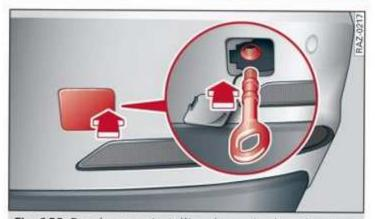
Fig. 189 Rear bumper: installing the towing loop (version 1)
