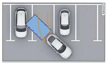
Fig. 127 Orientation line display when parking
