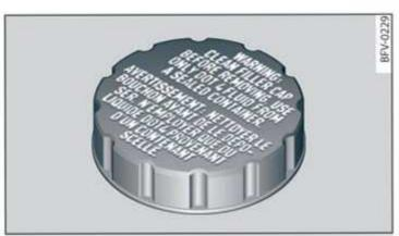
Fig. 168 Engine compartment: cap on brake fluid reservoir
