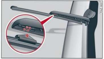
Fig. 49 Rear window wiper: installing the wiper blade
