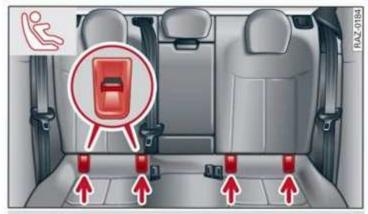
Fig. 65 Rear bench seat: lower LATCH anchors
