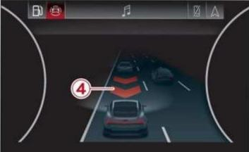
Applies to: vehicles with adaptive cruise assist: Fig. 116 Instrument cluster: distance warning with or without area view
