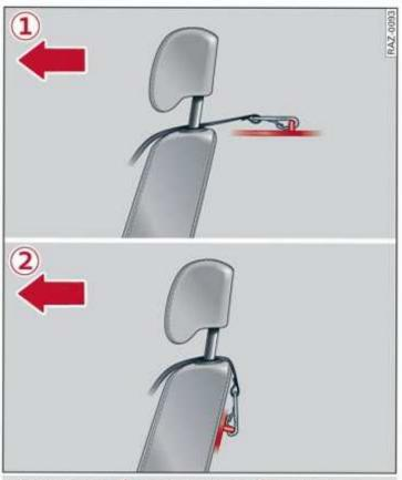
Fig. 67 Version 1 rear shelf / Version 2 rear backrest: securing the upper strap on the top tether anchor
