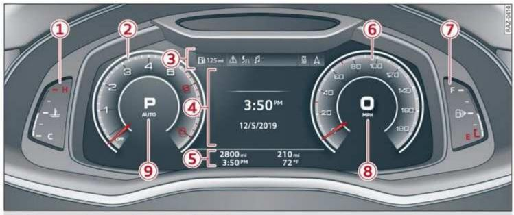
Fig. 3 Instrument cluster overview (Audi virtual cockpit)
