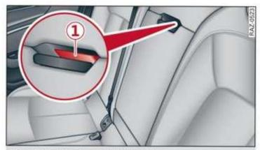
Fig. 75 Center backrest: release lever
