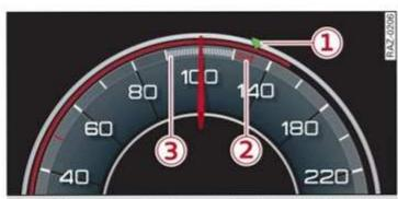
Fig. 109 Instrument cluster: speedometer: predictive control display
