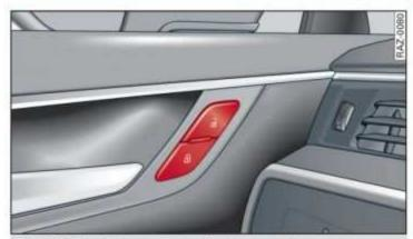
Fig. 21 Driver's door: central locking switch
