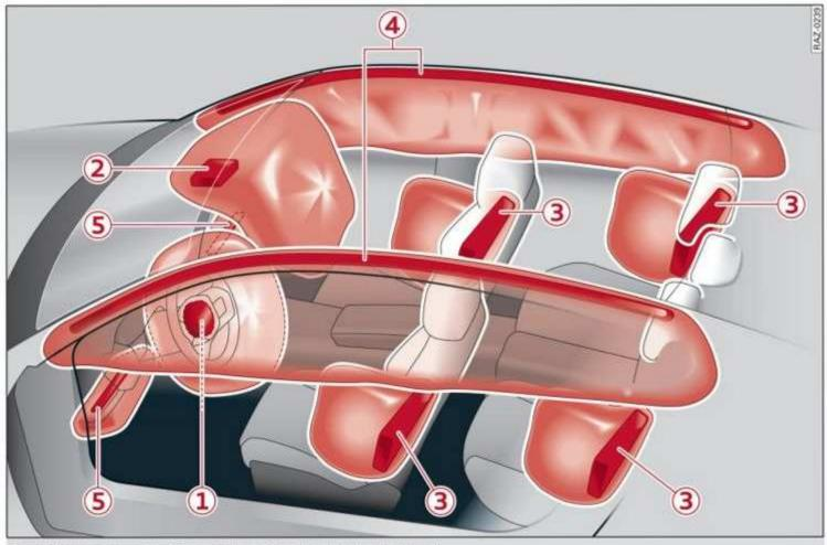
Fig. 63 Airbag overview image (enlarged section: deployed airbags)
