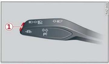
Fig. 106 Turn signal lever: button for lane guidance and lane departure warning
