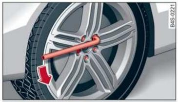
Fig. 181 Wheel: loosening the wheel bolts
