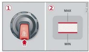
Fig. 167 Engine compartment - Coolant expansion tank (diagram): 1) cover with release button; 2) markings
