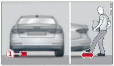
Fig. 30 Vehicle rear: foot motion (example)
