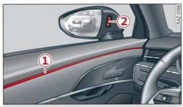
Fig. 122 Front door: warning strip
