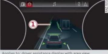
Applies to: driver assistance display with area view Fig. 114 Instrument cluster: narrow area
