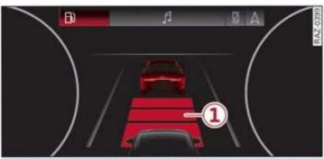
Applies to: driver assistance display without area view Fig. 107 Instrument cluster: brake intervention request
