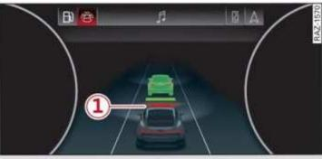
Applies to: driver assistance display with area view Fig. 113 Instrument cluster: safe start monitor
