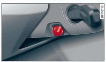
Fig. 54 Steering column: switch for adjusting the steering
