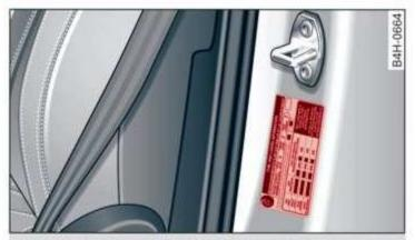
Fig. 173 Driver's side B-pillar: tire pressure label
