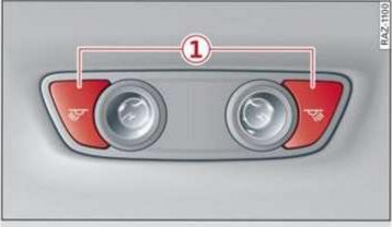
Fig. 42 Headliner: reading lights
