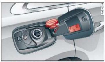
Fig. 161 Fuel filler door with attached fuel cap
