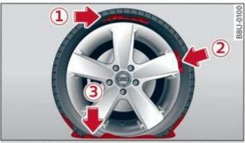
Fig. 176 Tire: tire damage that cannot be repaired
