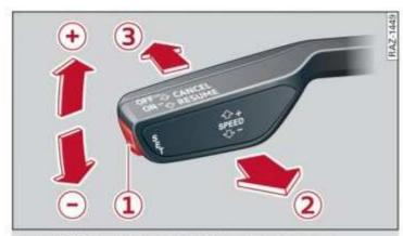
Fig. 100 Operating lever: switching the system on
