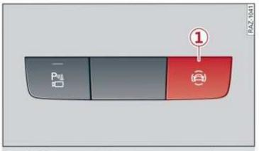
Fig. 95 Center console: driver assistance systems button
