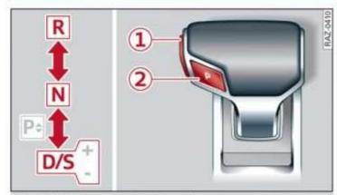
Fig. 87 Center console: selector lever
