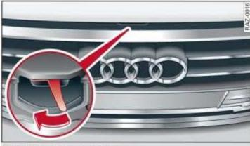
Fig. 163 Unlocked hood: lever
