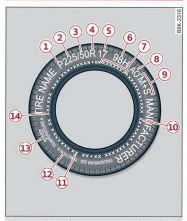
Fig. 171 Tire designations on the sidewall
