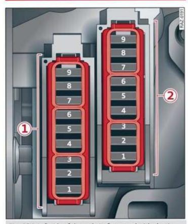
$\label{eq:Fig. 194} \textbf{ Left side of the cockpit: fuse panel with plastic clip}$
