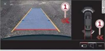
Fig. 132 Upper display: rear cross-traffic assist display
