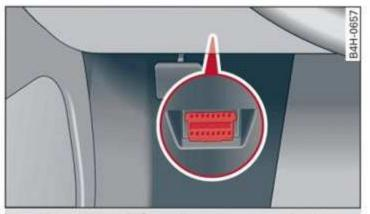
Fig. 196 Driver's side footwell: connection port for the On Board Diagnostic System (OBD)
