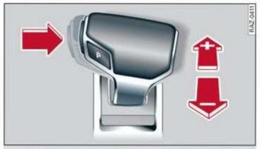
Fig. 88 Center console: shifting manually with the selector lever
