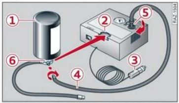
Fig. 177 Components of the tire mobility kit
