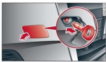
Fig. 188 Front bumper: installing the towing loop
