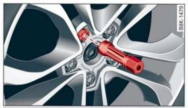
Fig. 184 Wheel: internal hex socket to turn the wheel bolts
