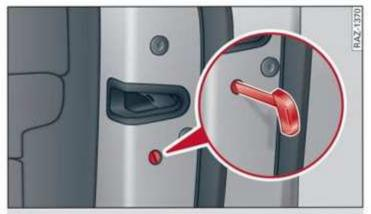
Fig. 23 Door: mechanically locking
