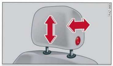
Fig. 56 Front seat: adjusting the head restraint
