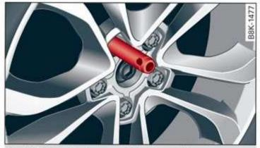
Fig. 185 Wheel: alignment pin in the top hole
