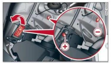
Fig. 186 Engine compartment: connectors for jump start cables or a charger
