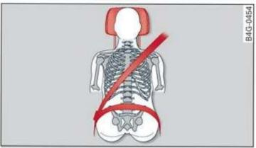
Fig. 55 Correctly-adjusted head restraint
