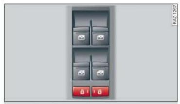
Fig. 34 Driver's door: controls
