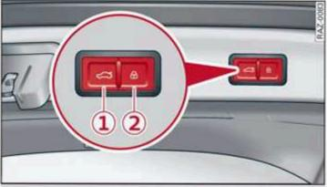
Fig. 30 Luggage compartment lid: 1 closing button\*, 2 lock button\* (vehicles with convenience key\*)
