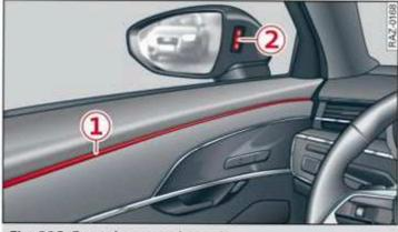
Fig. 118 Front door: warning strip
