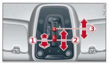
Fig. 37 Headliner: panoramic glass roof and sunshade\* buttons (shown on the Avant/allroad as an example)
