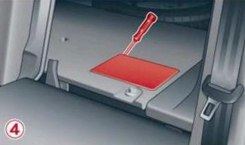
Fig. 188 Left side of cockpit: cover (3), luggage compartment floor: fuse panel cover (4)
