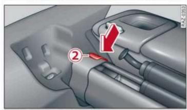
Fig. 79 Luggage compartment: removing the partition net
