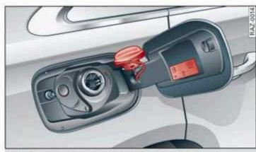
Fig. 157 Fuel filler door with attached fuel cap
