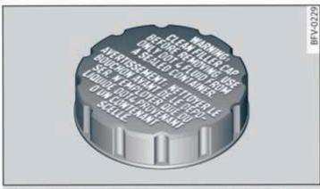
Fig. 164 Engine compartment: cap on brake fluid reservoir
