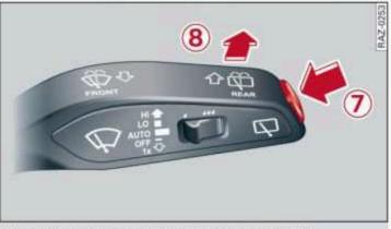
Fig. 48 Lever: rear window wiper (Avant/allroad)
