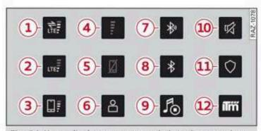
Fig. 14 Upper display: common symbols in the status bar
