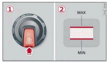
Fig. 163 Engine compartment - Coolant expansion tank (diagram): 1) cover with release button; 2) markings
