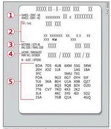
Fig. 193 Vehicle identification label
