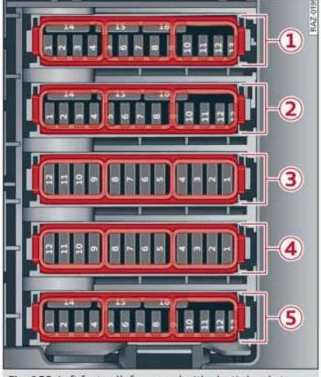
Fig. 189 Left footwell: fuse panel with plastic bracket
