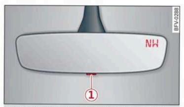
Fig. 51 Rearview mirror: digital compass is switched on
