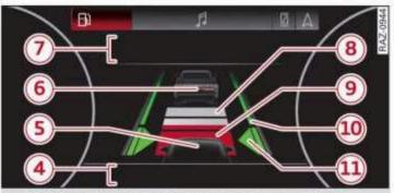
Fig. 103 Instrument cluster: driver assistance display
