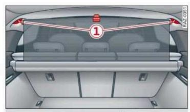
Fig. 78 Luggage compartment: installing the partition net
