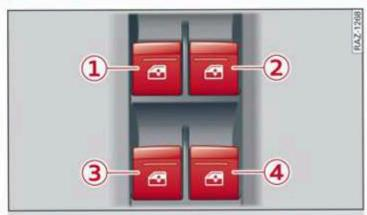
Fig. 36 Driver's door: power window switch
