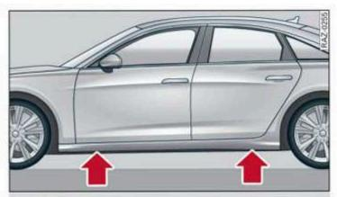
Fig. 178 Sill panels: markings
