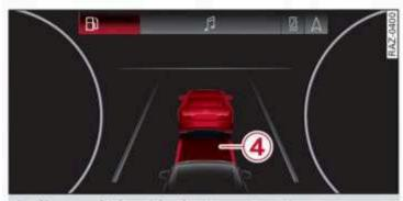
Applies to: vehicles with adaptive cruise assist: Fig. 113 Instrument cluster: distance warning
