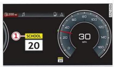
Fig. 97 Instrument cluster: traffic sign recognition
