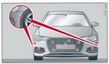
Fig. 94 Front area: sensors and cameras
