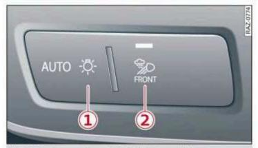
Fig. 38 Instrument panel: light button module
