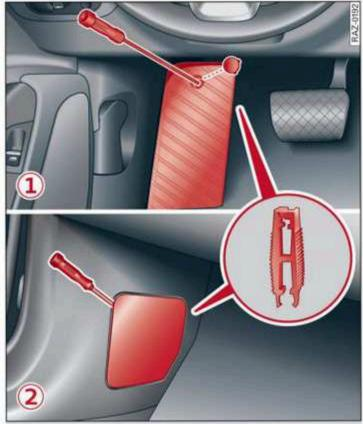
Fig. 187 Driver's side footwell (left-hand drive vehicles): footrest (1), front passenger's side footwell (right-hand drive vehicles): cover (2)
