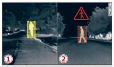
Fig. 99 Instrument cluster: pedestrian marking and warning
