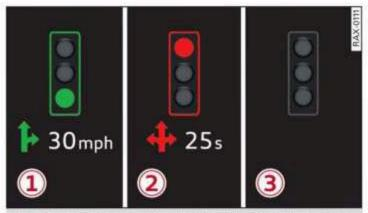
Fig. 98 Instrument cluster: traffic light information display
