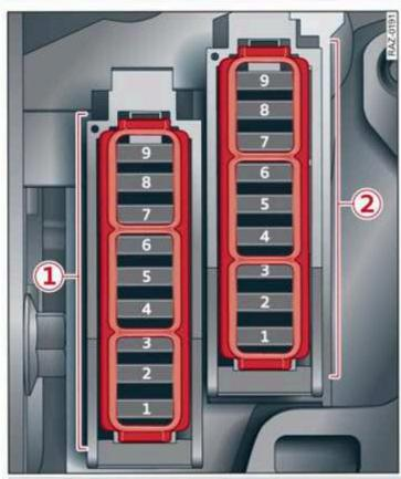
Fig. 190 Left side of the cockpit: fuse panel with plastic clip
