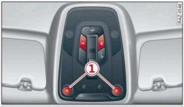
Fig. 42 Headliner: interior lighting
