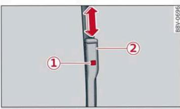
Fig. 49 Windshield wipers: changing the wiper blades
