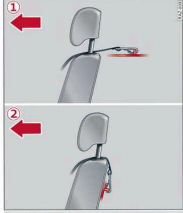
Fig. 68 Version 1 rear shelf / Version 2 rear backrest: securing the upper strap on the top tether anchor
