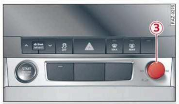
Fig. 19 MMI On/Off knob with joystick function
