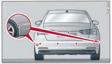
Fig. 95 Rear area: sensors and cameras
