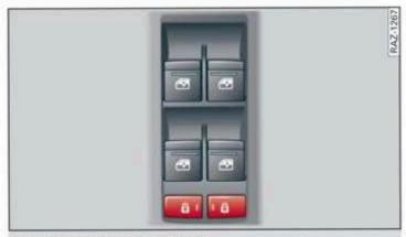
Fig. 35 Driver's door: controls
