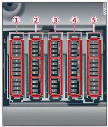
Fig. 191 Luggage compartment floor: fuse panel with plastic clip
