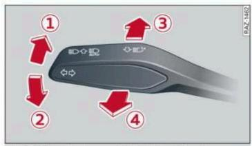
Fig. 39 Operating lever: switching the light functions on and off
