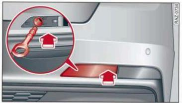
Fig. 186 Rear bumper: installing the towing loop (version 2)
