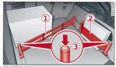
Fig. 81 Luggage compartment: securing attachments
