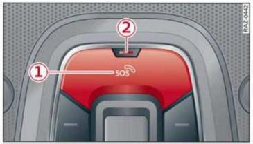
Fig. 139 Front headliner: cover for the emergency call but-
