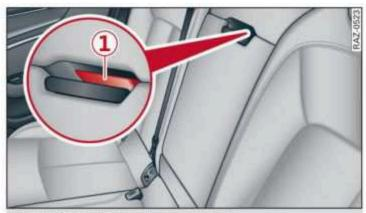
Fig. 76 Center backrest: release lever
