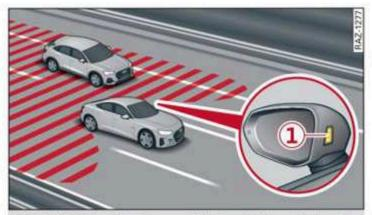
Fig. 116 Driving situations and displays in the exterior mirror
