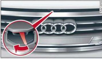
Fig. 159 Unlocked hood: lever
