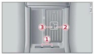
Fig. 136 Storage compartment under the center armrest: Audi phone box with connections
