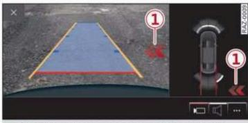
Fig. 128 Upper display: rear cross-traffic assist display
