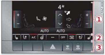
Fig. 85 Center console: lower display and switch panel
