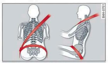
Fig. 59 Lap/shoulder belt positioning
