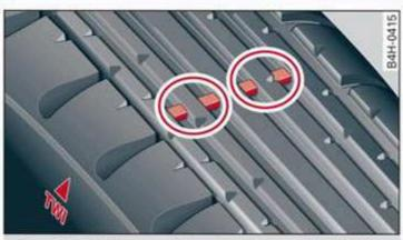
Fig. 168 Tire profile: treadwear indicator
