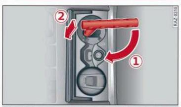
Fig. 91 Center console: releasing the parking lock using the emergency release
