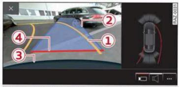
Fig. 125 Upper display: aiming at a parking space
