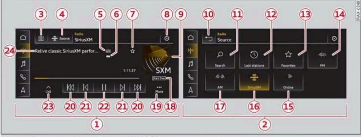
Fig. 151 Upper display: left side: playback view of radio functions, right side: sources
