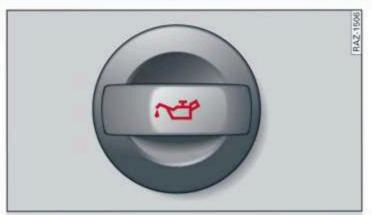
Fig. 162 Engine compartment: engine oil filling opening cover (example)
