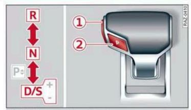
Fig. 88 Center console: selector lever
