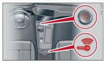
Fig. 87 Center console: starting the engine
