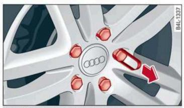
Fig. 175 Wheel: wheel bolts with caps
