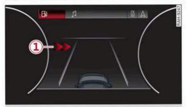
Fig. 120 Instrument cluster: directional display from the intersection assistant
