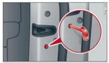
Fig. 24 Door: mechanically locking
