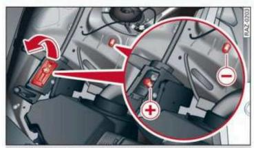
Fig. 165 Engine compartment: connectors for a charger or jump start cables
