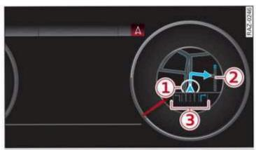
Fig. 146 Instrument cluster: default view: turning maneuver when route guidance has started
