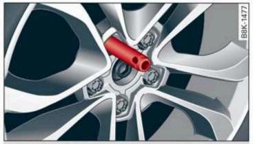
Fig. 181 Wheel: alignment pin in the top hole
