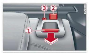
Fig. 74 Outer backrest: release lever, latching indicator with red marking and lock\*
