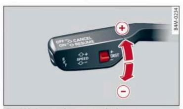
Fig. 109 Operating lever: setting the distance
