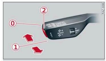
Fig. 110 Lever: using adaptive cruise assist
