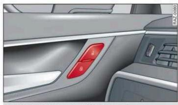
Fig. 20 Driver's door: central locking switch
