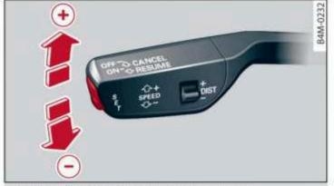
Fig. 105 Operating lever: changing the speed
