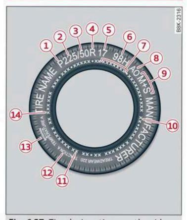
Fig. 167 Tire designations on the sidewall
