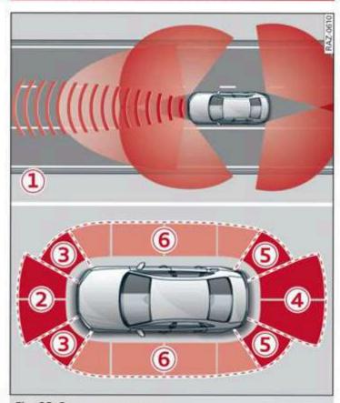
Fig. 92 Sensor coverage area
