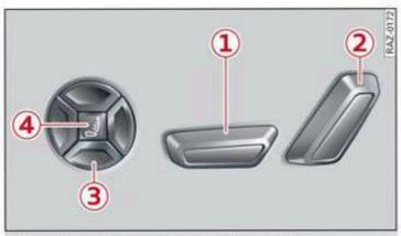
Fig. 53 Front seat: seat adjustment buttons
