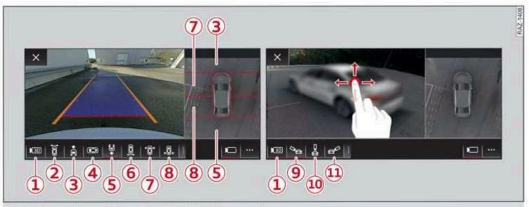
Fig. 126 Upper display: left: rear view. Right side: 3D surroundings.
