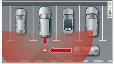
Fig. 127 Sensor detection range for rear cross-traffic assist
