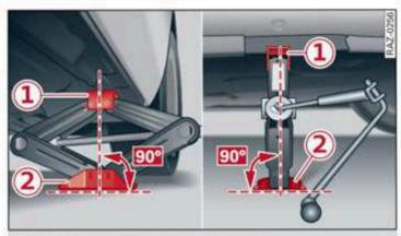
Fig. 179 Sill: positioning the vehicle jack
