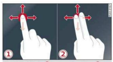
Fig. 11 Touch display: 1 dragging with one finger, 2 dragging with two fingers
