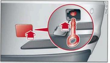
Fig. 185 Rear bumper: installing the towing loop (version 1)
