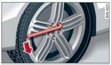
Fig. 177 Wheel: loosening the wheel bolts
