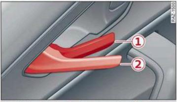
Fig. 22 Door handle: 1 standard operation, 2 emergency operation
