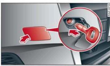
Fig. 184 Front bumper: installing the towing loop
