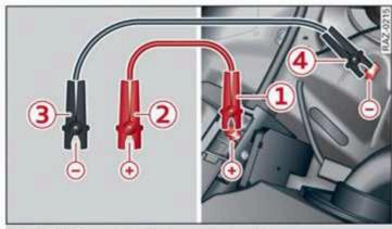
Fig. 183 Connecting the jump start cables
