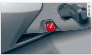
Fig. 55 Steering column: switch for adjusting the steering
