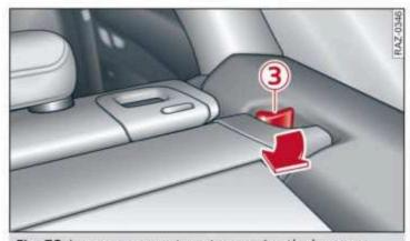
Fig. 73 Luggage compartment: removing the luggage compartment cover
