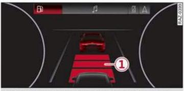
Fig. 107 Instrument cluster: brake intervention request
