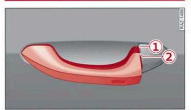
Fig. 21 Door handle: 1 standard operation, 2 emergency operation
