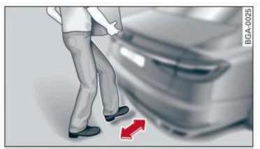
Fig. 31 Vehicle rear: foot motion (example)
