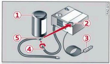
Fig. 173 Components of the tire mobility kit
