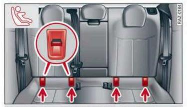
Fig. 66 Rear bench seat: lower LATCH anchors
