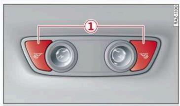
Fig. 43 Headliner: reading lights
