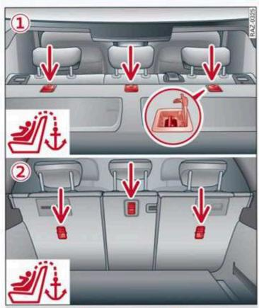
Fig. 67 Version 1 rear shelf / Version 2 rear backrest: top tether anchors for securing a child safety seat with an upper strap
