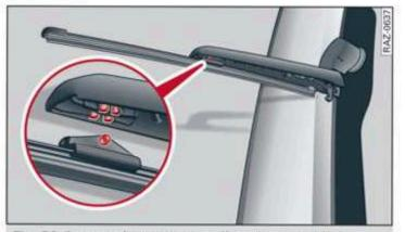
Fig. 50 Rear window wiper: installing the wiper blade
