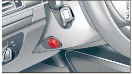
Fig. 76 Switch for adjusting the steering wheel position
