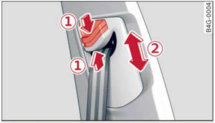
Fig. 150 Safety belt height adjustment for the front seats – loop-around fittings
