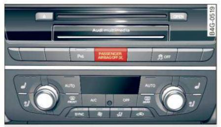
Fig. 154 Section from the instrument panel: PASSENGER AIR BAG OFF light
