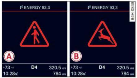
Fig. 111 Instrument cluster: (A) pedestrian warning/(B) wild animal warning, when the night vision assist image is not selected in the instrument cluster display
