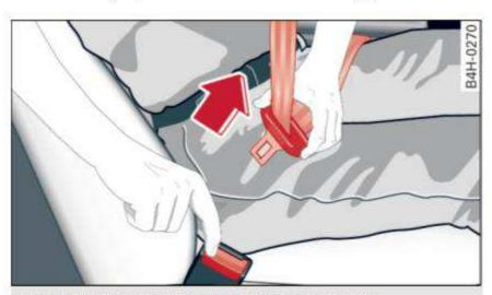
Fig. 149 Releasing the tongue from the buckle
