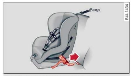
Fig. 169 Lower anchorages: proper mounting
