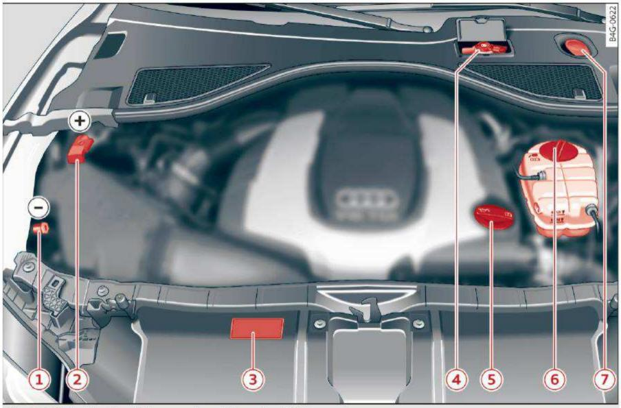
Fig. 179 Typical location of the reservoir and the engine oil filler opening
