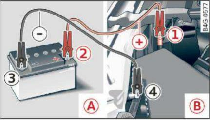
Fig. 206 Jump starting with the battery of another vehicle:
