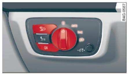
Fig. 36 Instrument panel: light switch with all-weather lights
