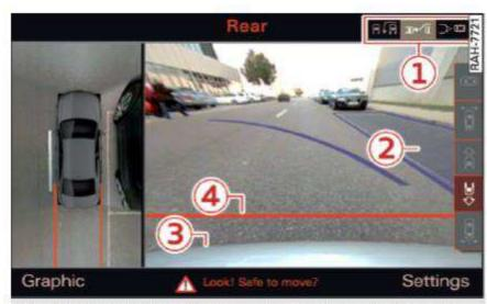
Fig. 134 Infotainment: blue surfaces aligned in the parking space
