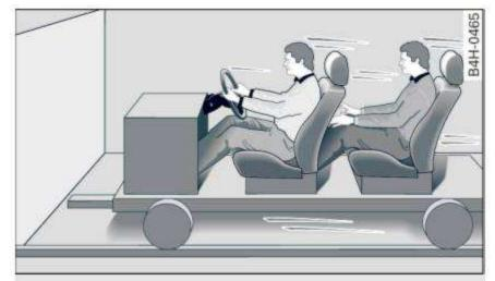
Fig. 141 Unbelted occupants in a vehicle heading for a wall
