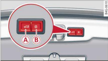
Fig. 26 Luggage compartment lid: (A) closing button, (B) lock button (vehicles with convenience key\*)
