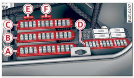
Fig. 204 Luggage compartment: fuse panel with plastic bracket
