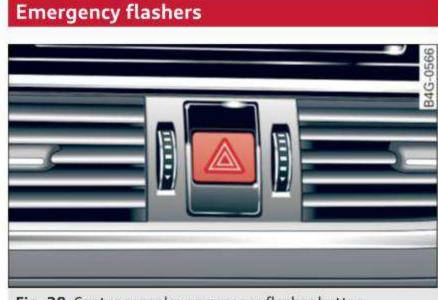
Fig. 38 Center console: emergency flasher button
