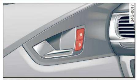
Fig. 19 Driver's door: central locking switch
