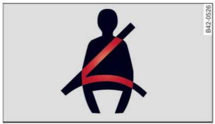
Fig. 140 Safety belt warning light in the instrument cluster - enlarged
