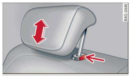
Fig. 53 Rear seat: adjusting the head restraint
