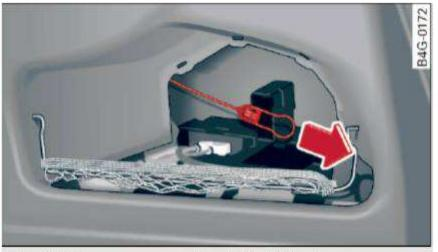
Fig. 175 Luggage compartment: fuel filler door emergency release
