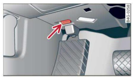
Fig. 176 Footwell on left side of the vehicle: connection port for the On-Board Diagnostic System (OBD)
