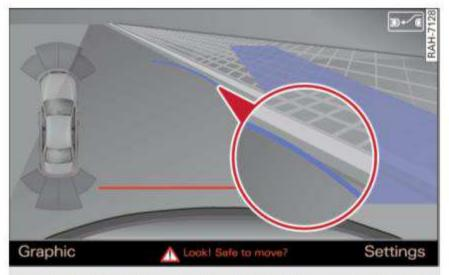
Fig. 123 Infotainment: contact of the blue curved line with the curb
