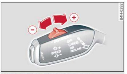
Fig. 96 Operating lever: setting the distance
