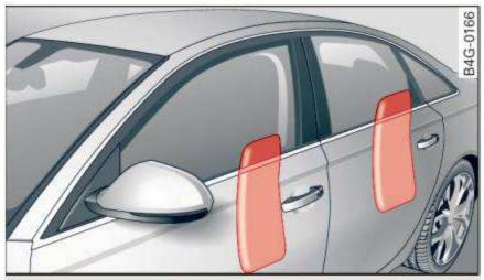
Fig. 158 Inflated side airbags on left side of vehicle, rear side airbag
