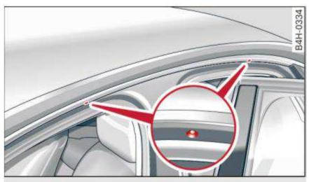
Fig. 64 Attachment points for the roof rack
