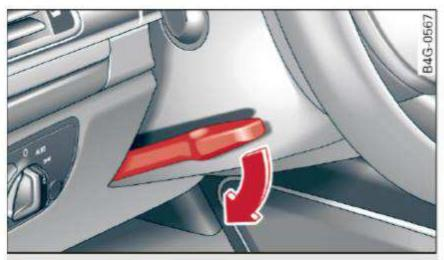
Fig. 75 Lever on the steering column
