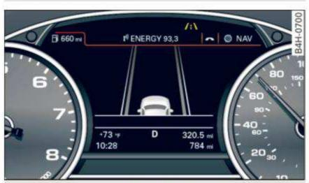
Fig. 102 Instrument cluster: active lane assist is switched on but not ready to provide warnings
