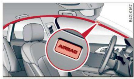
Fig. 159 Side curtain airbags, driver's side: side curtain airbag location
