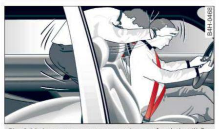
Fig. 144 A rear passenger not wearing a safety belt will fly forward and strike the driver
