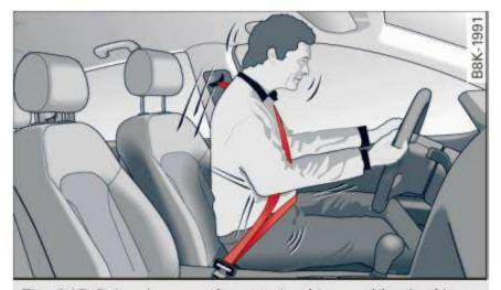
Fig. 145 Driver is correctly restrained in a sudden braking maneuver
