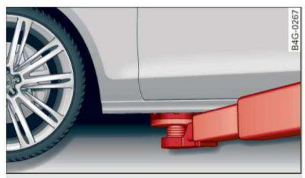
Fig. 212 Front lifting point
