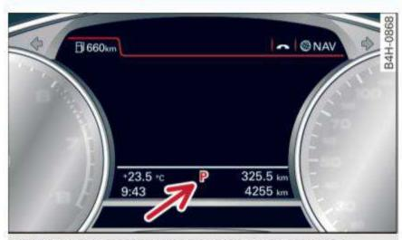
Fig. 82 Instrument cluster: selector lever positions
