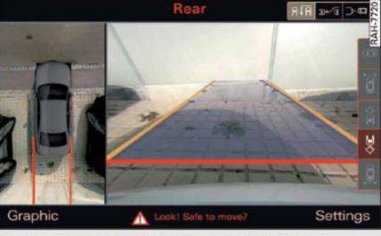
Fig. 133 Infotainment system: aligning the vehicle
