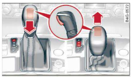
Fig. 83 Selector lever lock
