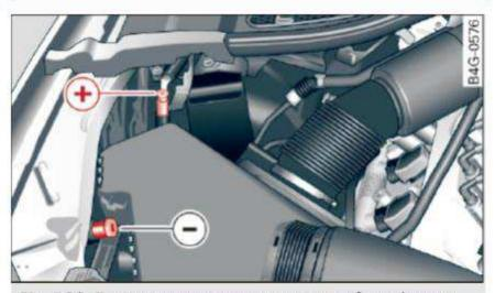
Fig. 183 Engine compartment: connectors for a charger and jump start cables
