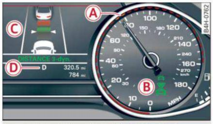
Fig. 93 Instrument cluster: adaptive cruise control
