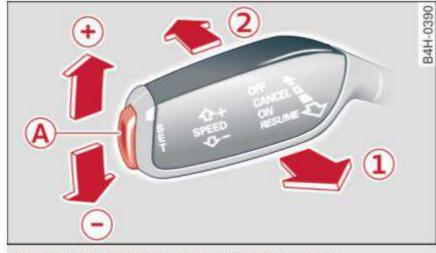
Fig. 87 Operating lever: cruise control system
