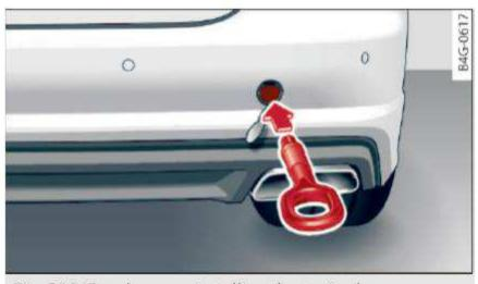
Fig. 210 Rear bumper: installing the towing loop
