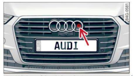
Fig. 112 Front of the vehicle: night vision assist camera
