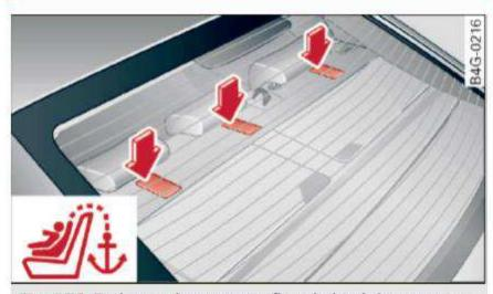
Fig. 170 Tether anchors: recess flaps behind the rear seatbacks
