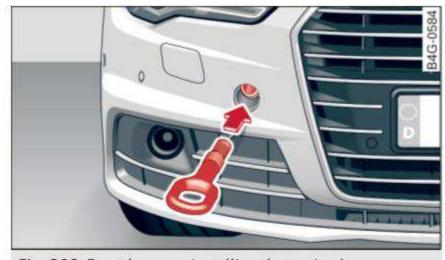
Fig. 208 Front bumper: installing the towing loop
