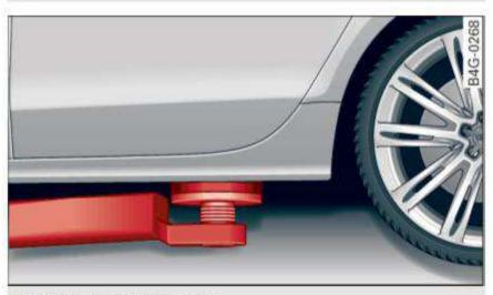
Fig. 213 Rear lifting point
