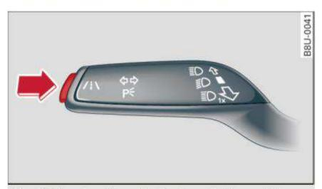
Fig. 99 Turn signal lever: button for active lane assist
