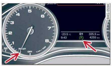
**Fig. 79** Instrument cluster: engine switched off (stop phase)
