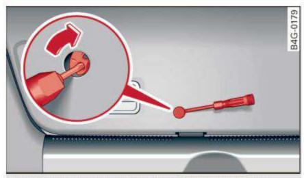
Fig. 28 Inner luggage compartment lid: access to the emergency release
