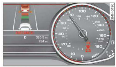
Fig. 97 Instrument cluster: request for driver intervention
