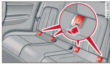
Fig. 167 Lower anchorages, covers marked
