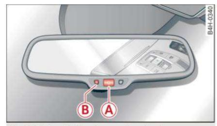
Fig. 43 Automatic dimming rearview mirror\*
