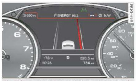
Fig. 101 Instrument cluster: active lane assist is switched on and providing warnings
