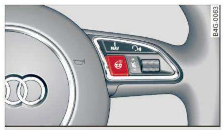
Fig. 74 Steering wheel: steering wheel heating button
