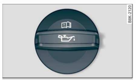
Fig. 180 Engine compartment: engine oil filler opening cover
