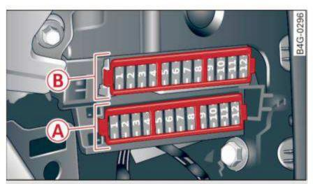
Fig. 203 Front passenger side cockpit: fuse panel with plastic bracket
