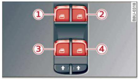
Fig. 31 Driver's door: power window controls
