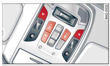
Fig. 39 Front headliner: interior lighting controls
