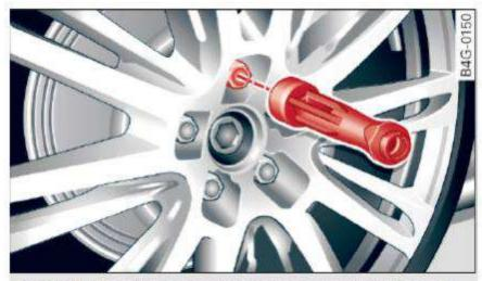
Fig. 198 Changing a wheel: using the screwdriver handle (with the blade removed) to turn the bolts
