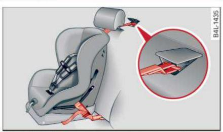
Fig. 171 Tether strap: proper routing and mounting
