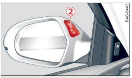
Fig. 104 Display on the exterior mirror
