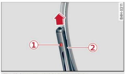
Fig. 48 Removing windshield wiper blades
