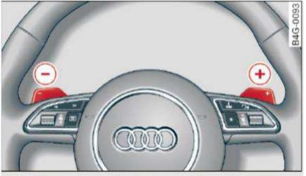
Fig. 85 Steering wheel: shifting manually with the shift paddles\*
