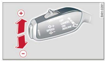
Fig. 94 Operating lever: changing the speed
