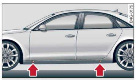
Fig. 195 Sill panels: markings
