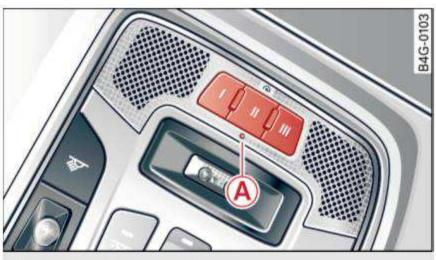
Fig. 35 Headliner: controls
