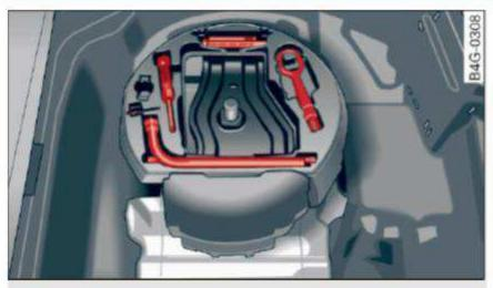
Fig. 191 Luggage compartment: vehicle tool kit
