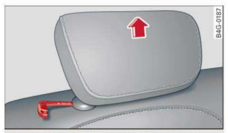
Fig. 54 Rear seat: removing the head restraint, release point
