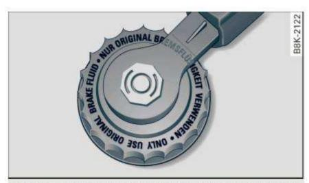
Fig. 182 Engine compartment: cap on brake fluid reservoir
