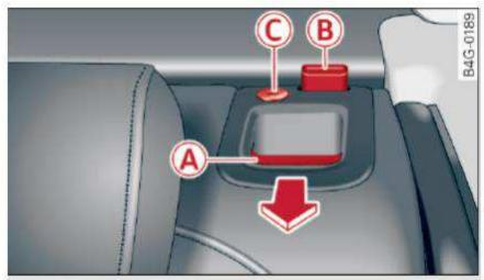
Fig. 65 Backrest: release lever, securing knob and lock\*
