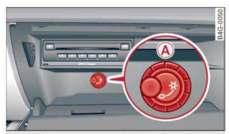
Fig. 63 Glove compartment: switching cooling mode on/
