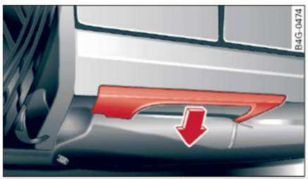
Fig. 197 Sill: removing the cover
