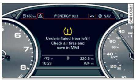
Fig. 189 Instrument cluster: indicator light with message
