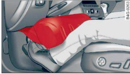
Fig. 156 Inflated airbags protecting in a frontal collision
