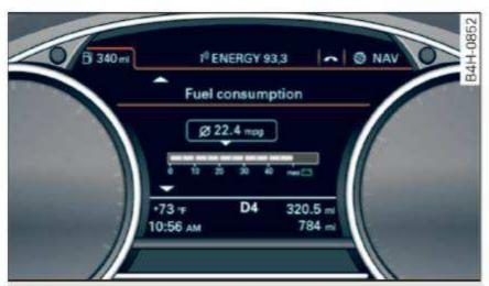
Fig. 8 Instrument cluster: fuel consumption display
