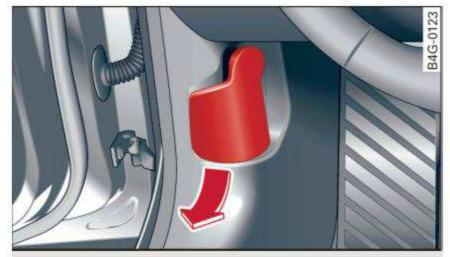
Fig. 177 Driver footwell: release lever
