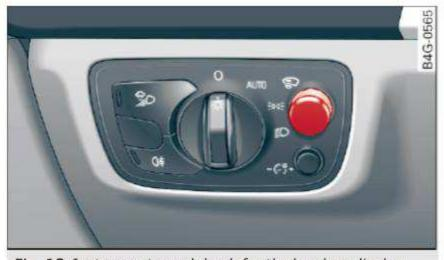
Fig. 13 Instrument panel: knob for the head-up display
