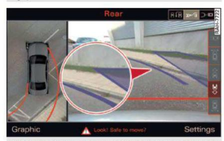
Fig. 135 Infotainment: contact of the blue curved line with the curb
