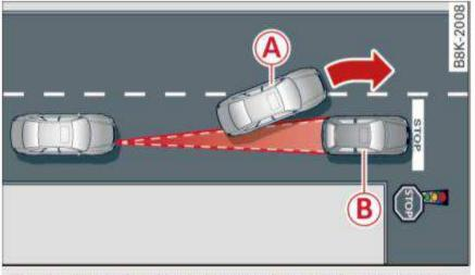
Fig. 91 Example: object changing lanes and stationary object
