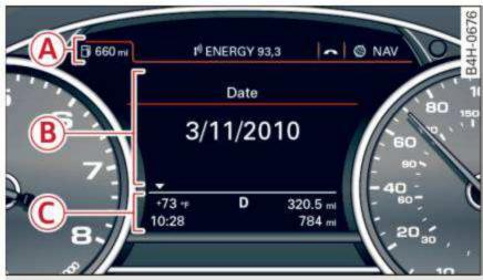
Fig. 4 Driver information system in the instrument cluster
