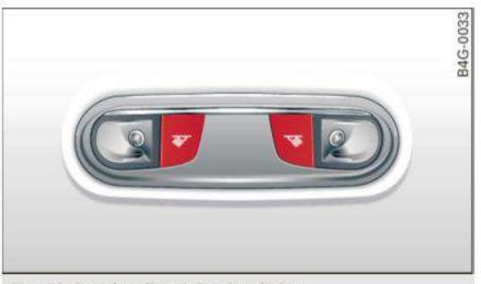
Fig. 40 Rear headliner: Reading light
