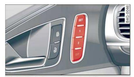
Fig. 55 Driver's door: memory function buttons
