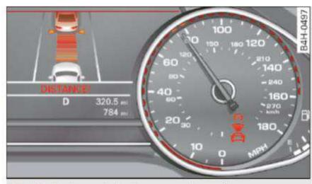
Fig. 98 Instrument cluster: approach warning
