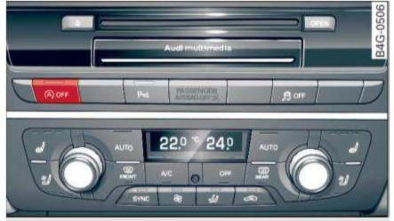
Fig. 80 Center console: Start/Stop system button
