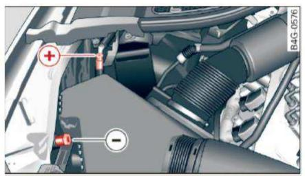
Fig. 205 Engine compartment: connectors for jump start cables and charger
