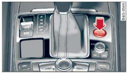
Fig. 77 Center console: START ENGINE STOP button
