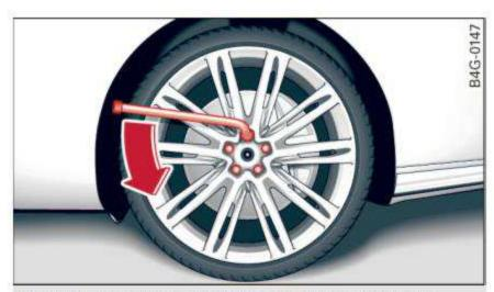
Fig. 194 Changing a wheel: loosening the wheel bolts
