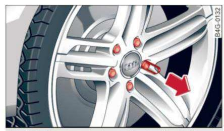
Fig. 193 Changing a wheel: removing the wheel bolt caps
