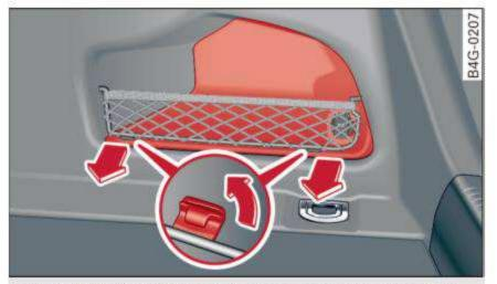
Fig. 174 Right side trim in the luggage compartment: removing the trim
