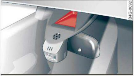
Fig. 100 Windshield: camera window for active lane assist
