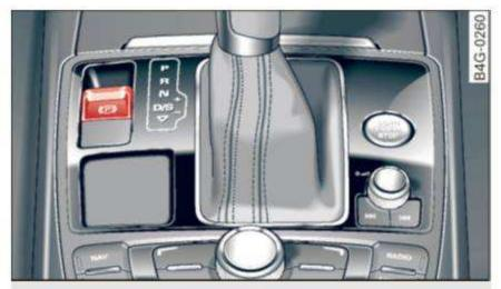
Fig. 81 Center console: parking brake
