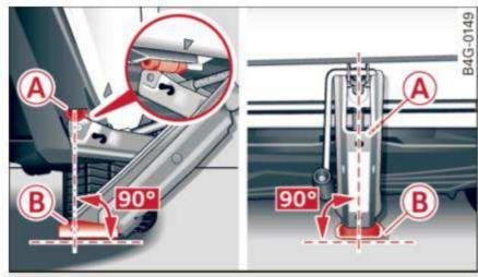
Fig. 196 Sill: positioning the vehicle jack
