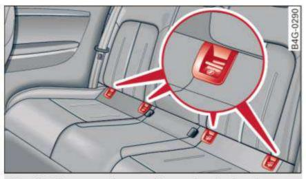
Fig. 168 Rear seats: lower anchorage bracket locations
