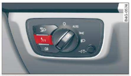
Fig. 113 Area around the light switch: night vision assist button
