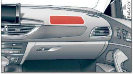
Fig. 152 Location of front passenger's airbag: in the instrument panel
