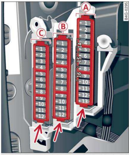
Fig. 202 Driver side cockpit: fuse panel with plastic bracket
