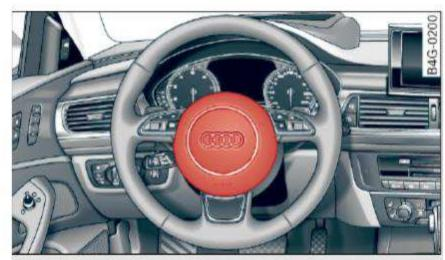
Fig. 151 Location of driver airbag: in steering wheel
