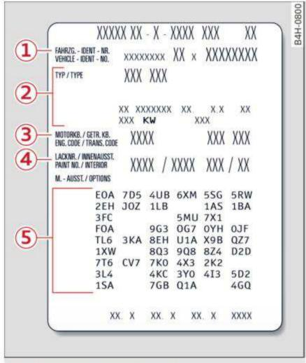
Fig. 214 Vehicle identification label
