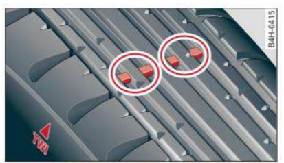
Fig. 186 Tire profile: treadwear indicator
