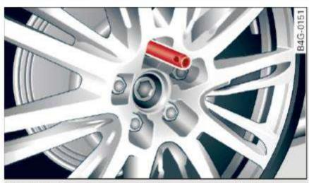
Fig. 199 Changing a wheel: alignment pin inside the top
