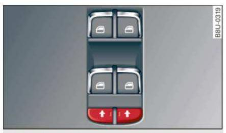
Fig. 30 Section of driver's door: child safety lock buttons
