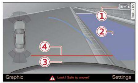
Fig. 122 Infotainment: blue surfaces aligned in the parking space
