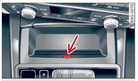
Fig. 86 Front center console: emergency release for the selector lever
