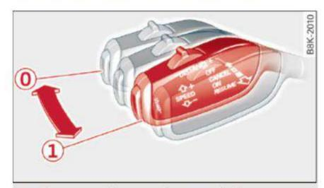
Fig. 92 Operating lever: switching on and off
