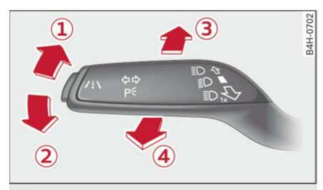
Fig. 37 Turn signal and high beam lever
