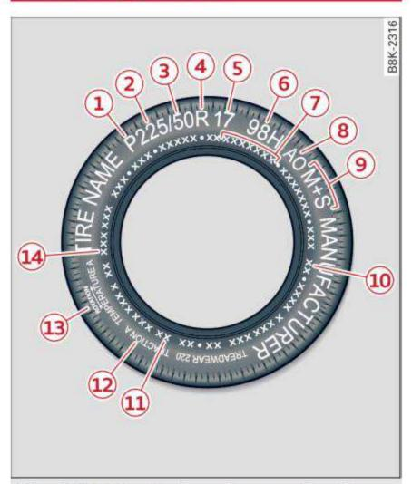
Fig. 185 Tire designations on the sidewall
