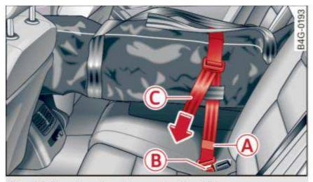
Fig. 70 Rear bench seat: securing the ski bag
