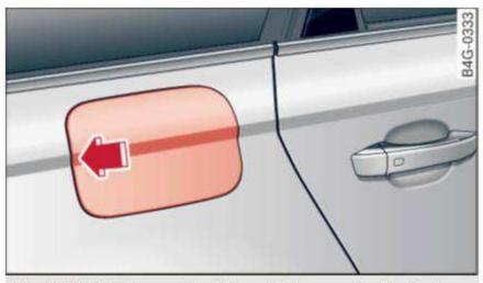
Fig. 172 Right rear side of the vehicle: opening the fuel filler door
