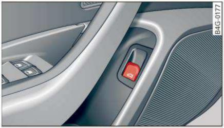
Fig. 25 Driver's door: opening/closing the luggage compartment lid
