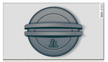
Fig. 181 Engine compartment: coolant expansion tank cover
