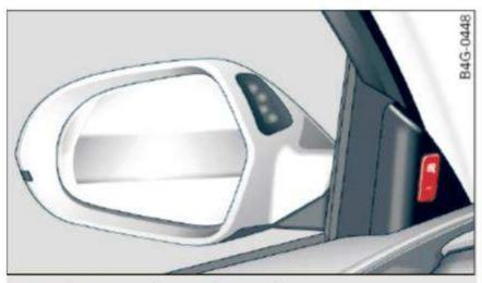
Fig. 107 Driver's door: side assist button
