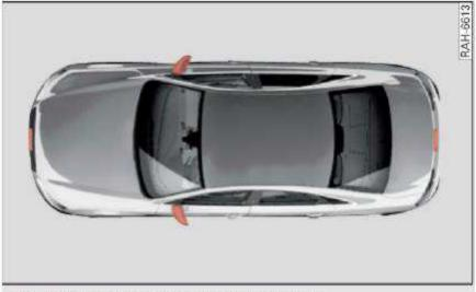
Fig. 124 Location of peripheral cameras
