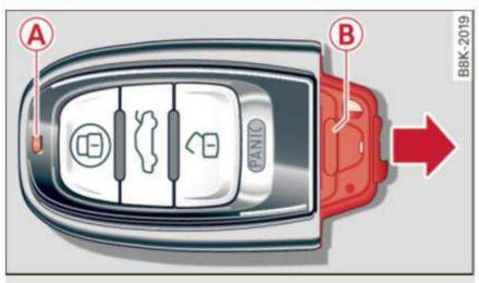
Fig. 16 Remote control key: removing the battery holder
