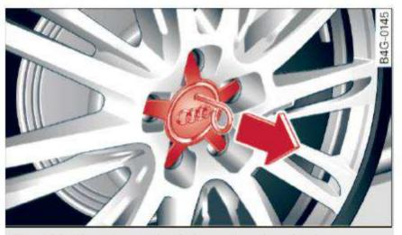
Fig. 192 Changing a wheel: Removing the wheel cover
