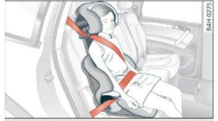
Fig. 165 Rear seat: child properly restrained in a booster seat
