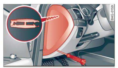
Fig. 201 Driver's side cockpit: cover
