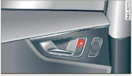
Fig. 20 Rear door: central locking switch
