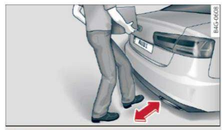
Fig. 27 Rear of the vehicle: foot movement
