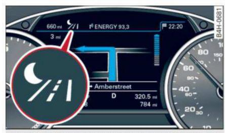
Fig. 109 Instrument cluster: symbol when the infrared image is not visible
