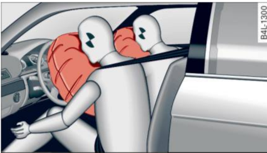
Fig. 221 Inflated front airbags
