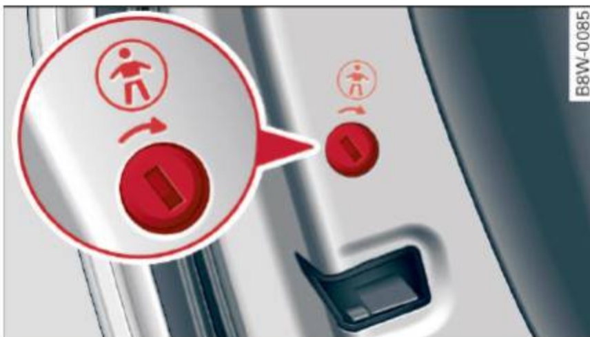
Fig. 39 Rear door: child safety lock
