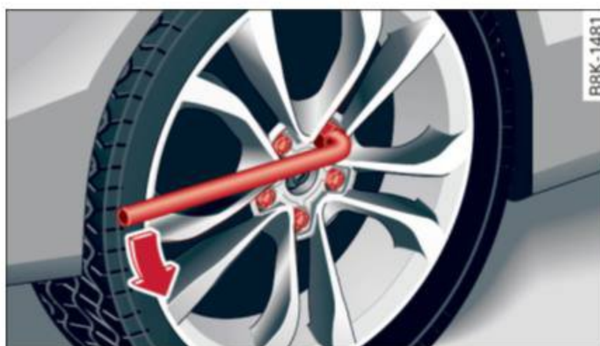
Fig. 263 Wheel: loosening the wheel bolt
