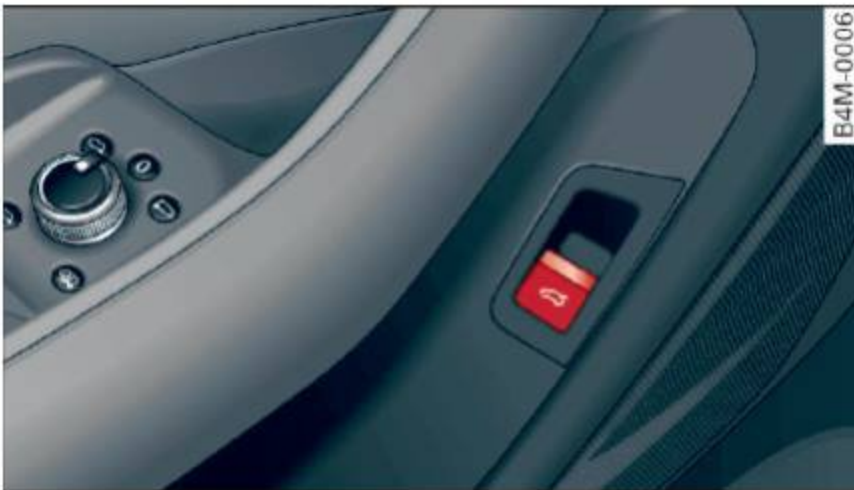
Fig. 34 Driver's door: opening the luggage compartment lid
