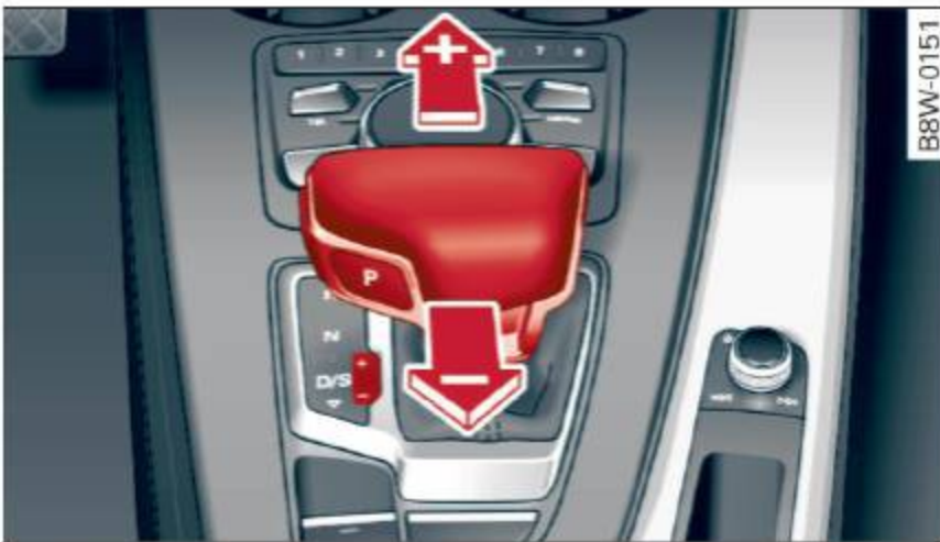
Fig. 84 Center console: shifting manually with the selector lever
