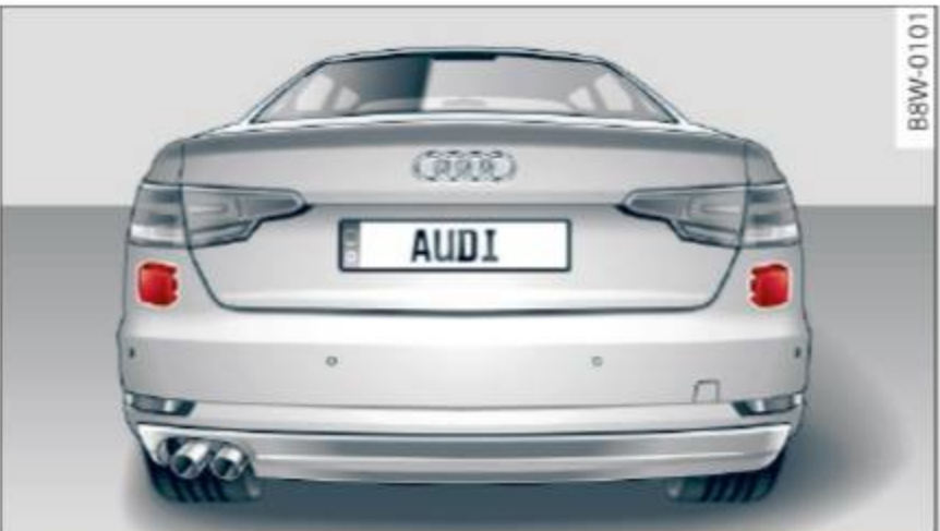
Fig. 112 Rear of the vehicle: position of the sensors
