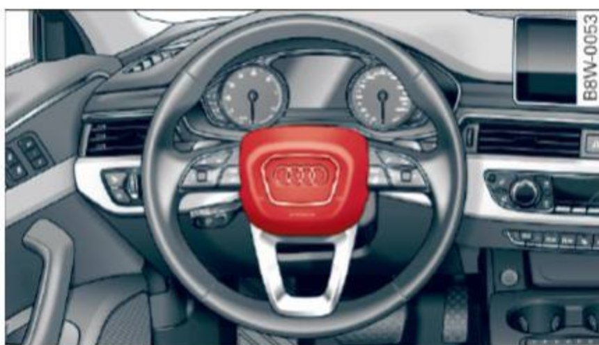
Fig. 219 Location of driver airbag: in steering wheel
