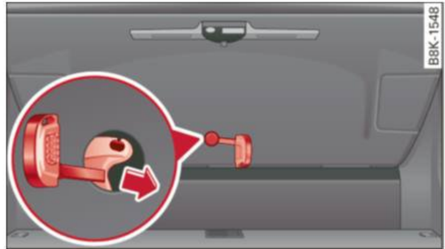
Fig. 36 Inner luggage compartment lid: access to the emergency release
