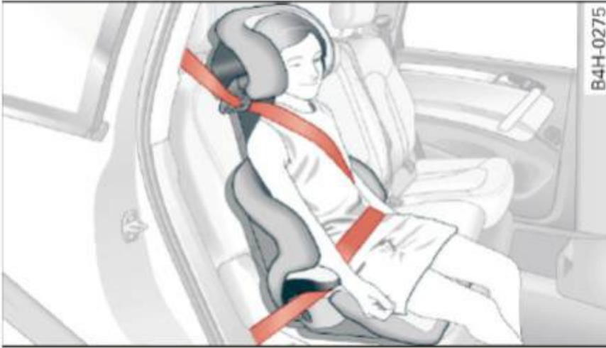
Fig. 233 Rear seat: child properly restrained in a booster seat
