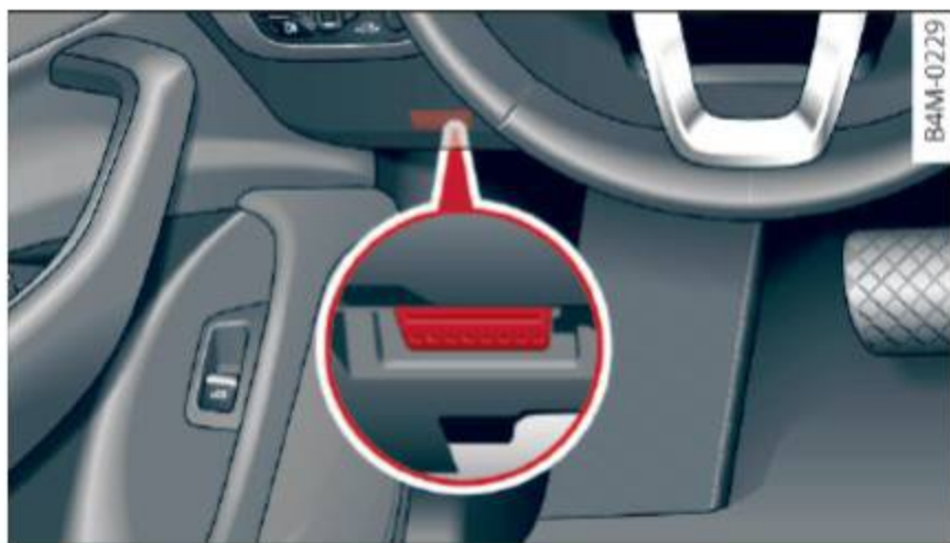
Fig. 24 Location of Data Link Connector (DLC)
