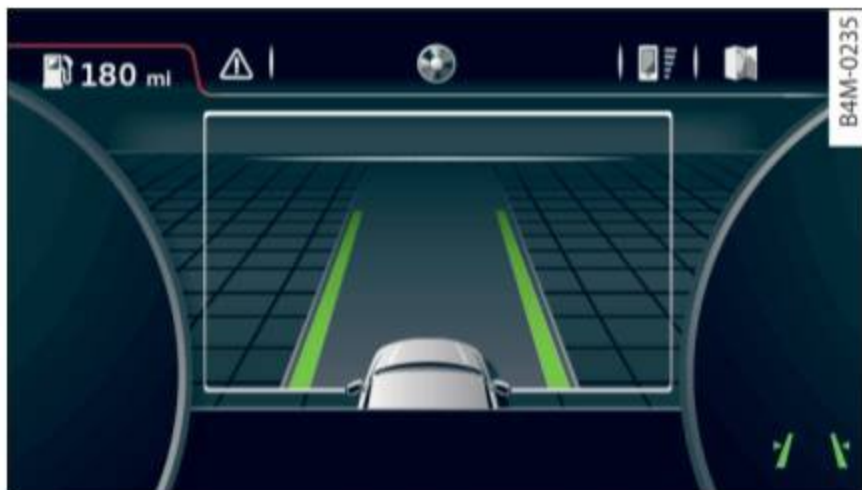
Fig. 107 Instrument cluster (multi-color display): active lane assist is switched on and ready to provide warnings
