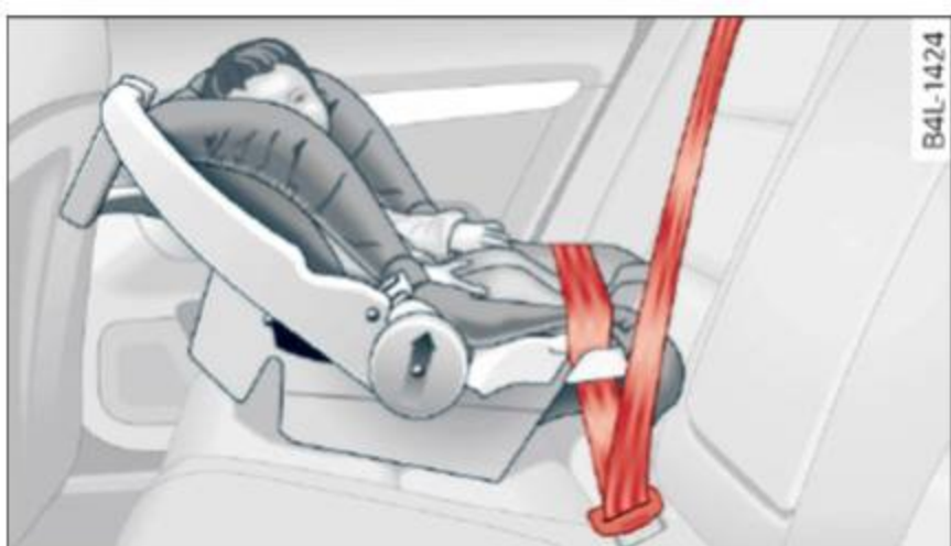
Fig. 230 Schematic overview: rearward-facing infant seat, properly installed on the rear seat
