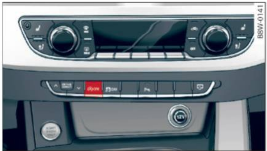
Fig. 81 Center console: Start/Stop system button
