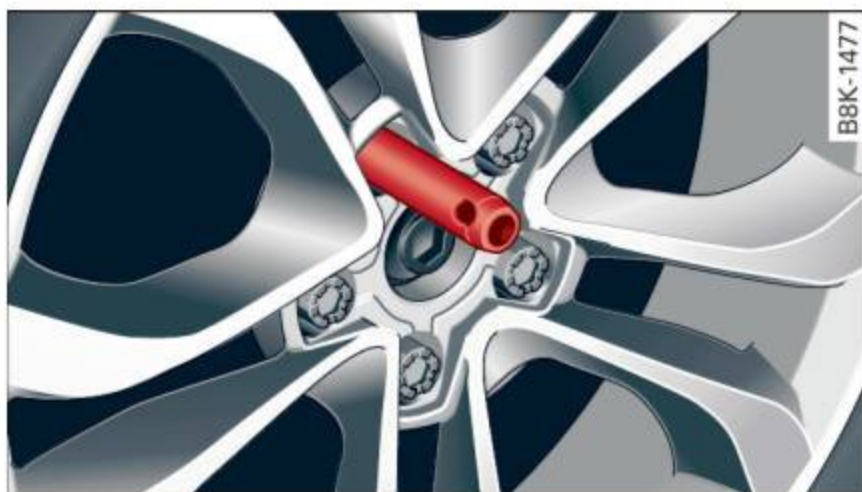
Fig. 267 Wheel: alignment pin in the top hole
