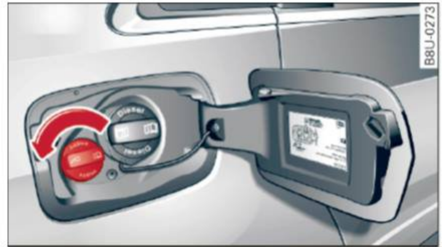
Fig. 243 Right rear side of the vehicle: removing the AdBlue cap
