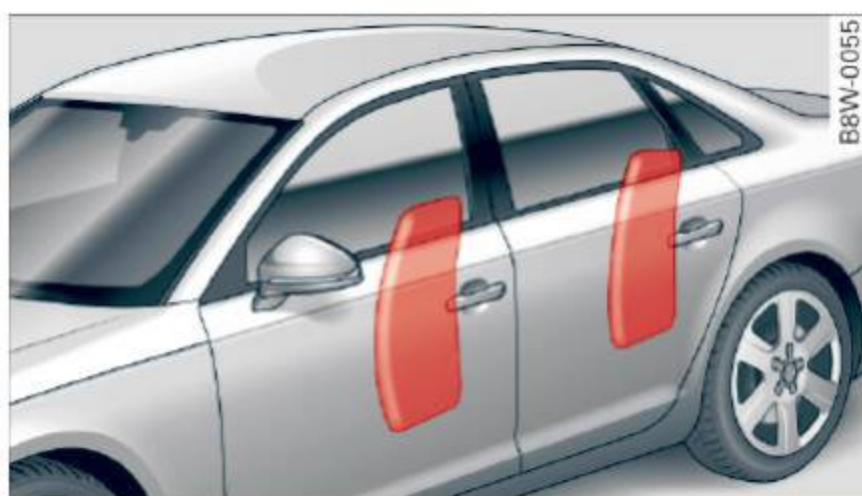
Fig. 226 Inflated side airbags on left side of vehicle, rear side airbag optional equipment
