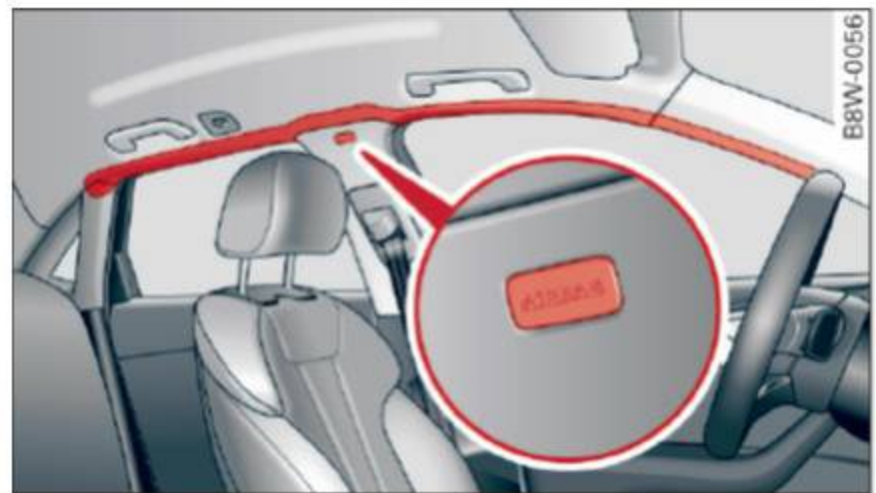
Fig. 227 Side curtain airbags, driver's side: location
