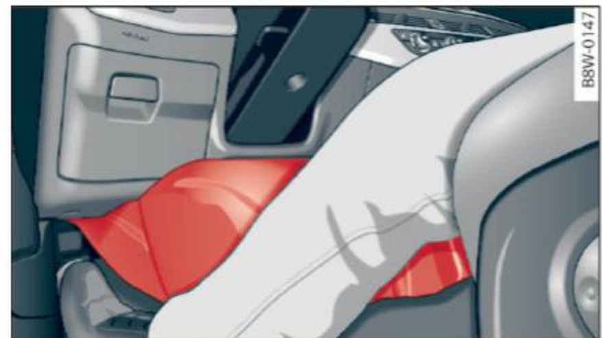
Fig. 224 Inflated airbags protecting in a frontal collision
