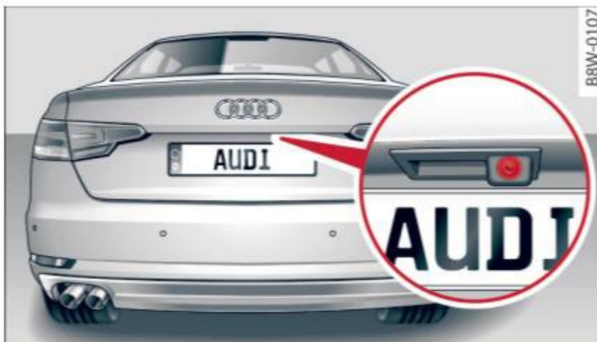
Fig. 124 Luggage compartment lid: location of the rearview camera
