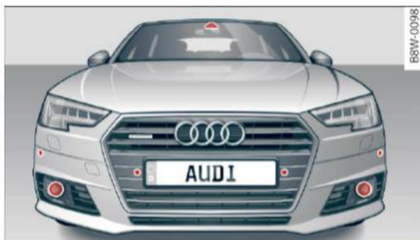
Fig. 90 Front of the vehicle: sensors and video camera
