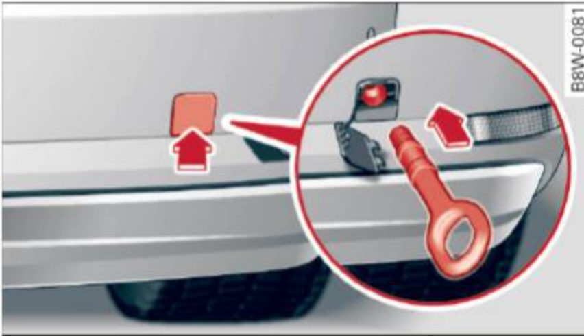
Fig. 277 Rear bumper: installing the towing loop
