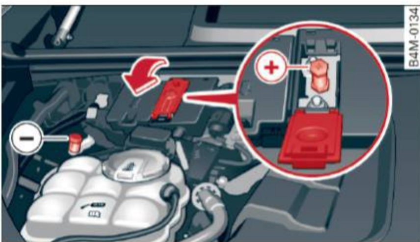
Fig. 251 Engine compartment: Connectors for charger and jumper cables
