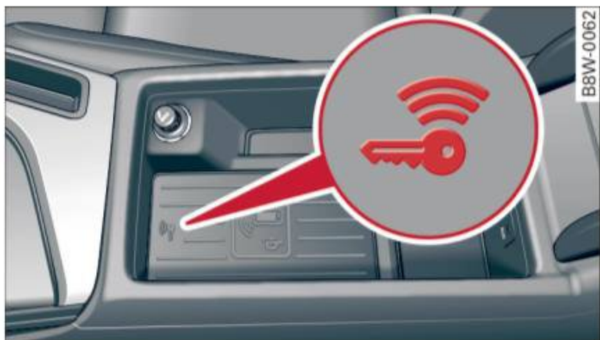
Fig. 78 Center console/remote control key: starting the engine if there is a malfunction
