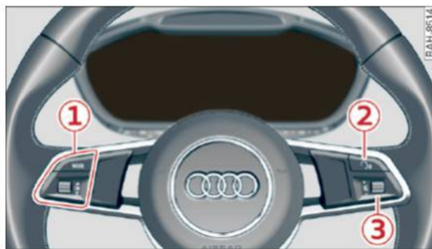
Fig. 12 Multifunction steering wheel
