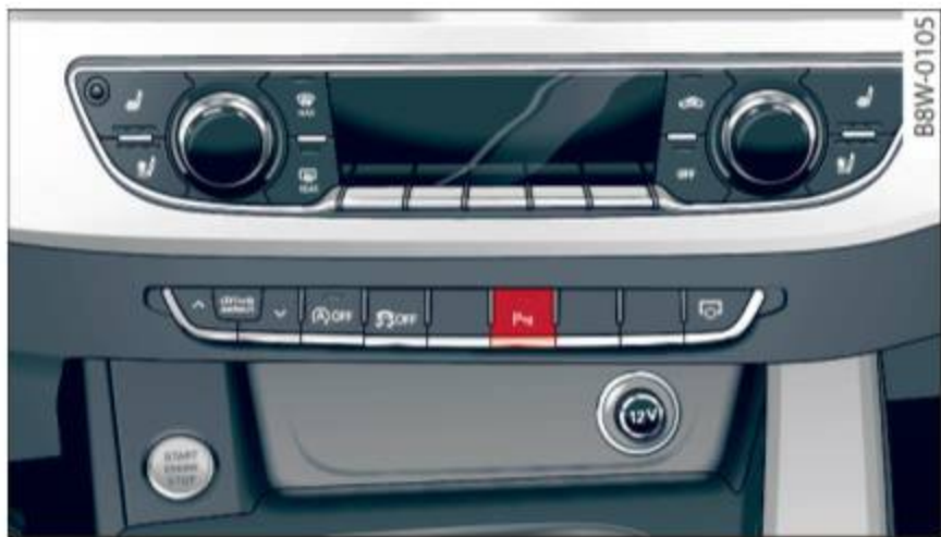
Fig. 120 Center console: parking aid button
