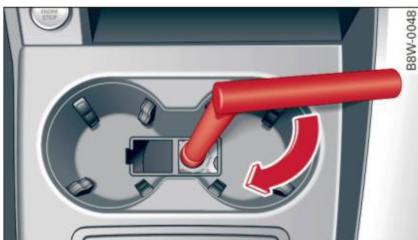
Fig. 87 Front cup holder: parking lock emergency release
