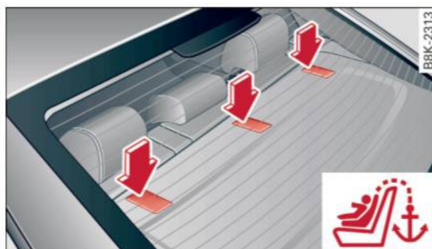
Fig. 237 Tether anchors: recess flaps behind the rear seatbacks
