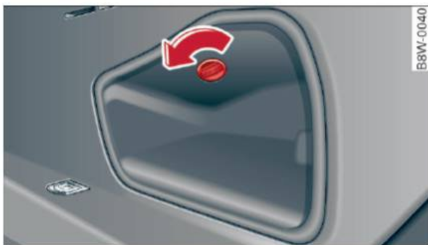
Fig. 241 Luggage compartment: opening the side trim panel
