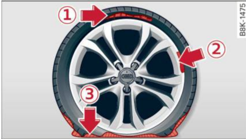
Fig. 259 Tire: tire damage that cannot be repaired
