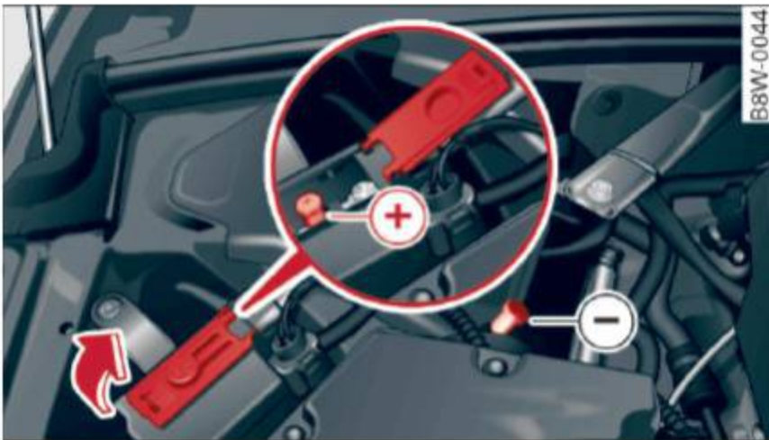
Fig. 274 Engine compartment: connectors for jump start cables and a charger
