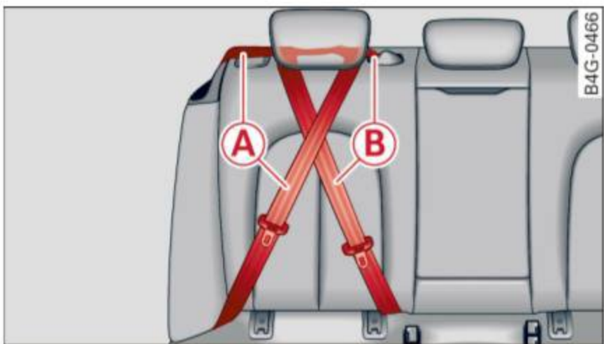
Fig. 229 Schematic overview: keep unused safety belts away from children in child safety seats. (A) - outer rear safety belt, (B) - center rear safety belt
