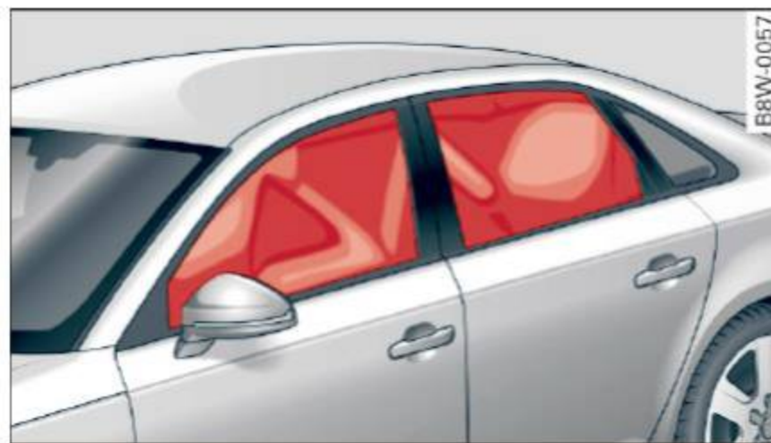
Fig. 228 Illustration of principle: Inflated side curtain airbags on the left side
