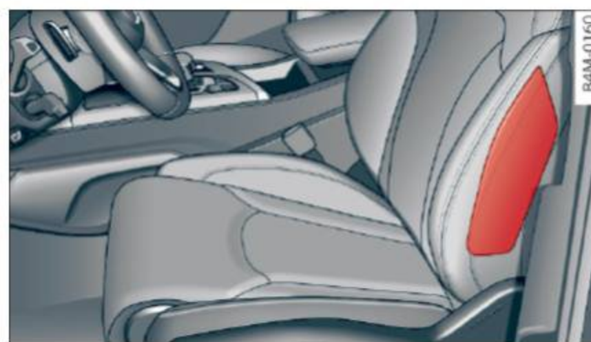
Fig. 225 Side airbag location in the driver's seat
