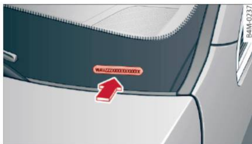
Fig. 281 Windshield (front left): Vehicle Identification Number (VIN)
