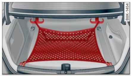
Fig. 84 Luggage compartment: cargo net at the top of the luggage compartment
