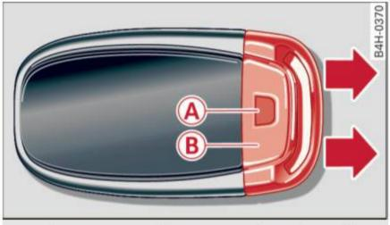
Fig. 19 Remote master key: removing the mechanical key
