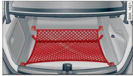
Fig. 83 Luggage compartment: cargo net stretched out
