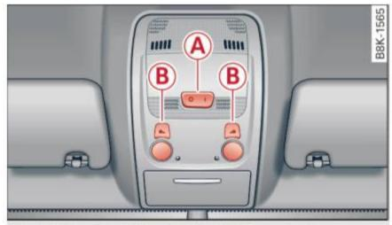
Fig. 45 Front headliner: interior lighting controls
