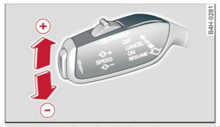
Fig. 118 Selector lever: changing the speed
