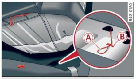
Fig. 30 Rear bench seat: emergency release cable
