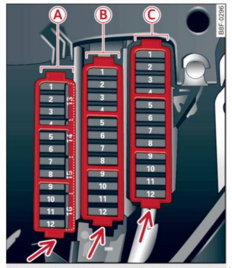
Fig. 206 Left cockpit: fuse panel with plastic clip
