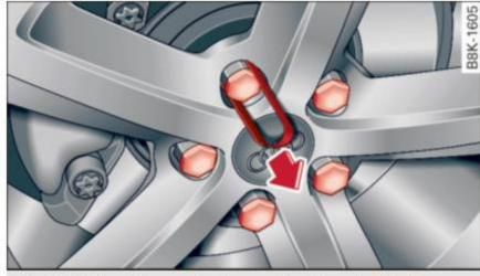
Fig. 199 Changing a wheel: removing the wheel bolt caps
