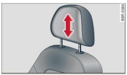
Fig. 63 Front seat: adjusting the head restraints
