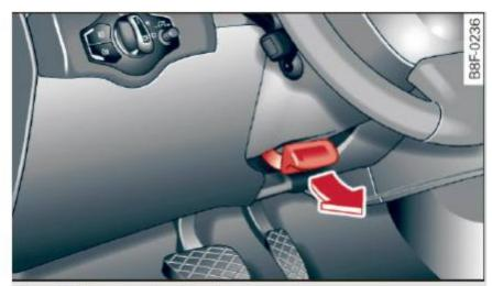
Fig. 95 Lever under the steering column
