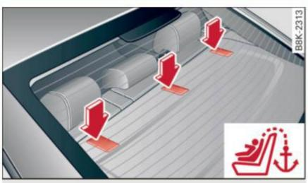
Fig. 169 Sedan Tether anchors: recess flaps behind the rear seatbacks
