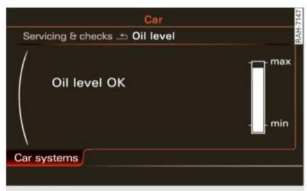
Fig. 182 MMI Display: Oil level indicator
