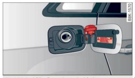
Fig. 176 Fuel filler flap with attached fuel cap
