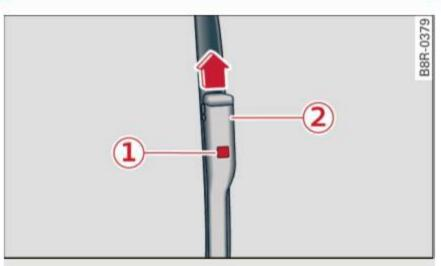
Fig. 56 Removing windshield wiper blade
