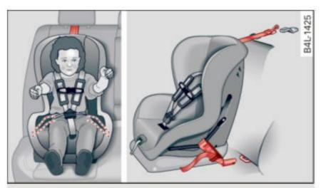
Fig. 162 Schematic overview: installation of the attachments applicable to a LATCH seat
