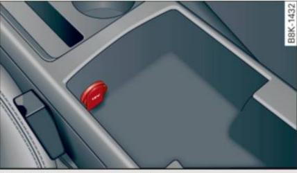
Fig. 70 Center console: socket
