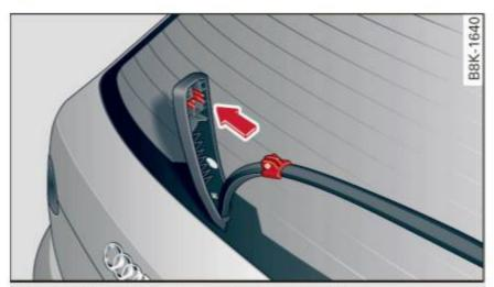
Fig. 57 Rear wiper: Removing the wiper blade
