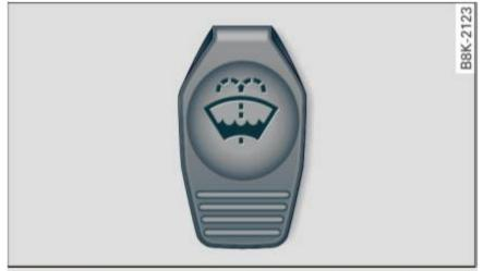
Fig. 187 Engine compartment: Cover on the windshield and headlight\* washer fluid container
