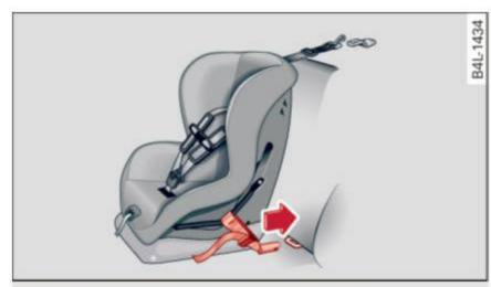
Fig. 168 Lower anchorages: proper mounting
