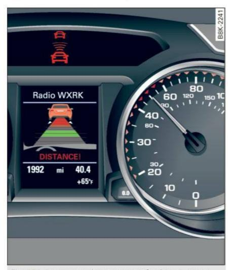
Fig. 121 Instrument cluster: request for driver intervention
