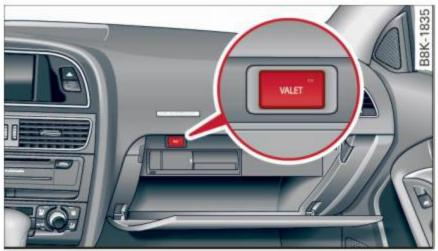
Fig. 38 Glove compartment: valet parking button
