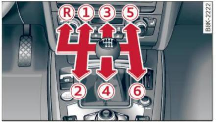
Fig. 104 Gearshift pattern: 6-speed manual transmission
