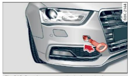
Fig. 212 Front bumper: screwing in the towing loop
