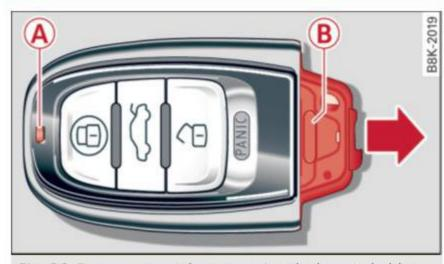
Fig. 20 Remote master key: removing the battery holder
