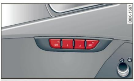
Fig. 66 Driver's door: memory function buttons
