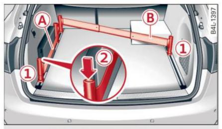
Fig. 88 Luggage compartment: securing attachments
