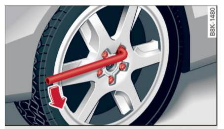
Fig. 200 Changing a wheel: loosening the wheel bolts
