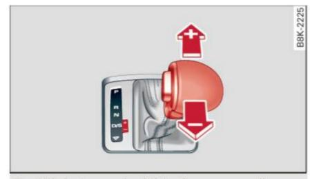
Fig. 108 Center console: shifting the gears manually
