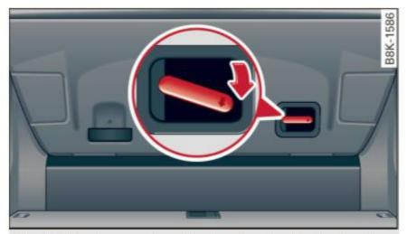
Fig. 32 Trunk escape handle: view from inside the closed rear lid
