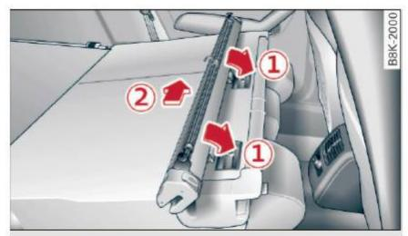
Fig. 81 Folded backrest: installing the partition net
