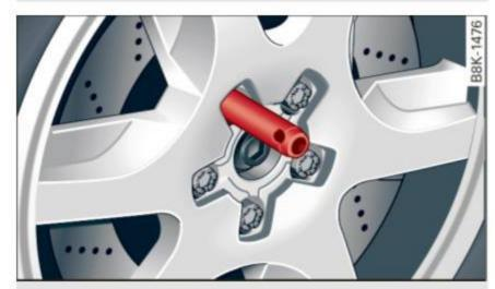
Fig. 204 Changing a wheel: alignment pin inside the top hole
