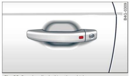
Fig. 22 Door handle: locking the vehicle
