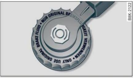
Fig. 185 Engine compartment: Cover on the brake fluid reservoir
