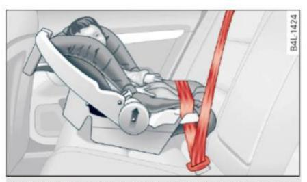
**Fig. 161** Schematic overview: rearward-facing infant seat, properly installed on the rear seat
