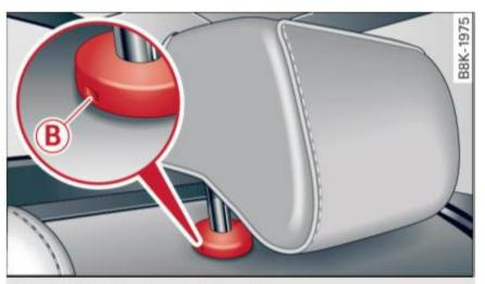
Fig. 65 Rear head restraints: release
