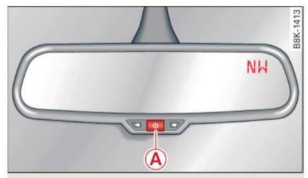
Fig. 58 Rearview mirror: Digital compass activated
