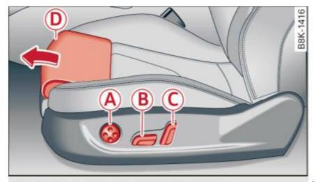
Fig. 61 Front seats: power seat adjustment
