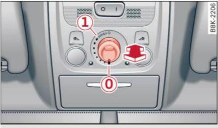
Fig. 36 Section of headliner: knob for sunroof
