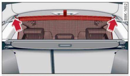
Fig. 79 Behind the backrest: hanging the partition net
