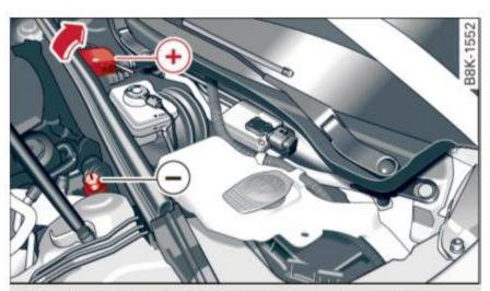
Fig. 209 Engine compartment: Connectors for jumper cables and charger
