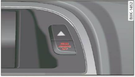
Fig. 155 Section from the instrument panel: PASSENGER AIR BAG OFF light
