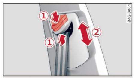
Fig. 151 Safety belt height adjustment for the front seats loop-around fittings
