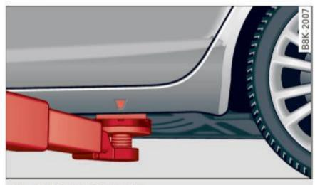
Fig. 217 Rear lifting point
