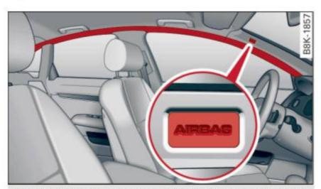
Fig. 158 Side curtain system, driver's side: side curtain airbag location
