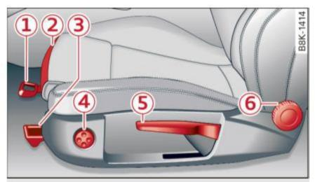
Fig. 60 Front seats: manual seat adjustment
