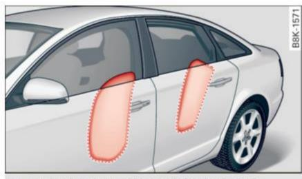
Fig. 157 Inflated side airbags on left side of vehicle
