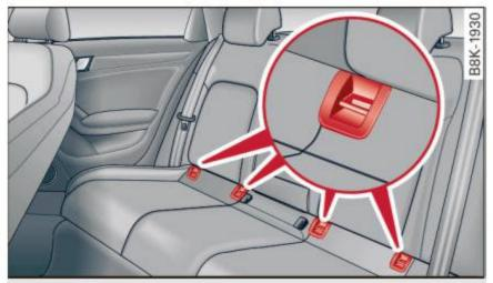
Fig. 167 Rear seats: lower anchorage bracket locations
