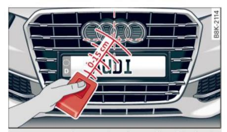
Fig. 41 Distance between the radiator grille and the hand transmitter
