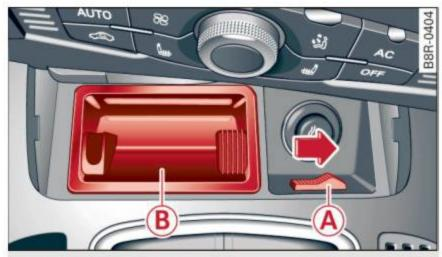
Fig. 110 Front center console: Removing the ashtray insert
