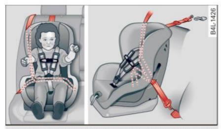
Fig. 163 Schematic overview: installation of the seat using the vehicle's safety belt system
