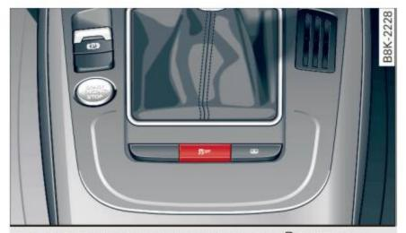
Fig. 173 Version A: lower center console, 身 OFF button
