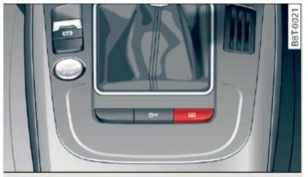
Fig. 53 Without MMI: Button for rear window sun shade
