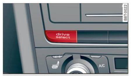
Fig. 128 Center console: Control for Audi drive select
