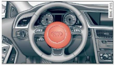
Fig. 152 Location of driver airbag: in steering wheel
