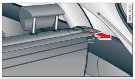
**Fig. 77** Right front section of the luggage compartment: removing the luggage compartment cover
