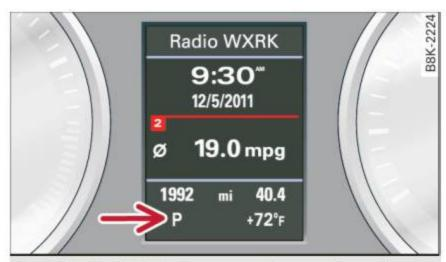
**Fig. 105** Display in the instrument cluster: selector lever in position P
