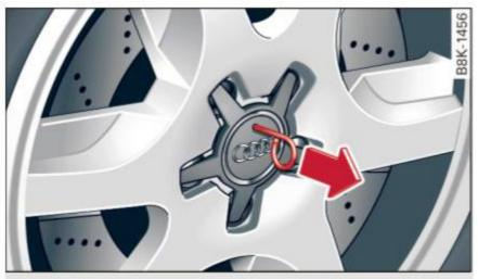
Fig. 198 Changing a wheel: removing the wheel cover
