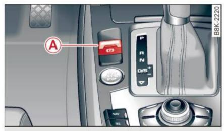
Fig. 100 Center console: Parking brake
