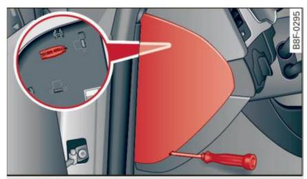
Fig. 205 Left cockpit: fuse panel cover
