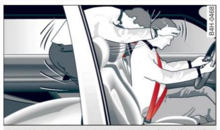
**Fig. 145** A rear passenger not wearing a safety belt will fly forward and strike the driver
