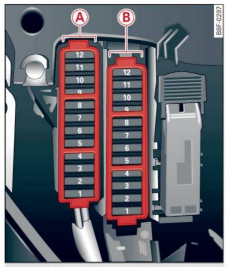
Fig. 207 Right cockpit: fuse panel with plastic clip
