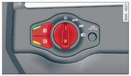
Fig. 42 Instrument panel: headlight control switch
