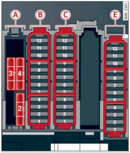
Fig. 208 Right luggage compartment: fuse panel with plastic clip
