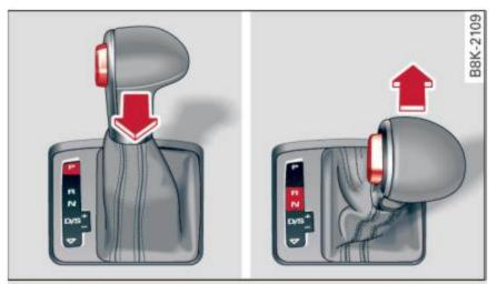
Fig. 106 Shift gate: selector lever lock positions and release button highlighted
