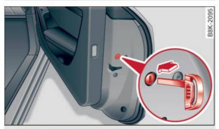
Fig. 25 Front passenger's door/rear doors\*: emergency lock
