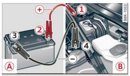
Fig. 210 Jump starting with the battery of another vehicle:
