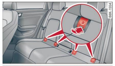
Fig. 166 Lower anchorages, covers marked
