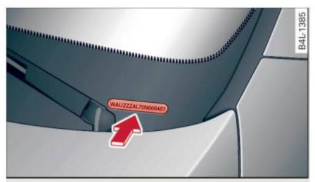
Fig. 218 Vehicle Identification Number (VIN) plate: location on driver's side dash panel
