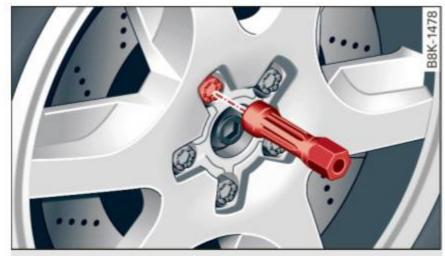
Fig. 203 Changing a wheel: using the screwdriver handle (with the blade removed) to turn the bolts
