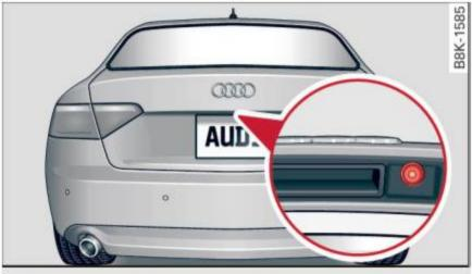
Fig. 133 Trunk lid: Location of the rear view camera
