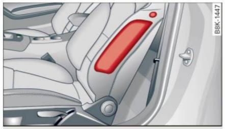
Fig. 156 Side airbag location in the driver's seat
