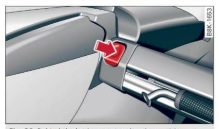
Fig. 80 Behind the backrest: removing the partition net
