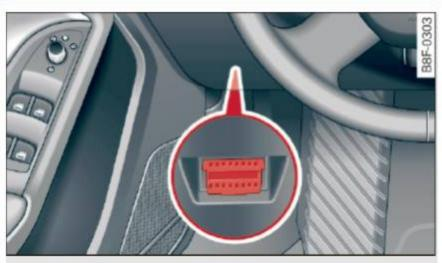
Fig. 17 Location of Data Link Connector (DLC)
