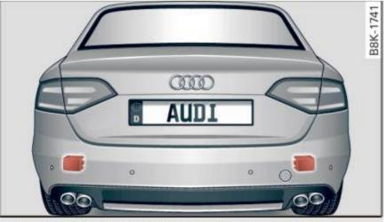
Fig. 126 Rear of the vehicle: position of the sensors
