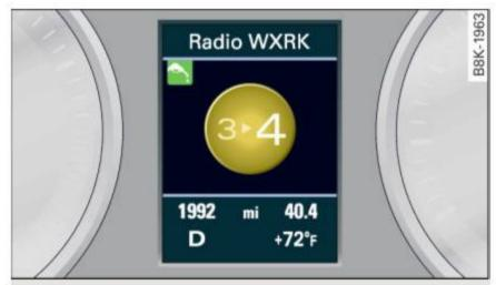
Fig. 14 Display: enhanced shift indicator
