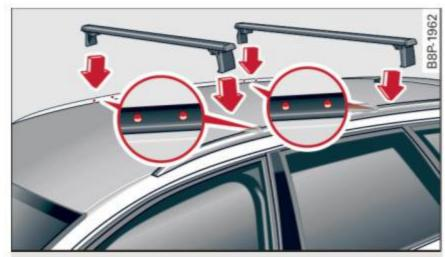
Fig. 75 allroad: Roof rack attachment points
