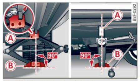
Fig. 202 Sill: positioning the vehicle jack
