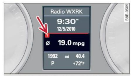
Fig. 10 Trip computer display: memory level 1
