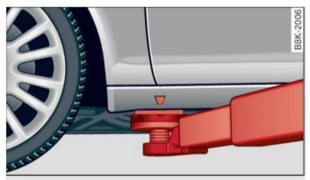
Fig. 216 Front lifting point
