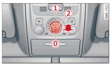
Fig. 37 Section from headliner: knob for sunroof.
