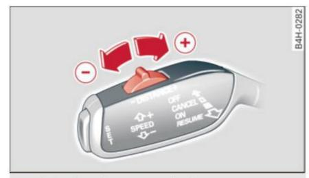
Fig. 120 Selector lever: setting the distance
