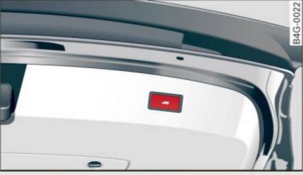
Fig. 29 Locking switch in the rear lid
