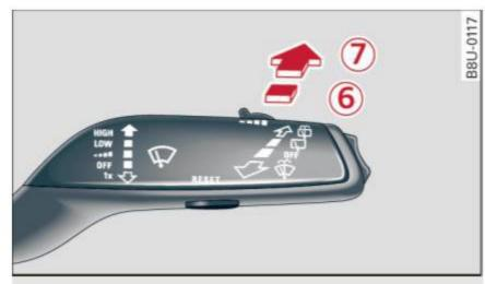
Fig. 55 allroad: Rear wiper actuation
