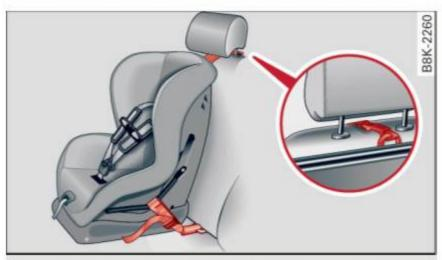
Fig. 172 allroad Tether strap: proper routing and mounting
