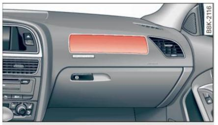
Fig. 153 Location of front passenger's airbag: in the instrument panel
