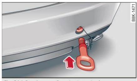
Fig. 214 Rear bumper: Screwing in towing loop
