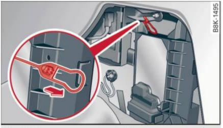
Fig. 178 Luggage compartment: Emergency opening of fuel filler flap
