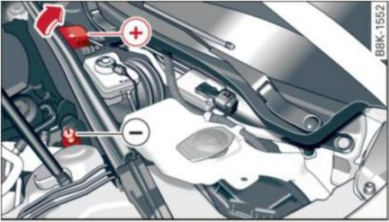
Fig. 186 Engine compartment: Connectors for charger and jumper cables
