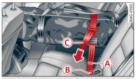
Fig. 90 Rear bench seat: securing the ski sack
