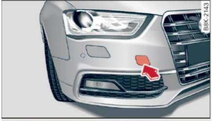
Fig. 211 Front bumper: removing the cover cap
