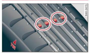
Fig. 189 Tire profile: treadwear indicator
