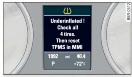
Fig. 192 Instrument cluster: indicator light with message
