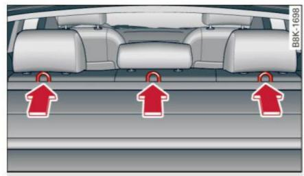
Fig. 170 allroad Tether anchors: attachment hook locations behind the rear seatbacks
