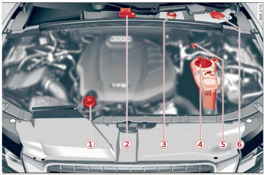
Fig. 181 Typical layout for containers and engine oil filler cap
