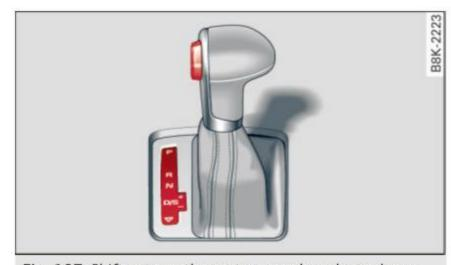
Fig. 107 Shift gate on the center console: selector lever with release button
