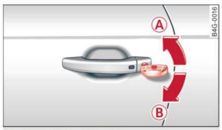
Fig. 24 Driver's door: lock cylinder
