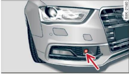
Fig. 112 Front of the vehicle: Position of radar sensor
