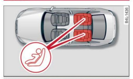
Fig. 165 Schematic overview: LATCH anchorage point locations
