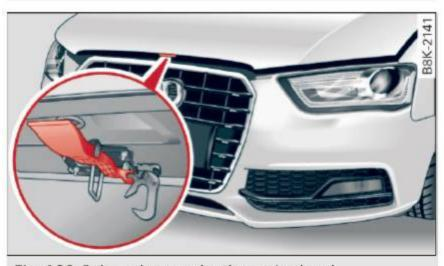
Fig. 180 Release lever under the engine hood
