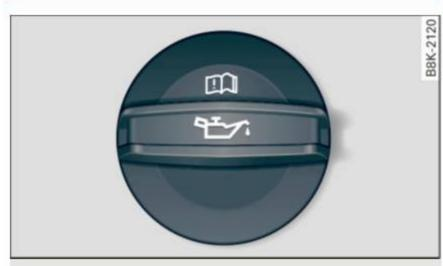
Fig. 183 Engine compartment: Cover on the oil filler neck
