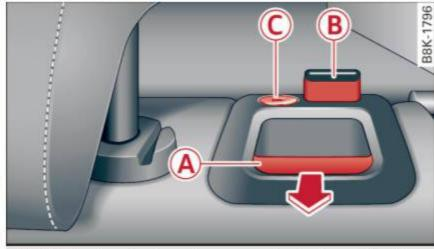
Fig. 78 Backrest: release lever, securing knob and latch\*
