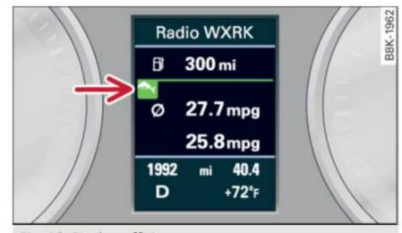
Fig. 13 Display: efficiency program
