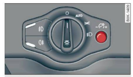
Fig. 47 Instrument illumination
