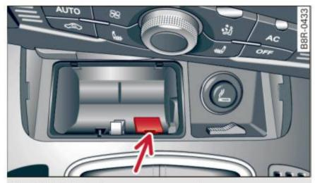
Fig. 111 Selector lever emergency release
