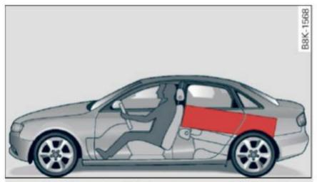
**Fig. 140** Safe load positioning: place heavy objects as low and as far forward as possible.
