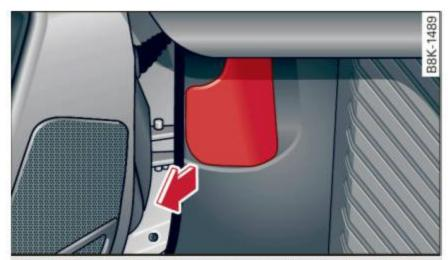
Fig. 179 Driver's side footwell: engine hood release lever
