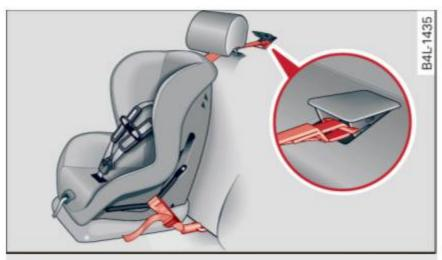
Fig. 171 Sedan Tether strap: proper routing and mounting
