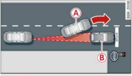
Fig. 114 Example: object changing lanes and stationary object
