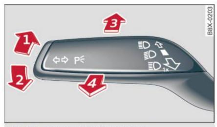
Fig. 43 Turn signal and high beam lever
