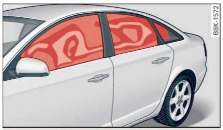
Fig. 159 Illustration of principle: Inflated side curtain airbags on the left side
