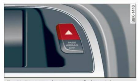
Fig. 44 Center console: emergency flasher switch
