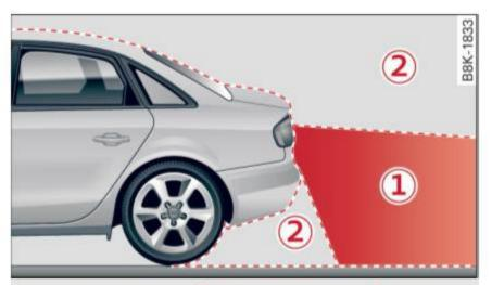
Fig. 132 Covered area (1) and uncovered area (2) of the rear view camera
