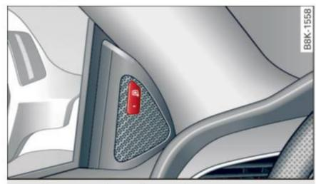
Fig. 127 Driver's door: Side assist button
