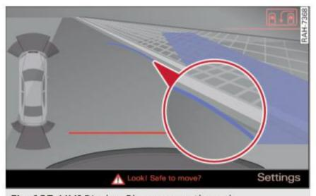
Fig. 137 MMI Display: Blue curve on the curb
