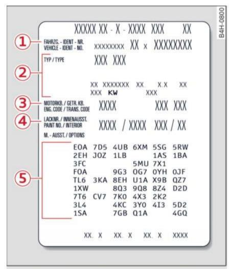
Fig. 219 The vehicle identification label: inside the luggage compartment
