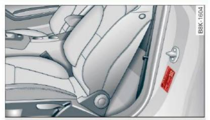
Fig. 190 Driver's side B-pillar: tire pressure label
