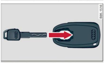
Fig. 98 Insert emergency key into the adapter
