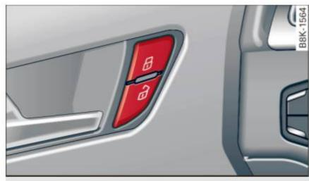
Fig. 23 Driver's door: power locking switch
