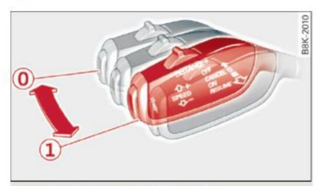
Fig. 116 Selector lever: switching on/off
