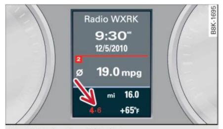
Fig. 12 Display: Gearshift indicator
