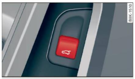
Fig. 28 Driver's door: Unlocking the rear lid
