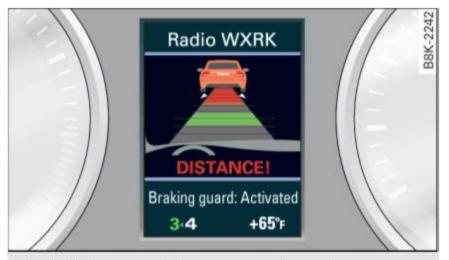
Fig. 122 Instrument cluster: approach warning
