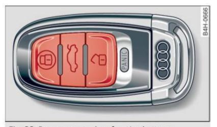
Fig. 22 Remote master key: function buttons
