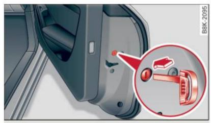
Fig. 26 Front passenger's door/rear doors\*: emergency lock
