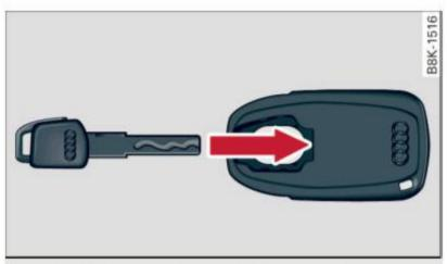
Fig. 96 Insert emergency key into the adapter
