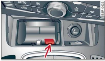
Fig. 109 Selector lever emergency release
