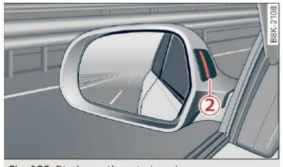
Fig. 122 Display on the exterior mirror
