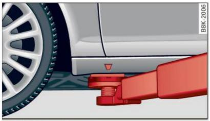
Fig. 218 Front lifting point
