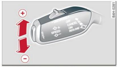
Fig. 116 Selector lever: changing the speed
