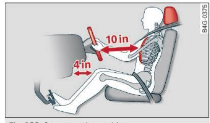
Fig. 139 Correct seating position
