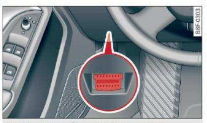
Fig. 18 Location of Data Link Connector (DLC)
