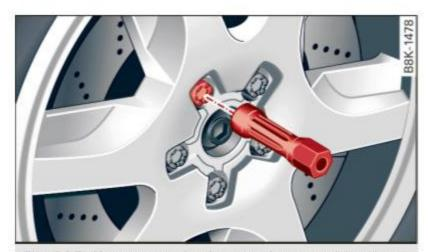
Fig. 205 Changing a wheel: using the screwdriver handle (with the blade removed) to turn the bolts
