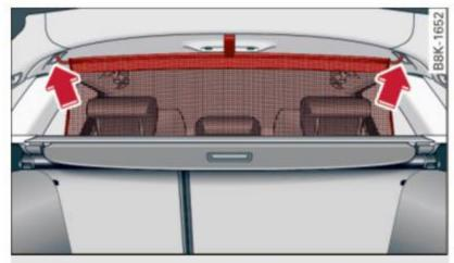
Fig. 77 Behind the backrest: hanging the partition net
