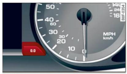
Fig. 6 Instrument cluster: reset button
