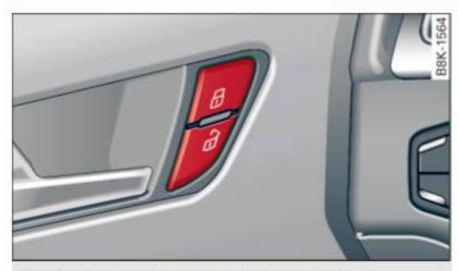
Fig. 24 Driver's door: power locking switch
