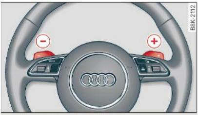
Fig. 107 Steering wheel: Shift buttons\*
