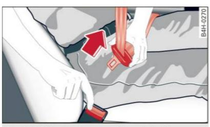
Fig. 151 Releasing the tongue from the buckle
