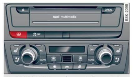
Fig. 50 With MMI: Button for rear window sun shade
