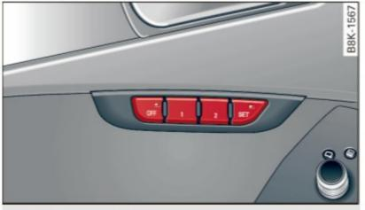
Fig. 64 Driver's door: memory function buttons
