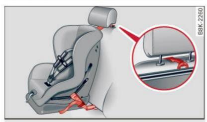
Fig. 173 allroad Tether strap: proper routing and mounting
