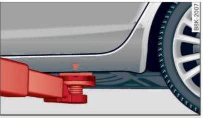
Fig. 219 Rear lifting point
