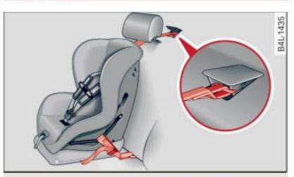
Fig. 172 Sedan Tether strap: proper routing and mounting
