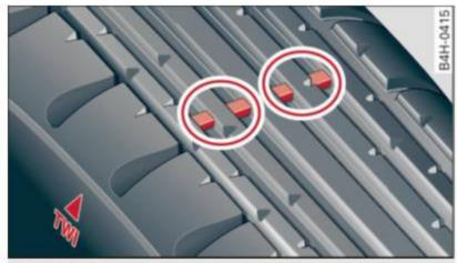
Fig. 191 Tire tread: tread wear indicators (TWI)
