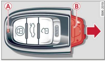
Fig. 21 Remote master key: removing the battery holder
