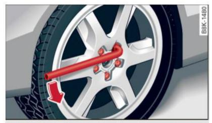
Fig. 202 Changing a wheel: loosening the wheel bolts
