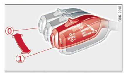
Fig. 114 Selector lever: switching on/off
