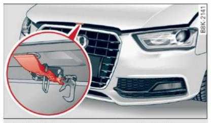
Fig. 181 Release lever under the engine hood
