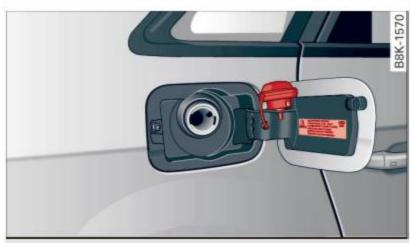
Fig. 177 Fuel filler flap with attached fuel cap
