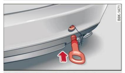
Fig. 216 Rear bumper: Screwing in towing loop
