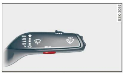
Fig. 8 Wiper lever: controls for the menu display
