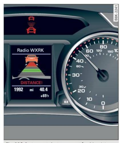
Fig. 119 Instrument cluster: request for driver intervention
