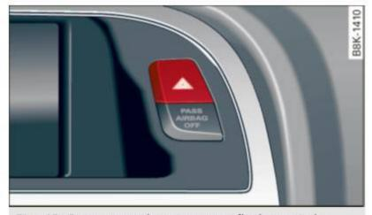
Fig. 42 Center console: emergency flasher switch
