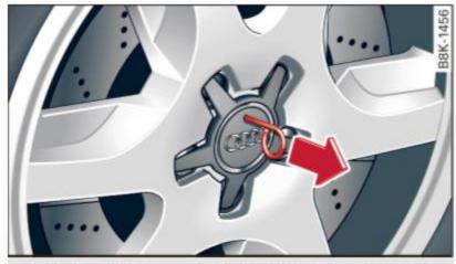
Fig. 200 Changing a wheel: removing the wheel cover
