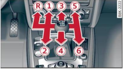
Fig. 102 Gearshift pattern: 6-speed manual transmission
