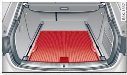
Fig. 90 Luggage compartment: cargo area floor reversed
