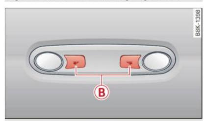
Fig. 44 Rear headliner: rear reading lights
