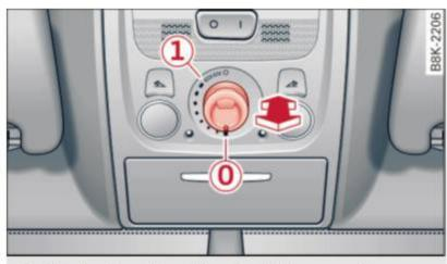
Fig. 37 Section of headliner: knob for sunroof
