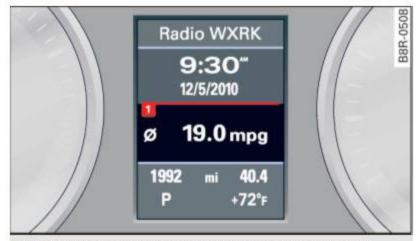
Fig. 9 Trip computer display: Average fuel mileage
