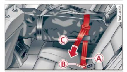
Fig. 88 Rear bench seat: securing the ski sack
