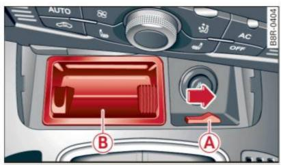
Fig. 108 Front center console: Removing the ashtray insert
