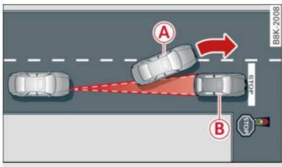
Fig. 112 Example: object changing lanes and stationary object
