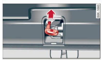
Fig. 32 Rear lid opening: access to the emergency release
