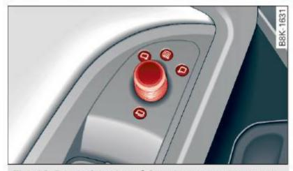
Fig. 46 Forward section of driver's armrest: power mirror controls
