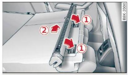
Fig. 79 Folded backrest: installing the partition net
