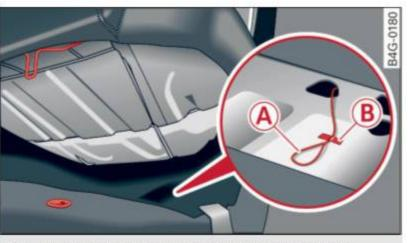
Fig. 31 Rear bench seat: emergency release cable
