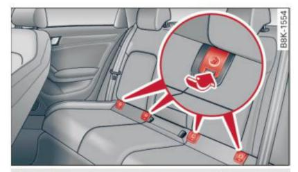
Fig. 167 Lower anchorages, covers marked
