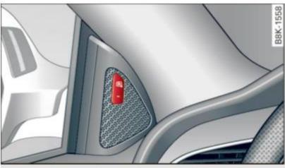
Fig. 125 Driver's door: Side assist button
