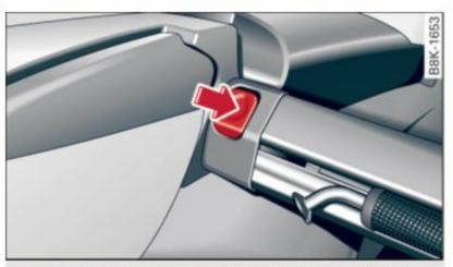
Fig. 78 Behind the backrest: removing the partition net
