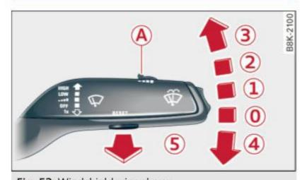
Fig. 52 Windshield wiper lever
