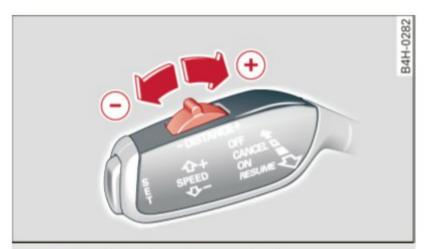
Fig. 118 Selector lever: setting the distance
