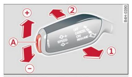
Fig. 100 Control lever with push-button
