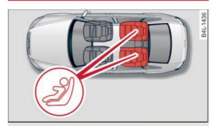
Fig. 166 Schematic overview: LATCH anchorage point locations
