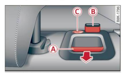
Fig. 76 Backrest: release lever, securing knob and latch\*
