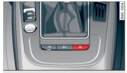
Fig. 51 Without MMI: Button for rear window sun shade
