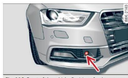
Fig. 110 Front of the vehicle: Position of radar sensor
