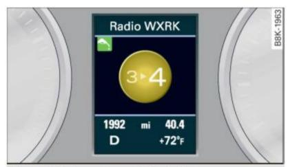
Fig. 14 Display: enhanced shift indicator
