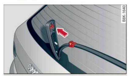
Fig. 55 Rear wiper: Removing the wiper blade
