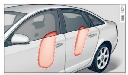
Fig. 158 Inflated side airbags on left side of vehicle
