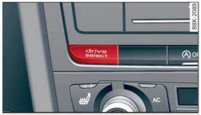
Fig. 126 Center console: Control for Audi drive select
