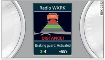
Fig. 120 Instrument cluster: approach warning
