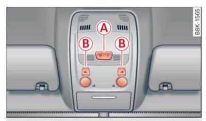
Fig. 43 Front headliner: interior lighting controls
