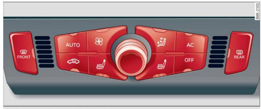
Fig. 91 Automatic climate control system: control
