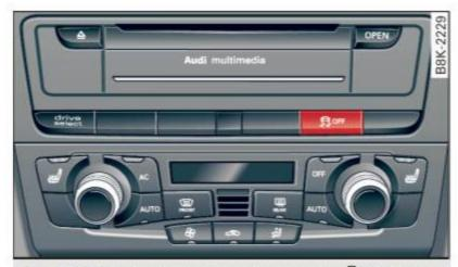
Fig. 175 Version B: upper center console, ♬ OFF button
