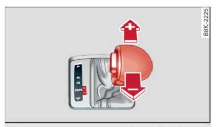
Fig. 106 Center console: shifting the gears manually
