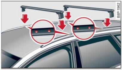
Fig. 73 allroad: Roof rack attachment points
