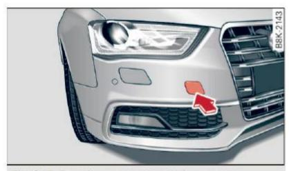
Fig. 213 Front bumper: removing the cover cap
