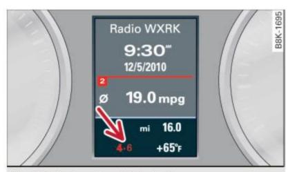
Fig. 12 Display: Gearshift indicator
