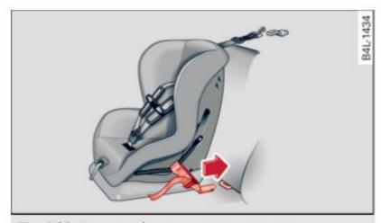
Fig. 169 Lower anchorages: proper mounting
