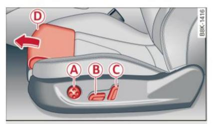
Fig. 59 Front seats: power seat adjustment
