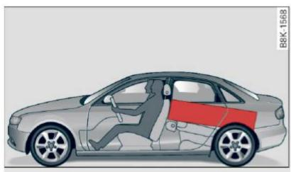
**Fig. 141** Safe load positioning: place heavy objects as low and as far forward as possible.
