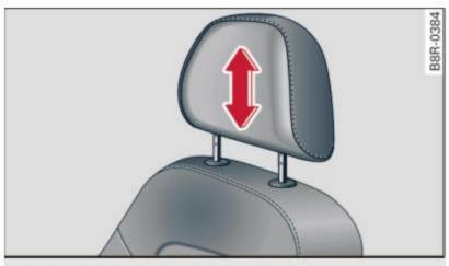
Fig. 61 Front seat: adjusting the head restraints
