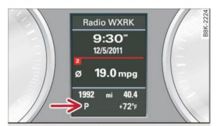
Fig. 103 Display in the instrument cluster: selector lever in position P
