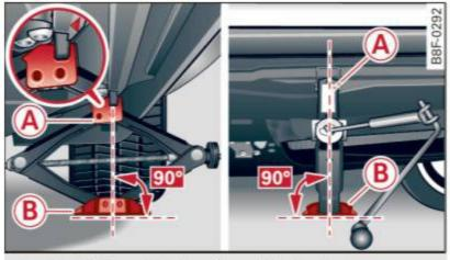
Fig. 204 Sill: positioning the vehicle jack
