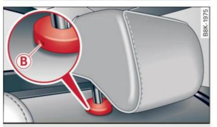
Fig. 63 Rear head restraints: release
