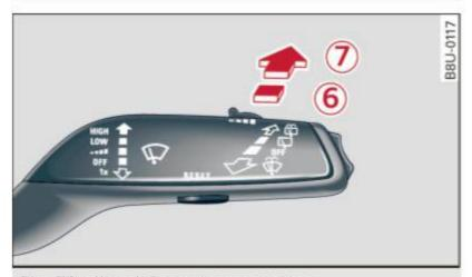
Fig. 53 allroad: Rear wiper actuation
