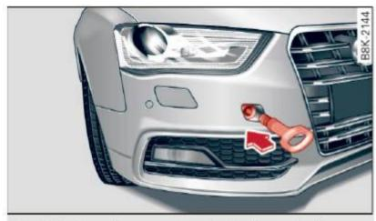
Fig. 214 Front bumper: screwing in the towing loop
