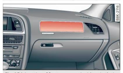
**Fig. 154** Location of front passenger's airbag: in the instrument panel
