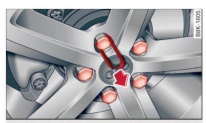
Fig. 201 Changing a wheel: removing the wheel bolt caps
