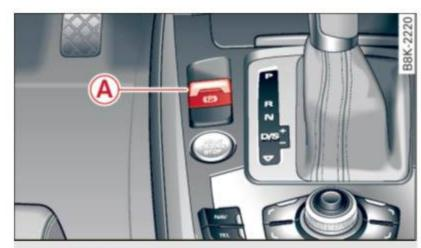
Fig. 98 Center console: Parking brake
