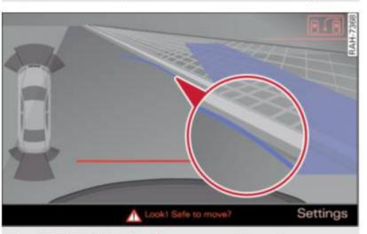
Fig. 135 MMI Display: Blue curve on the curb
