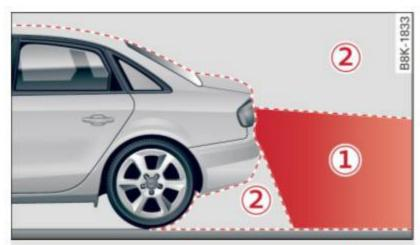
Fig. 130 Covered area (1) and uncovered area (2) of the rear view camera
