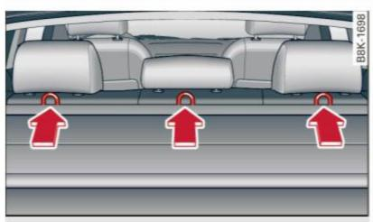
Fig. 171 allroad Tether anchors: attachment hook locations behind the rear seatbacks
