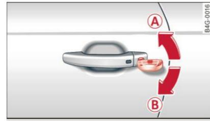
Fig. 36 Key turns for opening and closing
