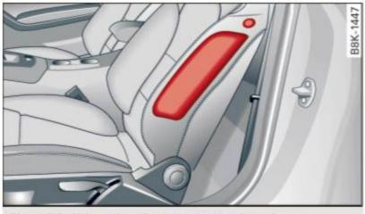
Fig. 157 Side airbag location in the driver's seat
