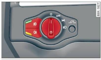
Fig. 40 Instrument panel: headlight control switch
