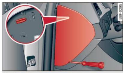
Fig. 207 Left cockpit: fuse panel cover
