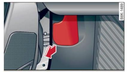
Fig. 180 Driver's side footwell: engine hood release lever
