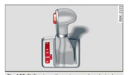
**Fig. 105** Shift gate on the center console: selector lever with release button
