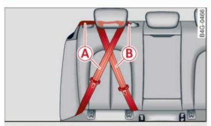
Fig. 161 Schematic overview: keep unused safety belts away from children in child safety seats. (A) - outer rear safety belt, (B) - center rear safety belt
