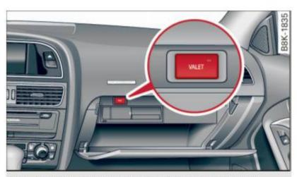
Fig. 39 Glove compartment: valet parking button
