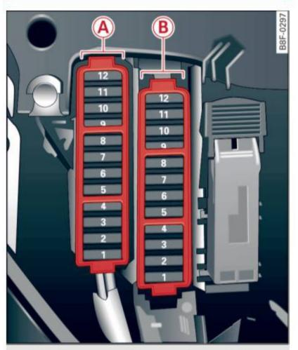
Fig. 209 Right cockpit: fuse panel with plastic clip
