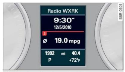
Fig. 7 Instrument cluster: center display
