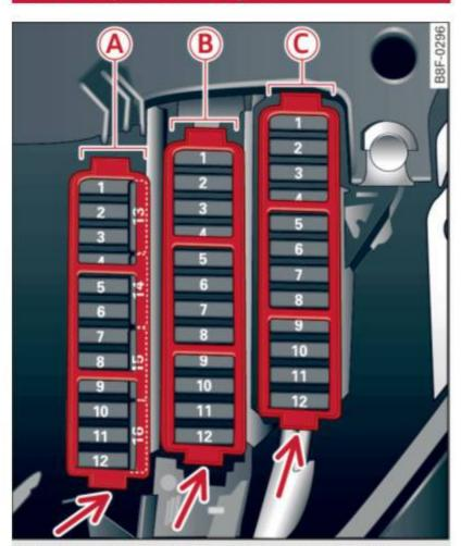
Fig. 208 Left cockpit: fuse panel with plastic clip
