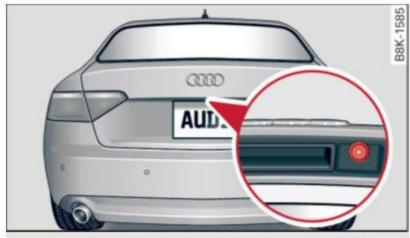
Fig. 131 Trunk lid: Location of the rear view camera
