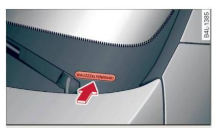
Fig. 220 Vehicle Identification Number (VIN) plate: location on driver's side dash panel
