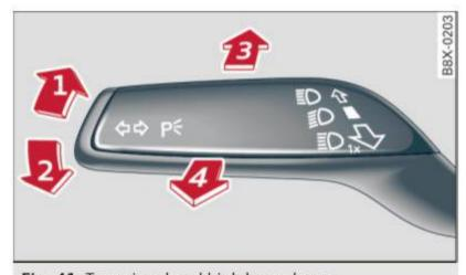
Fig. 41 Turn signal and high beam lever
