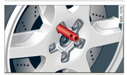
Fig. 206 Changing a wheel: alignment pin inside the top hole
