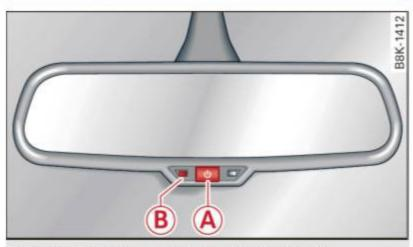
Fig. 47 Automatic dimming rearview mirror\*
