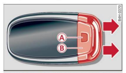
Fig. 20 Remote master key: removing the mechanical key
