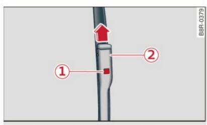
Fig. 54 Removing windshield wiper blade
