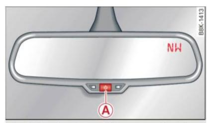
Fig. 56 Rearview mirror: Digital compass activated
