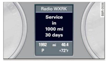
Fig. 17 Display: Service interval display
