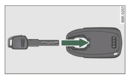
Fig. 31 Insert emergency key into the adapter
