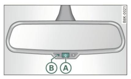
Fig. 61 Inside rear view mirror
