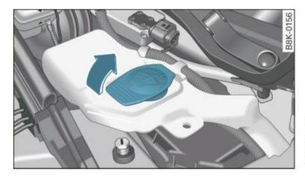
Fig. 205 Engine compartment: Windshield and headlight\* washer fluid container
