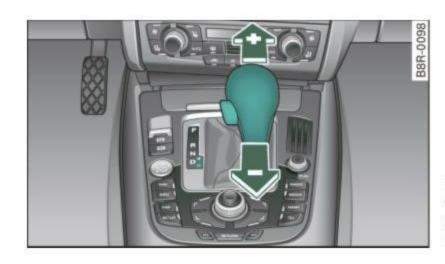
Fig. 142 Center console: shifting the multitronic/tiptronic manually
