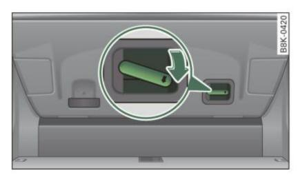
Fig. 213 Trunk escape handle: view from inside the closed trunk
