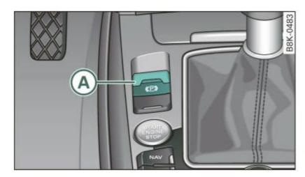
Fig. 103 Center console: Parking brake
