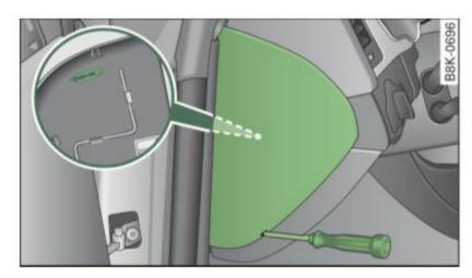
Fig. 223 Instrument panel left: Face cover
