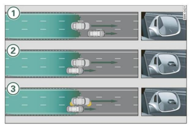
Fig. 133 Side assist: Vehicles dropping back quickly
