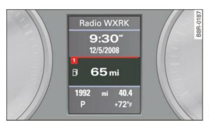
Fig. 16 Trip computer display: Fuel range
