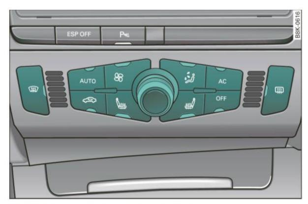
Fig. 90 Controls of the deluxe automatic climate control
