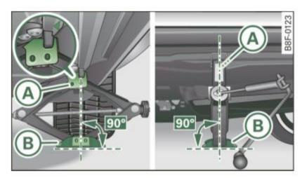
Fig. 220 Close-up: proper positioning of iack
