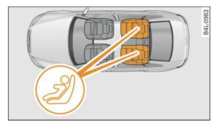
Fig. 185 Schematic overview: LATCH anchorage point locations
