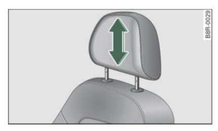
Fig. 68 Front seat: Adjusting the head restraint
