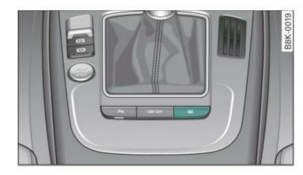
Fig. 57 without MMI: Button for rear window sun shade
