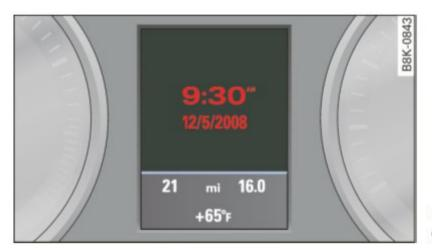
Fig. 4 Instrument cluster: time and date
