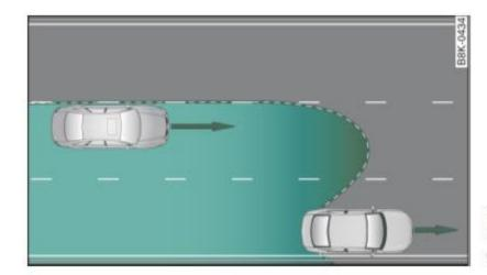
Fig. 134 Lanes of a normal width are in detection area
