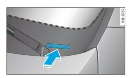
Fig. 235 Vehicle Identification Number (VIN) plate: location on driver's side dash panel
