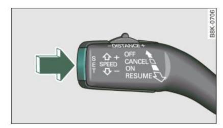
Fig. 109 Control lever: Storing speed
