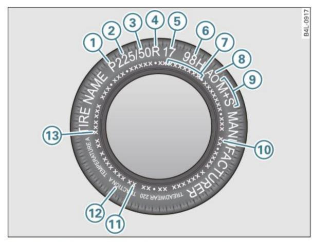
Fig. 210 Tire specification codes on the sidewall of a tire
