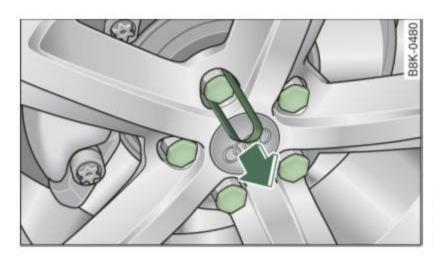
Fig. 217 Changing a wheel: removing the wheel bolt caps
