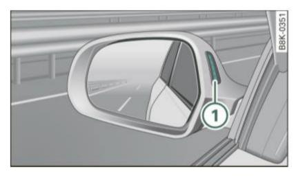
Fig. 127 Signal light on the outside mirror - driver's side
