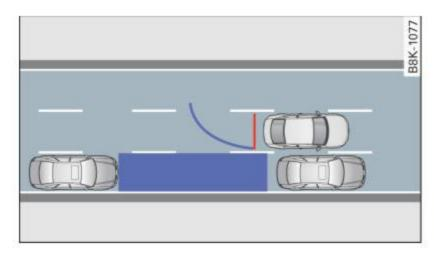
Fig. 148 Parking mode 2: parallel parking
