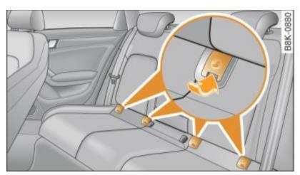
Fig. 186 Lower anchorages, covers marked
