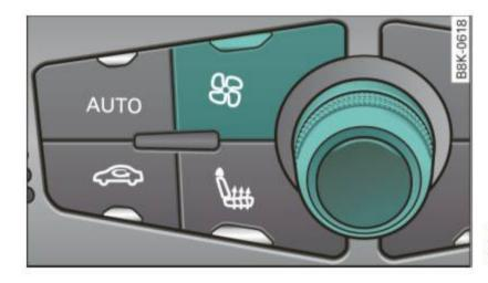
Fig. 92 Fan button and regulator
