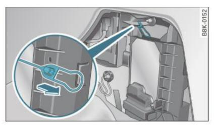
Fig. 196 Luggage compartment: Emergency opening of fuel filler flap
