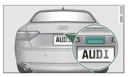
Fig. 39 Position of handle in the rear lid
