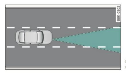
Fig. 107 Radar sensor measurement range
