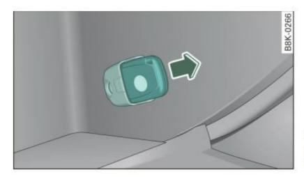
Fig. 30 Glove compartment: Adapter for emergency key
