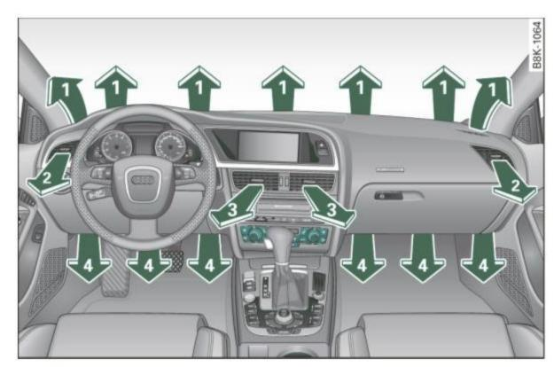
Fig. 98 Instrument panel: Location of air vents
