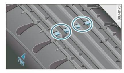
Fig. 208 Tire tread: tread wear indicators (TWI)
