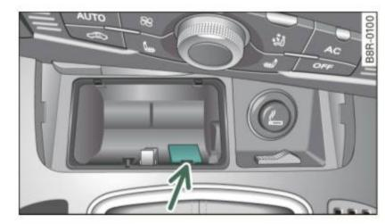
Fig. 146 Emergency release for selector lever
