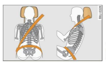
Fig. 169 Head restraint and safety belt position as seen from the side
