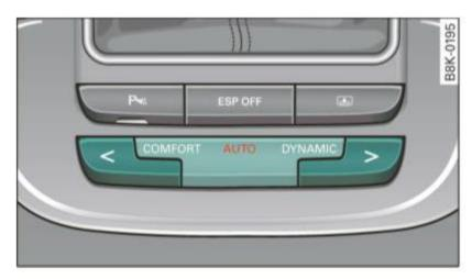
Fig. 136 Shift gate: Control for Audi drive select
