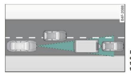
Fig. 120 Vehicle traveling ahead outside the detection range of the radar sensor
