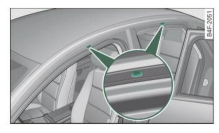
Fig. 81 Mounting locations for roof rack
