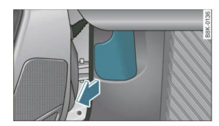
Fig. 197 Driver's side footwell: engine hood release lever
