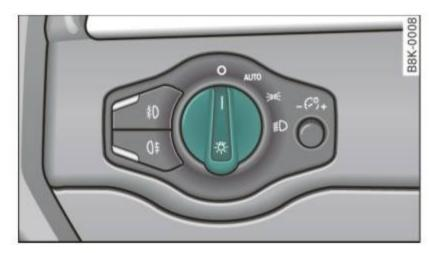
Fig. 47 Instrument panel: Headlight control switch
