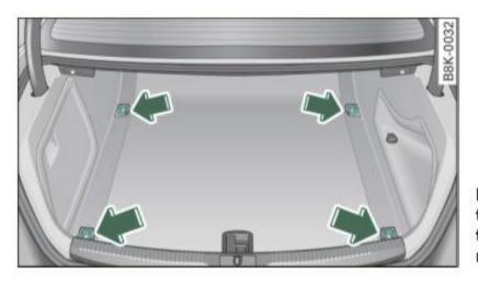
Fig. 74 Location of the tie-down rings in the luggage compart-
