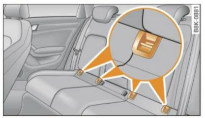
Fig. 187 Rear seats: lower anchorage bracket locations
