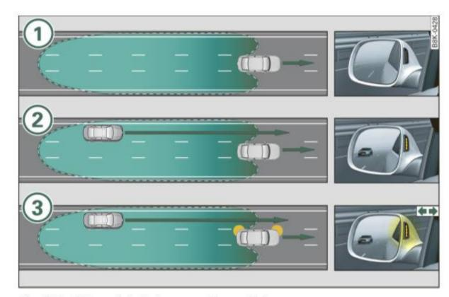
Fig. 130 Side assist: Fast approaching vehicles
