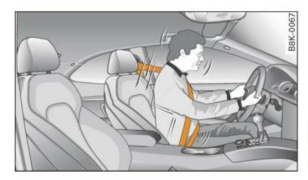
Fig. 167 Driver is correctly restrained in a sudden braking maneuver
