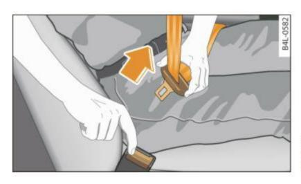
Fig. 171 Releasing the tongue from the buckle
