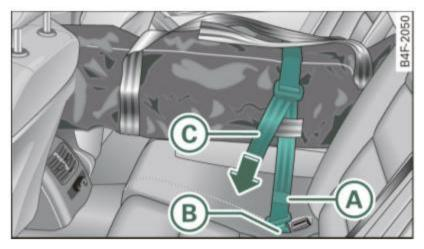
Fig. 80 Ski sack: securing with rear seat safety belt
