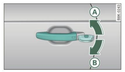
Fig. 42 Key turns for opening and closing
