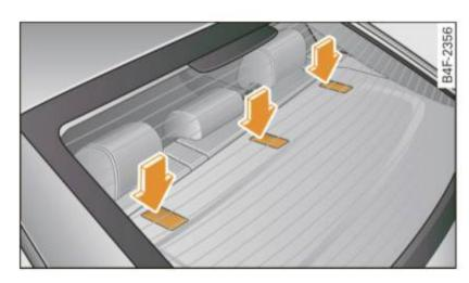
Fig. 189 Tether anchors: recess flaps behind the rear seatbacks
