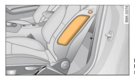
Fig. 177 Side airbag location in the driver's seat
