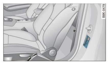
Fig. 206 Tire pressure label: located either on driver's side B-pillar or inside the fuel filler flap
