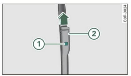
Fig. 60 Removing the wiper blade
