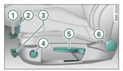
Fig. 65 Controls on the driver's seat
