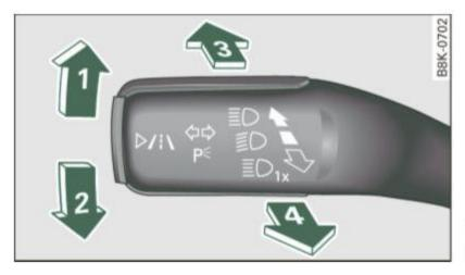
Fig. 52 Turn signal and high beam lever
