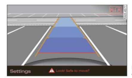
Fig. 152 MMI Display: Aligning the vehicle
