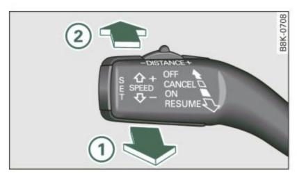
Fig. 111 Control lever: Turning adaptive cruise control off temporarily
