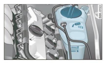
Fig. 202 Engine compartment: Coolant expansion tank
