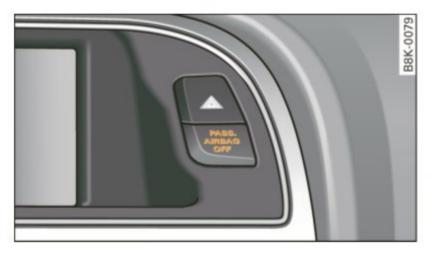
Fig. 176 Section from the instrument panel: PASSENGER AIRBAG OFF light
