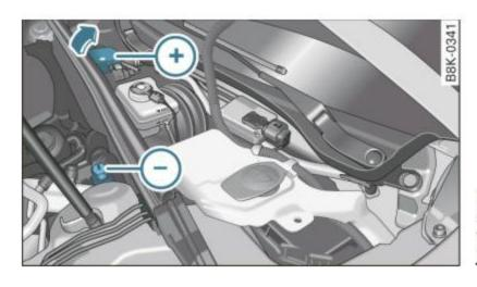
Fig. 204 Engine compartment: Connectors for charger and jumper cables
