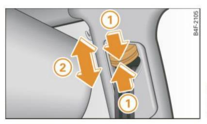
Fig. 172 Safety belt height adjustment for the front seats - looparound fittings
