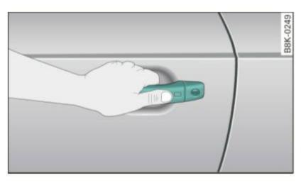
Fig. 33 Convenience key: Unlocking vehicle door
