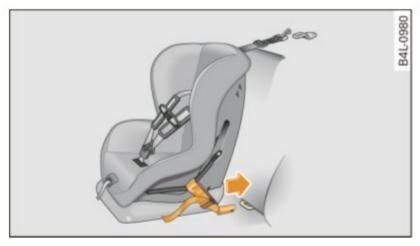
Fig. 188 Lower anchorages: proper mounting
