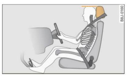
Fig. 159 Correct head restraint position for driver
