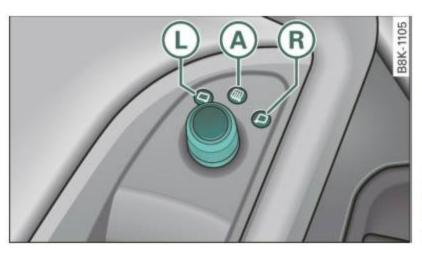
Fig. 62 Forward section of driver's armrest: power mirror controls
