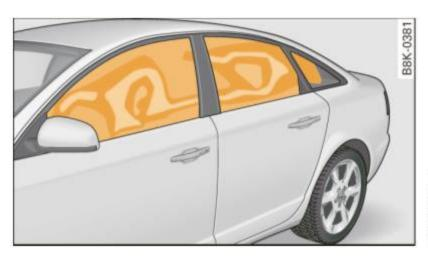
Fig. 180 Illustration of principle: Inflated side curtain airbags on the left side
