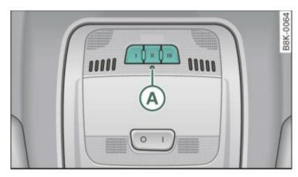
Fig. 155 Overhead console: HomeLink® keypad
