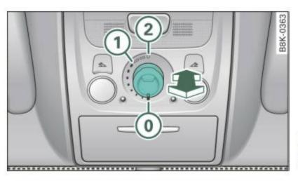
Fig. 44 Section of headliner: Knob for sliding/tilting sunroof
