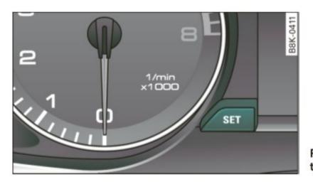
Fig. 20 SET button in the instrument cluster
