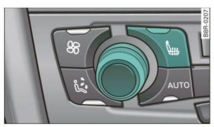
Fig. 99 Seat heating button and regulator
