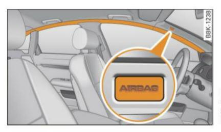
Fig. 179 Side curtain system, driver's side: side curtain airbag location
