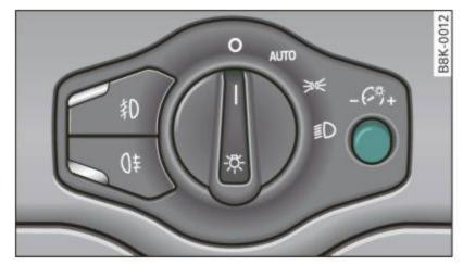
Fig. 49 Instrument lighting
