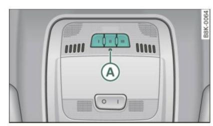
Fig. 157 Overhead console: HomeLink® keypad
