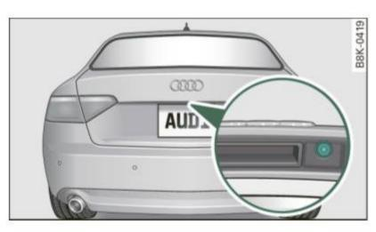
Fig. 150 Trunk lid: Location of the rear view camera
