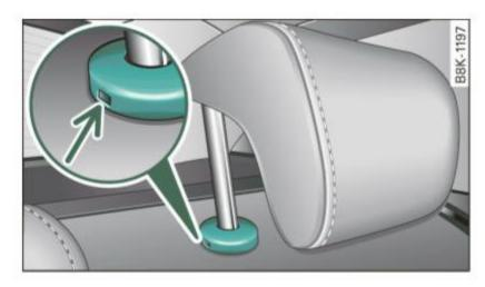
Fig. 71 Rear head restraints: release
