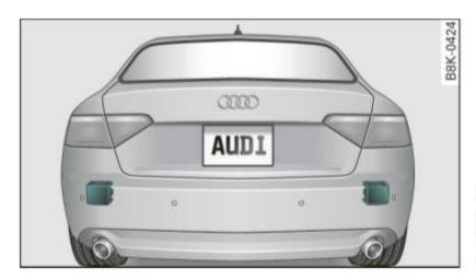
Fig. 126 Rear bumper: Position of radar sensors (not visible on outside)
