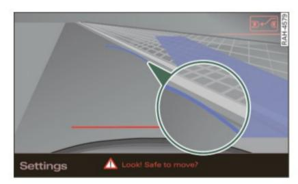
Fig. 154 MMI Display: Blue curve on the curb
