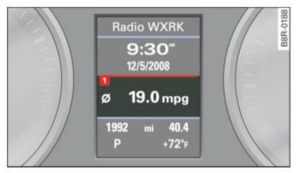
Fig. 17 Trip computer display: Average fuel mileage
