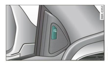
Fig. 128 Driver's door: Side assist button
