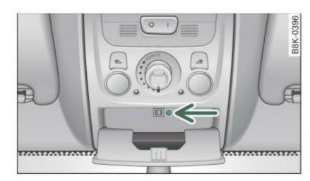
Fig. 45 Section from headliner: Unscrewing the lighting unit
