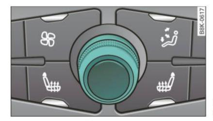
Fig. 91 Temperature setting regulator
