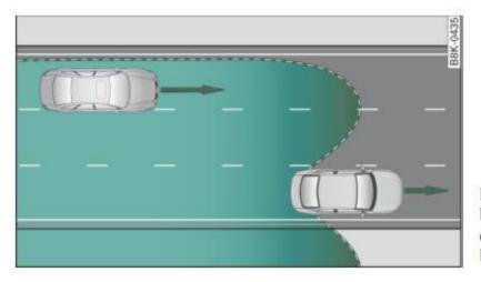
Fig. 135 Narrow lanes: Side assist may detect vehicles two lanes away
