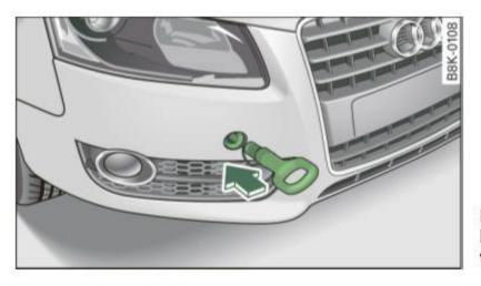
Fig. 230 Front bumper: screwing in the towing loop
