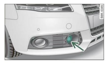
Fig. 106 Front bumper: Position of radar sensor
