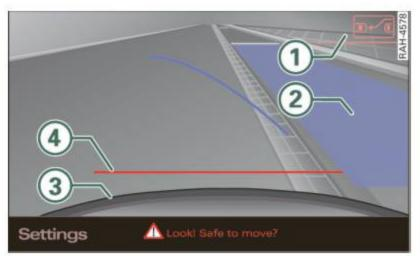
Fig. 153 MMI Display: blue surface in the parking spot
