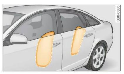
Fig. 178 Inflated side airbags on left side of vehicle
