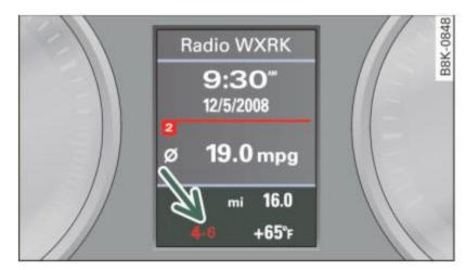
Fig. 11 Display: Gearshift indicator
