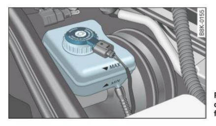
Fig. 203 Engine compartment: Brake fluid reservoir
