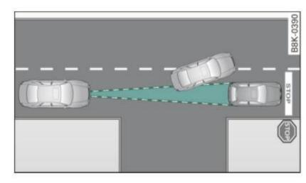
Fig. 124 Sheering out and stationary vehicle
