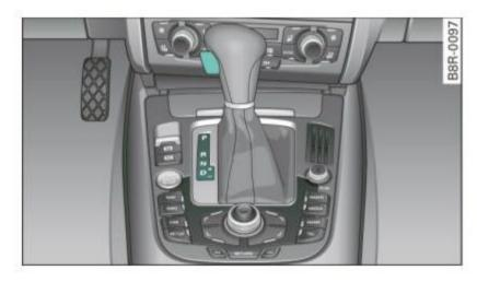
Fig. 139 Shift gate on the center console: selector lever with release button
