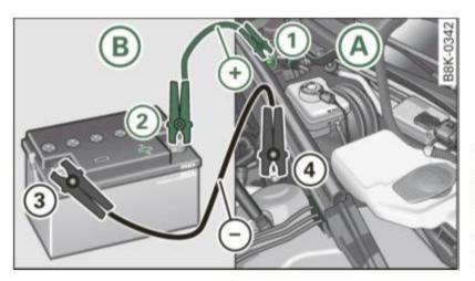
Fig. 228 Jump starting with the battery of another vehicle: (A) discharged vehicle battery, (B) booster battery
