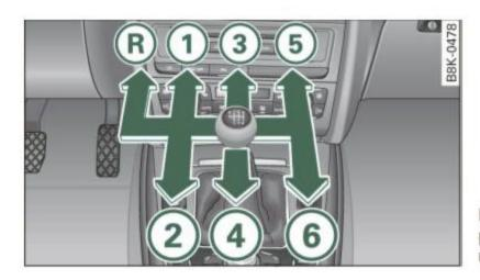
Fig. 138 Gearshift pattern: 6-speed manual transmission
