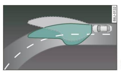
Fig. 50 Adaptive light when driving
