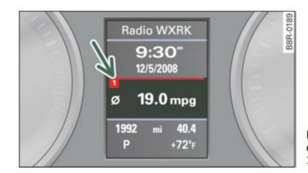
Fig. 18 Trip computer display: memory level 1
