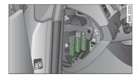
Fig. 224 Fuse panel layout
