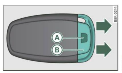
Fig. 26 Remote master key: Removing the mechanical key
