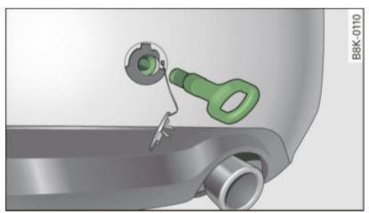
Fig. 231 Rear bumper: Screwing in towing loop
