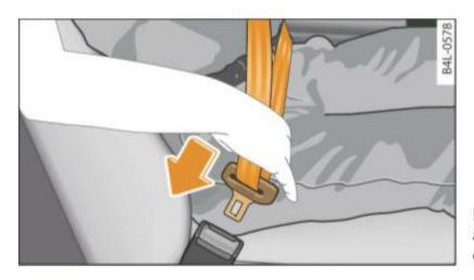
Fig. 168 Belt buckle and tongue on the driver's seat
