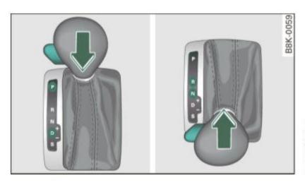
Fig. 141 Shift gate: selector lever lock positions and interlock button highlighted
