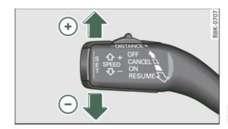
Fig. 110 Control lever: Changing speed
