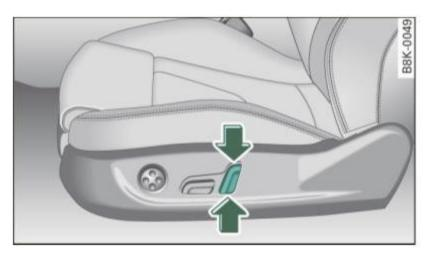
Fig. 69 Front seat: Adjusting head restraint electrically\*
