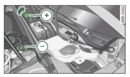
Fig. 227 Engine compartment: Connectors for jumper cables and charger
