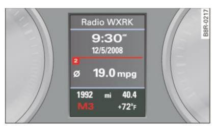
Fig. 143 Display: manual shift program, selected gear highlighted
