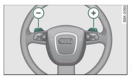
Fig. 144 Steering wheel: Shift buttons
