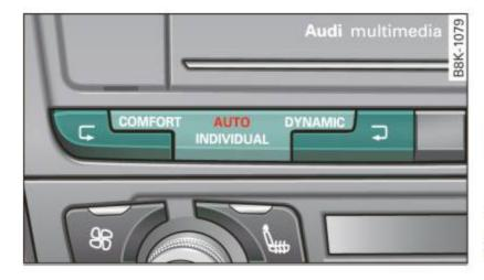
Fig. 137 Center console: Control for Audi drive select
