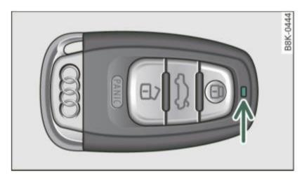
Fig. 25 Check light in the master key
