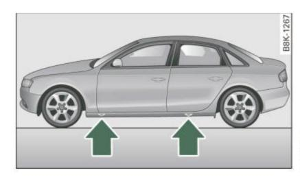
Fig. 219 Changing a wheel: mounting points for the jack
