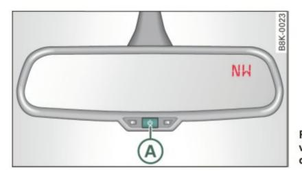
Fig. 63 Inside rear view mirror: digital compass activated
