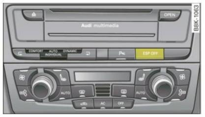
Fig. 192 Center console with ESP switch
