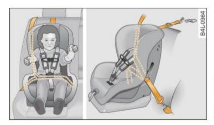
Fig. 183 Schematic overview: installation of the seat using the vehicle's safety belt system
