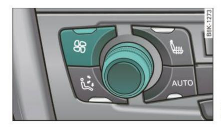
Fig. 96 Fan button and regulator
