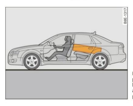
Fig. 161 Safe load positioning: place heavy objects as low and as far forward as possible.
