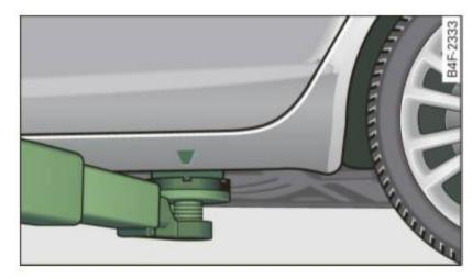
Fig. 234 Rear lifting point
