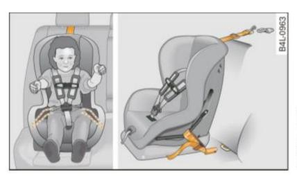
Fig. 182 Schematic overview: installation of the attachments applicable to a LATCH seat
