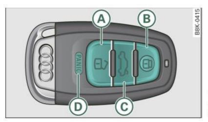
Fig. 32 Remote control: function buttons
