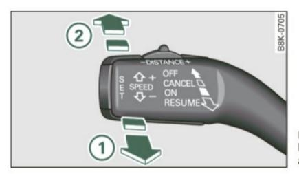
Fig. 108 Control lever: Switching on and off
