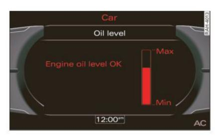
Fig. 200 MMI Display: Oil level indicator
