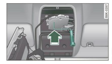
Fig. 46 Section from headliner: Crank for emergency operation
