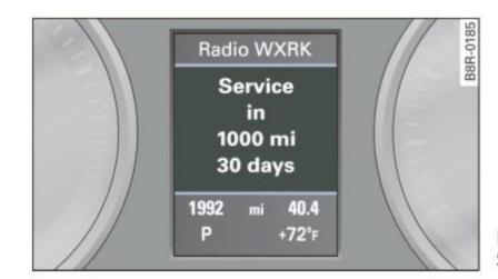
Fig. 14 Display: Service interval display
