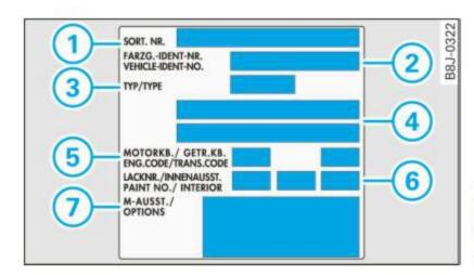
Fig. 236 The vehicle identification label - inside the luggage compartment
