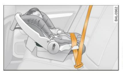
Fig. 181 Schematic overview: rearwardfacing infant seat, properly installed on the rear seat
