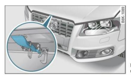
Fig. 198 Release lever under the engine hood
