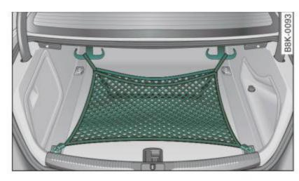
Fig. 76 Cargo net hooked up
