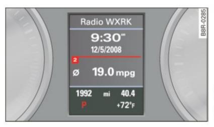
Fig. 140 Display in the instrument cluster: selector lever in position P
