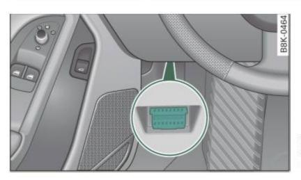
Fig. 15 Location of **Data Link Connector** (DLC)
