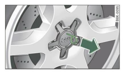
Fig. 216 Changing a wheel: removing the wheel cover
