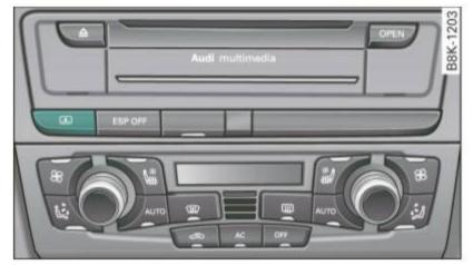
Fig. 56 with MMI: **Button for rear window** sun shade
