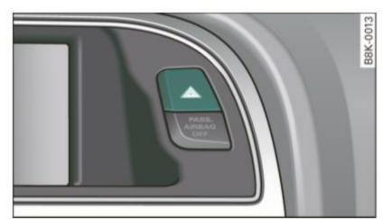
Fig. 51 Emergency flasher switch
