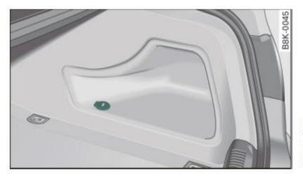
Fig. 86 Section of the trim panel of the luggage compartment: 12-volt socket
