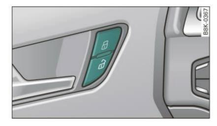
Fig. 36 Driver's door: power locking switch
