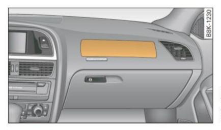
Fig. 174 Location of front passenger's airbag: in the instrument panel
