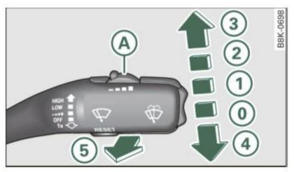
Fig. 58 Windshield wiper lever
