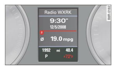
Fig. 10 Display: outside temperature
