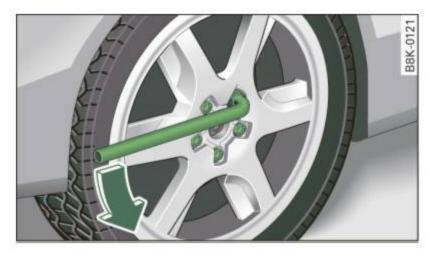
Fig. 218 Changing a wheel: loosening the wheel bolts
