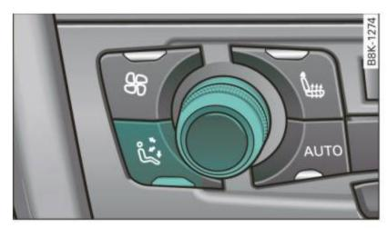
Fig. 97 Air distribution button and regulator
