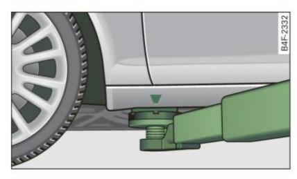
Fig. 233 Front lifting point
