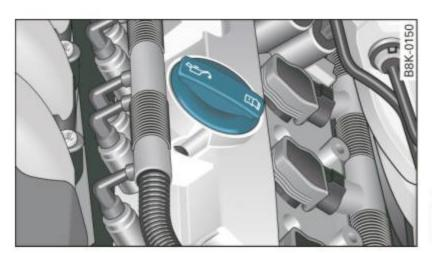
Fig. 201 Engine compartment: Oil filler cap location
