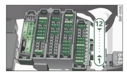
Fig. 226 Fuse panel layout
