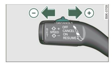
Fig. 112 Control lever: Setting distance
