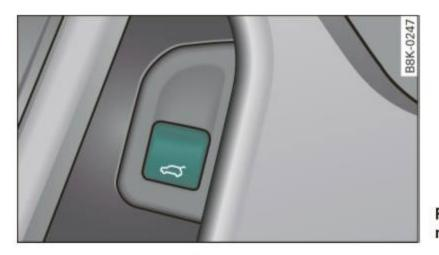
Fig. 38 Driver's door: remote rear lid release
