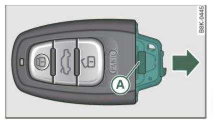
Fig. 27 Remote master key: Removing the battery holder
