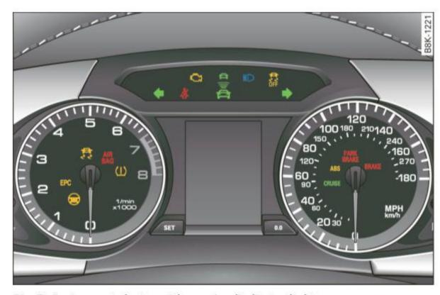
Fig. 7 Instrument cluster with warning/indicator lights
