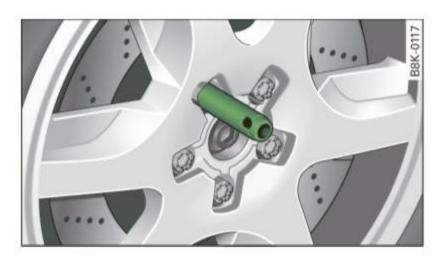
Fig. 222 Changing a wheel: alignment pin inside the top hole
