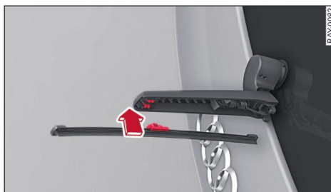
Fig. 46 Rear window wiper: Attaching the wiper blade
