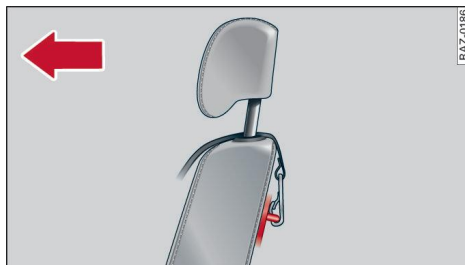
Fig. 66 Rear backrest: Hooking strap into top tether anchorage
