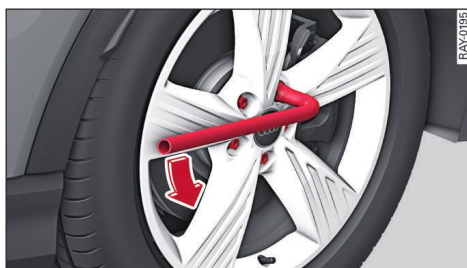
Fig. 172 Wheel: Loosening the wheel bolts
