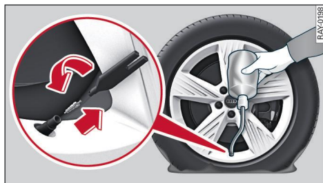
Fig. 169 Tyres: Filling the tyre
