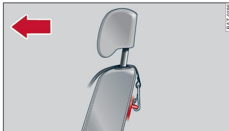
Fig. 68 Rear backrest: securing the upper belt to the top tether anchor
