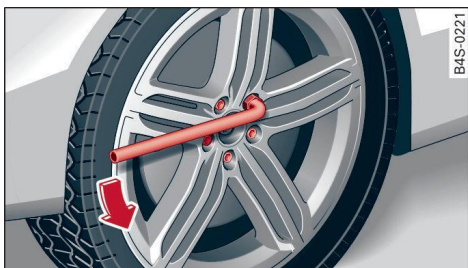
Fig. 163 Wheel: loosening the wheel bolts
