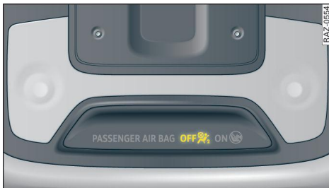
Fig. 65 Headliner: indicator light to display the status of the front passenger's airbag
