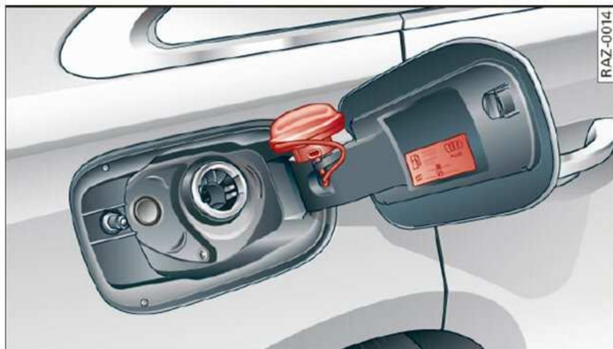
Fig. 137 Fuel filler door with attached fuel cap
