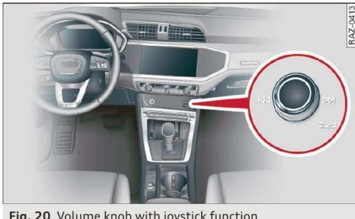
Fig. 20 Volume knob with joystick function
