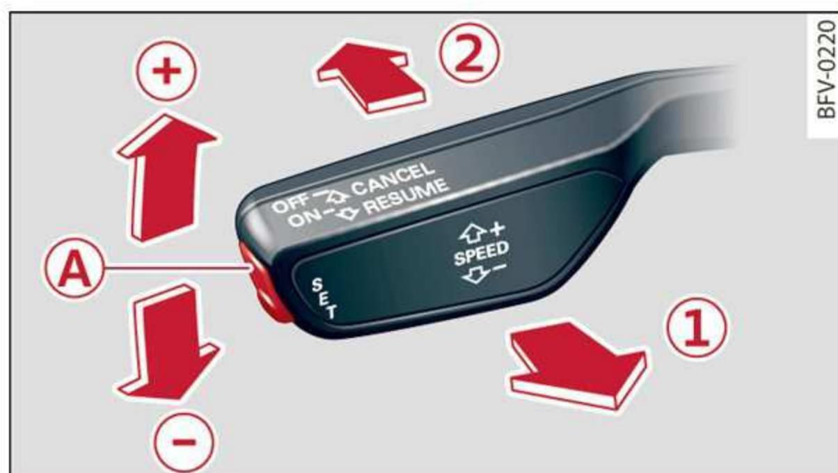
Fig. 90 Lever: switching on the cruise control system
