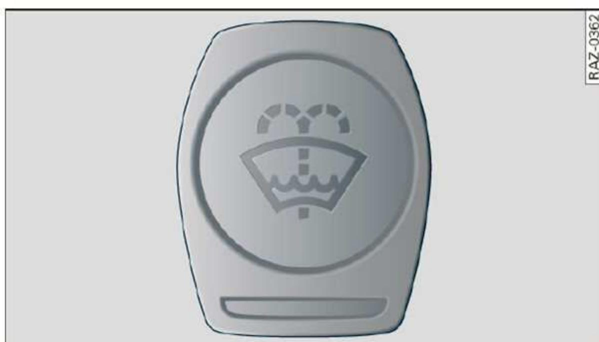
Fig. 147 Engine compartment: washer fluid reservoir cap
