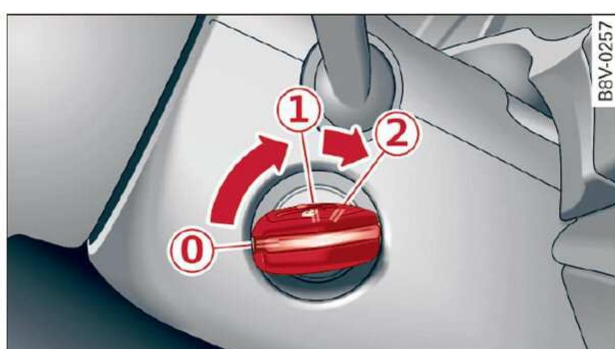
Fig. 79 Steering column: ignition lock
