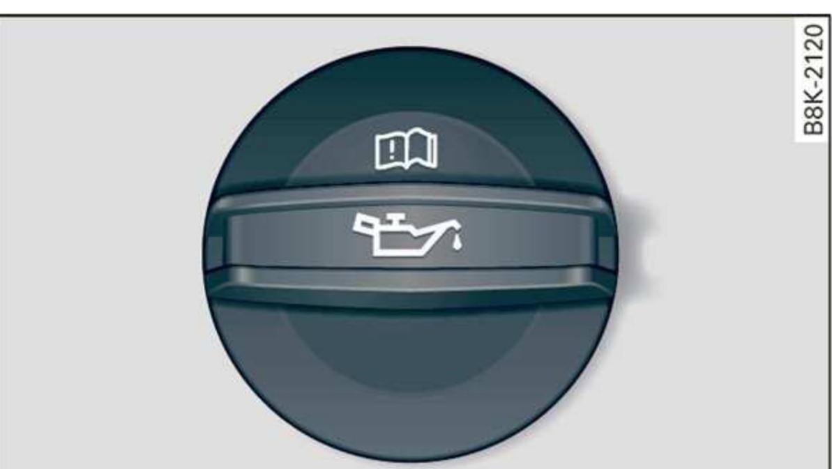
Fig. 143 Engine compartment: engine oil filler opening cover
