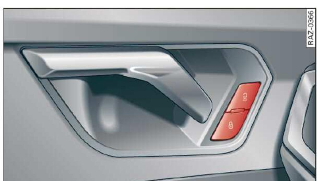
Fig. 21 Driver's door: central locking switch
