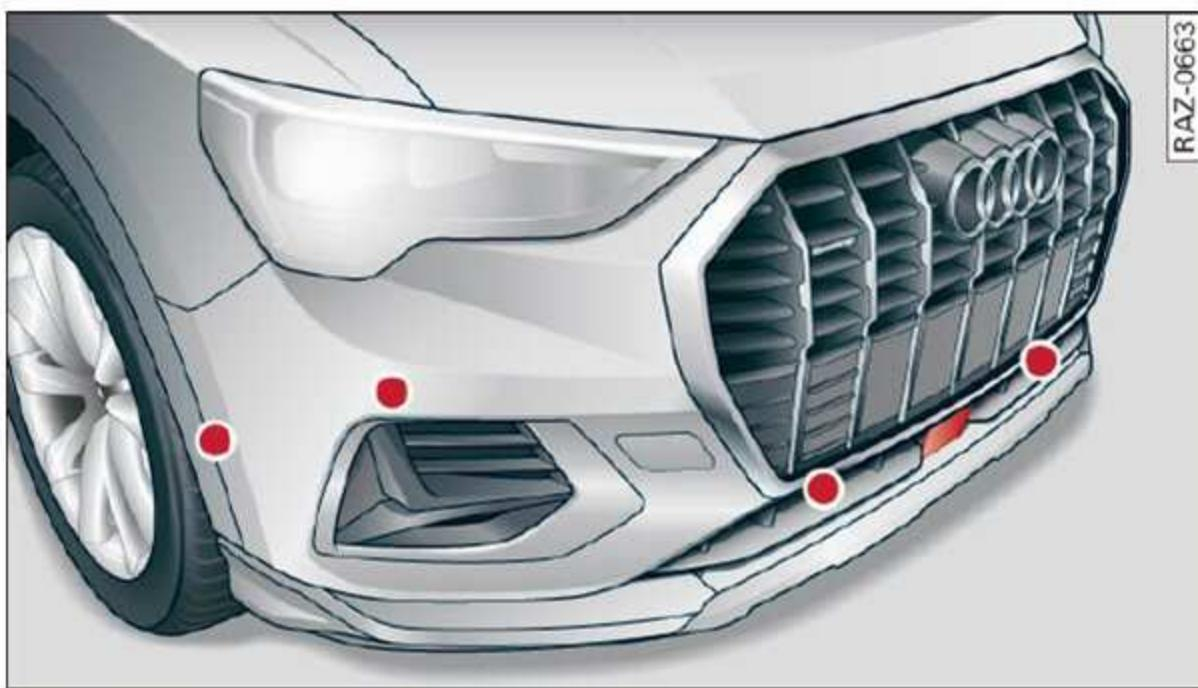
Fig. 86 Positions of the outer front sensors
