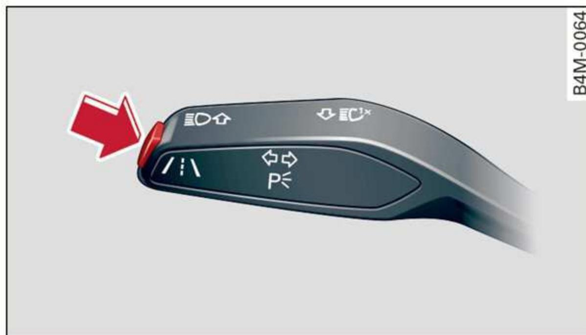
Fig. 103 Turn signal lever: switching the lane departure warning on or off
