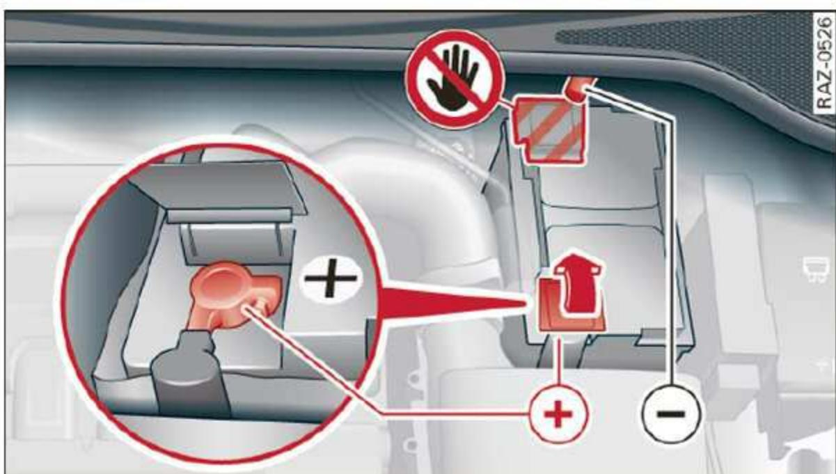
Fig. 146 Engine compartment with battery: connections for charger and jump start cable
