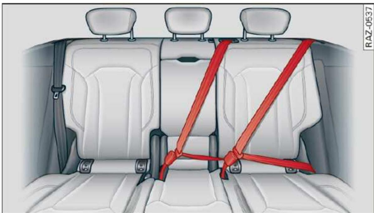
Fig. 67 Rear bench seat: securing unused safety belts
