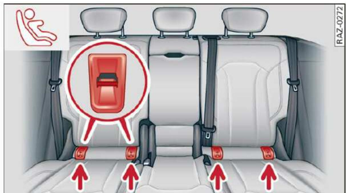
Fig. 64 Rear bench seat: lower LATCH anchors
