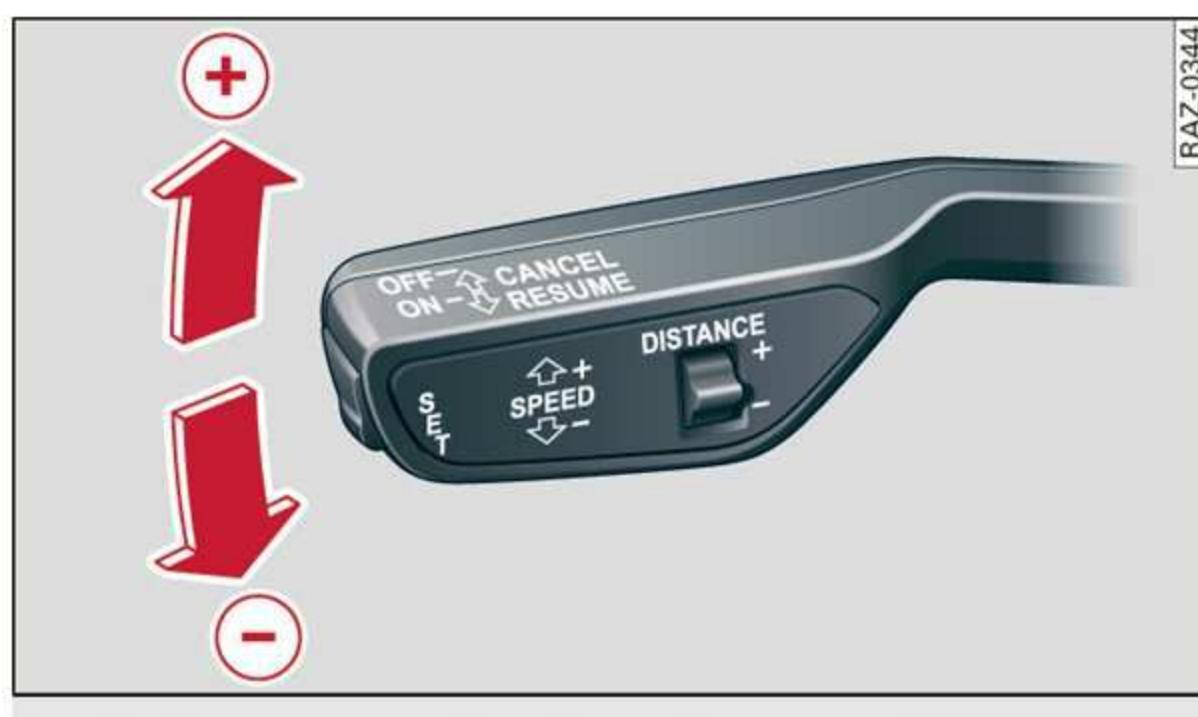
Fig. 96 Operating lever: changing the speed
