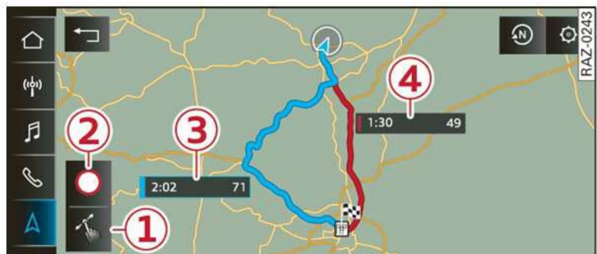
**Fig. 128** Center display: display of alternative routes in the overview map
