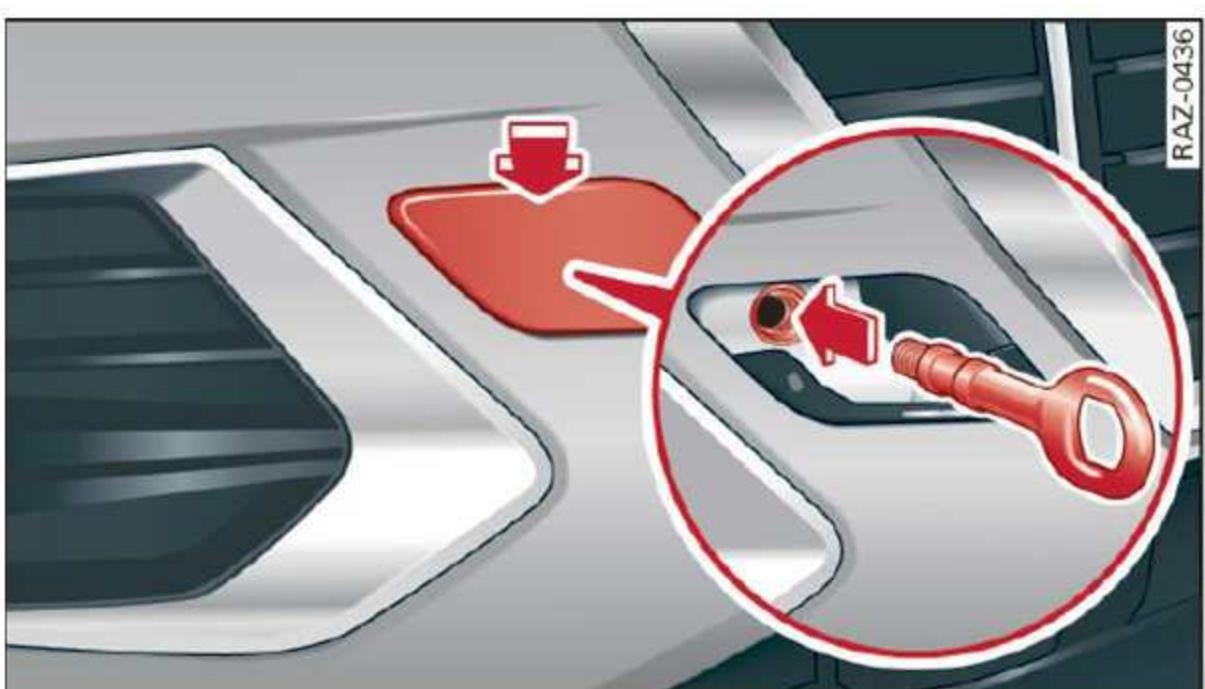
Fig. 163 Front bumper: installing the towing loop
