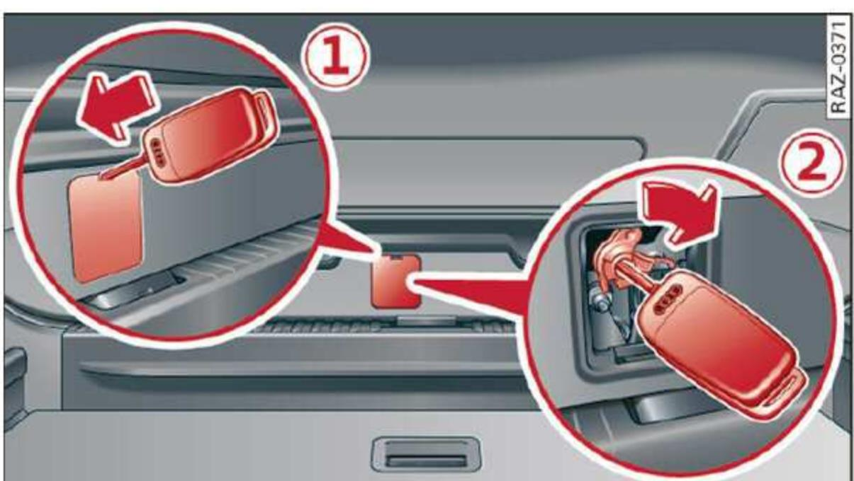
Fig. 31 Rear lid opening: access to the emergency release
