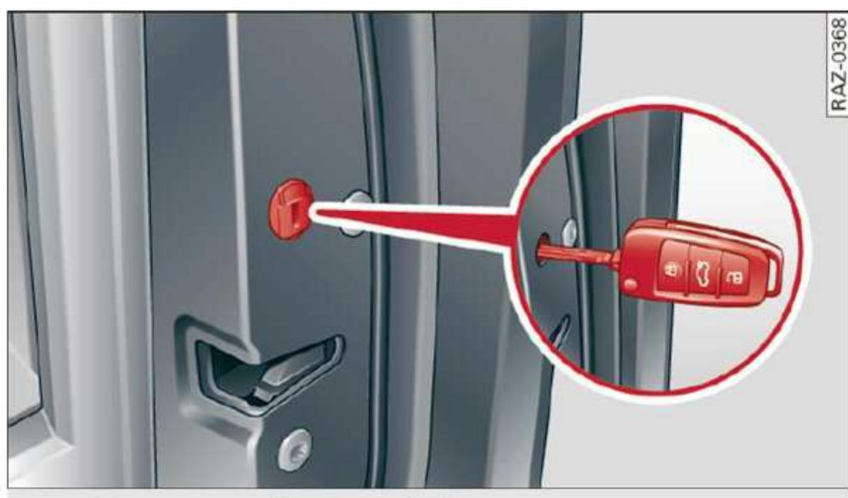
**Fig. 23** Door: mechanically locking
