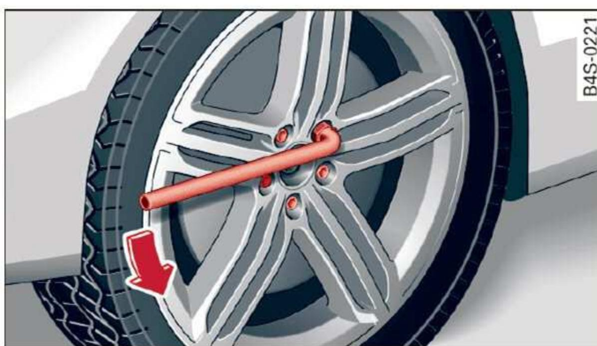
Fig. 155 Wheel: loosening the wheel bolt
