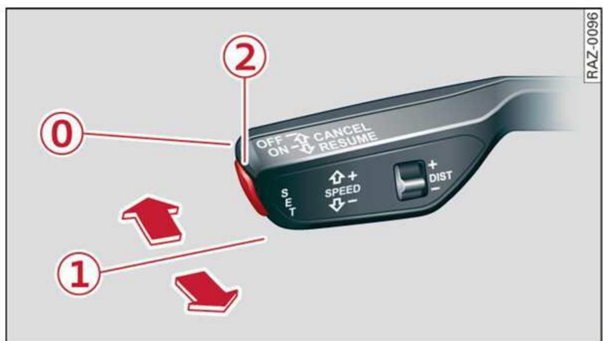
Fig. 98 Lever: overriding the control
