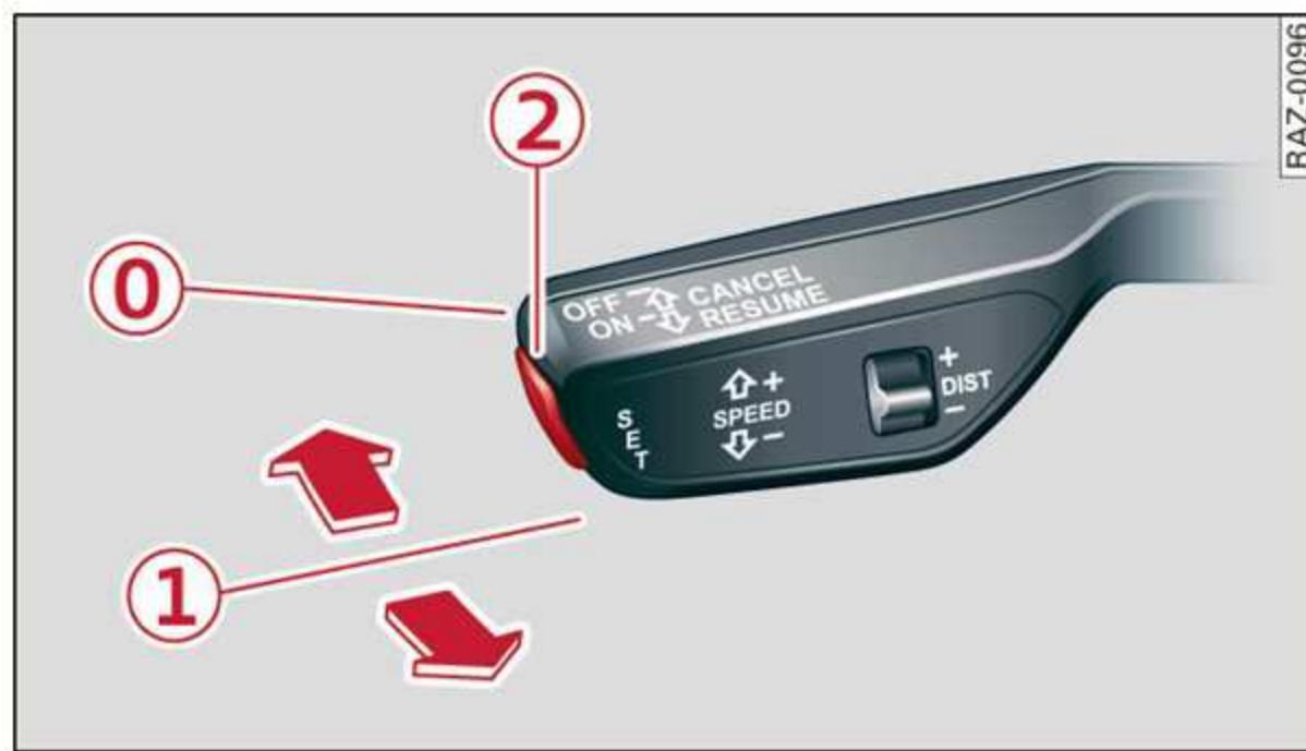
Fig. 95 Lever: using adaptive cruise assist
