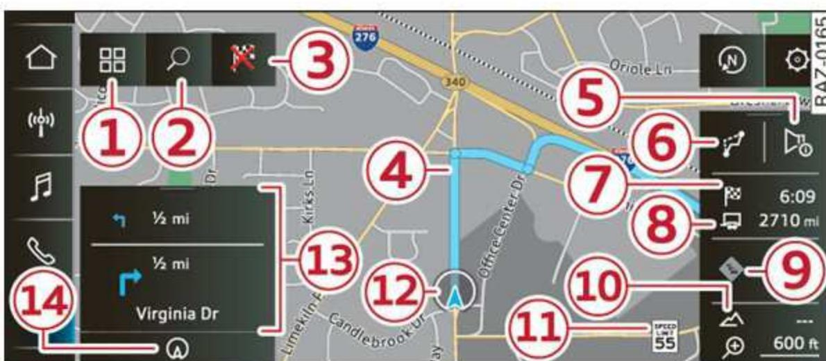
Fig. 125 Center display: diagram: active route guidance (standard map)
