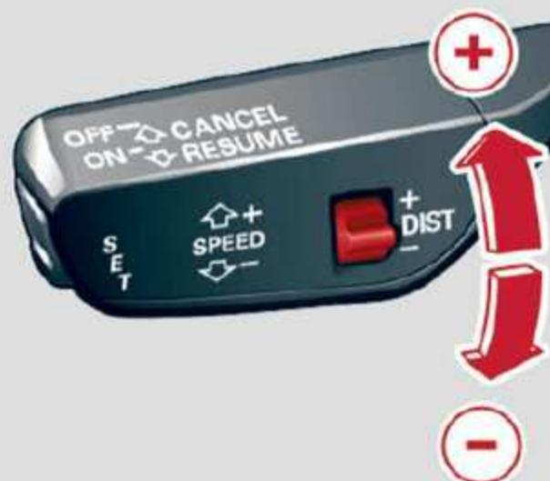
**Fig. 97** Operating lever: setting the distance
