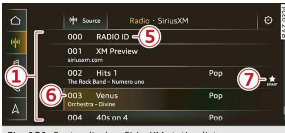
Fig. 131 Center display: SiriusXM station list
