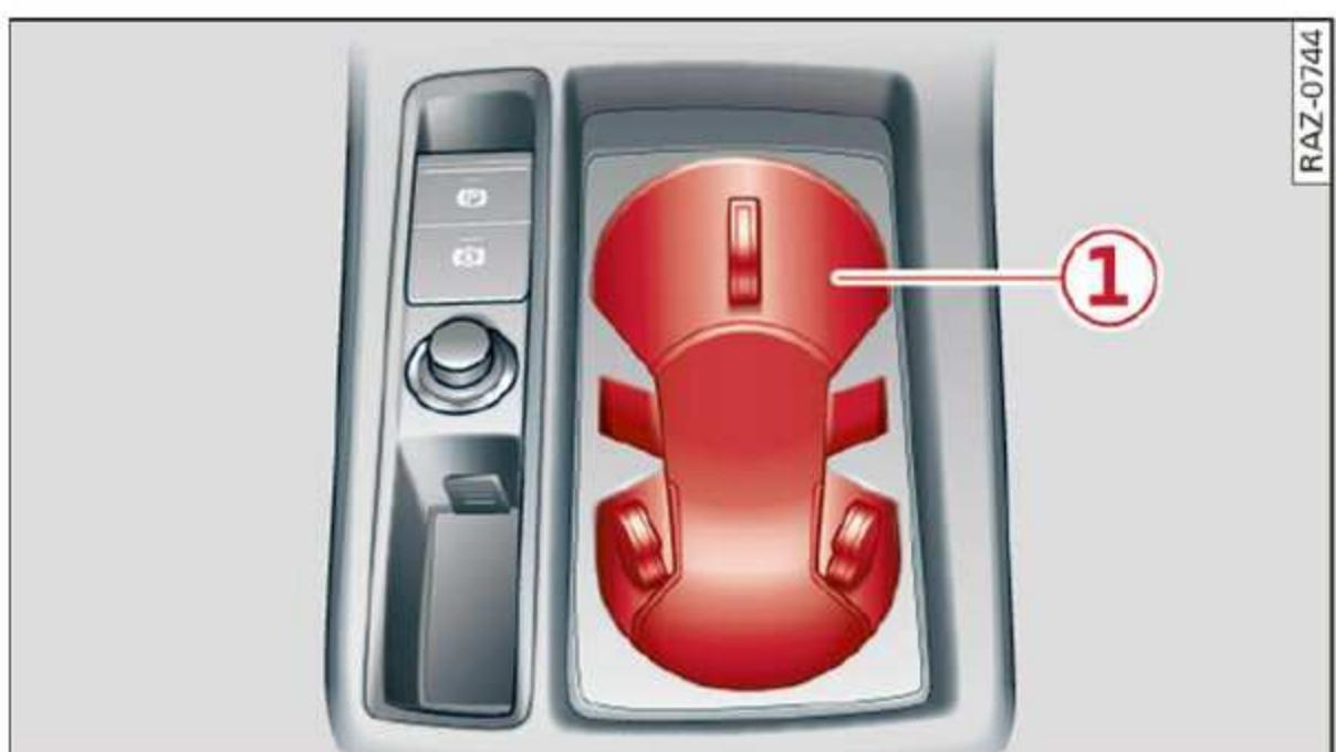
Fig. 68 Front center console: cup holder
