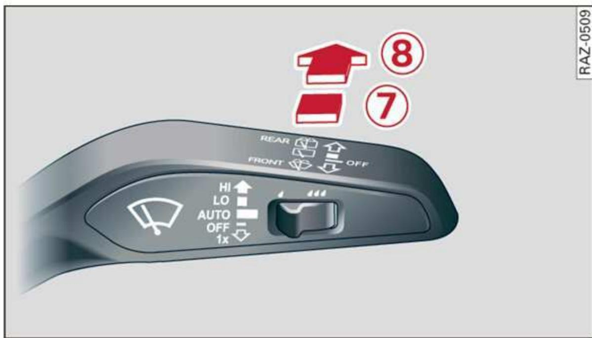
Fig. 44 Lever: rear window wiper
