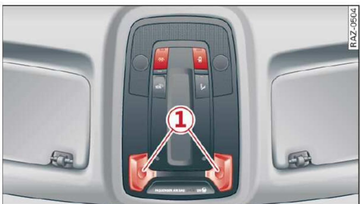
Fig. 39 Headliner: interior lighting
