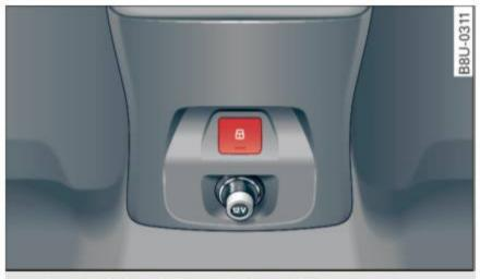
Fig. 19 Rear center console: central locking switch
