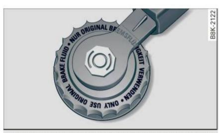
Fig. 144 Engine compartment: cap on brake fluid reservoir
