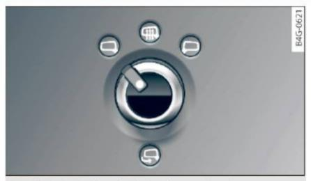
Fig. 38 Driver's door: knob for the exterior mirrors
