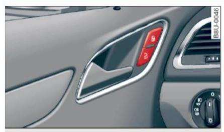
Fig. 18 Driver's door: central locking switch
