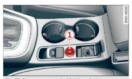
Fig. 53 Front center console: 12 Volt socket\*
