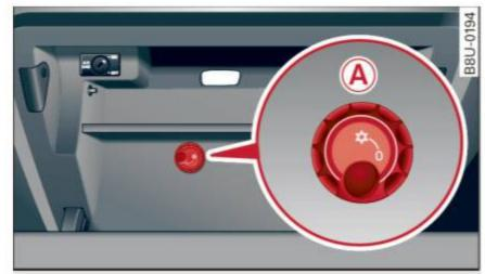
Fig. 56 Glove compartment: switching cooling mode\* on/
