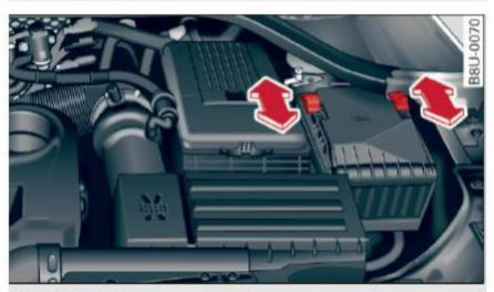
Fig. 163 Engine compartment: removing the fuse panel
