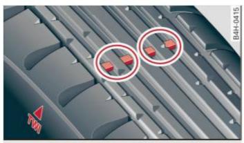
Fig. 148 Tire profile: treadwear indicator
