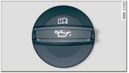
Fig. 142 Engine compartment: engine oil filler opening cover
