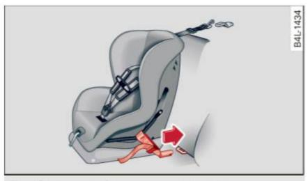
Fig. 131 Lower anchorages: proper mounting
