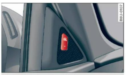
Fig. 85 Driver's door: side assist button
