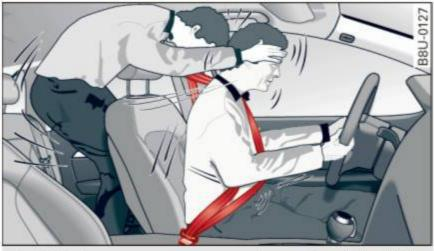
Fig. 108 A rear passenger not wearing a safety belt will fly forward and strike the driver
