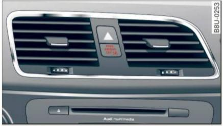
Fig. 118 Section from the instrument panel: PASSENGER AIR BAG OFF light
