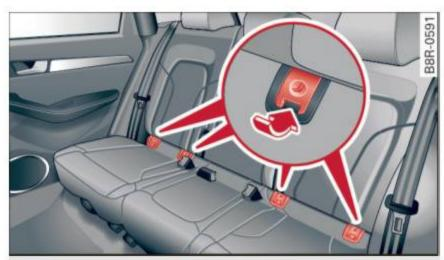
Fig. 129 Rear seats: lower anchorages, covers marked
