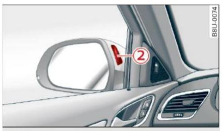
Fig. 82 Display on the exterior mirror
