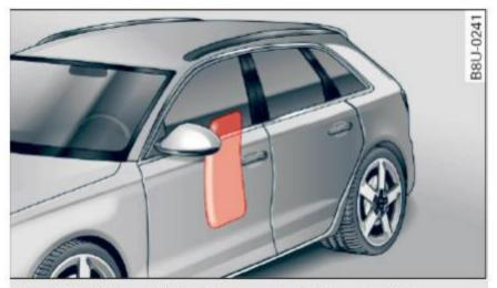
Fig. 120 Inflated side airbags on left side of vehicle
