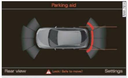
Fig. 90 Infotainment system: visual distance display
