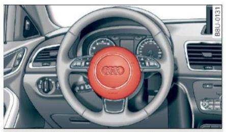
Fig. 115 Location of driver airbag: in steering wheel
