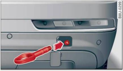
Fig. 169 Rear bumper: installing the towing loop
