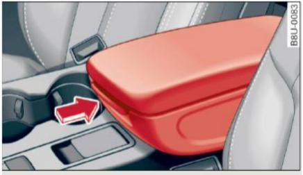
Fig. 49 Armrest between the driver's seat and passenger's seat
