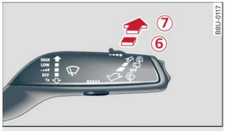
Fig. 42 Actuate the rear window wiper
