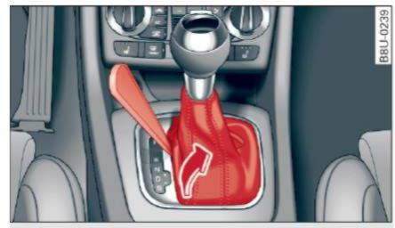
Fig. 77 Selector lever: removing the cover
