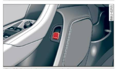
Fig. 23 Driver's door: opening the luggage compartment
