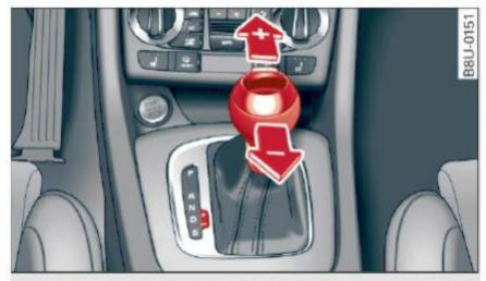
Fig. 75 Center console: shifting manually with the selector lever
