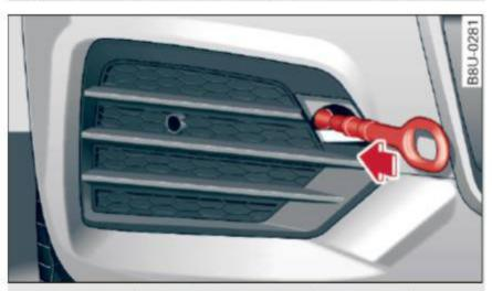
Fig. 167 Front bumper on the right side: screw in the towing loop
