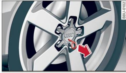
Fig. 153 Changing a wheel: removing the wheel cover
