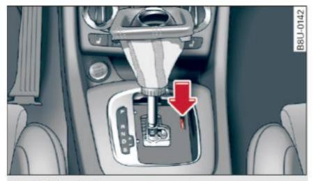
Fig. 78 Selector lever: emergency release
