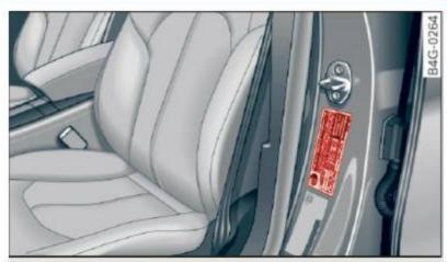
Fig. 149 Driver's side B-pillar: tire pressure label
