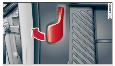
Fig. 138 Driver footwell: release lever
