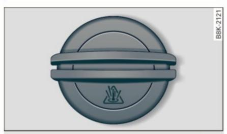
Fig. 143 Engine compartment: coolant expansion tank cover
