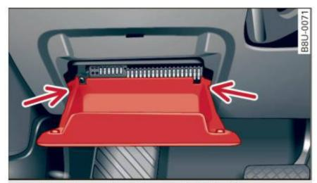
Fig. 162 Driver's side of the cockpit: folding the storage compartment down
