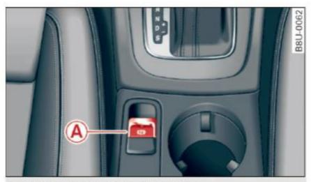
Fig. 72 Center console: parking brake
