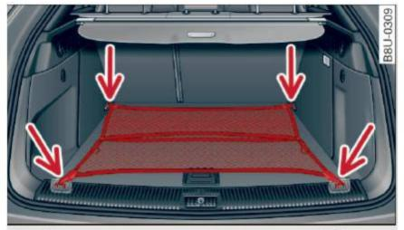
Fig. 60 Luggage compartment: cargo net stretched out
