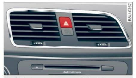
Fig. 34 Center console: emergency flasher button
