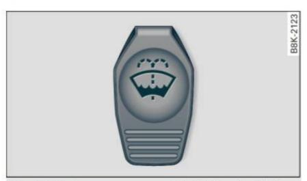
Fig. 146 Engine compartment: windshield washer fluid reservoir
