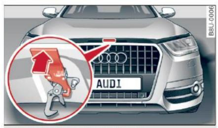
Fig. 139 Rocker switch under the hood
