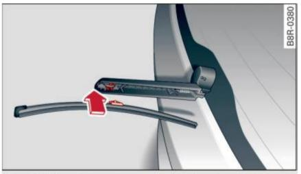
Fig. 44 Rear window wiper: removing the wiper blade
