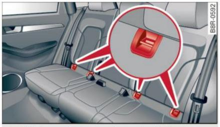
Fig. 130 Rear seats: lower anchorage bracket locations
