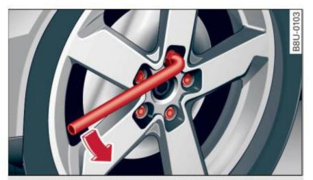
Fig. 155 Changing a wheel: loosening the wheel bolts
