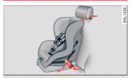
Fig. 133 Tether strap: proper routing and mounting
