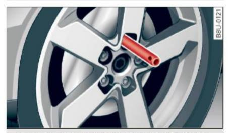
Fig. 171 Changing a wheel: alignment pin inside the top
