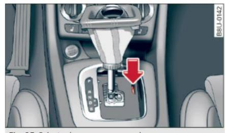
Fig. 95 Selector lever: emergency release
