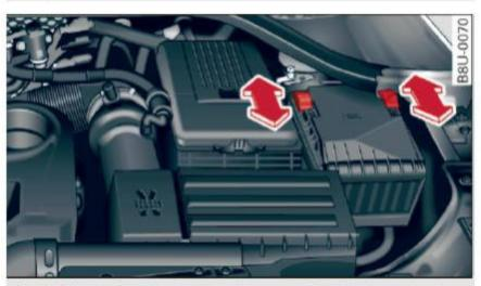
Fig. 173 Engine compartment: removing the fuse panel
