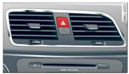
Fig. 38 Center console: emergency flasher switch
