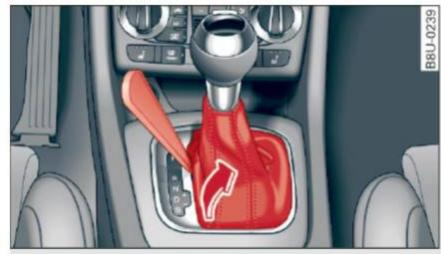
Fig. 94 Selector lever: removing the cover
