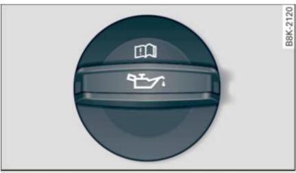
Fig. 151 Engine compartment: Cover on the oil filler neck
