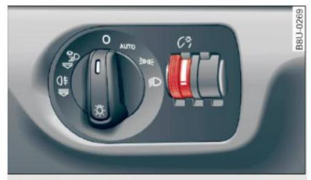
Fig. 41 Instrument illumination
