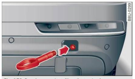
Fig. 179 Rear bumper: installing the towing loop
