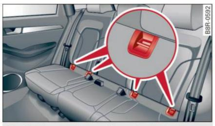
Fig. 136 Rear seats: lower anchorage bracket locations
