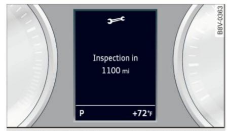
**Fig. 15** Instrument cluster: example of a service interval display
