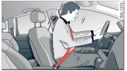
Fig. 115 Driver is correctly restrained in a sudden braking maneuver
