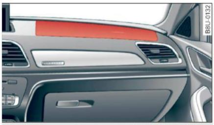
Fig. 122 Location of front passenger's airbag: in the instrument panel
