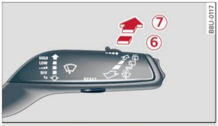
Fig. 46 Actuate the rear window wiper
