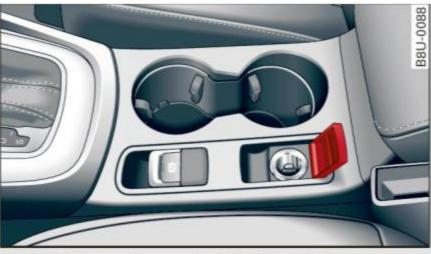
Fig. 59 Front center console: 12 Volt socket\*
