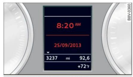
Fig. 9 Instrument cluster: time and date
