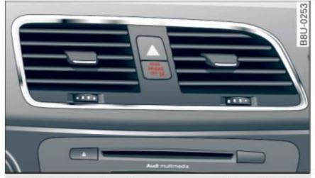
Fig. 124 Section from the instrument panel: PASSENGER AIR BAG OFF light
