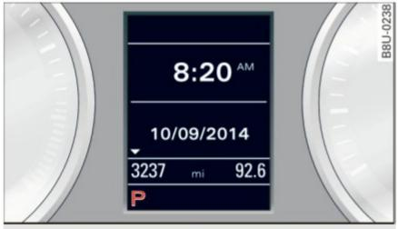
Fig. 90 Instrument cluster: selector lever positions
