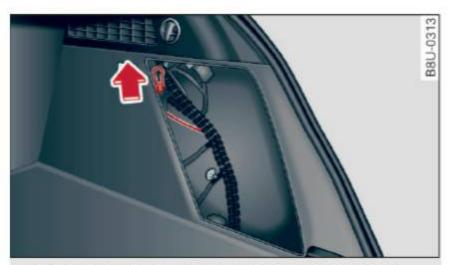
**Fig. 146** Side trim panel in the luggage compartment: emergency release mechanism
