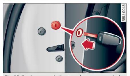
Fig. 25 Front passenger's door/rear door: emergency lock
