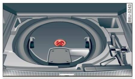
Fig. 164 Luggage compartment: space-saving spare tire (compact spare tire)
