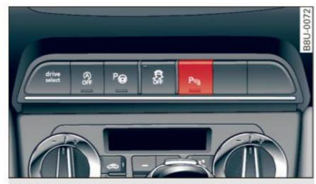
Fig. 97 Center console: parking system button
