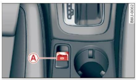
Fig. 81 Center console: parking brake
