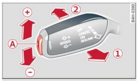
Fig. 82 Lever: cruise control system
