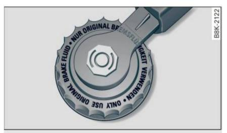
Fig. 153 Engine compartment: Cover on the brake fluid reservoir
