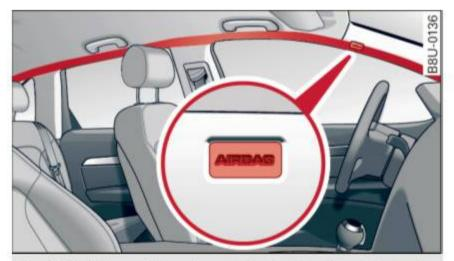
Fig. 127 Side curtain system, driver's side: side curtain airbag location
