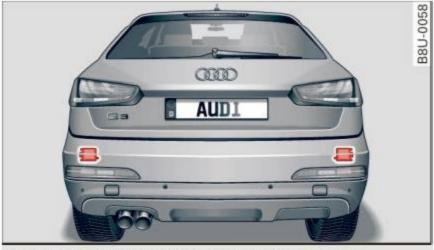
Fig. 86 Rear of the vehicle: position of the sensors
