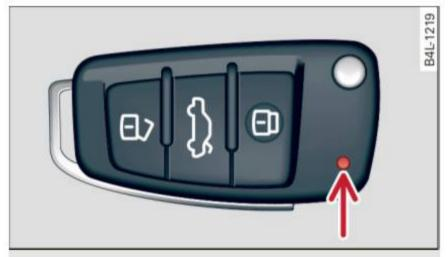
Fig. 18 Remote control key: LED
