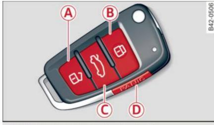
Fig. 20 Remote master key: function buttons
