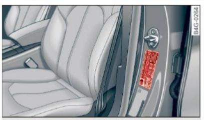
Fig. 158 Driver's side B-pillar: tire pressure label
