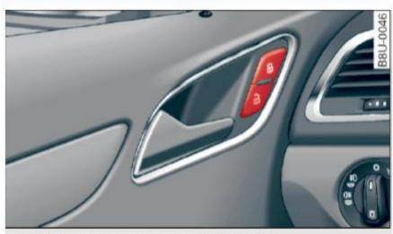
Fig. 22 Driver's door: power locking switch
