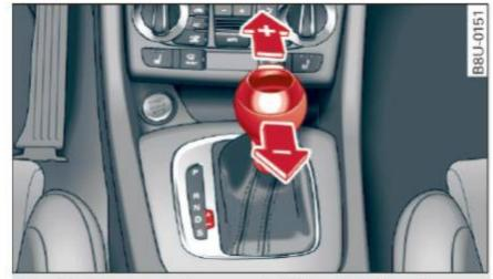
Fig. 92 Center console: manual shifting with the selector lever
