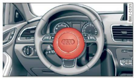
Fig. 121 Location of driver airbag: in steering wheel
