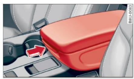
Fig. 53 Armrest between the driver's seat and passenger's seat
