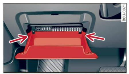
Fig. 172 Driver's side of the cockpit: folding the storage compartment down
