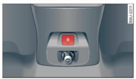
Fig. 23 Rear center console: power locking switch
