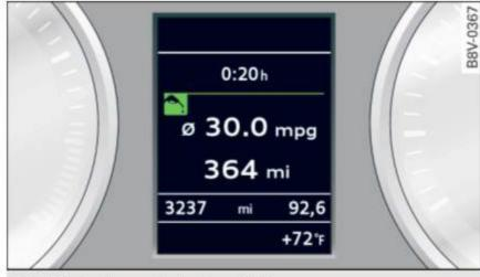
Fig. 12 Instrument cluster: efficiency program
