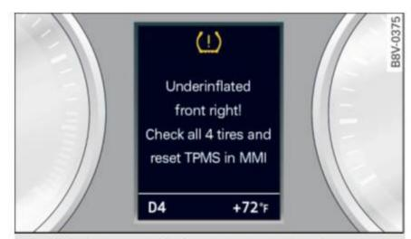
Fig. 160 Instrument cluster: indicator light with message
