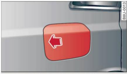
Fig. 144 Right rear vehicle side: Opening the fuel filler flap
