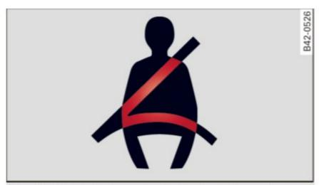
Fig. 110 Safety belt warning light in the instrument cluster - enlarged
