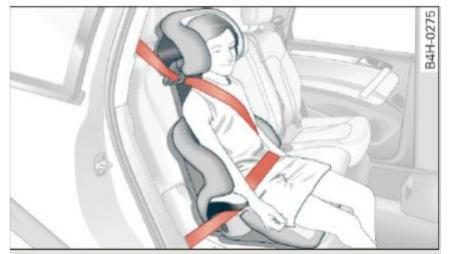
Fig. 133 Rear seat: child properly restrained in a booster seat
