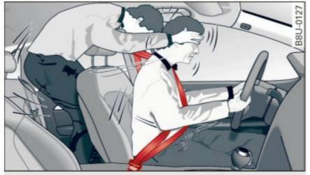
Fig. 114 A rear passenger not wearing a safety belt will fly forward and strike the driver
