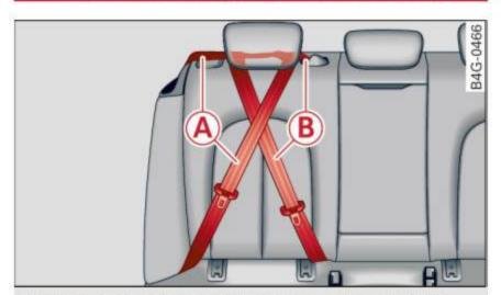
Fig. 129 Schematic overview: keep unused safety belts away from children in child safety seats. (A) - outer rear safety belt, (B) - center rear safety belt
