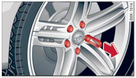
Fig. 166 Changing a wheel: removing the wheel bolt caps
