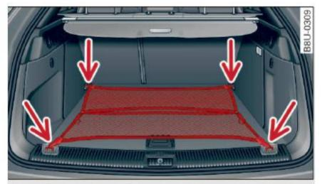
Fig. 70 Luggage compartment: cargo net stretched out
