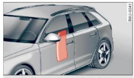
Fig. 126 Inflated side airbags on left side of vehicle
