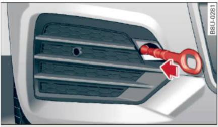
**Fig. 177** Front bumper on the right side: screw in the towing loop
