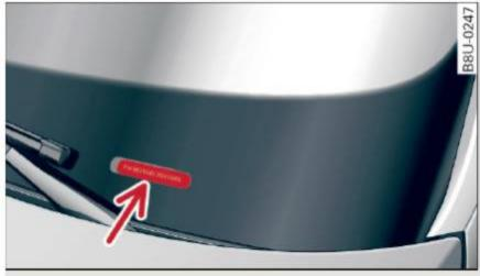
Fig. 183 Location on driver's side dash panel: Vehicle Identification Number (VIN) plate
