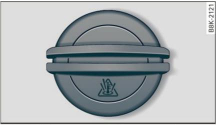
Fig. 152 Engine compartment: Cover on the coolant expansion tank
