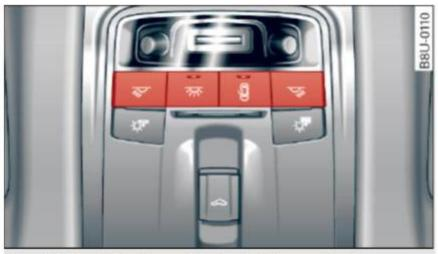
Fig. 39 Front headliner: interior lighting controls
