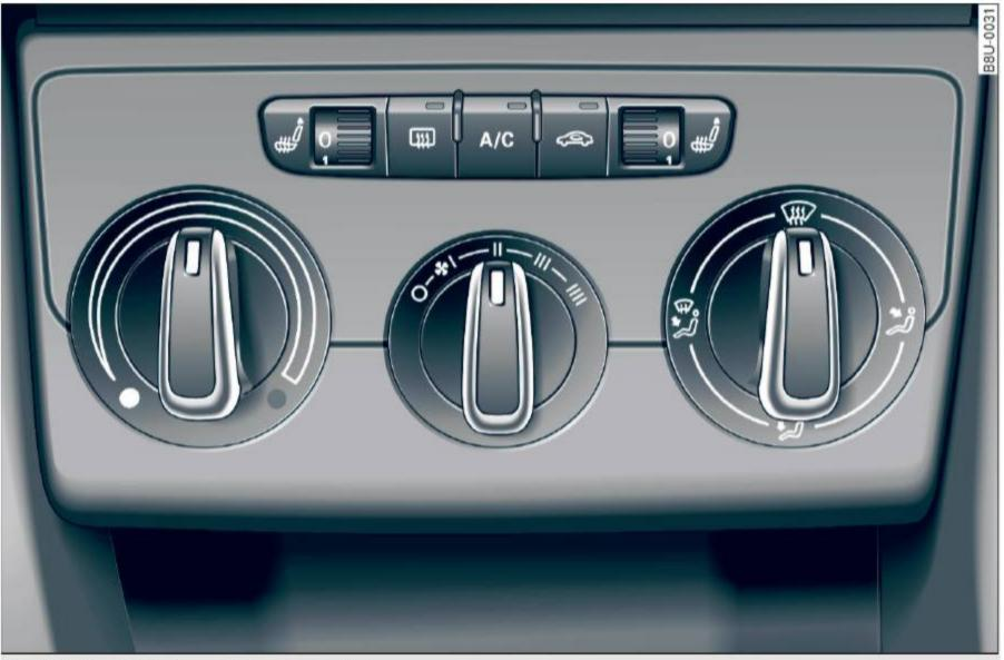
Fig. 75 Manual climate control system controls
