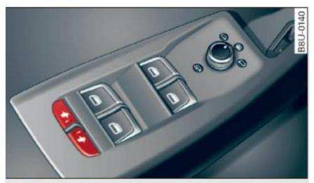
Fig. 31 Section of driver's door: controls
