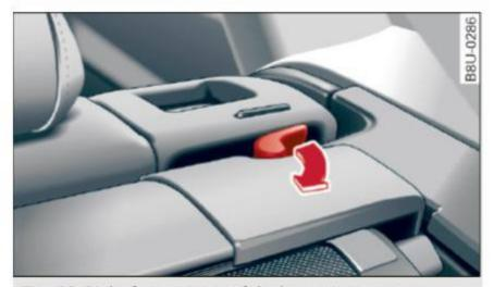
**Fig. 68** Right front section of the luggage compartment: removing the luggage compartment cover
