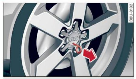
Fig. 165 Changing a wheel: removing the wheel cover
