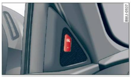
Fig. 87 Driver's door: side assist button
