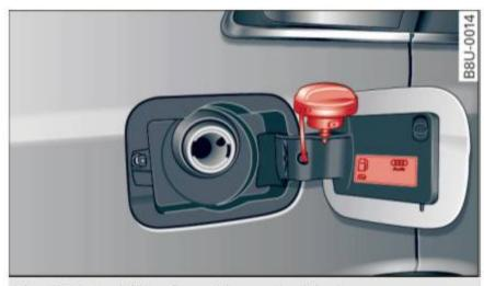
Fig. 145 Fuel filler flap with attached fuel cap
