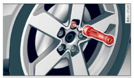
Fig. 170 Changing a wheel: using the hexagonal socket (with the blade removed) to turn the bolts
