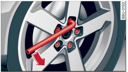
Fig. 167 Changing a wheel: loosening the wheel bolts
