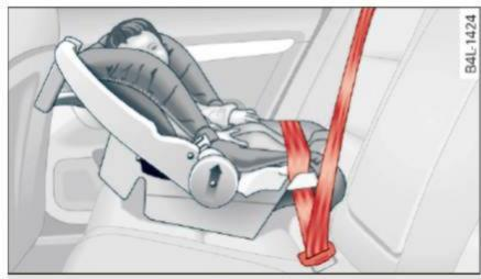
Fig. 130 Schematic overview: rearward-facing infant seat, properly installed on the rear seat
