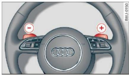
Fig. 93 Steering wheel: manual shifting with the shift paddles\*
