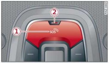
Fig. 148 Front headliner: cover for the emergency call but-
