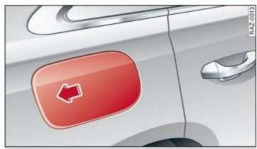
Fig. 164 Right rear side of the vehicle: opening the fuel filler door
