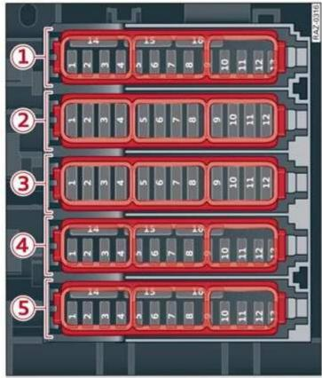
Fig. 197 Front passenger's footwell (right-hand drive vehicle): fuse panel with plastic clip
