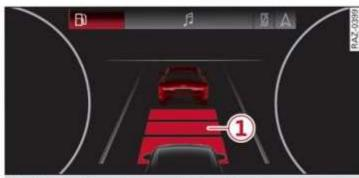
Applies to: driver assistance display without area view Fig. 111 Instrument cluster: brake intervention request
