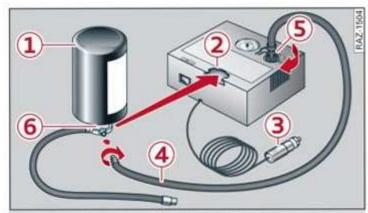
Fig. 181 Components of the tire mobility kit
