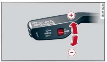
Fig. 114 Operating lever: setting the distance
