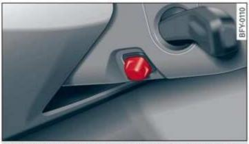
Fig. 60 Steering column: switch for adjusting the steering wheel position
