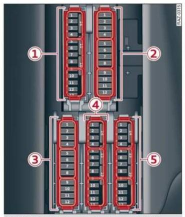
Fig. 196 Driver's footwell (left-hand drive vehicle): fuse panel with plastic clip
