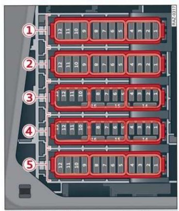
Fig. 199 Left side of the luggage compartment: fuse panel with plastic clip
