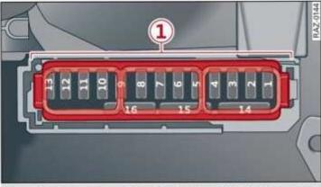
Fig. 198 Driver side cockpit: fuse panel with plastic bracket
