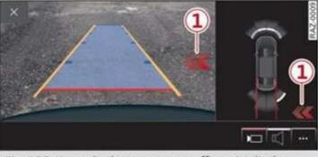
Fig. 137 Upper display: rear cross-traffic assist display
