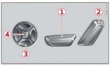
Fig. 52 Front seat: seat adjustment buttons
