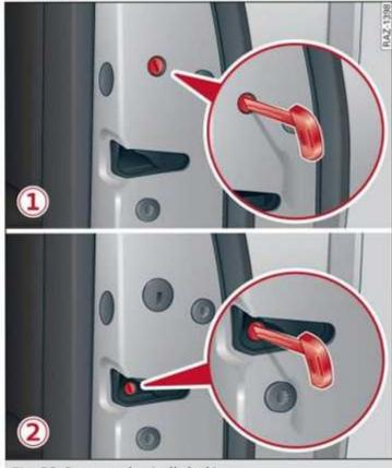
Fig. 23 Door: mechanically locking
