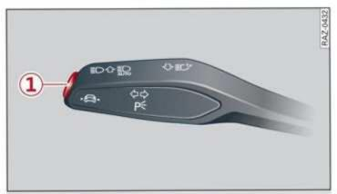
Fig. 121 Turn signal lever: button for lane departure warning and lane guidance for adaptive cruise assist\*
