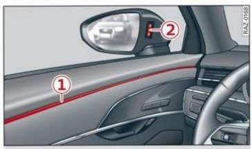
Fig. 126 Front door: warning strip
