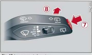
Fig. 47 Lever: rear window wiper
