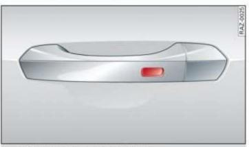
Fig. 25 Door handle: sensor for locking
