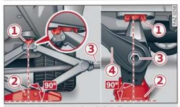
Fig. 187 Sill: positioning the vehicle jack
