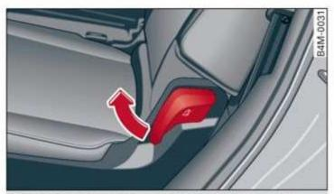
Fig. 55 Second row seats: adjusting the backrest angle
