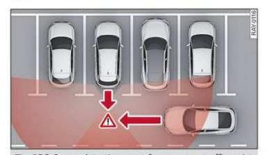
Fig. 136 Sensor detection range for rear cross-traffic assist
