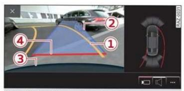
Fig. 133 Upper display: aiming at a parking space
