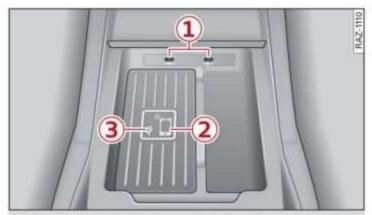
Fig. 145 Storage compartment under the center armrest: Audi phone box with connections
