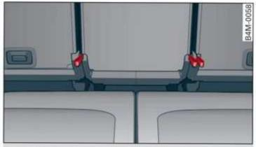
Fig. 82 Luggage compartment: release straps\*
