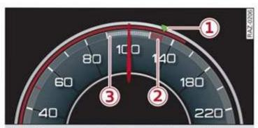
Fig. 113 Instrument cluster: speedometer: predictive control display
