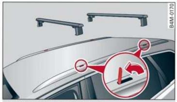
Fig. 86 Roof rail: mounting points
