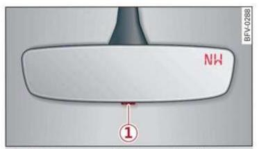
Fig. 50 Rearview mirror: digital compass is switched on
