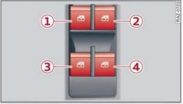
Fig. 33 Driver's door: power window switch
