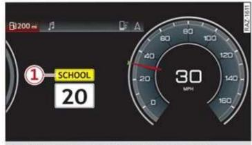
Fig. 101 Instrument cluster: traffic sign recognition
