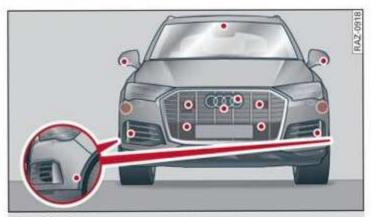
Fig. 97 Front area: sensors and cameras
