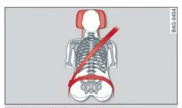
Fig. 61 Correctly-adjusted head restraint
