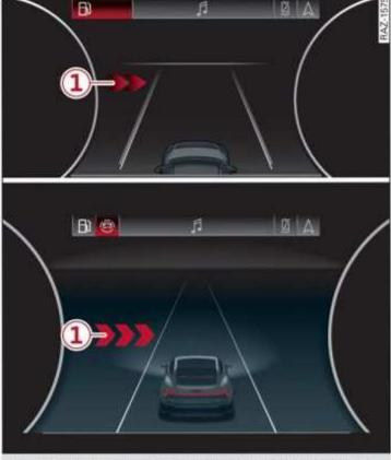
Fig. 128 Instrument cluster: intersection assistant direction display with or without area view
