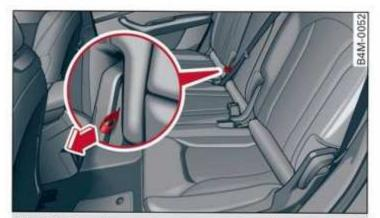
Fig. 81 Second row seats: release strap on the center backrest
