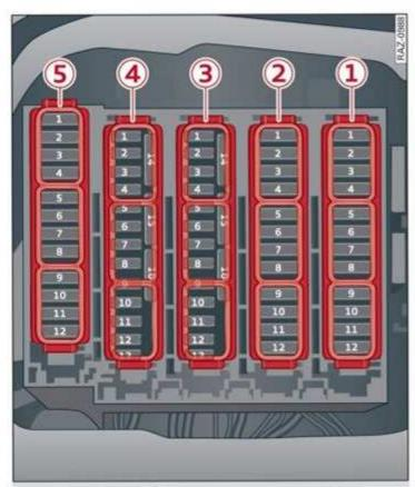
Fig. 200 Left side of the luggage compartment: fuse panel with plastic clip (plug-in hybrid drive\*)
