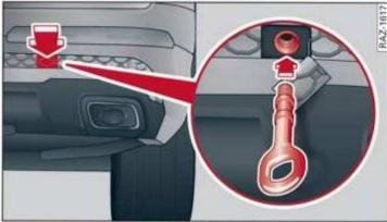
Fig. 193 Rear bumper: installing the towing loop
