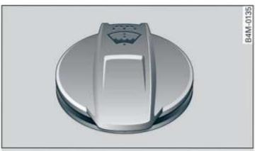
Fig. 174 Engine compartment: washer fluid reservoir cap
