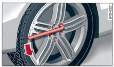
Fig. 185 Wheel: loosening the wheel bolts
