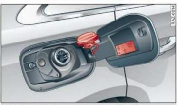
Fig. 165 Fuel filler door with attached fuel cap
