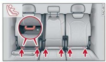
Fig. 72 Second row rear bench seat: lower LATCH anchors
