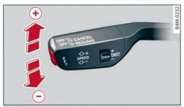
Fig. 109 Operating lever: changing the speed
