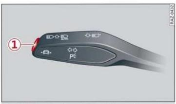
Fig. 110 Turn signal lever: button for lane guidance and lane departure warning
