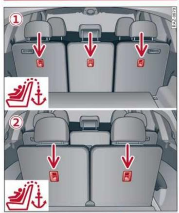
Fig. 74 ① Second row rear bench seat / ② third row rear bench seat: top tether anchors for securing a child safety seat with an upper strap
