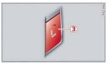
Fig. 149 Front headliner: online roadside assistance button
