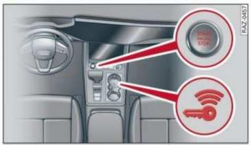
Fig. 89 Center console: starting the engine
