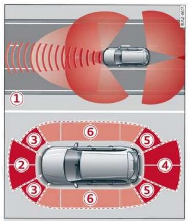
Fig. 95 Sensor coverage area
