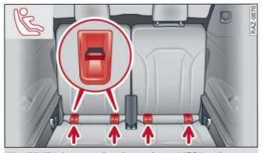
Fig. 73 Third row rear bench seat: lower LATCH anchors
