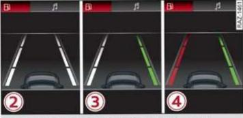
Applies to: driver assistance display without area view Fig. 122 Instrument cluster: lane departure warning
