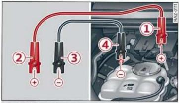
Fig. 191 Connecting the jump start cables
