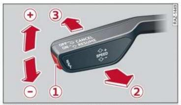
Fig. 104 Operating lever: switching the system on
