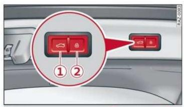
Fig. 29 Luggage compartment lid: 1 closing button\*, 2 lock button\* (vehicles with convenience key\*)
