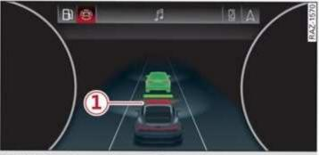
Applies to: driver assistance display with area view Fig. 117 Instrument cluster: safe start monitor
