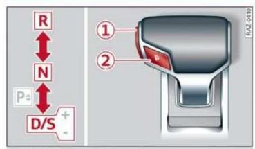
Fig. 90 Center console: selector lever
