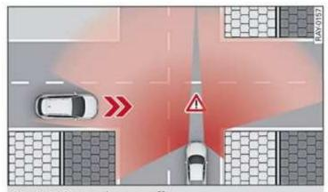
Fig. 127 Detected cross-traffic
