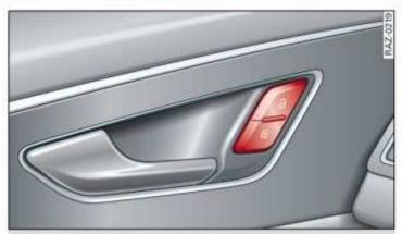
Fig. 21 Driver's door: central locking switch
