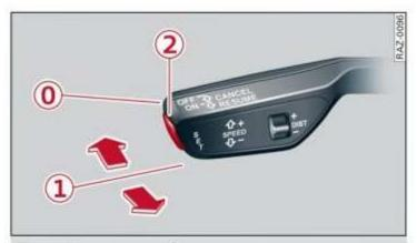
Fig. 115 Lever: using adaptive cruise assist
