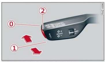
Fig. 108 Lever: using adaptive cruise assist
