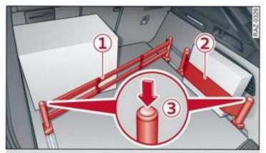
Fig. 84 Luggage compartment: securing attachments
