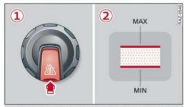
Fig. 171 Engine compartment - Coolant expansion tank (diagram): 1 cover with release button; 2 markings
