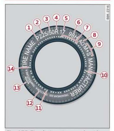
Fig. 175 Tire designations on the sidewall
