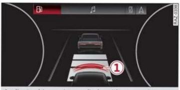
Applies to: driver assistance display without area view Fig. 116 Instrument cluster: safe start monitor
