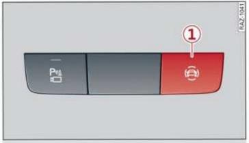
Fig. 99 Center console: driver assistance systems button
