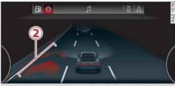
Applies to: driver assistance display with area view Fig. 124 Instrument cluster: side assist display
