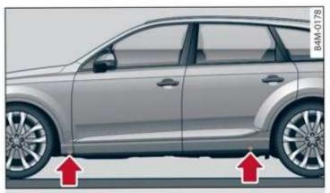
Fig. 186 Sill panels: markings
