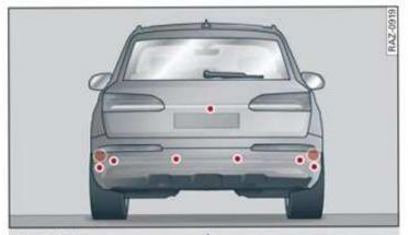
Fig. 98 Rear area: sensors and cameras
