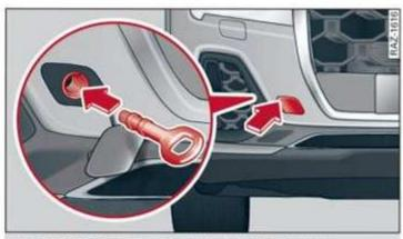
Fig. 192 Front bumper: installing the towing loop
