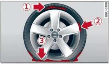
Fig. 180 Tire: tire damage that cannot be repaired
