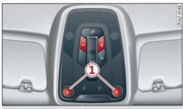
Fig. 39 Headliner: interior lighting
