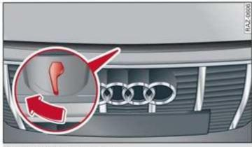
Fig. 167 Unlocked hood: lever
