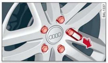
Fig. 183 Wheel: wheel bolts with caps
