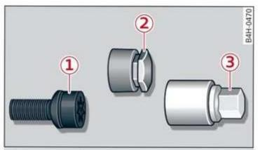
Fig. 184 Anti-theft wheel bolt with cap and adapter
