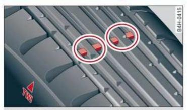
Fig. 176 Tire profile: treadwear indicator
