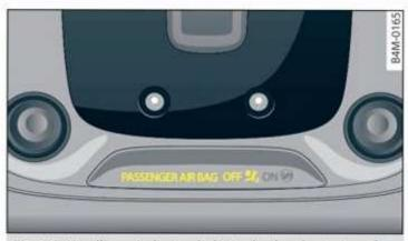
Fig. 71 Headliner: indicator light to display the status of the front passenger's airbag
