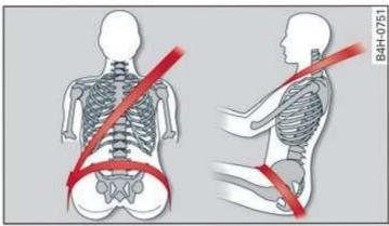
Fig. 64 Lap/shoulder belt positioning
