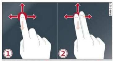
Fig. 12 Touch display: 1 dragging with one finger, 2 dragging with two fingers
