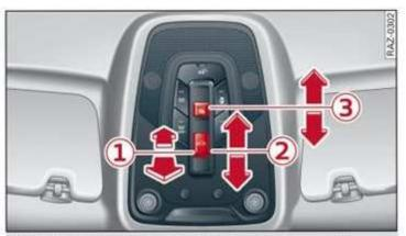
Fig. 34 Headliner: panoramic glass roof and sunshade\* buttons
