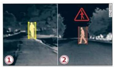
Fig. 103 Instrument cluster: pedestrian marking and warning
