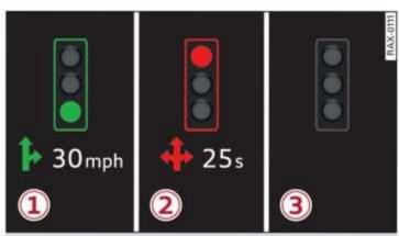
Fig. 102 Instrument cluster: traffic light information display
