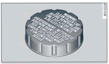
Fig. 167 Engine compartment: cap on brake fluid reservoir
