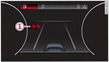
Fig. 123 Instrument cluster: directional display from the intersection assistant
