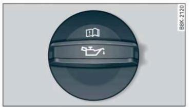
Fig. 165 Engine compartment: engine oil filling opening cover (example)
