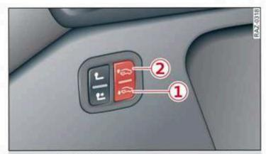
Fig. 80 Left side of the luggage compartment: rear lowering button
