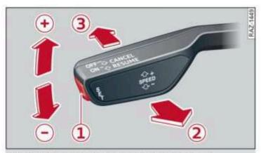
Fig. 103 Operating lever: switching the system on
