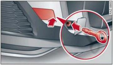
Fig. 188 Front bumper: installing the towing loop (version 2)
