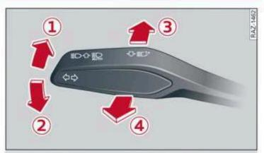
Fig. 35 Operating lever: switching the light functions on and off
