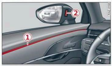
Fig. 121 Front door: warning strip
