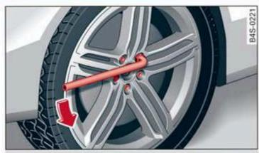
Fig. 180 Wheel: loosening the wheel bolts
