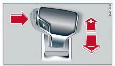
Fig. 91 Center console: shifting manually with the selector lever
