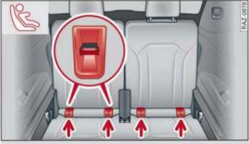
Fig. 72 Third row rear bench seat: lower LATCH anchors
