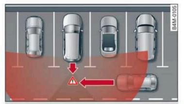
Fig. 131 Sensor detection range for rear cross-traffic assist
