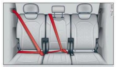
Fig. 75 Second row rear bench seat: securing safety belts that are not used
