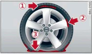
Fig. 175 Tire: tire damage that cannot be repaired
