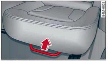
Fig. 55 Second row seats: adjusting the seat position
