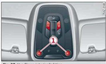
Fig. 38 Headliner: interior lighting
