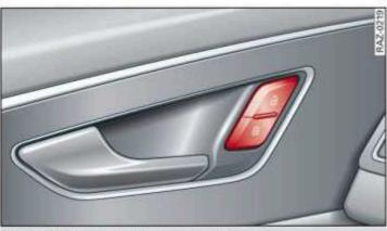
Fig. 20 Driver's door: central locking switch
