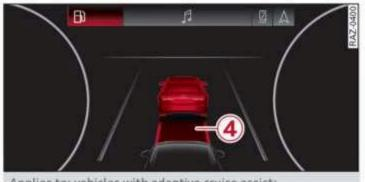
Applies to: vehicles with adaptive cruise assist: Fig. 116 Instrument cluster: distance warning
