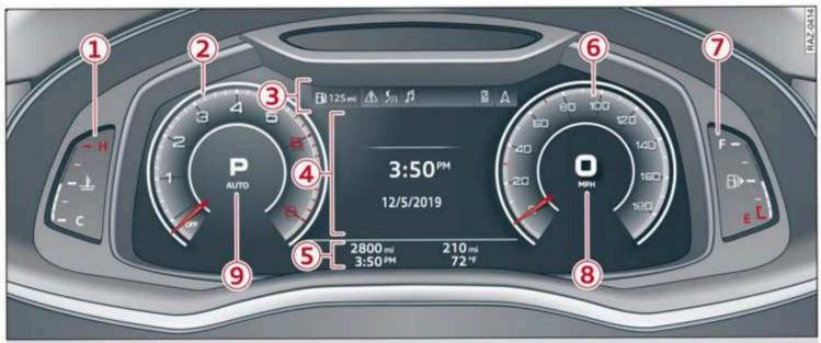
Fig. 2 Instrument cluster overview (Audi virtual cockpit)
