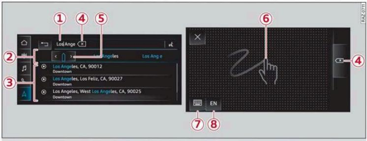
Fig. 16 Upper/lower display: text input
