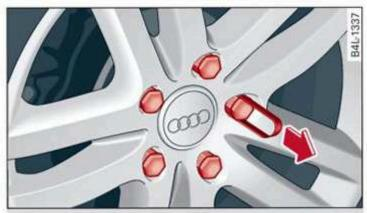
Fig. 178 Wheel: wheel bolts with caps
