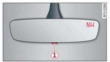
Fig. 49 Rearview mirror: digital compass is switched on
