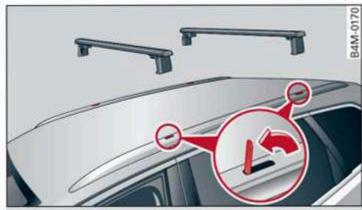
Fig. 86 Roof rail: mounting points
