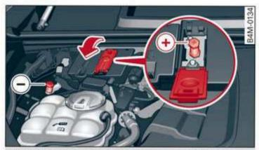
Fig. 185 Engine compartment: connectors for jump start cables or a charger
