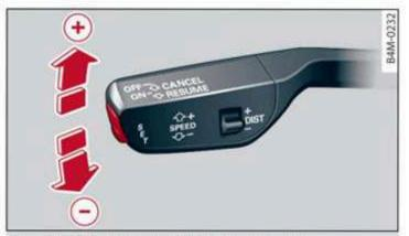
Fig. 108 Operating lever: changing the speed
