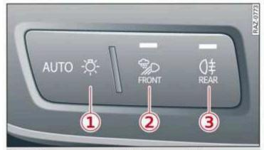
Fig. 34 Instrument panel: light button module
