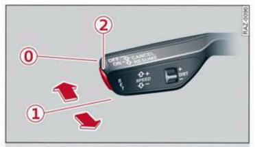
Fig. 107 Lever: using adaptive cruise assist
