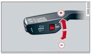
Fig. 112 Operating lever: setting the distance
