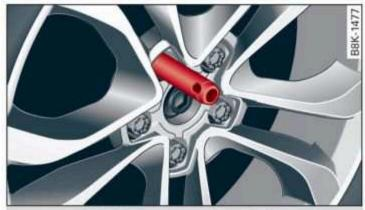
Fig. 184 Wheel: alignment pin in the top hole
