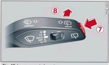
Fig. 46 Lever: rear window wiper
