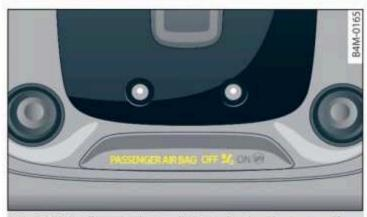
Fig. 70 Headliner: indicator light to display the status of the front passenger's airbag
