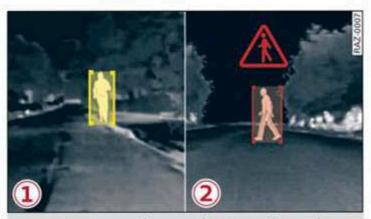
Fig. 102 Instrument cluster: pedestrian marking and warning
