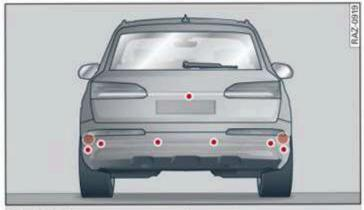
Fig. 98 Rear area: sensors and cameras
