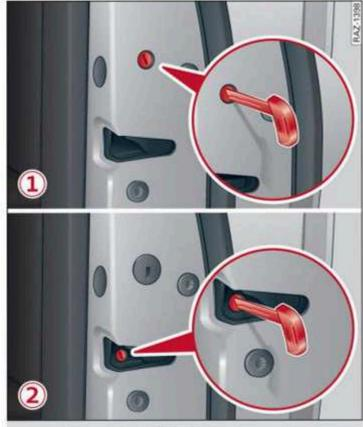
Fig. 22 Door: mechanically locking
