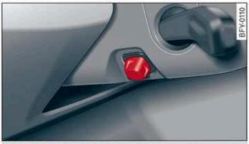
Fig. 59 Steering column: switch for adjusting the steering wheel position
