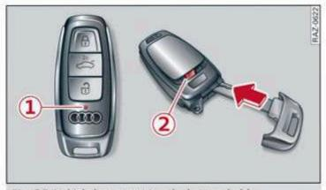
Fig. 25 Vehicle key: removing the battery holder
