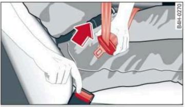
Fig. 66 Releasing the belt buckle from the belt latch
