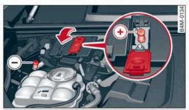
Fig. 168 Engine compartment: connectors for a charger or jump start cables
