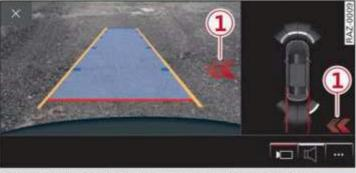
Fig. 132 Upper display: rear cross-traffic assist display
