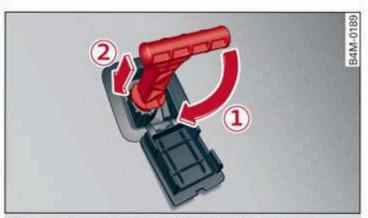
Fig. 93 Footwell: releasing the parking lock using the emergency release
