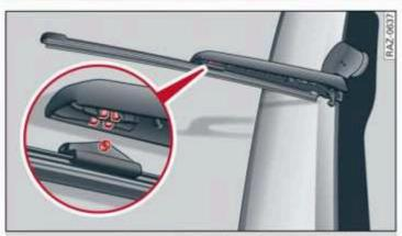
Fig. 48 Rear window wiper: installing the wiper blade
