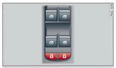
Fig. 31 Driver's door: controls
