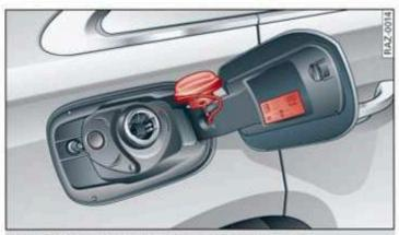
Fig. 160 Fuel filler door with attached fuel cap
