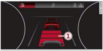
Fig. 110 Instrument cluster: brake intervention request
