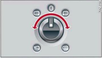
Fig. 41 Driver's door: knob for the exterior mirrors
