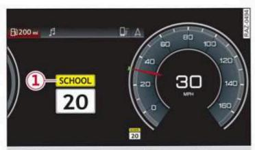
Fig. 100 Instrument cluster: traffic sign recognition
