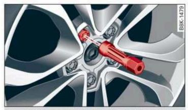
Fig. 183 Wheel: internal hex socket to turn the wheel bolts
