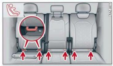
Fig. 71 Second row rear bench seat: lower LATCH anchors
