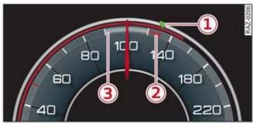
Fig. 111 Instrument cluster: speedometer: predictive control display
