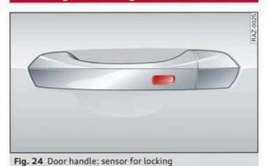
Depending on the vehicle equipment, you may have various options for unlocking and locking your vehicle. The settings in the MMI specify which doors will unlock ⇒ page 35.
