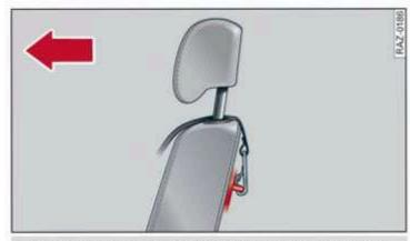
Fig. 74 Rear backrest: securing the upper belt to the top tether anchor
