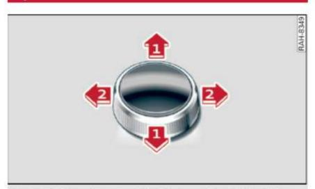
Fig. 162 Operating concept for the control knob with joystick function
