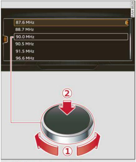
Fig. 153 Operating the control knob
