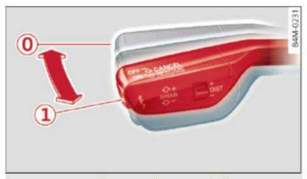
Fig. 98 Operating lever: switching on and off
