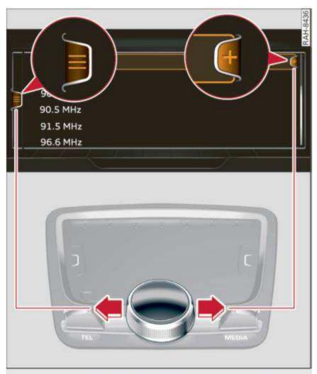
Fig. 163 Opening the selection/options menu with the control knob
