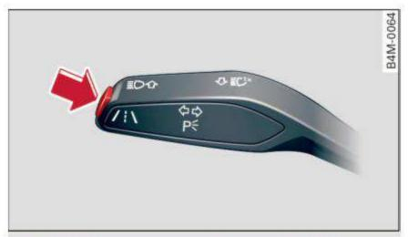
Fig. 105 Turn signal lever: traffic jam assist button
