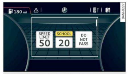
Fig. 90 Instrument cluster: traffic sign recognition
