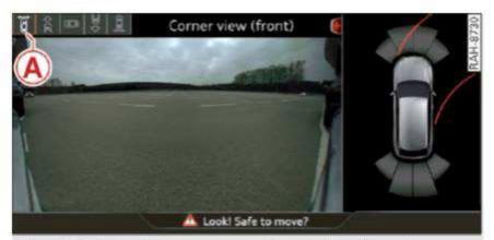
Fig. 139 Infotainment system: Corner view (front)
