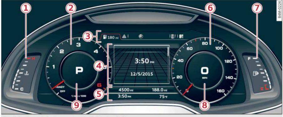
Fig. 4 Instrument cluster overview (Audi virtual cockpit)
