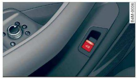
Fig. 24 Driver's door: opening the luggage compartment
