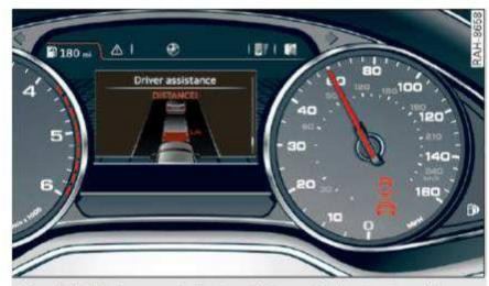
Fig. 107 Instrument cluster: distance indicator/warning
