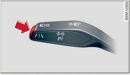
Fig. 109 Turn signal lever: button for active lane assist
