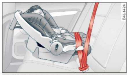
Fig. 242 Schematic overview: rearward-facing infant seat, properly installed on the rear seat
