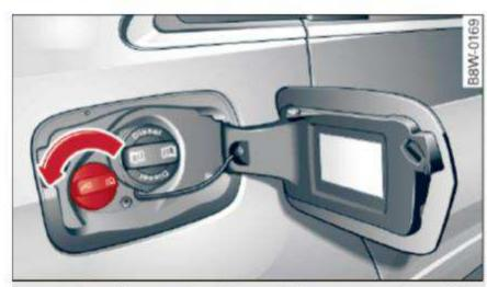
Fig. 258 Right rear side of the vehicle: removing the AdBlue cap
