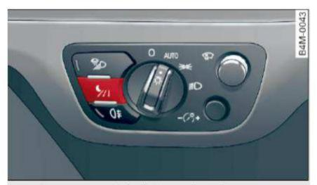
Fig. 125 Area around the light switch: night vision assist button
