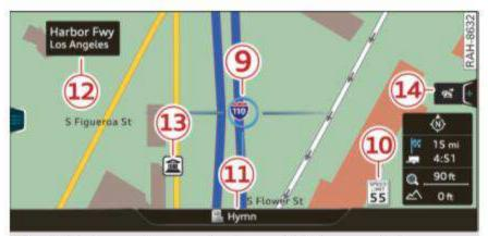
Fig. 193 Example: standard map with the crosshairs switched on
