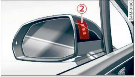
Fig. 113 Display on the exterior mirror
