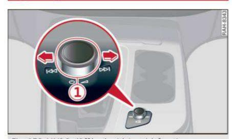
Fig. 150 MMI On/Off knob with joystick function
