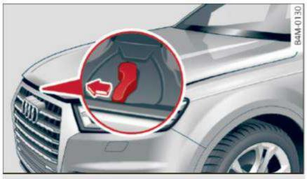
Fig. 262 Unlocked hood: lever
