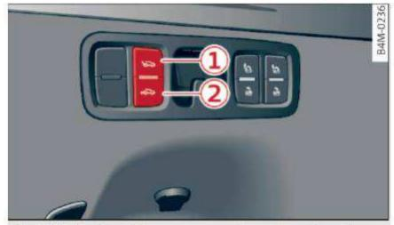
Fig. 127 Section of luggage compartment: rear lowering button
