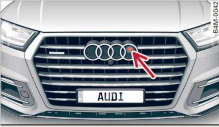
Fig. 124 Front of the vehicle: night vision assist camera
