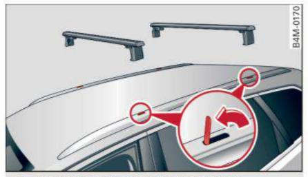
Fig. 74 Roof: mounting points for the roof rack
