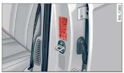
Fig. 271 Driver's side B-pillar: tire pressure label
