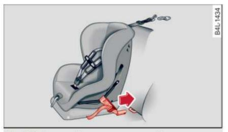
Fig. 249 Lower anchorages: proper mounting
