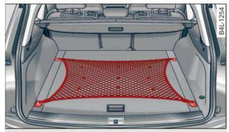
Fig. 72 Luggage compartment: cargo net stretched out
