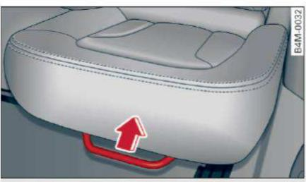
Fig. 54 Second row seats: adjusting the forward/back position
