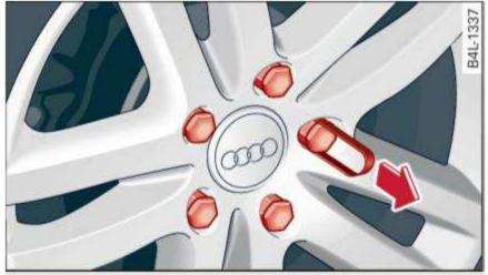
Fig. 276 Wheel: wheel bolts with caps
