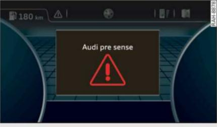
Fig. 108 Instrument cluster: approach warning
