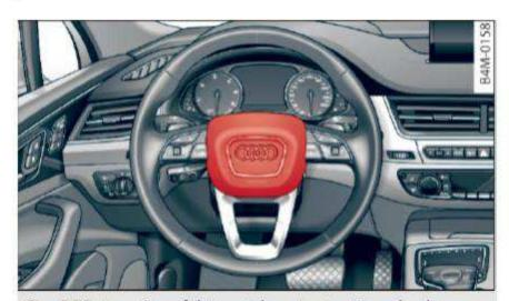
Fig. 233 Location of driver airbag: in steering wheel
