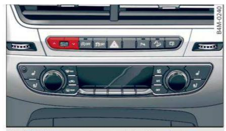
Fig. 126 Center console: controls for drive select
