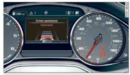
Fig. 101 Instrument cluster: safe start monitor
