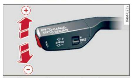
Fig. 100 Operating lever: changing the speed
