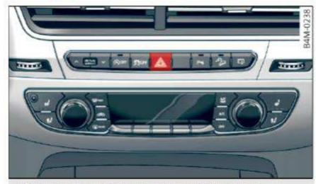
Fig. 35 Center console: emergency flasher button
