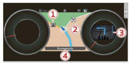
Fig. 168 Standard map when route guidance is active (Audi virtual cockpit)
