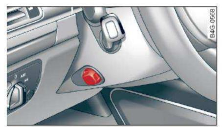
Fig. 80 Steering column: switch to adjust the steering wheel position
