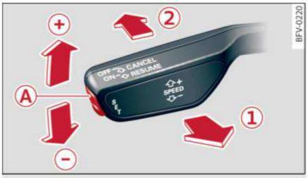
Fig. 89 Operating lever: cruise control system
