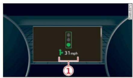
Fig. 181 Example: display of a speed recommendation
