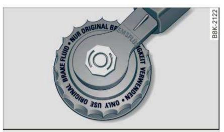
Fig. 266 Engine compartment: cap on brake fluid reservoir
