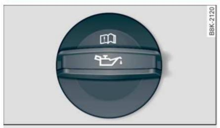
Fig. 264 Engine compartment: engine oil filler opening cover
