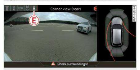
Fig. 140 Infotainment system: Corner view (rear)
