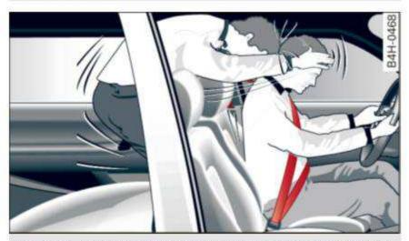
Fig. 226 A rear passenger not wearing a safety belt will fly forward and strike the driver
