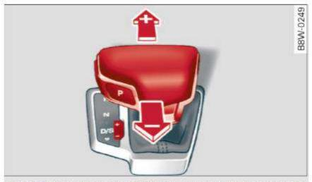
Fig. 86 Center console: shifting manually with the selector lever
