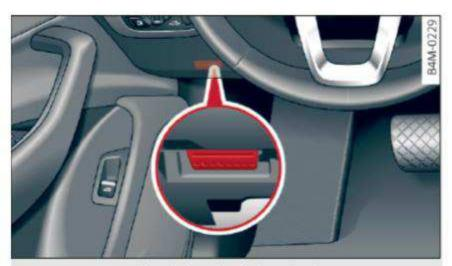
Fig. 260 Footwell on left side of the vehicle: connection port for the On-Board Diagnostic System (OBD)
