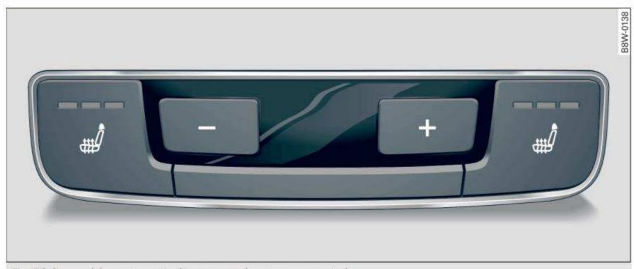
Fig. 76 3-zone deluxe automatic climate control system: rear controls
