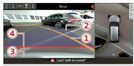
Fig. 144 Infotainment system: aiming at a parking space
