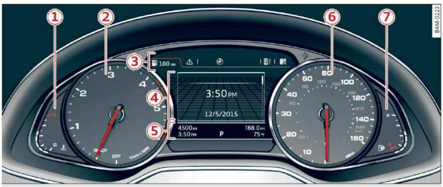
Fig. 3 Instrument cluster overview (analog)
