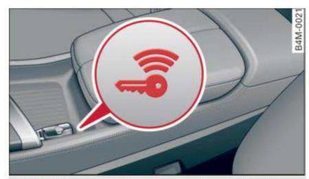
Fig. 82 Center console/remote control key: starting the engine if there is a malfunction
