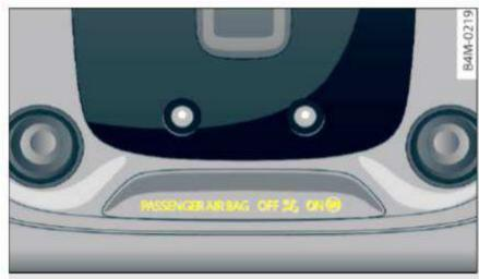
Fig. 236 Section from the headliner: PASSENGER AIR BAG OFF № ON light
