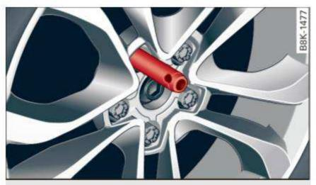
Fig. 281 Wheel: alignment pin in the top hole
