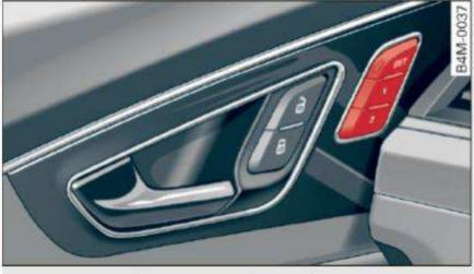
Fig. 62 Driver's door: memory function buttons
