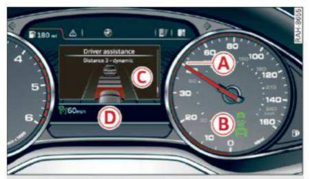
Fig. 99 Instrument cluster: adaptive cruise control
