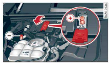
Fig. 267 Engine compartment: connectors for a charger and jump start cables
