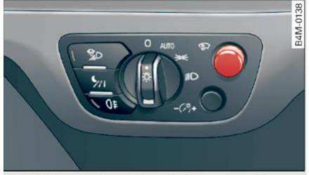
Fig. 14 Instrument panel: knob for the head-up display
