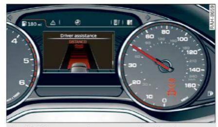
Fig. 104 Instrument cluster: request for driver intervention
