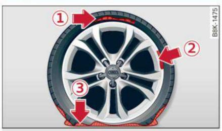
Fig. 273 Tire: tire damage that cannot be repaired
