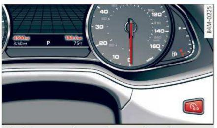
Fig. 5 Instrument cluster: odometer and reset button
