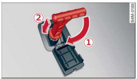
**Fig. 88** Driver's side footwell: releasing the parking lock using the emergency release
