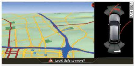
Fig. 130 Infotainment system: visual distance display
