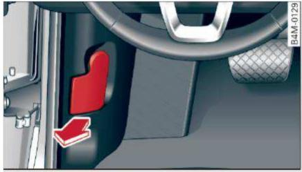
Fig. 261 Driver footwell: release lever
