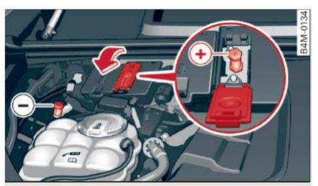
Fig. 288 Engine compartment: connectors for jump start cables and a charger
