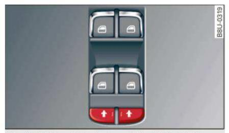
Fig. 28 Section of driver's door: child safety lock buttons
