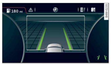
Fig. 111 Instrument cluster: active lane assist is switched on and ready to provide warnings
