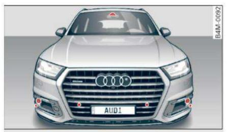
Fig. 95 Front of the vehicle: sensors and video camera
