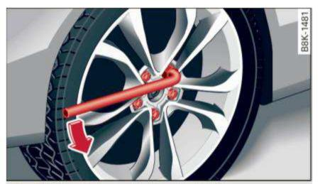
Fig. 277 Wheel: loosening the wheel bolt
