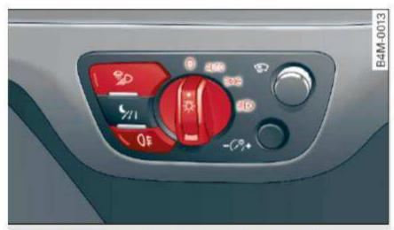
Fig. 33 Instrument panel: light switch with buttons
