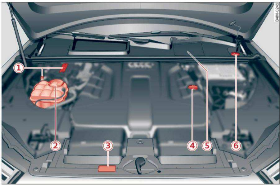
Fig. 263 Typical location of the reservoir and the engine oil filler opening
