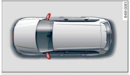
Fig. 137 Location of peripheral cameras
