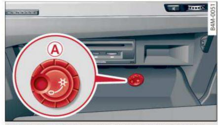
Fig. 67 Glove compartment: switching cooling mode on/ off
