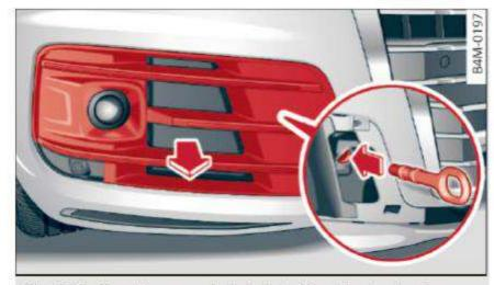
Fig. 291 Front bumper (trim): installing the towing loop
