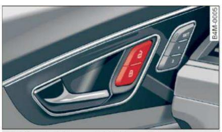
Fig. 21 Driver's door: central locking switch
