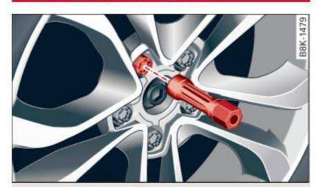
Fig. 280 Wheel: internal hex socket to turn the wheel bolts
