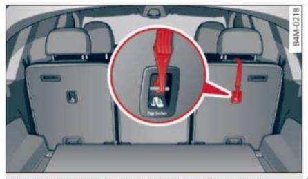
Fig. 253 Tether strap: proper routing and mounting
