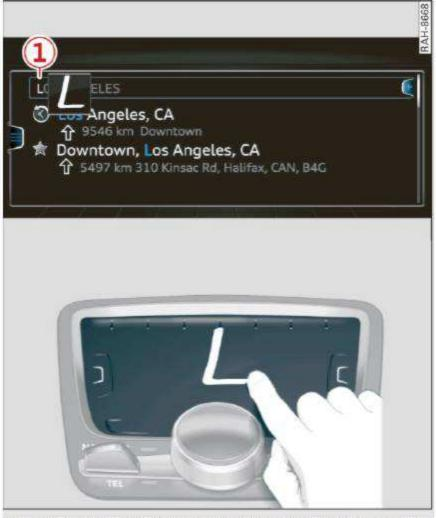
Fig. 157 Example: entering a navigation destination using the MMI touch
