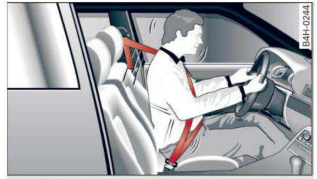
Fig. 227 Driver is correctly restrained in a sudden braking maneuver
