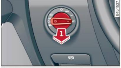
Fig. 57 Instrument panel: light switch
