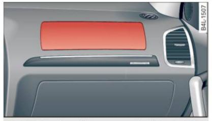
Fig. 209 Location of front passenger's airbag: in the instrument panel
