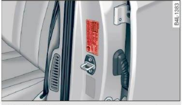
**Fig. 250** Tire pressure label: located on driver's side B-pillar
