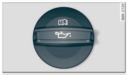
**Fig. 245** Engine compartment: cover on the engine oil filler neck
