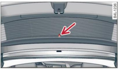
Fig. 67 Sun shade pulled up on the rear lid window
