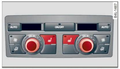
Fig. 118 Center console rear: Seat heating with fourzone automatic comfort air conditioning\*
