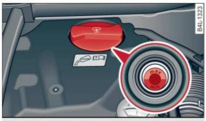
Fig. 246 Engine compartment: Coolant expansion tank
