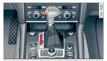
Fig. 162 Shift gate on the center console: selector lever with release button
