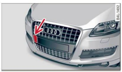
**Fig. 129** Front bumper: Position of radar sensor (not visible from outside)
