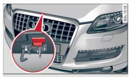
Fig. 241 Release lever under the engine hood
