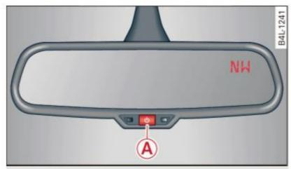
Fig. 75 Inside rear view mirror: digital compass activated
