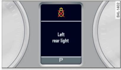
Fig. 14 Display: defective light bulb warning
