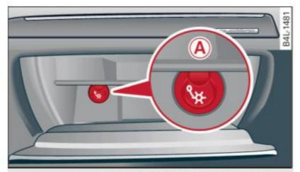
Fig. 106 Glove box with cooling box open and switched on
