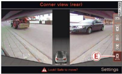
Fig. 181 MMI display: Corner view (rear) mode
