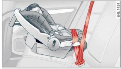
Fig. 217 Schematic overview: rearward-facing infant seat, properly installed on the rear seat
