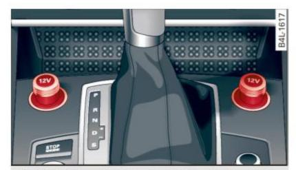
Fig. 103 Section from center console: 12-volt outlets
