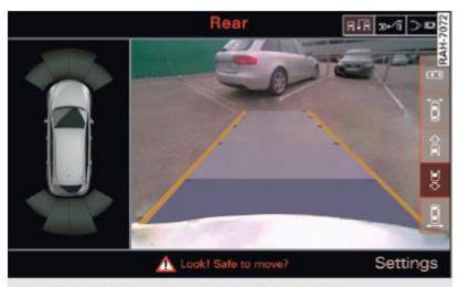
Fig. 185 MMI display: Aligning the vehicle
