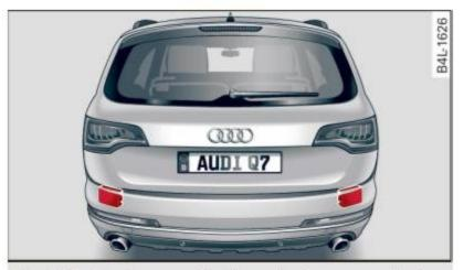
**Fig. 150** Rear bumper: Position of radar sensors (not visible on outside)
