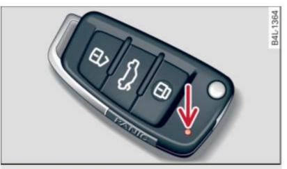
Fig. 29 Check light in the master key
