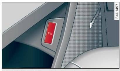
Fig. 39 Driver's door: Unlocking the rear lid
