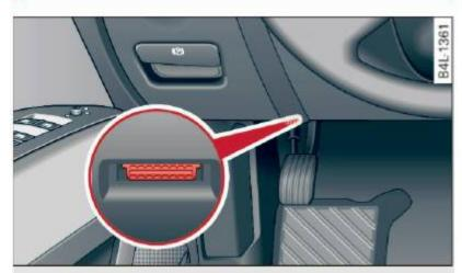
Fig. 22 Location of Data Link Connector (DLC)
