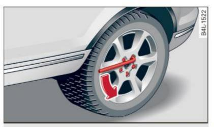
Fig. 263 Changing a wheel: loosening the wheel bolts
