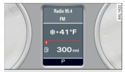
**Fig. 160** Display in the instrument cluster: selector lever in position P
