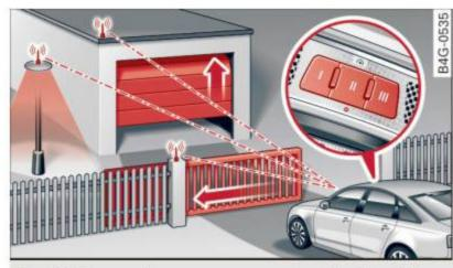
Fig. 53 Garage door opener: examples of using with different systems
