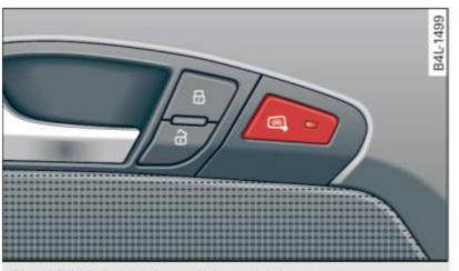
Fig. 152 Driver's door: Side assist button
