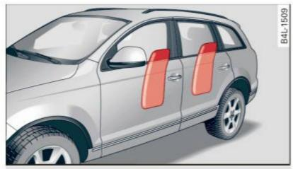
Fig. 213 Inflated side airbags on left side of vehicle, rear side airbag optional equipment
