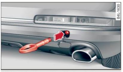
Fig. 277 Rear bumper: Screwing in towing loop
