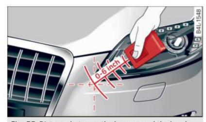
Fig. 55 Distance between the bumper and the hand transmitter
