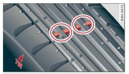
Fig. 252 Tire tread: tread wear indicators (TWI)
