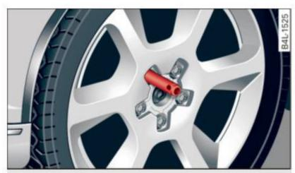
Fig. 266 Changing a wheel: alignment pin inside the top hole
