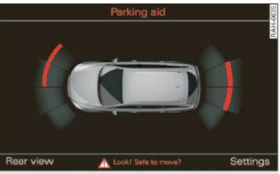
Fig. 171 MMI display: Visual distance display
