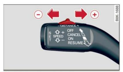
Fig. 136 Control lever: Setting distance
