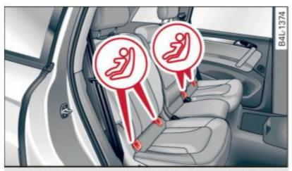
Fig. 222 Second row of seats: lower anchorage bracket locations
