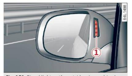
**Fig. 151** Signal light on the outside mirror - driver's side
