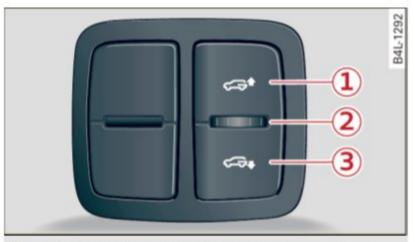
Fig. 193 Luggage compartment detail: Cargo mode switch
