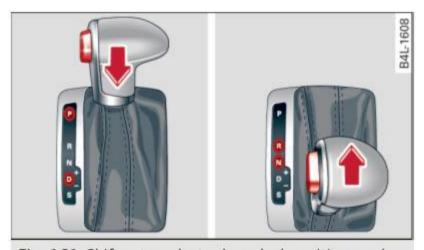
Fig. 161 Shift gate: selector lever lock positions and release button highlighted
