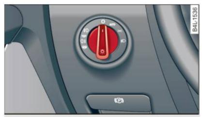
Fig. 56 Instrument panel: light switch
