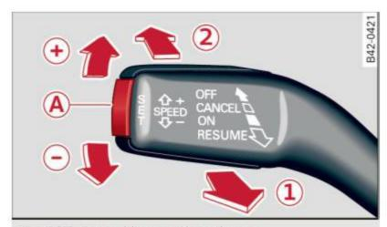
Fig. 127 Control lever with set button
