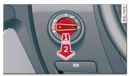
Fig. 58 Instrument panel: light switch
