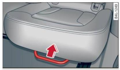
Fig. 80 Fore-and-aft adjustment
