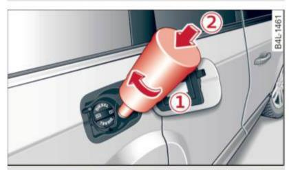
Fig. 239 AdBlue filler tube: inserting the refill bottle
