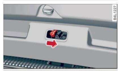
Fig. 42 Section of the luggage compartment: Emergency release
