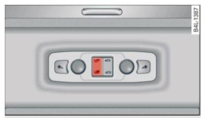
Fig. 52 Section of headliner in rear: Switch for sunshade
