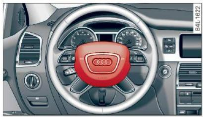
Fig. 208 Location of driver airbag: in steering wheel
