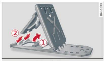
Fig. 258 Opening folding chocks
