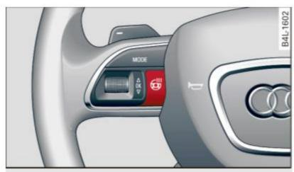
Fig. 119 Steering wheel: button for steering wheel heating
