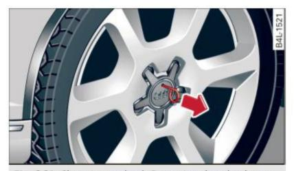
Fig. 261 Changing a wheel: Removing the wheel cover
