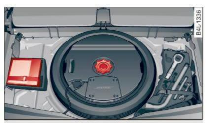
Fig. 260 Inflatable spare tire with compressor
