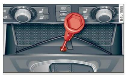
Fig. 165 Selector lever emergency release
