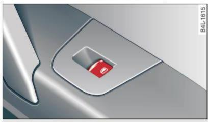
Fig. 47 Switch location front passengers door
