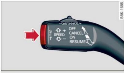
Fig. 132 Control lever: Storing speed
