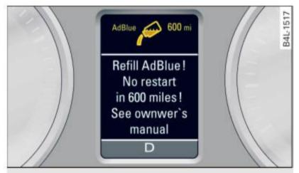
Fig. 237 Instrument cluster: indicator in the display
