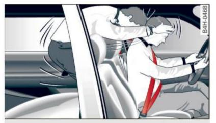
Fig. 201 A rear passenger not wearing a safety belt will fly forward and strike the driver
