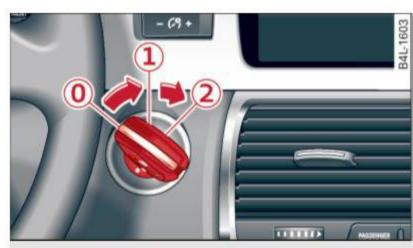
Fig. 122 Ignition switch positions
