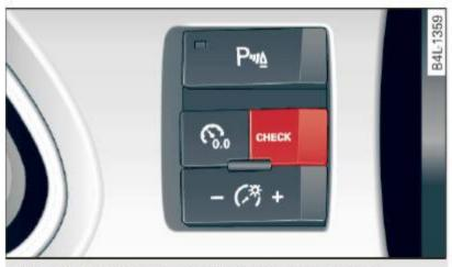
Fig. 23 CHECK button in the instrument cluster
