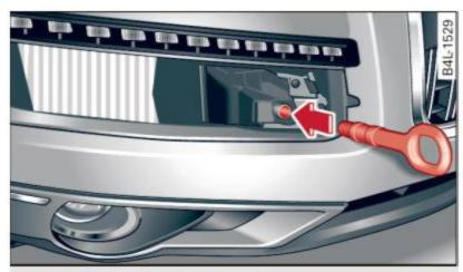
**Fig. 275** Right front bumper without cover: Screwing in towing loop
