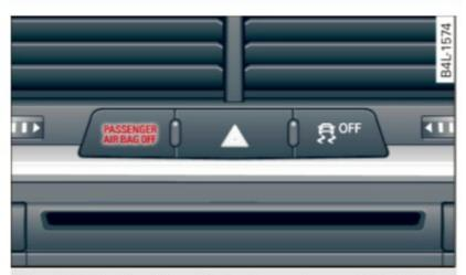
**Fig. 211** Section from the instrument panel: PASSENGER AIR BAG OFF light
