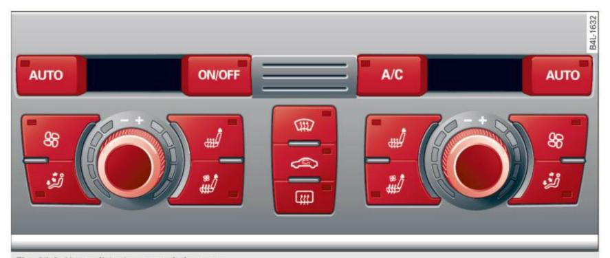
Fig. 114 Air conditioning control elements
