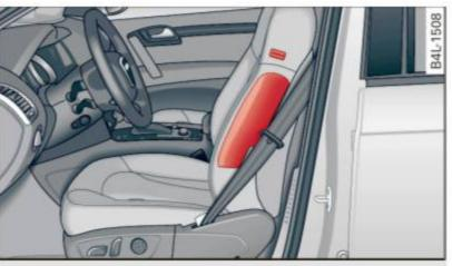
Fig. 212 Side airbag location in the driver's seat
