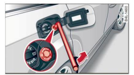
Fig. 238 Right rear vehicle side: removing the AdBlue cap
