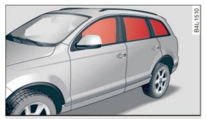
Fig. 215 Illustration of principle: Inflated side curtain airbags on the left side
