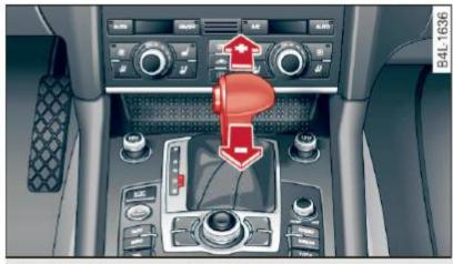
Fig. 163 Center console: shifting the gears manually
