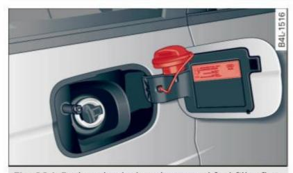
Fig. 234 Fuel cap hooked on the opened fuel filler flap
