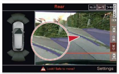
Fig. 187 MMI display: Contact of the blue curve with the curb
