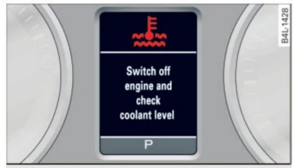
Fig. 25 Display: engine coolant level warning (priority 1)
