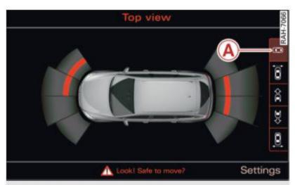
Fig. 179 MMI display: Top view mode
