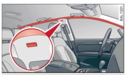
Fig. 214 Side curtain airbags, driver's side: location
