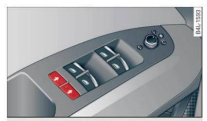
Fig. 43 Section from driver's door: controls
