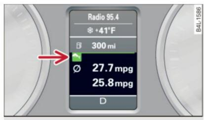
Fig. 19 Display: efficiency program
