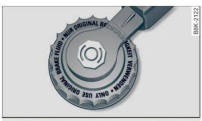
Fig. 247 Engine compartment: cover on the brake fluid reservoir
