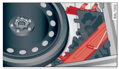
Fig. 257 Luggage compartment vehicle jack and folding chocks
