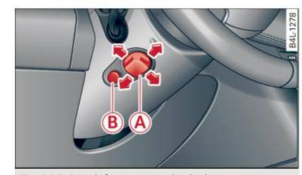
Fig. 118 Switch for steering wheel adjustment
