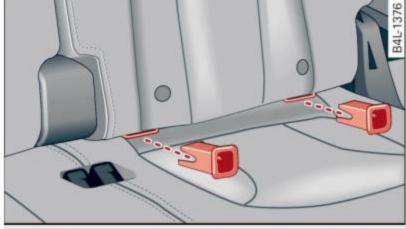
Fig. 223 Third row of seats: installing the guidance fix-
