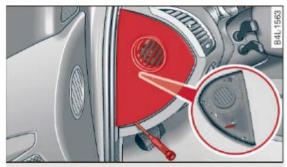
Fig. 266 Left cockpit: fuse panel cover
