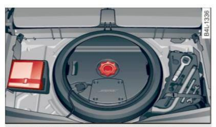
Fig. 259 Inflatable spare tire with compressor
