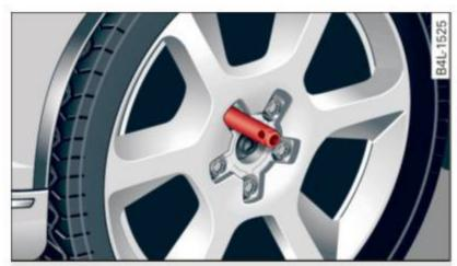
Fig. 265 Changing a wheel: alignment pin inside the top hole
