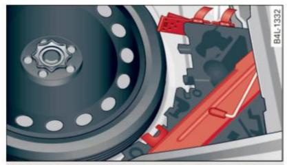
Fig. 256 Luggage compartment vehicle jack and folding chocks
