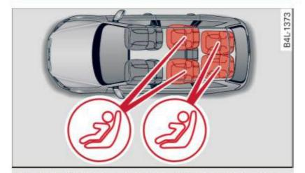
Fig. 220 Schematic overview: LATCH anchorage point locations
