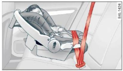
Fig. 216 Schematic overview: rearward-facing infant seat, properly installed on the rear seat
