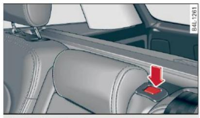
Fig. 87 Release lever for center seatback
