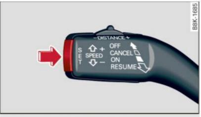
Fig. 129 Control lever: Storing speed
