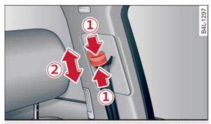
Fig. 206 Safety belt height adjustment – loop-around fittings
