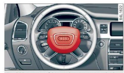
Fig. 207 Location of driver airbag: in steering wheel
