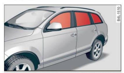
**Fig. 214** Illustration of principle: Inflated side curtain airbags on the left side
