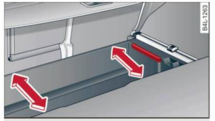
Fig. 93 Removing the cargo floor
