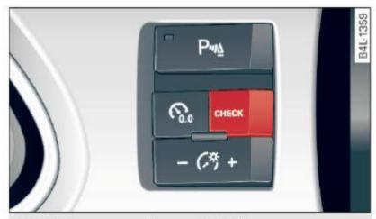
Fig. 24 Instrument cluster: CHECK button
