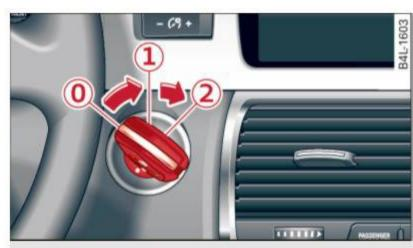
Fig. 119 Ignition switch positions
