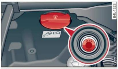
Fig. 245 Engine compartment: Coolant expansion tank
