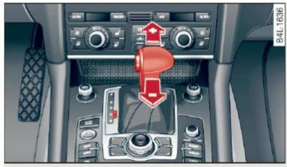
Fig. 160 Center console: shifting the gears manually
