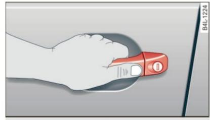
Fig. 44 Convenience key: unlocking vehicle door
