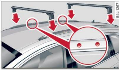
Fig. 95 Roof rails: front and rear mounting locations
