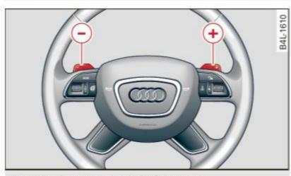
Fig. 161 Steering wheel: Shift buttons\*
