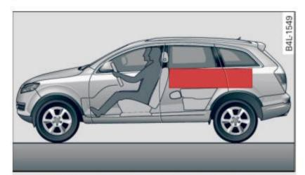
**Fig. 195** Safe load positioning: place heavy objects as low and as far forward as possible.
