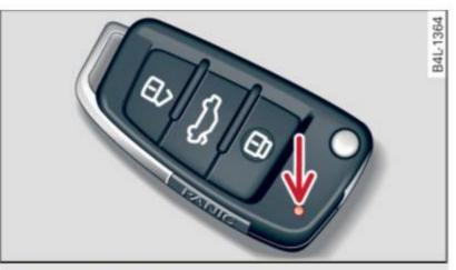
Fig. 29 Check light in the master key
