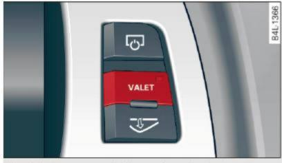
Fig. 31 Center console: button for valet key function
