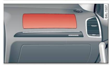
Fig. 208 Location of front passenger's airbag: in the instrument panel
