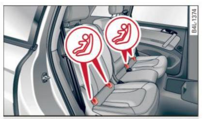
Fig. 221 Second row of seats: lower anchorage bracket locations
