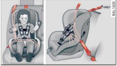
Fig. 218 Schematic overview: installation of the seat using the vehicle's safety belt system
