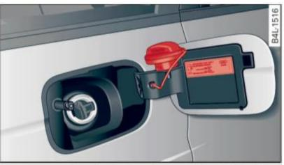
Fig. 233 Fuel cap hooked on the opened fuel filler flap
