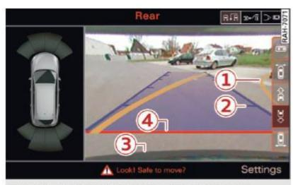
Fig. 181 MMI display: Aiming at a parking space
