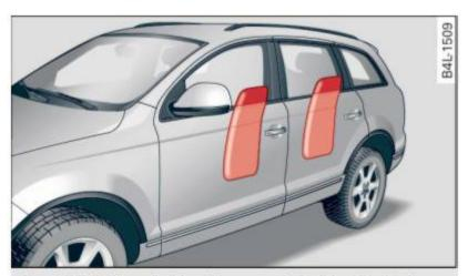
Fig. 212 Inflated side airbags on left side of vehicle, rear side airbag optional equipment
