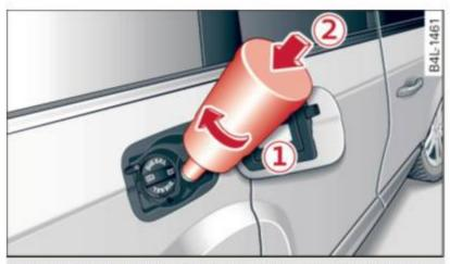
Fig. 238 AdBlue filler tube: inserting the refill bottle
