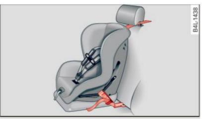
Fig. 228 Tether strap: proper routing and mounting
