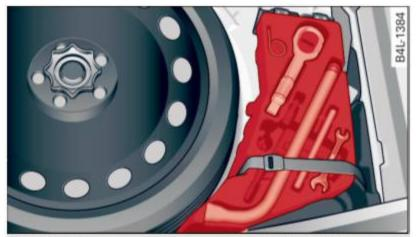
Fig. 255 Luggage compartment: vehicle tool kit
