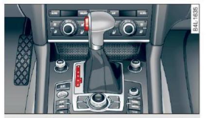
Fig. 159 Shift gate on the center console: selector lever with release button
