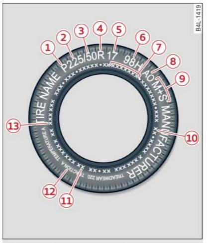
Fig. 253 Tire specification codes on the sidewall of a tire
