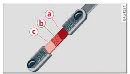
Fig. 242 Illustration of principle 1: Markers on oil dipstick
