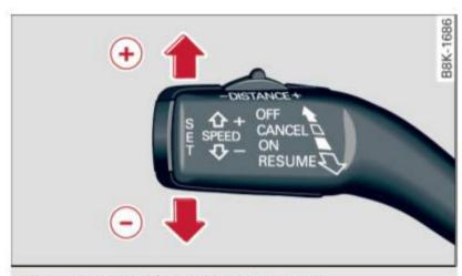
Fig. 130 Control lever: Changing speed
