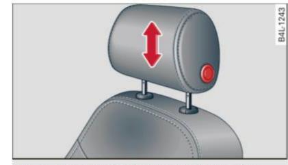
Fig. 81 Front seats head restraints: adjusting the height
