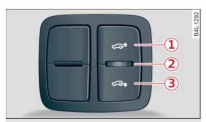
Fig. 190 Luggage compartment detail: Cargo mode switch
