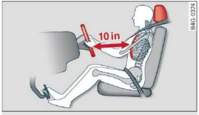
Fig. 193 Correct seating position
