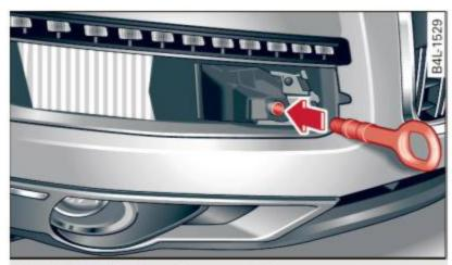
Fig. 274 Right front bumper without cover: Screwing in towing loop
