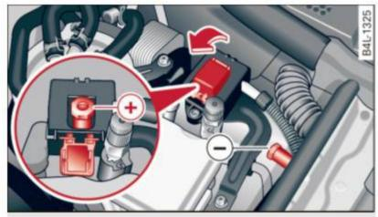
Fig. 247 Engine compartment: Connectors for charger and jumper cables
