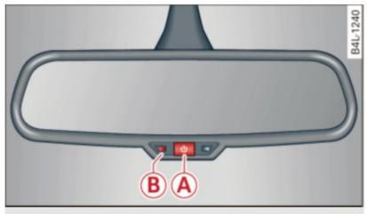
Fig. 71 Automatic dimming rearview mirror\*
