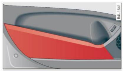
Fig. 107 Door panel with storage compartment.
