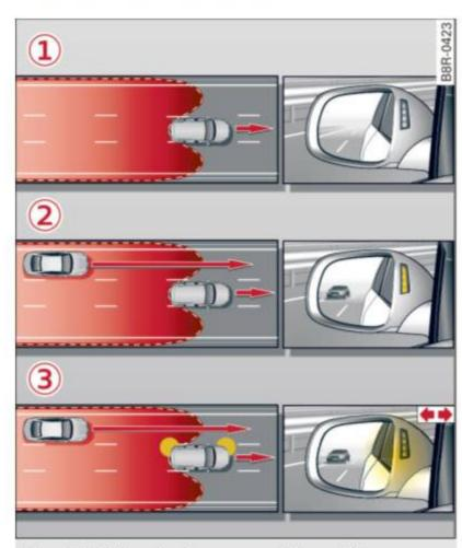
Fig. 151 Side assist: Fast approaching vehicles
