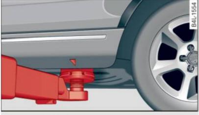
Fig. 279 Rear lifting point
