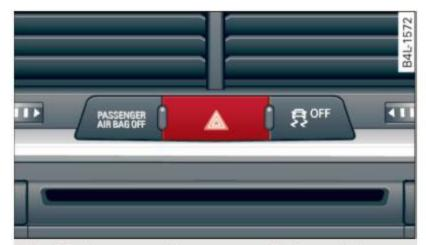
Fig. 57 Center console: emergency flasher switch
