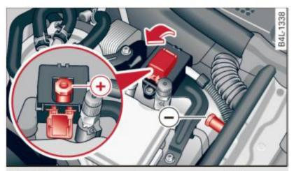
Fig. 271 Engine compartment: Connectors for jumper cables and charger
