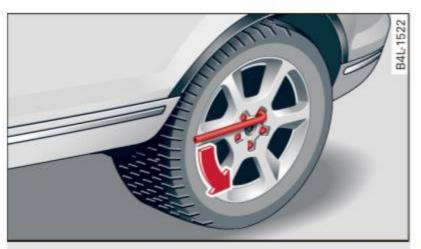
Fig. 262 Changing a wheel: loosening the wheel bolts
