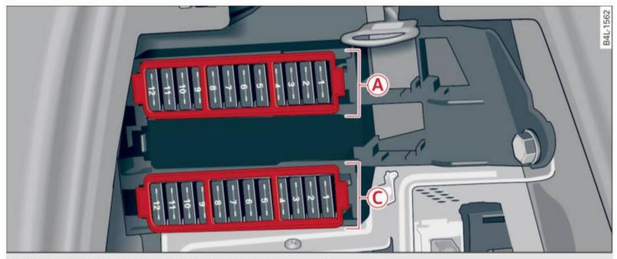
Fig. 270 Right luggage compartment: fuse panel with plastic clip
