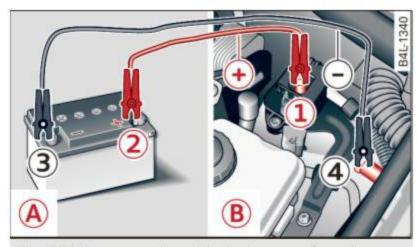
**Fig. 272** Jump starting with the battery of another vehicle: A – booster battery, B – discharged vehicle battery
