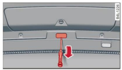
**Fig. 41** Section of the luggage compartment: Access to emergency release
