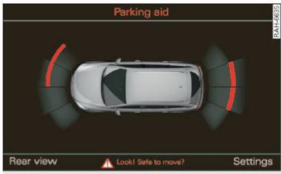
Fig. 168 MMI display: Visual distance display
