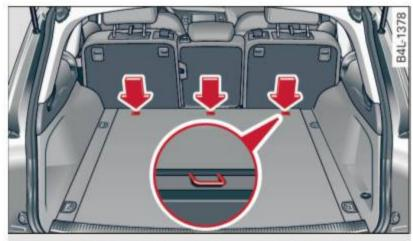
Fig. 226 Tether anchors for second row of seats: attachment hook locations
