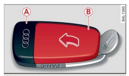
Fig. 30 Master key: opening the cover
