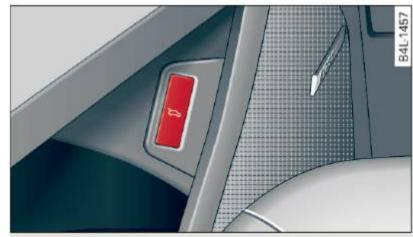
Fig. 37 Driver's door: remote rear lid release
