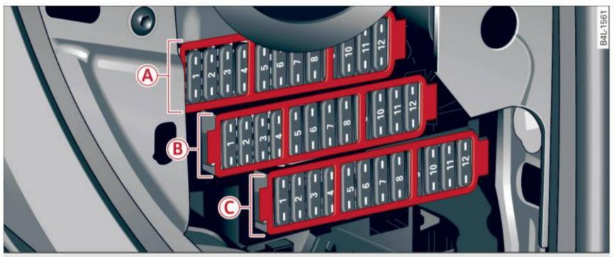
Fig. 269 Right cockpit: fuse panel with plastic clip
