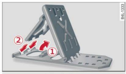
Fig. 257 Opening folding chocks
