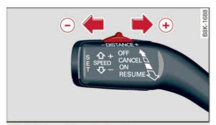
Fig. 133 Control lever: Setting distance
