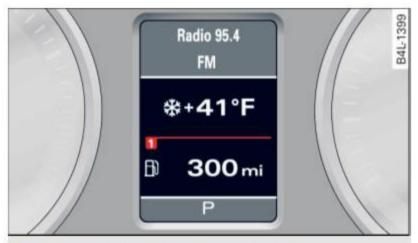
Fig. 9 Instrument cluster: center display
