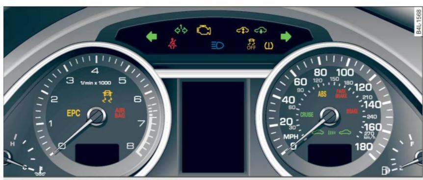
Fig. 8 Instrument cluster with warning/indicator lights
