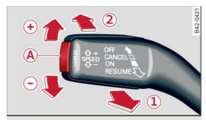
Fig. 124 Control lever with set button
