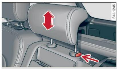
Fig. 83 Rear seat: center head restraint
