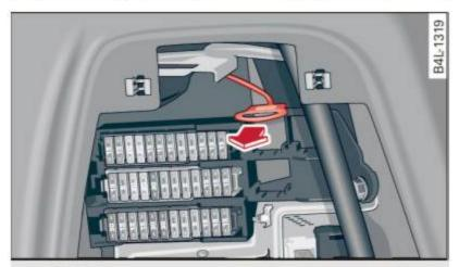
**Fig. 235** Luggage compartment: Emergency opening of fuel filler flap
