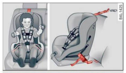
**Fig. 217** Schematic overview: installation of the attachments applicable to a LATCH seat
