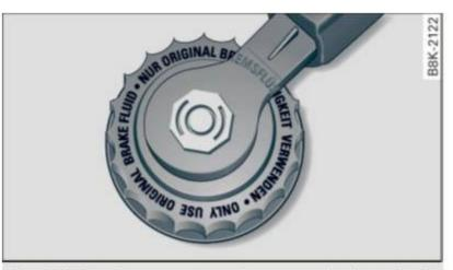
Fig. 246 Engine compartment: cover on the brake fluid reservoir
