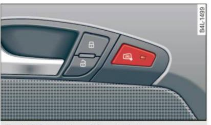
Fig. 149 Driver's door: Side assist button
