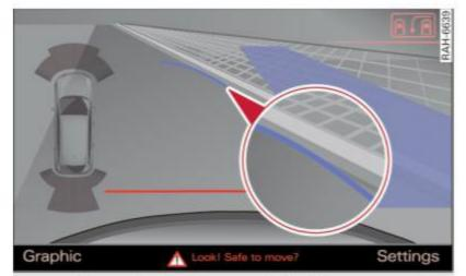
Fig. 172 MMI display: Contact of the blue curve with the curb
