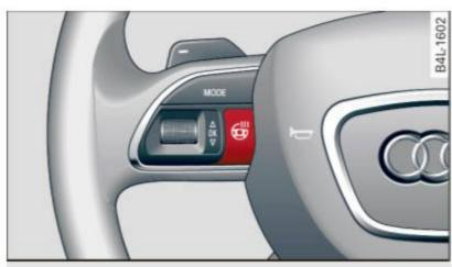
Fig. 116 Steering wheel: button for steering wheel heating
