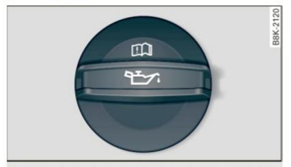
Fig. 244 Engine compartment: cover on the engine oil filler neck
