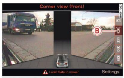
Fig. 177 MMI display: Corner view (front) mode
