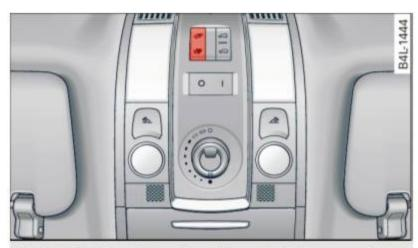
Fig. 51 Section of front headliner: Switch for sunshade
