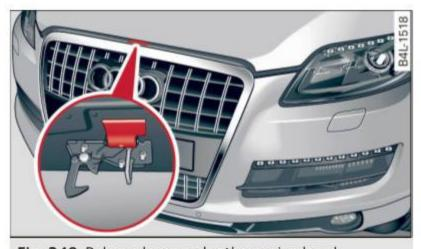
Fig. 240 Release lever under the engine hood
