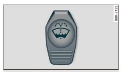
**Fig. 248** Engine compartment: cover on the windshield and headlight\* washer fluid reservoir
