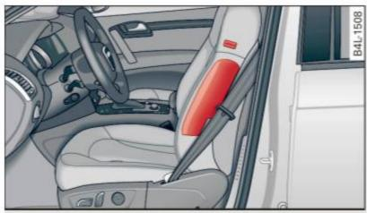
Fig. 211 Side airbag location in the driver's seat
