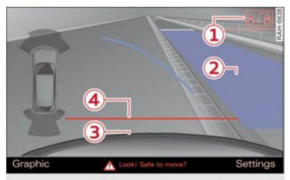
Fig. 171 MMI display: Blue surface aligned in the parking space
