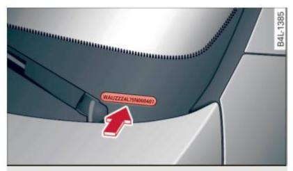
Fig. 280 Vehicle Identification Number (VIN) plate: location on driver's side dash panel
