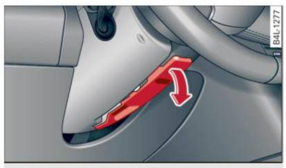
Fig. 117 Lever under the steering column
