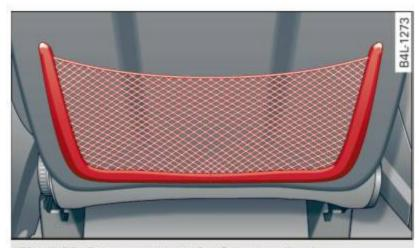
Fig. 109 Storage net on the front seatback
