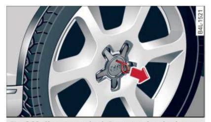
Fig. 260 Changing a wheel: Removing the wheel cover
