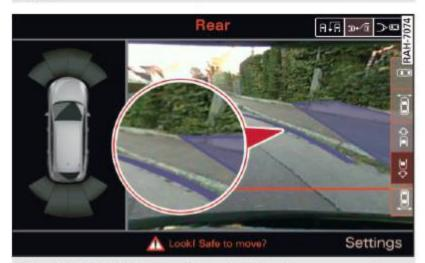
Fig. 184 MMI display: Contact of the blue curve with the curb
