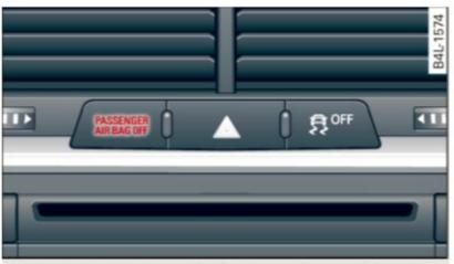
Fig. 210 Section from the instrument panel: PASSEN-GER AIR BAG OFF light
