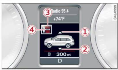
Fig. 189 Display: Adaptive Air Suspension
