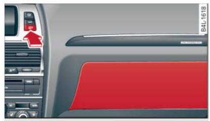
Fig. 102 Unlocking button for glove compartment
