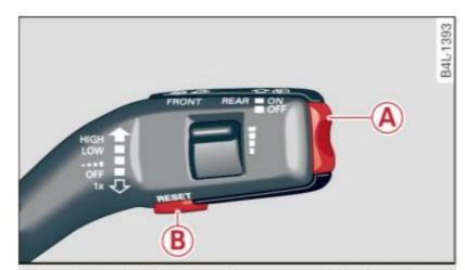
Fig. 18 Windshield wiper lever: controls for the trip computer
