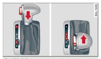
Fig. 158 Shift gate: selector lever lock positions and release button highlighted
