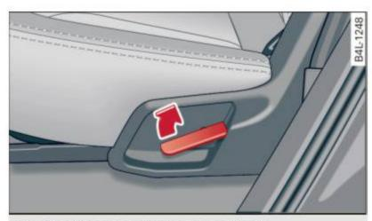
Fig. 86 Release lever for outer seatback
