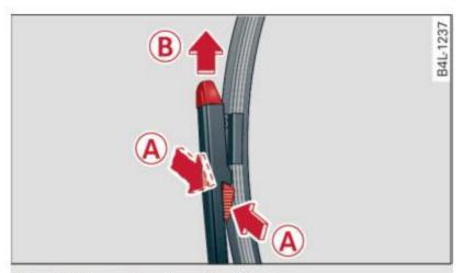
Fig. 67 Removing the wiper blades
