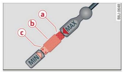
Fig. 243 Illustration of principle 2: Markers on oil dipstick
