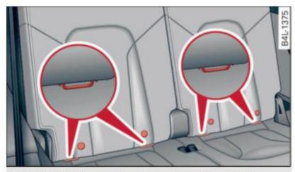
Fig. 222 Third row of seats: locator buttons for lower anchorages
