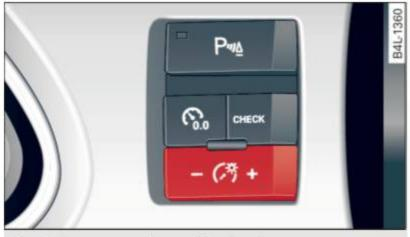
Fig. 7 Instrument cluster illumination
