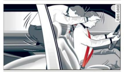
**Fig. 200** A rear passenger not wearing a safety belt will fly forward and strike the driver
