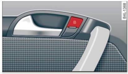
Fig. 35 Rear doors: power locking switch
