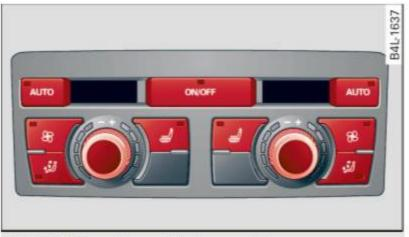
Fig. 113 Rear air conditioning controls
