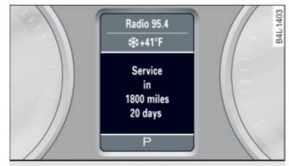
Fig. 15 Display: Service interval display
