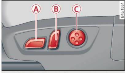
Fig. 74 Front seat: Controls for seat adjustment
