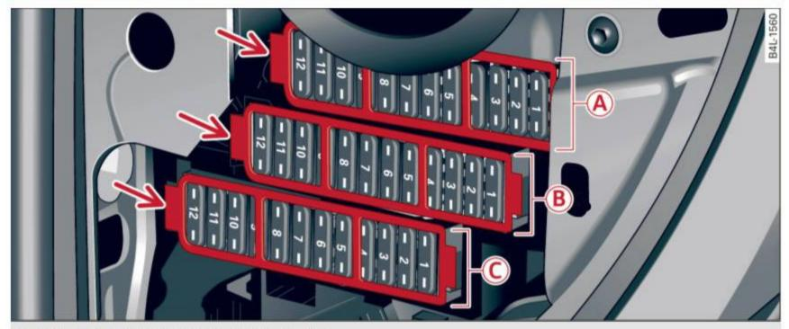
Fig. 268 Left cockpit: fuse panel with plastic clip
