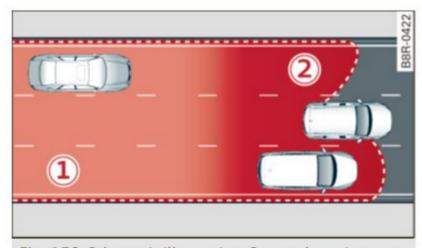
Fig. 150 Schematic illustration: Sensor detection area
