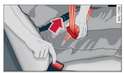
Fig. 205 Releasing the tongue from the buckle
