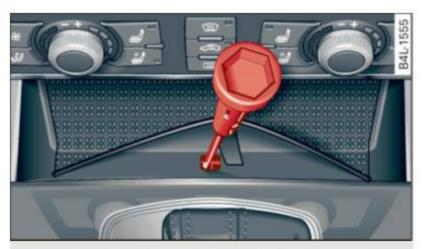
Fig. 162 Selector lever emergency release
