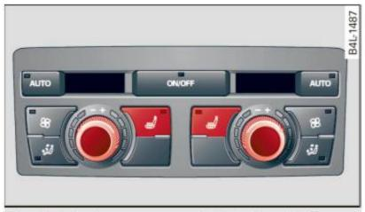
Fig. 115 Center console rear: Seat heating with fourzone automatic comfort air conditioning\*
