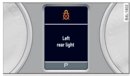
Fig. 14 Display: defective light bulb warning
