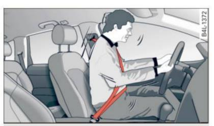
Fig. 201 Driver is correctly restrained in a sudden braking maneuver
