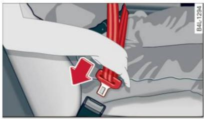
Fig. 202 Belt buckle and tongue on the driver's seat
