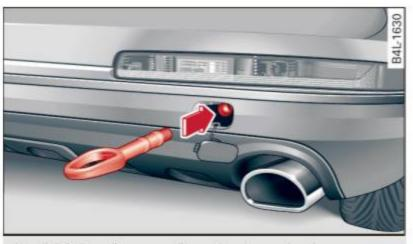
Fig. 276 Rear bumper: Screwing in towing loop
