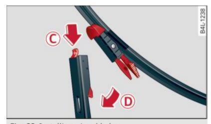
Fig. 68 Installing wiper blades
