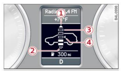
Fig. 188 Display: Adaptive Air Suspension
