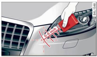
Fig. 192 Distance between the bumper and the hand transmitter
