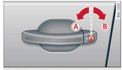
Fig. 48 Key turns for opening and closing
