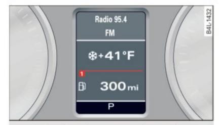
**Fig. 157** Display in the instrument cluster: selector lever in position P
