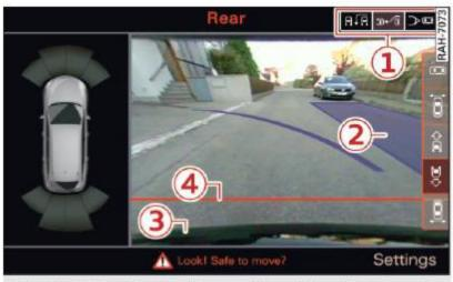
Fig. 183 MMI display: Blue surface aligned in the parking space
