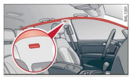
Fig. 213 Side curtain airbags, driver's side: location
