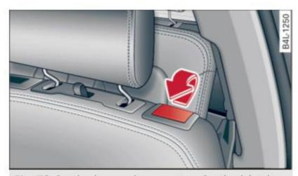
Fig. 78 Seatback second row seating: Seatback latch
