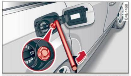
Fig. 237 Right rear vehicle side: removing the AdBlue cap
