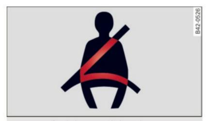
Fig. 196 Safety belt warning light in the instrument cluster - enlarged
