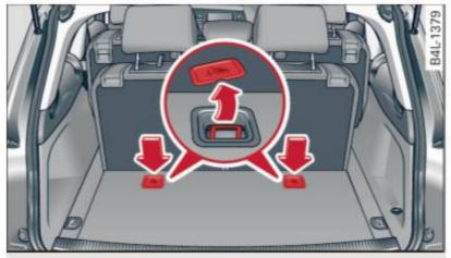
Fig. 227 Tether anchors for third row of seats: attachment hook locations
