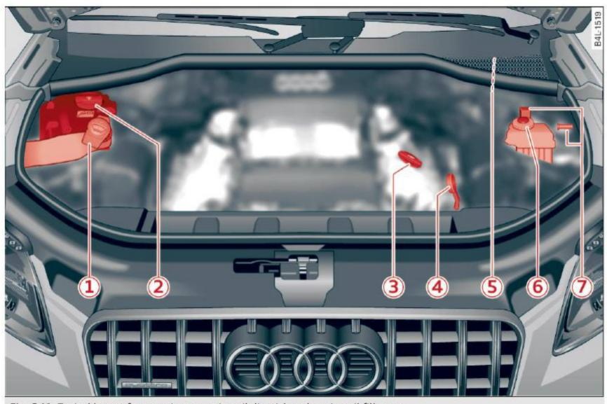
Fig. 241 Typical layout for containers, engine oil dipstick and engine oil filler cap
