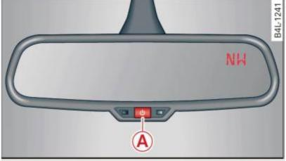
Fig. 72 Inside rear view mirror: digital compass activated
