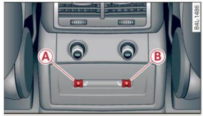
Fig. 114 Center console rear: Heated seats
