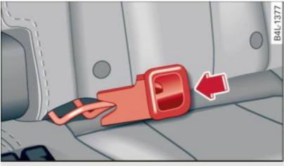
Fig. 224 Close-up: fitting the guidance fixture over the lower anchorage bracket
