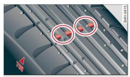
Fig. 251 Tire tread: tread wear indicators (TWI)
