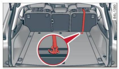
Fig. 229 Tether strap for second row seats: proper routing and mounting
