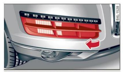
Fig. 273 Right front bumper: Removing the cover
