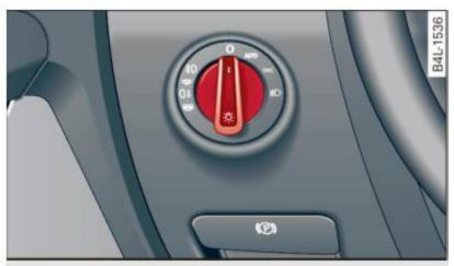
Fig. 53 Instrument panel: light switch
