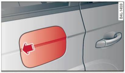
Fig. 232 Right rear vehicle side: Opening the fuel filler flap
