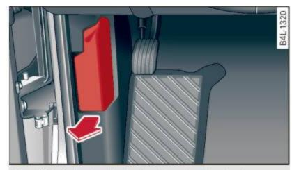
Fig. 239 Driver's side footwell: engine hood release lever
