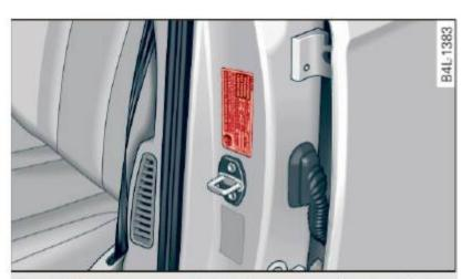
Fig. 249 Tire pressure label: located on driver's side Bpillar
