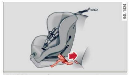
Fig. 225 Lower anchorages: proper mounting
