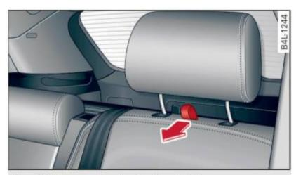
Fig. 82 Rear seat: outer head restraint
