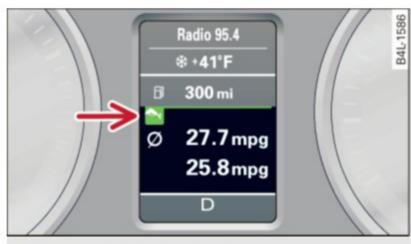
Fig. 19 Display: efficiency program
