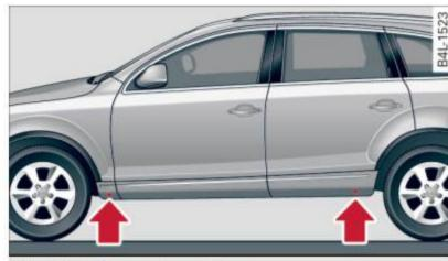
Fig. 263 Sill panels: markings
