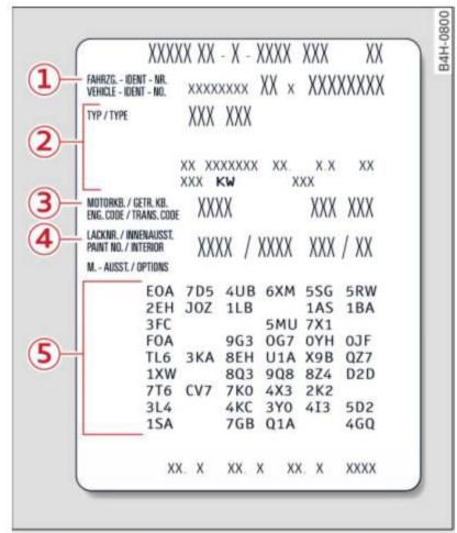
Fig. 281 Vehicle identification label: inside the luggage compartment
