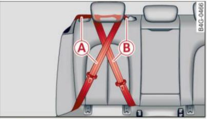
Fig. 215 Schematic overview: keep unused safety belts away from children in child safety seats. (A) - outer rear safety belt, (B) - center rear safety belt
