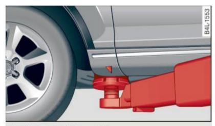
Fig. 278 Front lifting point
