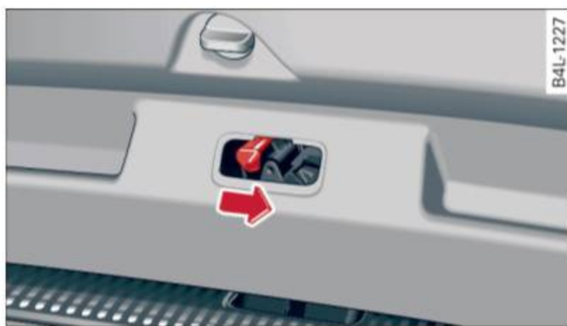
Fig. 42 Section of the luggage compartment: Emergency release
