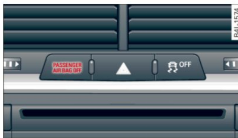
Fig. 212 Section from the instrument panel: PASSENGER AIR BAG OFF light
