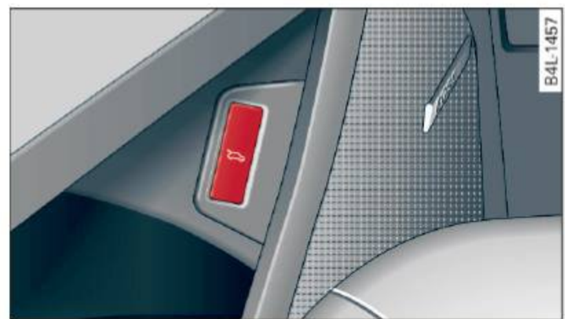
Fig. 37 Driver's door: remote rear lid release
