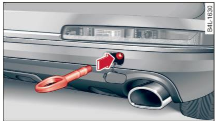
Fig. 278 Rear bumper: Screwing in towing loop
