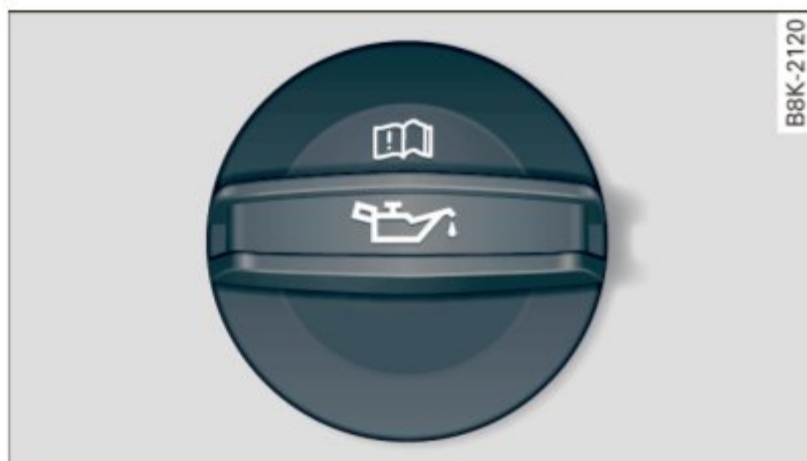
Fig. 246 Engine compartment: cover on the engine oil filler neck
