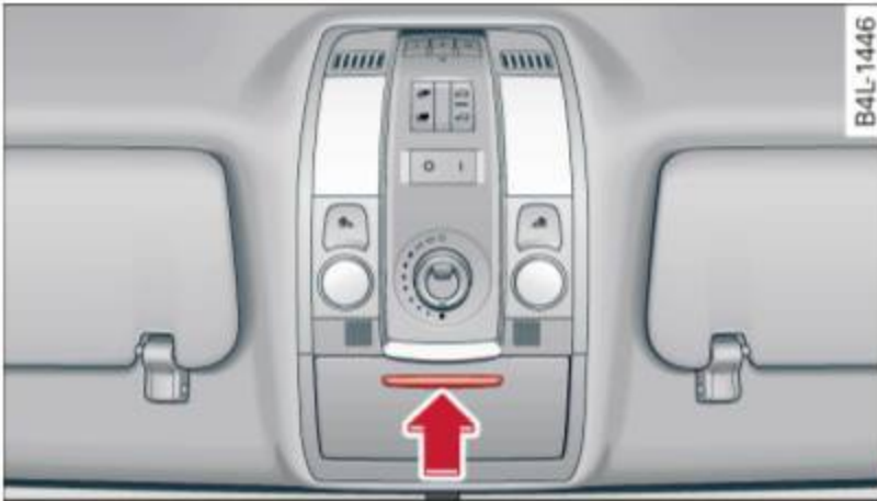
Fig. 105 Storage compartment in roof
