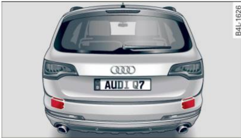
Fig. 147 Rear bumper: Position of radar sensors (not visible on outside)
