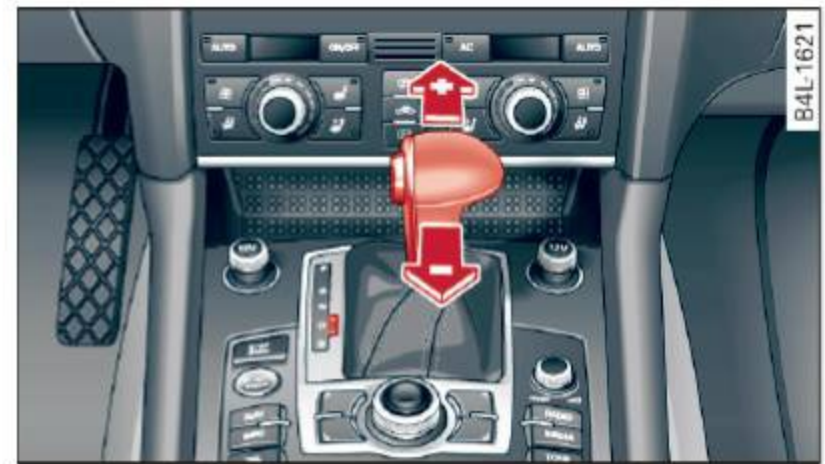
Fig. 160 Center console: shifting the tiptronic® manually
