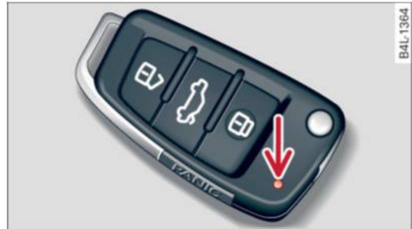
Fig. 29 Check light in the master key
