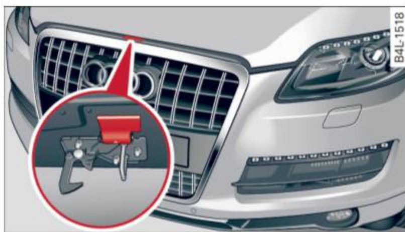
Fig. 242 Release lever under the engine hood
