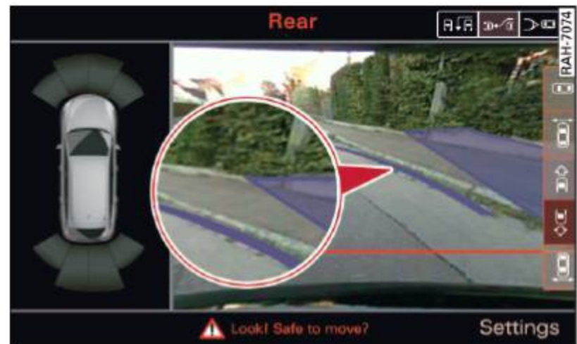
Fig. 185 MMI display: Contact of the blue curve with the curb
