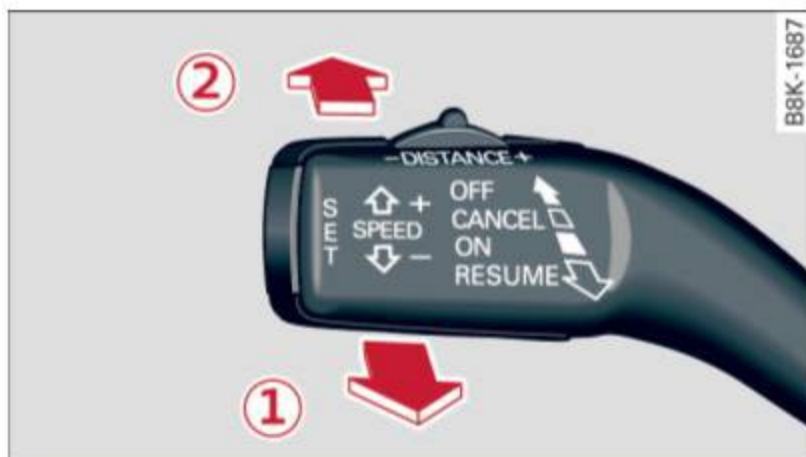
Fig. 131 Control lever: Turning adaptive cruise control off temporarily
