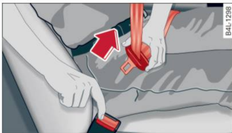
Fig. 207 Releasing the tongue from the buckle
