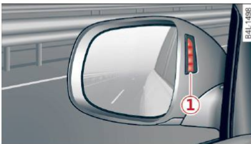
Fig. 148 Signal light on the outside mirror - driver's side
