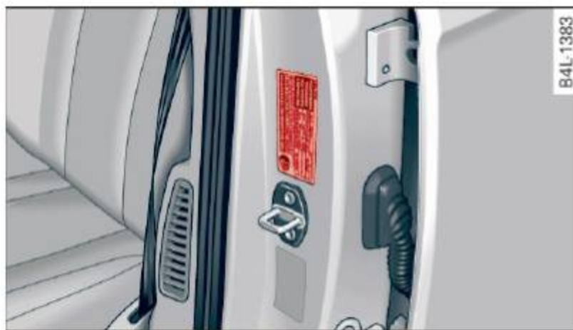
Fig. 251 Tire pressure label: located on driver's side B-pillar
