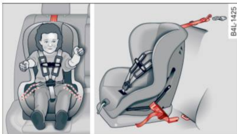
Fig. 219 Schematic overview: installation of the attachments applicable to a LATCH seat
