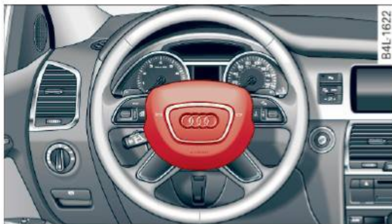
Fig. 209 Location of driver airbag: in steering wheel
