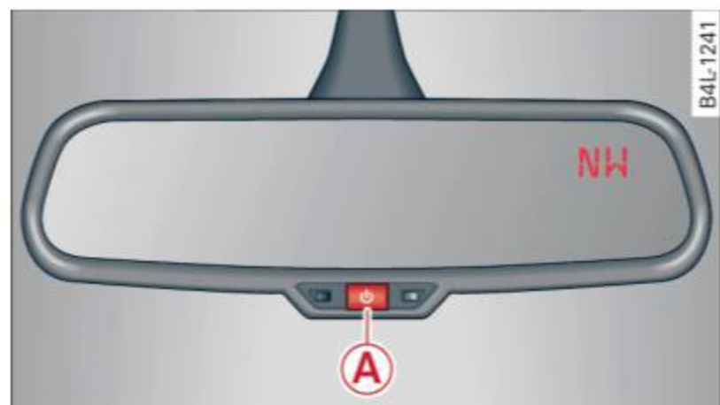
Fig. 72 Inside rear view mirror: digital compass activated
