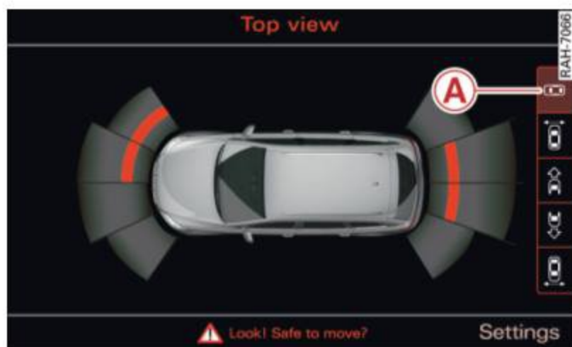
Fig. 177 MMI display: Top view mode
