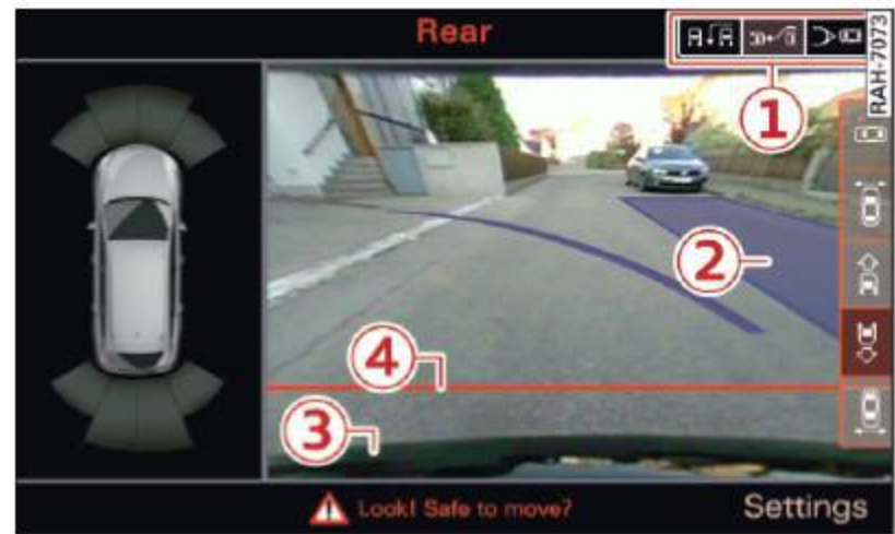
Fig. 184 MMI display: Blue surface aligned in the parking space
