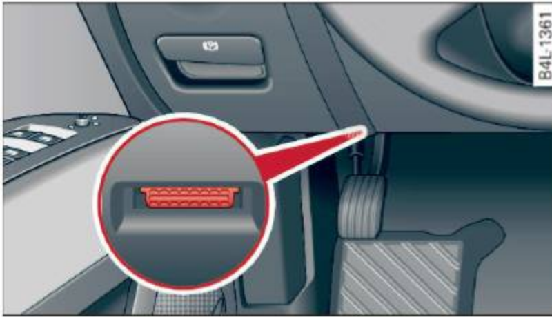
Fig. 22 Location of Data Link Connector (DLC)
