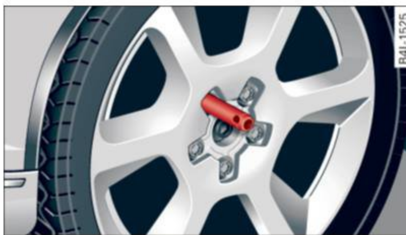
Fig. 267 Changing a wheel: alignment pin inside the top hole
