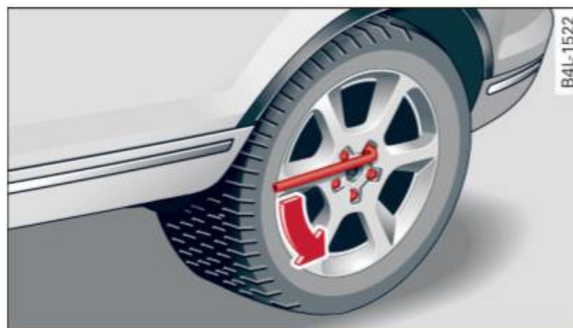
Fig. 264 Changing a wheel: loosening the wheel bolts
