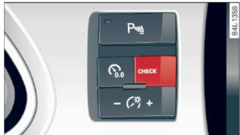
Fig. 23 CHECK button in the instrument cluster
