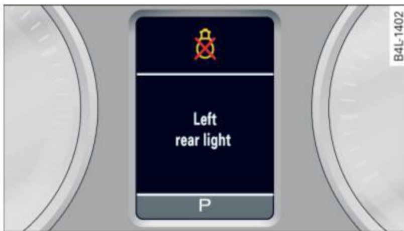
Fig. 14 Display: defective light bulb warning
