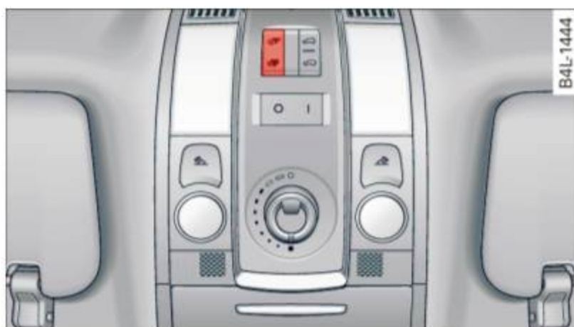
Fig. 51 Section of front headliner: Switch for sunshade
