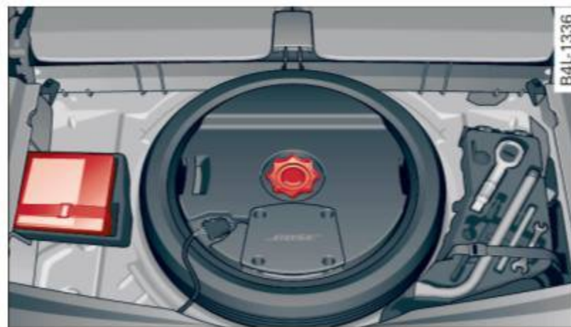
Fig. 261 Inflatable spare tire with compressor
