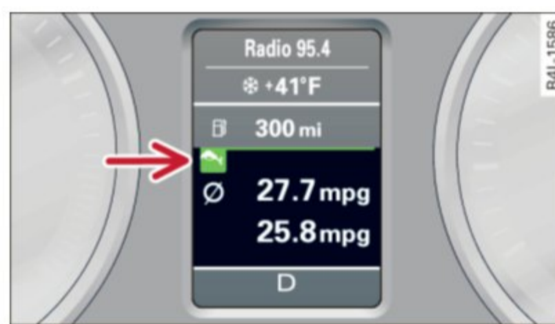
Fig. 19 Display: efficiency program
