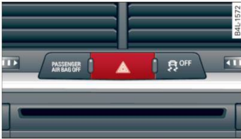
Fig. 57 Center console: emergency flasher switch
