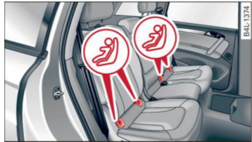
Fig. 223 Second row of seats: lower anchorage bracket locations
