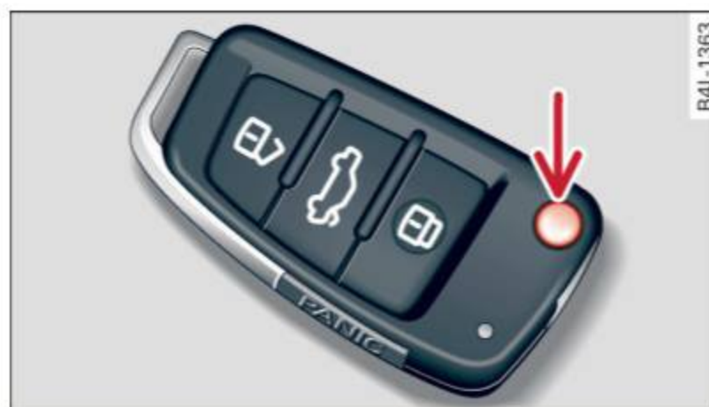
Fig. 28 Fold-up master key with remote control
