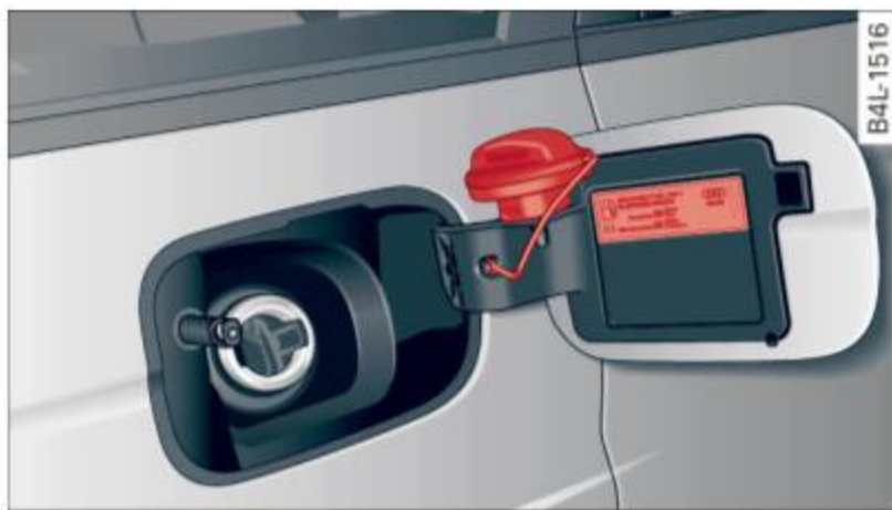
Fig. 235 Fuel cap hooked on the opened fuel filler flap
