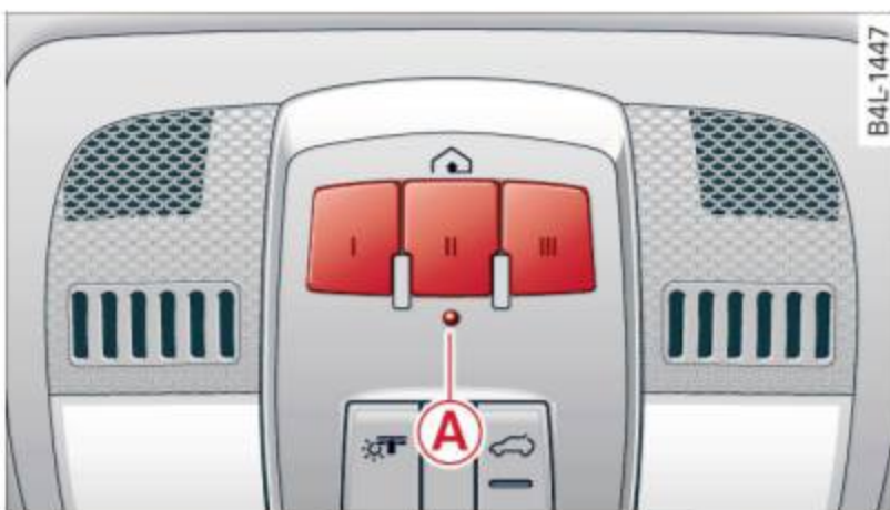
Fig. 194 Overhead console: HomeLink® keypad
