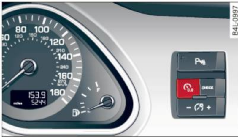
Fig. 5 Instrument cluster Odometer and reset button
