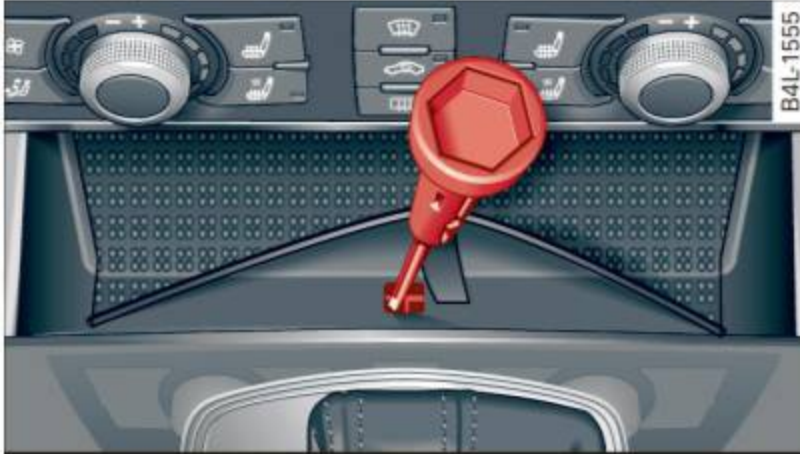
Fig. 163 Emergency release for selector lever
