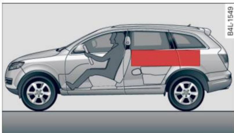
Fig. 197 Safe load positioning: place heavy objects as low and as far forward as possible.
