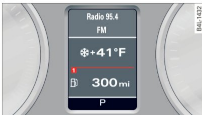
Fig. 158 Display in the instrument cluster: selector lever in position P
