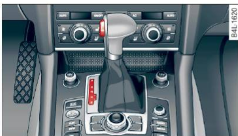
Fig. 157 Shift gate on the center console: selector lever with release button
