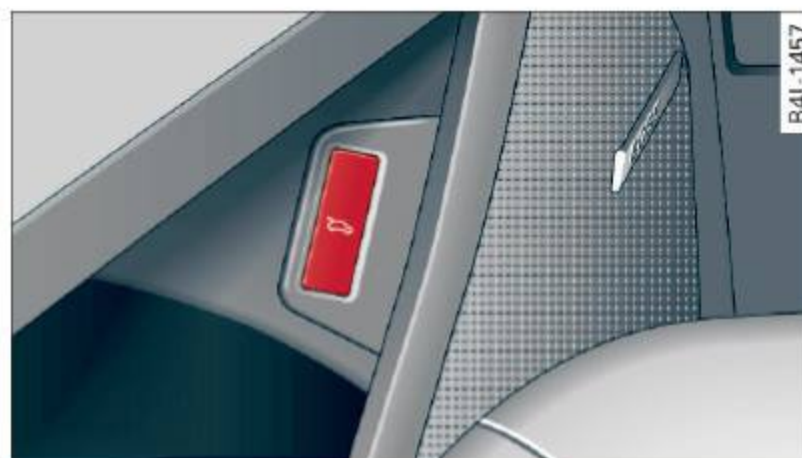
Fig. 39 Driver's door: Unlocking the rear lid
