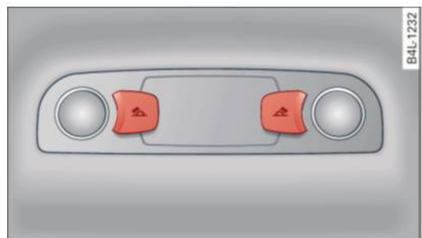
Fig. 60 Headliner: Rear reading lights
