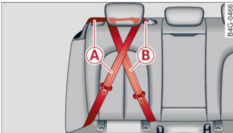
Fig. 217 Schematic overview: keep unused safety belts away from children in child safety seats. A - outer rear safety belt, B - center rear safety belt
