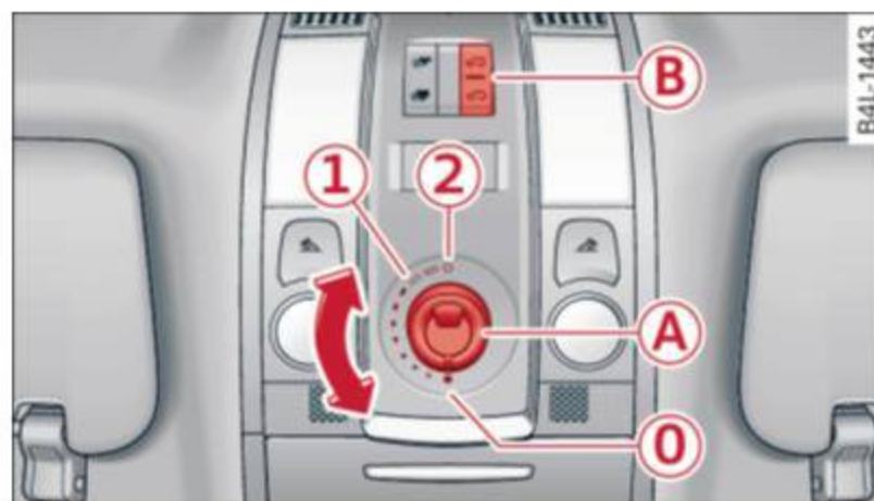
Fig. 49 Section of front headliner: Switch for Panoramic sliding sunroof
