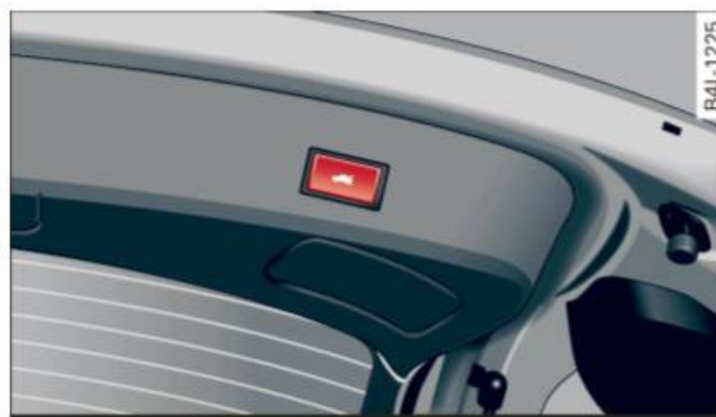
Fig. 40 Locking switch in the rear lid
