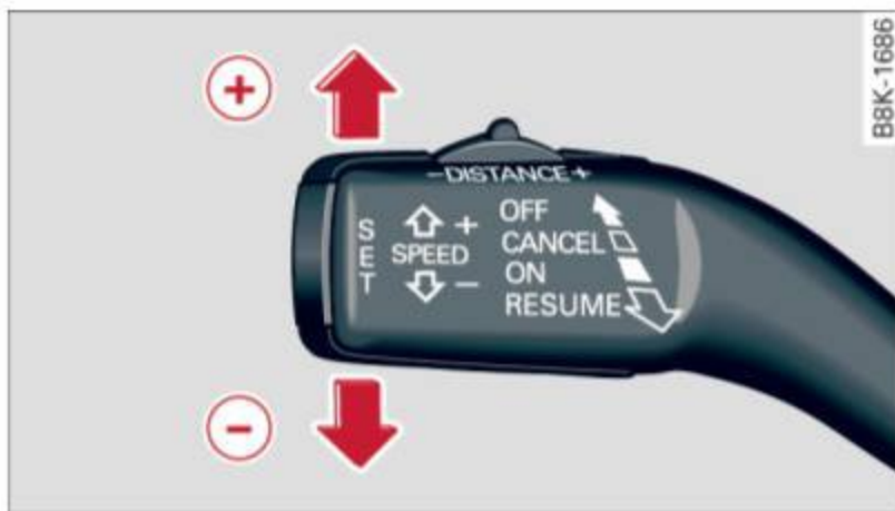
Fig. 130 Control lever: Changing speed
