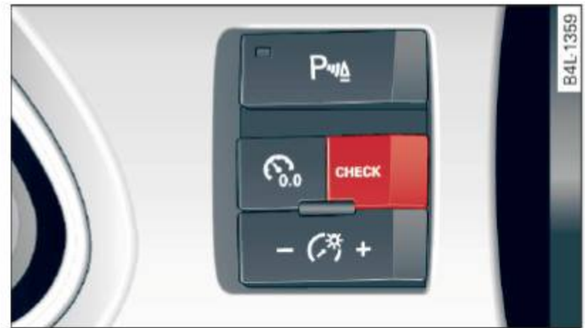
Fig. 24 Instrument cluster: CHECK button
