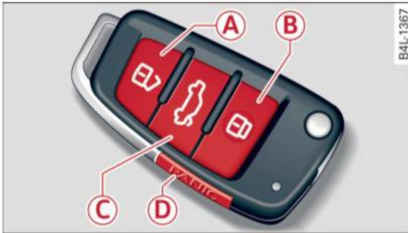
Fig. 32 Remote control: function buttons
