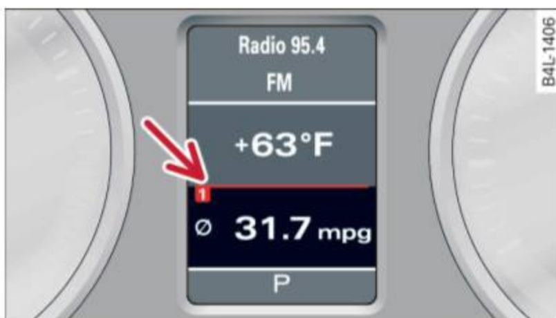
Fig. 17 Trip computer display: memory level 1
