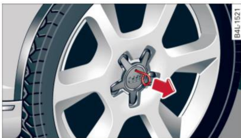
Fig. 262 Changing a wheel: Removing the wheel cover
