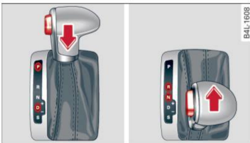
Fig. 159 Shift gate: selector lever lock positions and interlock button highlighted
