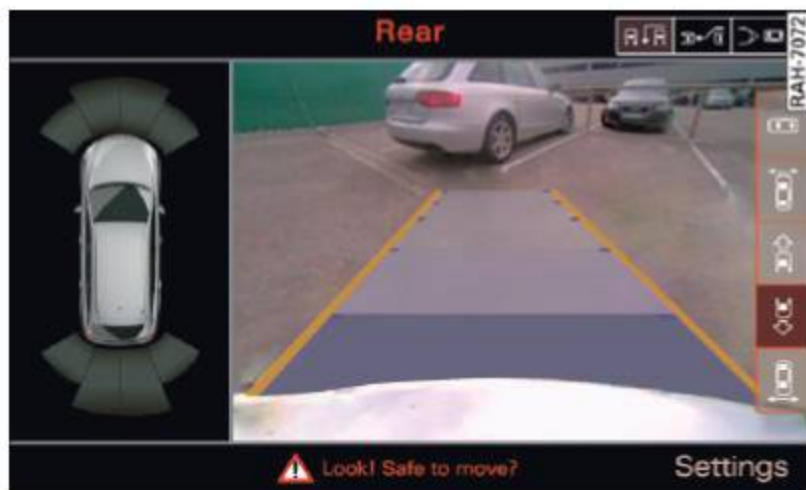
Fig. 183 MMI display: Aligning the vehicle
