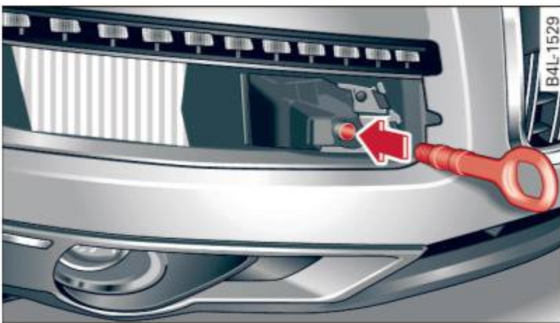
Fig. 276 Right front bumper without cover: Screwing in towing loop
