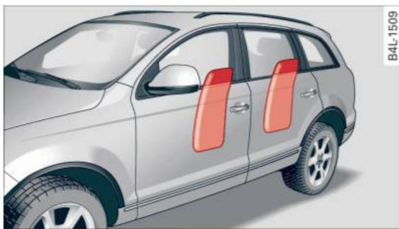
Fig. 214 Inflated side airbags on left side of vehicle, rear side airbag optional equipment
