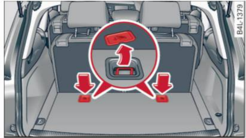
Fig. 229 Tether anchors for third row of seats: attachment hook locations
