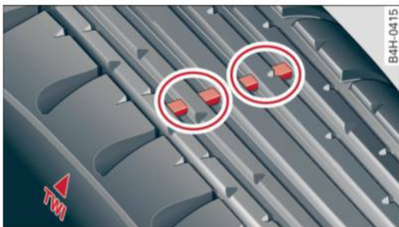
Fig. 253 Tire tread: tread wear indicators (TWI)
