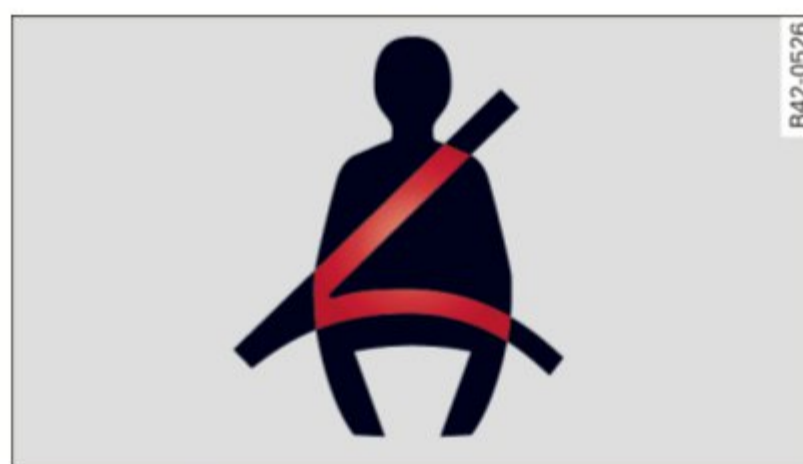
Fig. 198 Safety belt warning light in the instrument cluster - enlarged
