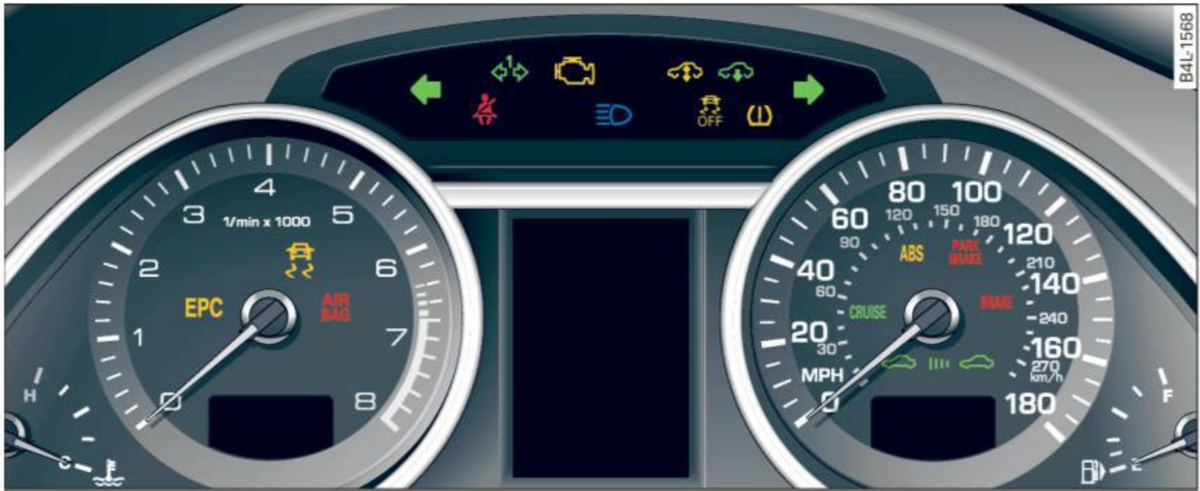
Fig. 8 Instrument cluster with warning/indicator lights
