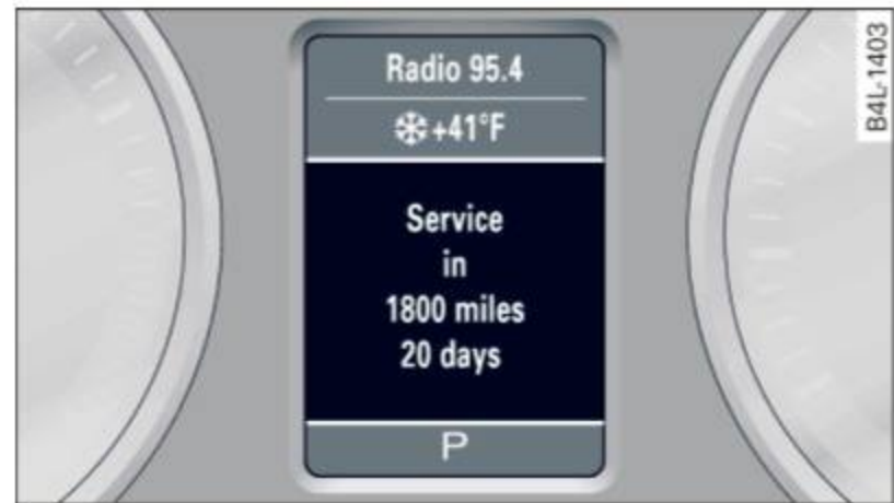
Fig. 15 Display: Service interval display
