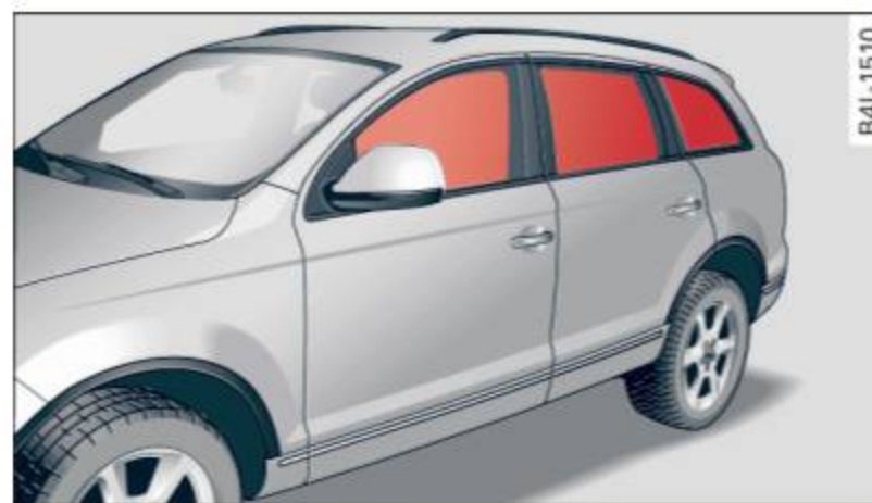
Fig. 216 Illustration of principle: Inflated side curtain airbags on the left side
