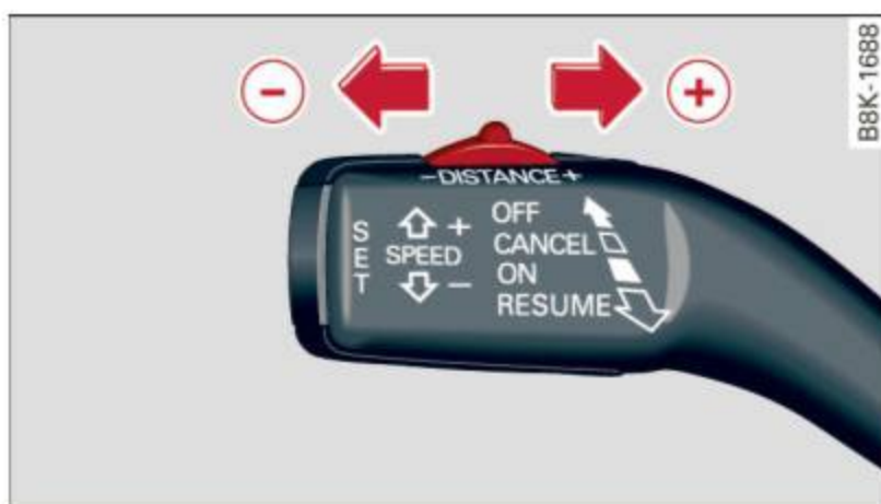
Fig. 133 Control lever: Setting distance
