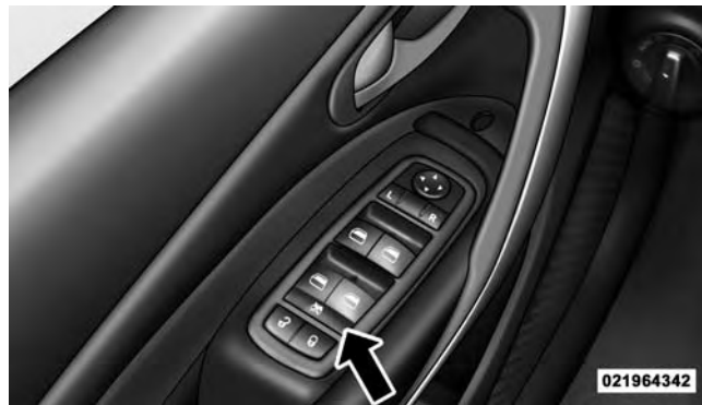
Window Lockout Switch
