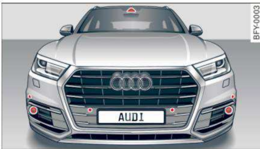
Fig. 100 Front of the vehicle: sensors and video camera
