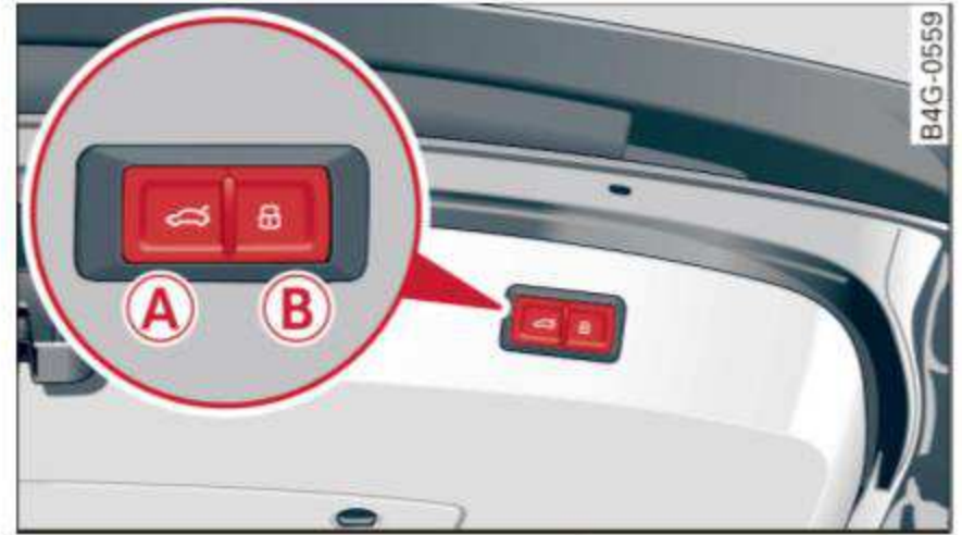
Fig. 28 Luggage compartment lid: (A) closing button, (B) lock button (vehicles with convenience key*)
