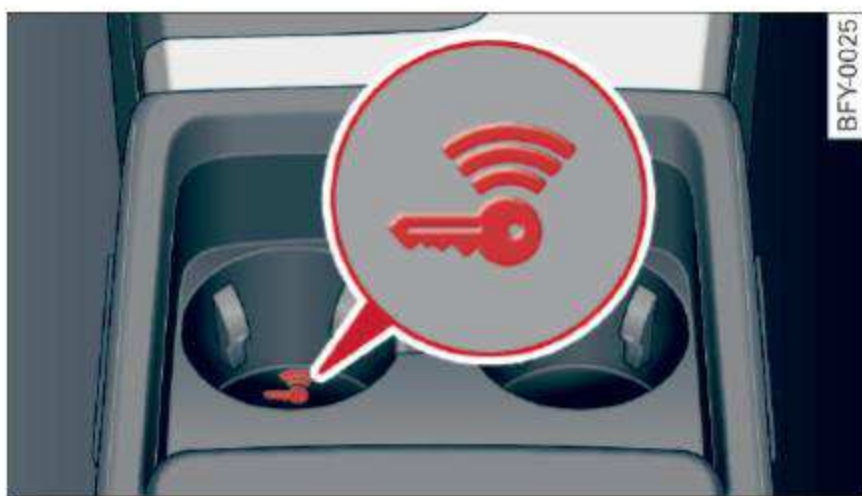
Fig. 87 Center console/remote control key: starting the engine if there is a malfunction
