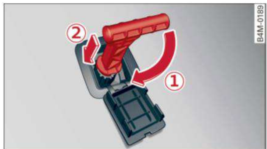
Fig. 93 Driver's side footwell: releasing the parking lock using the emergency release
