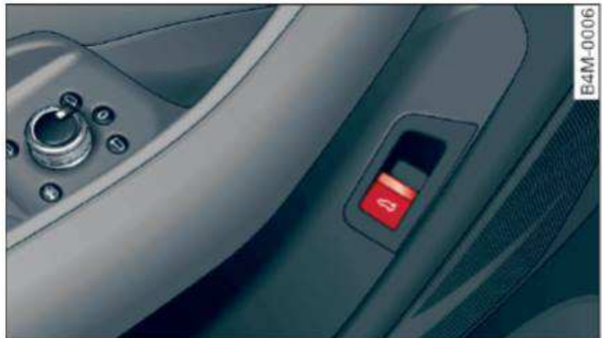
Fig. 26 Driver's door: opening the luggage compartment lid
