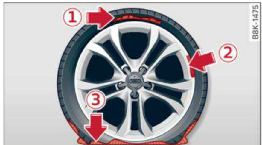
Fig. 271 Tire: tire damage that cannot be repaired
