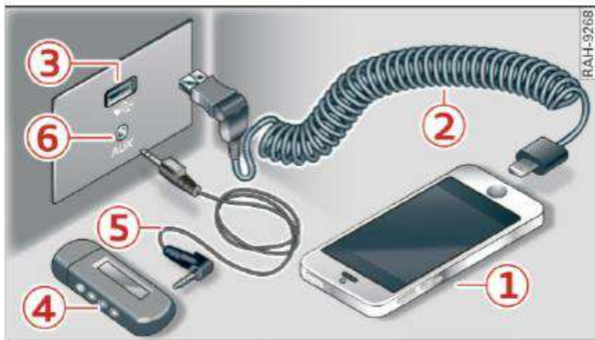
Fig. 209 Storage compartment under the center armrest and at the front* of the center console: diagram: Audi music interface
