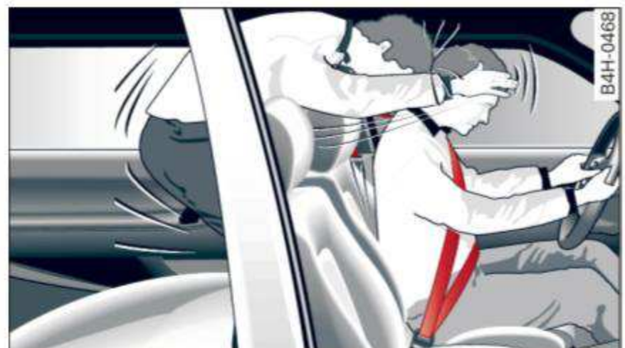
Fig. 226 A rear passenger not wearing a safety belt will fly forward and strike the driver
