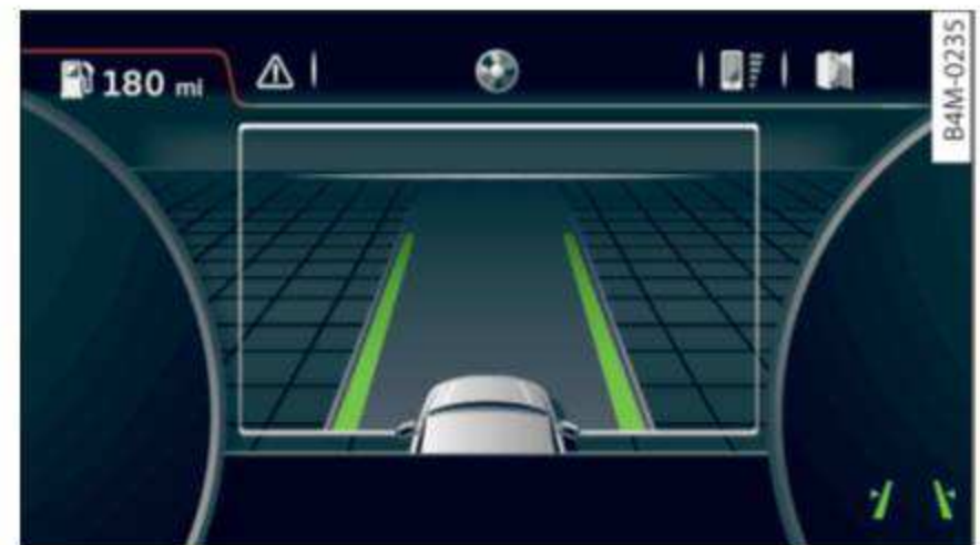
Fig. 116 Instrument cluster (multi-color display): active lane assist is switched on and ready to provide warnings
