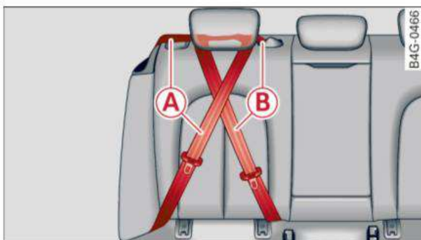
Fig. 241 Schematic overview: keep unused safety belts away from children in child safety seats. A - outer rear safety belt, B - center rear safety belt
