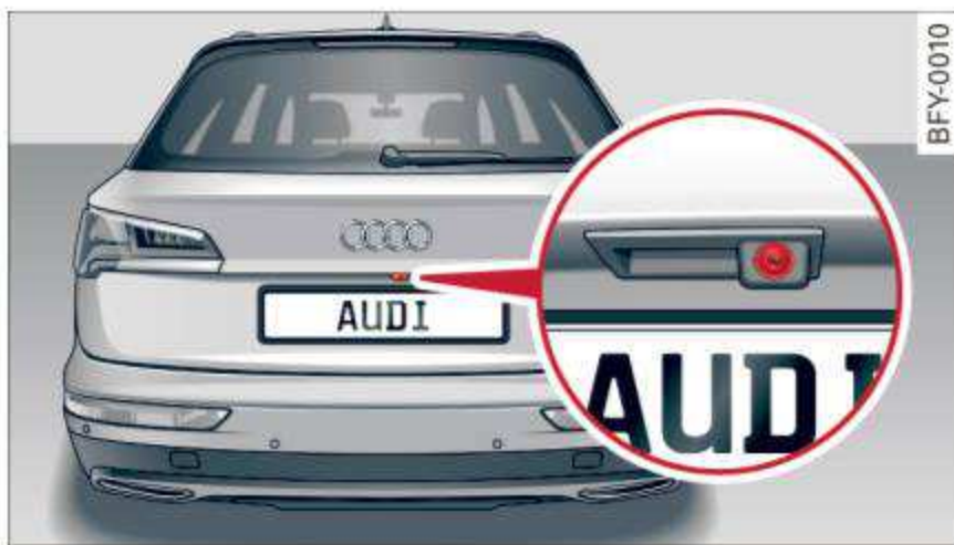
Fig. 133 Luggage compartment lid: location of the rearview camera
