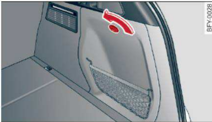
Fig. 255 Right side trim panel in the luggage compartment: opening the trim panel
