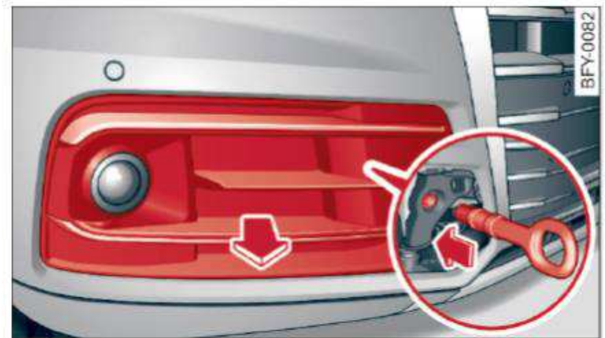
Fig. 288 Front bumper: installing the towing loop
