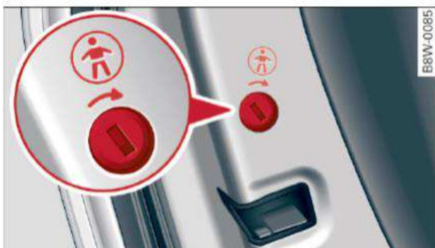
Fig. 32 Rear door: child safety lock
