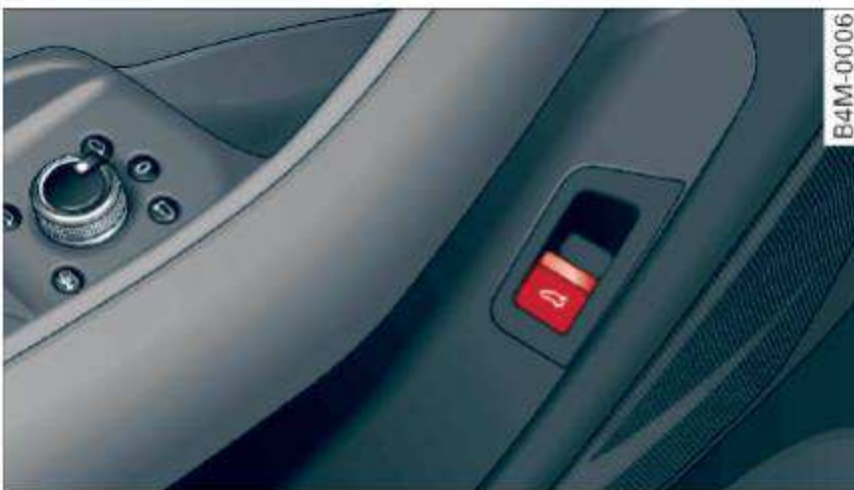
Fig. 27 Driver's door: opening the luggage compartment lid
