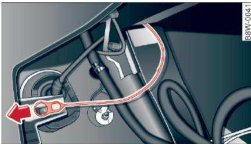
Fig. 256 Luggage compartment: fuel filler door emergency release
