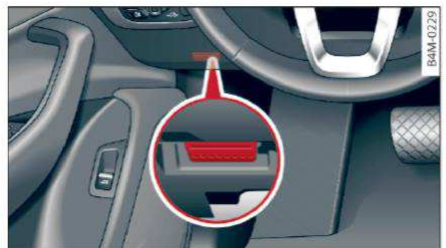
Fig. 257 Footwell on left side of the vehicle: connection port for the On-Board Diagnostic System (OBD)
