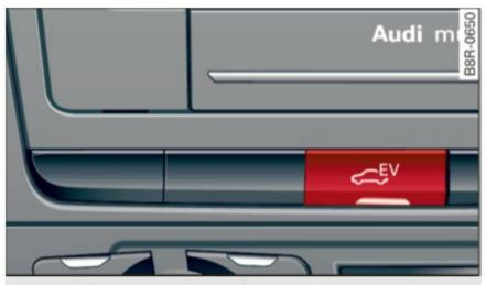
► To turn on EV mode, press the <a>B</a> button. The indicator light in the button will turn on. The indicator light also turns on in the instrument cluster display.
