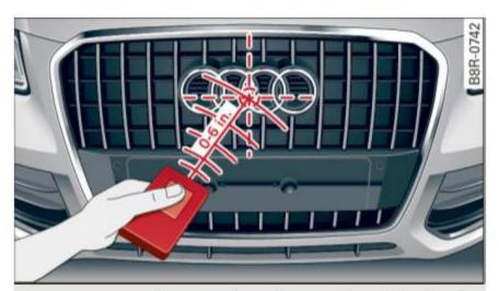
Fig. 45 Distance between the radiator grille and the hand transmitter
