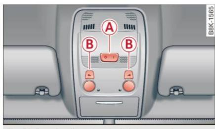
Fig. 51 Front headliner: interior lighting controls
