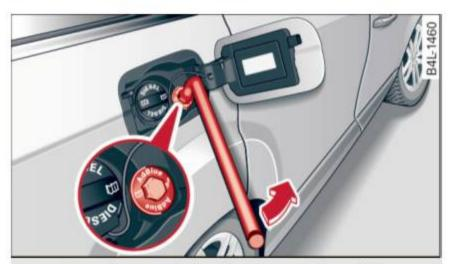
Fig. 193 Right rear vehicle side: removing the AdBlue cap
