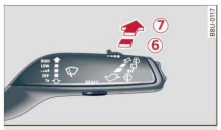
Fig. 57 Rear wiper actuation
