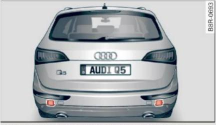
Fig. 130 Rear of the vehicle: Position of the sensors
