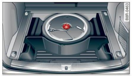
Fig. 212 Inflatable spare tire with compressor
