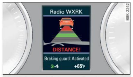
Fig. 126 Instrument cluster: approach warning
