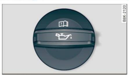
Fig. 199 Engine compartment: cover on the engine oil filler neck
