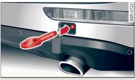
Fig. 232 Rear bumper: Screwing in towing loop
