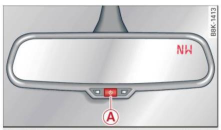
Fig. 62 Inside rear view mirror: digital compass activated
