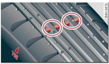
Fig. 205 Tire profile: Treadwear indicator
