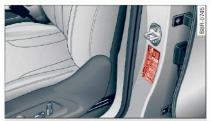
Fig. 206 Driver's side B-pillar: tire pressure label
