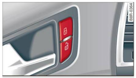
Fig. 32 Driver's door: power locking switch
