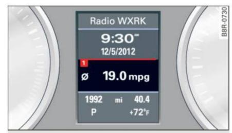
Fig. 15 Trip computer display: Average fuel mileage
