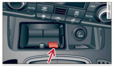
Fig. 140 Selector lever emergency release
