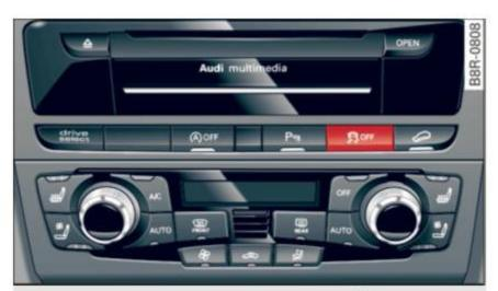
Fig. 186 Version B: Upper center console, 🕏 OFF button
