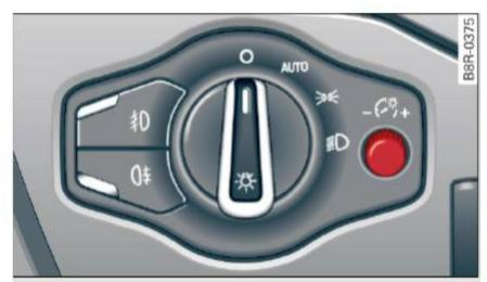
Fig. 53 Instrument illumination
