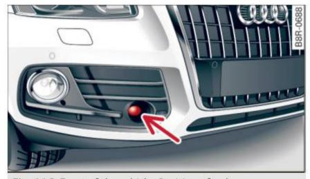
Fig. 116 Front of the vehicle: Position of radar sensor
