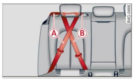
Fig. 173 Schematic overview: keep unused safety belts away from children in child safety seats. (A) - outer rear safety belt, (B) - center rear safety belt
