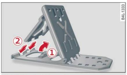
Fig. 210 Opening folding chocks
