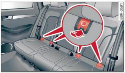
Fig. 179 Lower anchorages, covers marked
