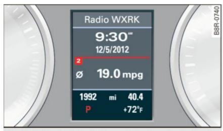
**Fig. 134** Display in the instrument cluster: selector lever in position P
