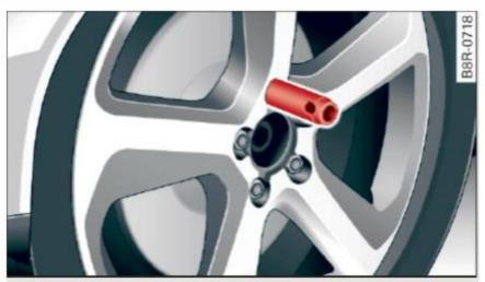
Fig. 222 Changing a wheel: alignment pin inside the top hole
