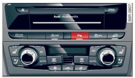
Fig. 145 Center console: Parking system switch
