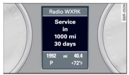
Fig. 14 Instrument cluster: Service interval display
