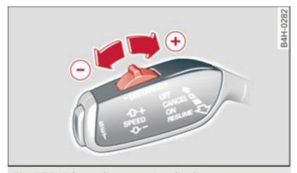
Fig. 122 Selector lever: setting the distance
