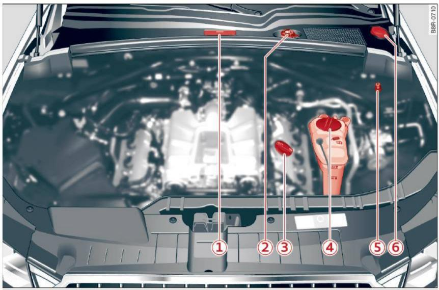
Fig. 196 Typical layout for containers and engine oil filler cap
