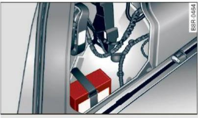
Fig. 213 Luggage compartment left side: compressor
