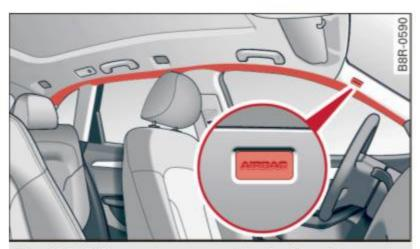
Fig. 172 Side curtain system, driver's side: side curtain airbag location
