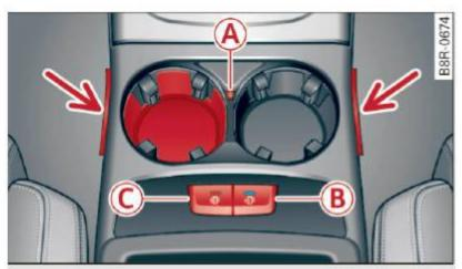
Fig. 84 Center console: climatized cupholder
