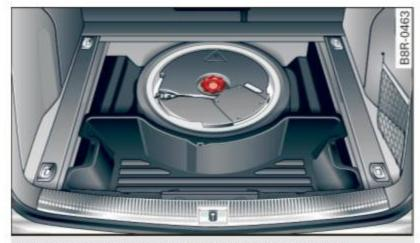
Fig. 212 Inflatable spare tire with compressor
