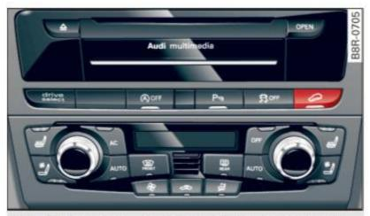
Fig. 188 Top of the center console: hill descent assist button
