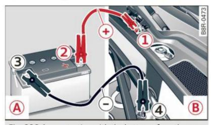
Fig. 228 Jump starting with the battery of another vehicle: (A) booster battery, (B) discharged vehicle battery
