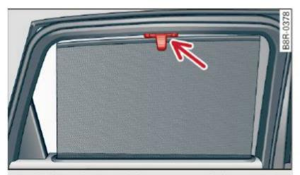
Fig. 52 Sun shade pulled up on a rear window
