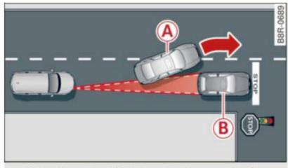
Fig. 116 Example: object changing lanes and stationary object
