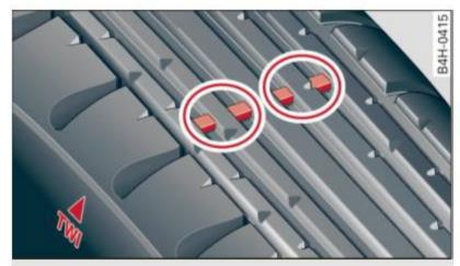
Fig. 205 Tire tread: tread wear indicators (TWI)
