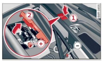
Fig. 201 Engine compartment: Connectors for charger and jumper cables
