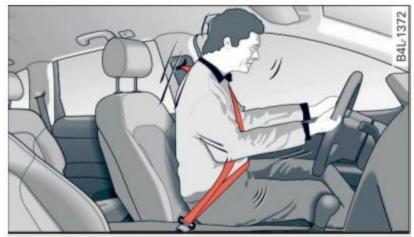
Fig. 160 Driver is correctly restrained in a sudden braking maneuver
