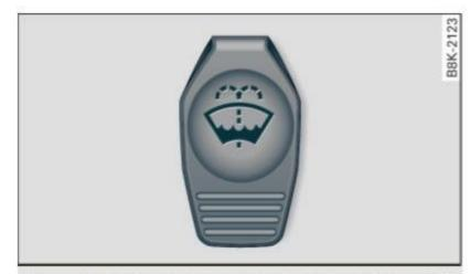
Fig. 202 Engine compartment: cover on the windshield and headlight\* washer fluid reservoir
