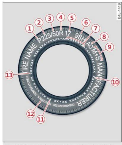
Fig. 207 Tire specification codes on the sidewall of a tire
