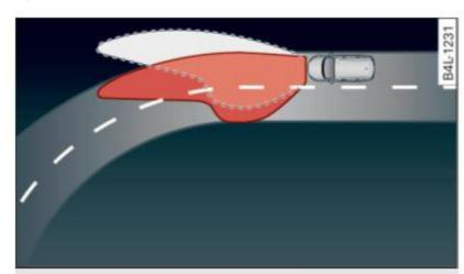
Fig. 46 Adaptive light when driving
