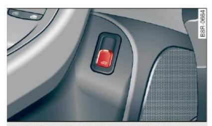
Fig. 34 Driver's door: remote rear lid release
