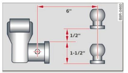
Fig. 190 Permitted ball position of the trailer hitch
