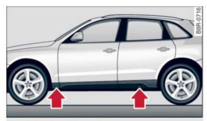
Fig. 219 Sill panels: markings
