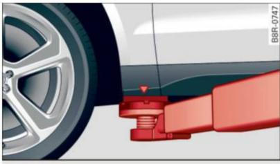
Fig. 234 Front lifting point
