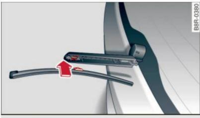
Fig. 56 Rear wiper: Removing the wiper blade
