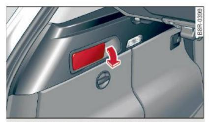
Fig. 71 Luggage compartment: release lever
