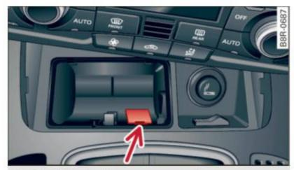
Fig. 138 Selector lever emergency release
