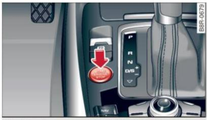
Fig. 100 Center console: START ENGINE STOP button
