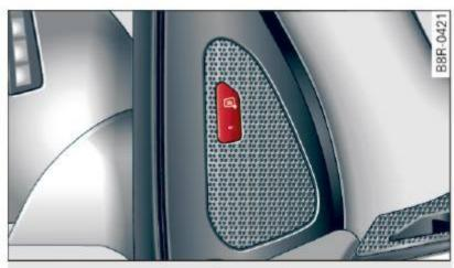
Fig. 129 Driver's door: Side assist button
