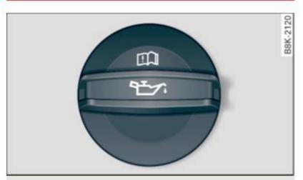
Fig. 198 Engine compartment: cover on the engine oil filler neck
