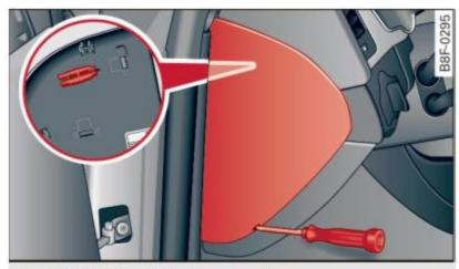
Fig. 223 Left cockpit: fuse panel cover
