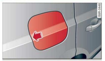
Fig. 191 Right rear vehicle side: Opening the fuel filler flap
