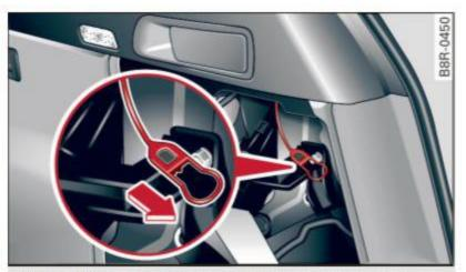
Fig. 193 Luggage compartment: Emergency opening of fuel filler flap
