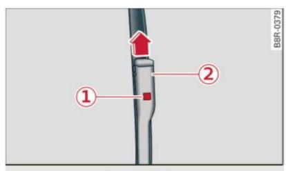
Fig. 55 Removing the wiper blade
