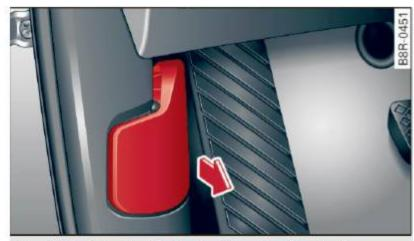
Fig. 194 Driver's side footwell: engine hood release lever
