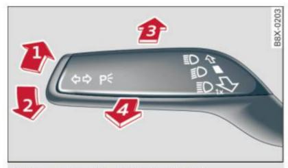
Fig. 48 Turn signal and high beam lever
