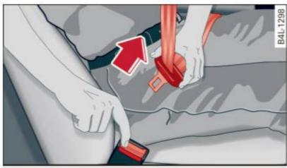
Fig. 164 Releasing the tongue from the buckle
