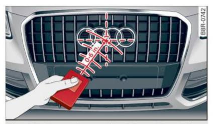
Fig. 151 Distance between the radiator grille and the hand transmitter
