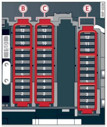
Fig. 226 Right luggage compartment: fuse panel with plastic clip
