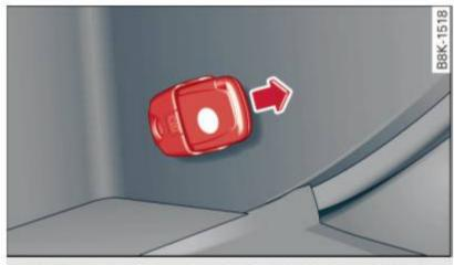
**Fig. 98** Glove compartment: Adapter for emergency key
