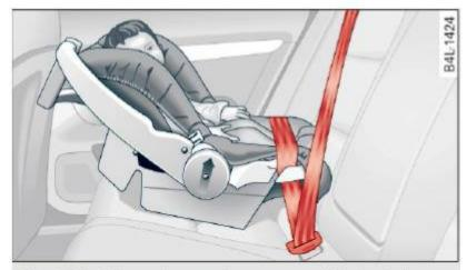
Fig. 175 Schematic overview: rearward-facing infant seat, properly installed on the rear seat
