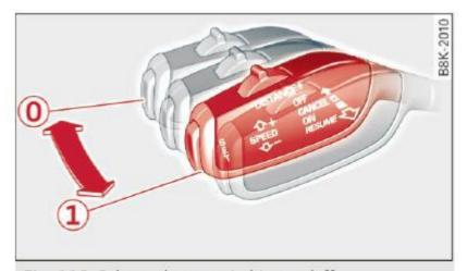
Fig. 118 Selector lever: switching on/off
