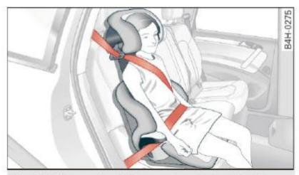
Fig. 178 Rear seat: child properly restrained in a booster seat
