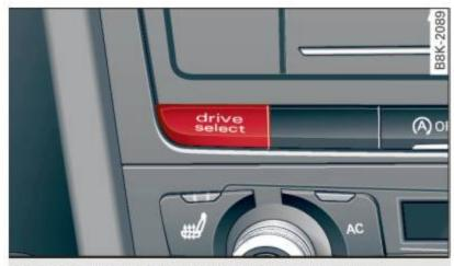
Fig. 130 Center console: Control for drive select
