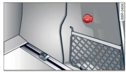
Fig. 88 Section of the trim panel of the luggage compartment: 12-volt socket
