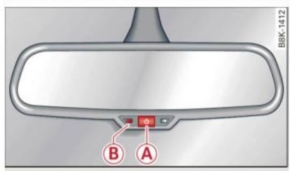
Fig. 58 Automatic dimming rearview mirror\*
