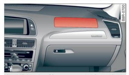
**Fig. 167** Location of front passenger's airbag: in the instrument panel
