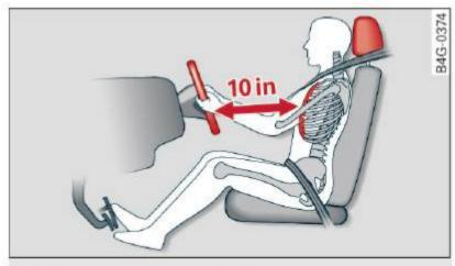
Fig. 152 Correct seating position
