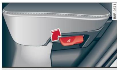
Fig. 69 Release lever for the outer backrest
