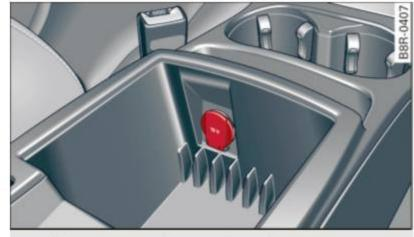
Fig. 89 Center console: 12-volt socket
