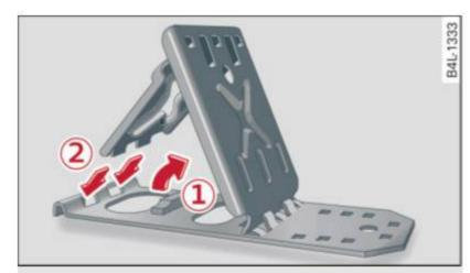
Fig. 210 Opening folding chocks
