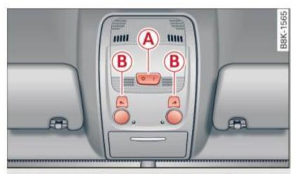
Fig. 49 Headliner: Front interior/reading lights
