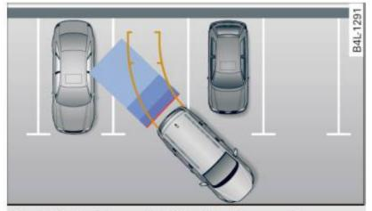
Fig. 139 Parking mode 1: Backing into a parking space
