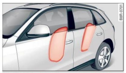
Fig. 171 Inflated side airbags on left side of vehicle
