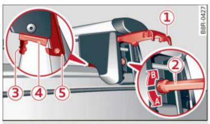
Fig. 80 Roof railing: installing a roof rack
