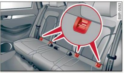
Fig. 181 Rear seats: lower anchorage bracket locations
