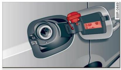
Fig. 192 Fuel filler flap with attached fuel cap
