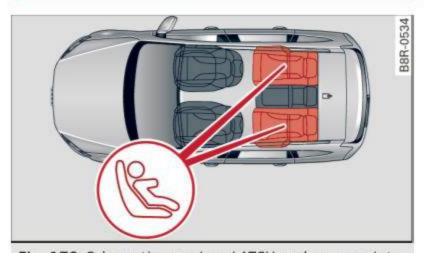
Fig. 179 Schematic overview: LATCH anchorage point locations
