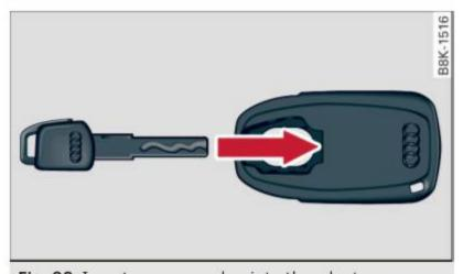
Fig. 99 Insert emergency key into the adapter
