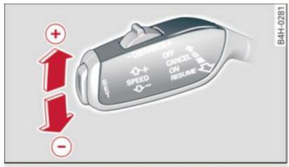
Fig. 120 Selector lever: changing the speed
