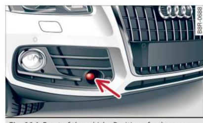
Fig. 114 Front of the vehicle: Position of radar sensor
