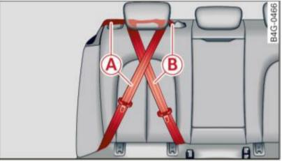
Fig. 174 Schematic overview: keep unused safety belts away from children in child safety seats. (A) - outer rear safety belt, (B) - center rear safety belt
