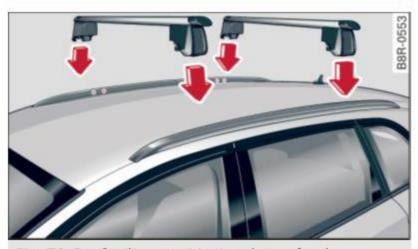
Fig. 79 Roof railing: positioning the roof rack
