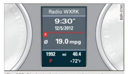
**Fig. 132** Display in the instrument cluster: selector lever in position P
