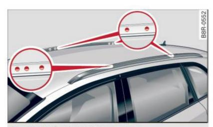
Fig. 78 Roof rack attachment points
