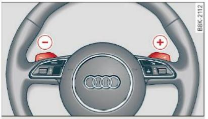
Fig. 136 Steering wheel: Shift buttons\*
