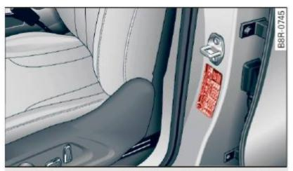
Fig. 203 Tire pressure label: located on driver's side Bpillar
