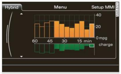
Fig. 112 MMI display: consumption display
