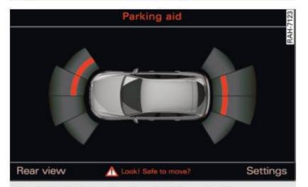
Fig. 144 MMI display: visual distance display
