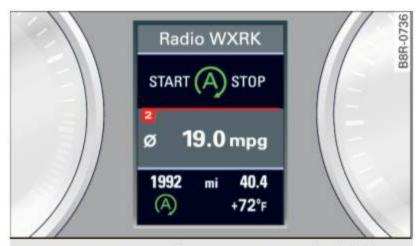
**Fig. 102** Instrument cluster: Engine switched off (stop phase)
