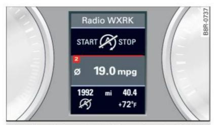
**Fig. 103** Instrument cluster: Engine-Stop temporarily unavailable
