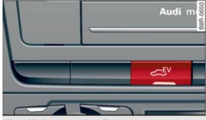
► To turn on EV mode, press the button. The indicator light in the button will turn on. The indicator light also turns on in the instrument cluster display.
