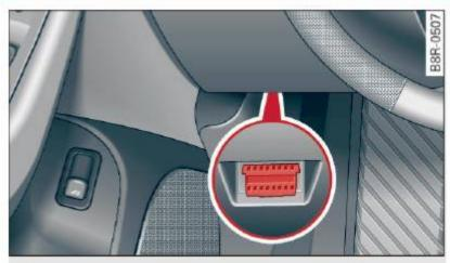
Fig. 21 Location of Data Link Connector (DLC)
