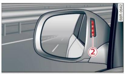
Fig. 126 Display on the exterior mirror
