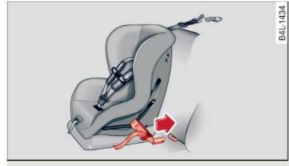
Fig. 182 Lower anchorages: proper mounting
