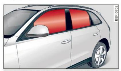
Fig. 173 Illustration of principle: Inflated side curtain airbags on the left side
