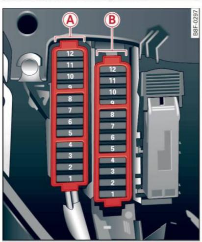
Fig. 225 Right cockpit: fuse panel with plastic clip
