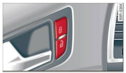
Fig. 32 Driver's door: power locking switch
