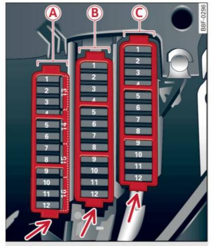
Fig. 224 Left cockpit: fuse panel with plastic clip
