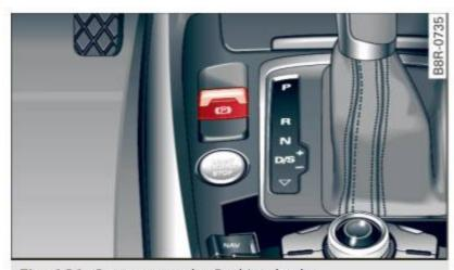
Fig. 101 Center console: Parking brake
