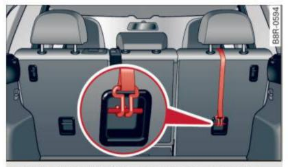
Fig. 185 Tether strap: proper routing and mounting
