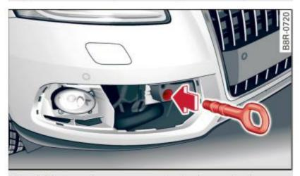
Fig. 230 Front bumper: screwing in the towing loop
