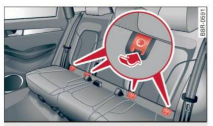
Fig. 180 Lower anchorages, covers marked
