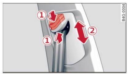
**Fig. 165** Safety belt height adjustment for the front seats – loop-around fittings
