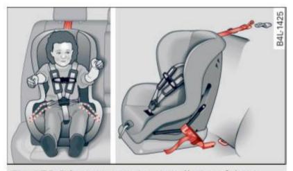
**Fig. 176** Schematic overview: installation of the attachments applicable to a LATCH seat
