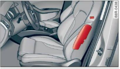
Fig. 170 Side airbag location in the driver's seat
