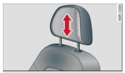
**Fig. 65** Front seats head restraints: adjusting the height
