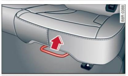
Fig. 64 Fore-and-aft adjustment
