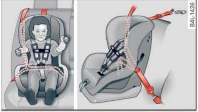
Fig. 177 Schematic overview: installation of the seat using the vehicle's safety belt system
