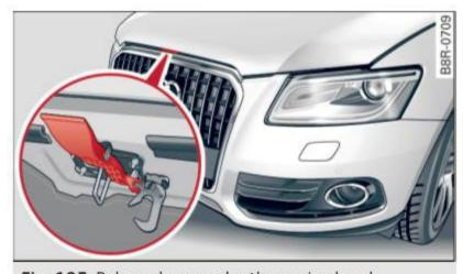
Fig. 195 Release lever under the engine hood
