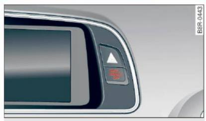
Fig. 169 Section from the instrument panel: PASSEN-GER AIR BAG OFF light
