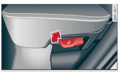
Fig. 63 Adjusting seatback angle
