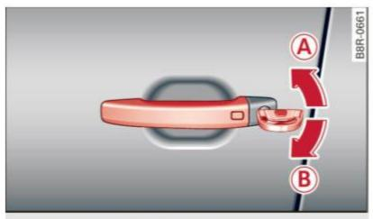
Fig. 31 Key turns for opening and closing
