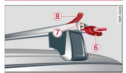
Fig. 81 Roof railing: installing cover profile into the roof rack
