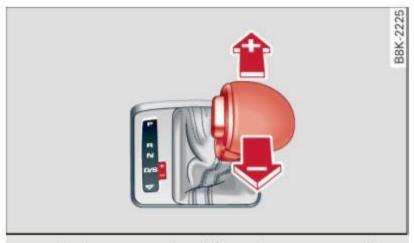
Fig. 135 Center console: shifting the gears manually
