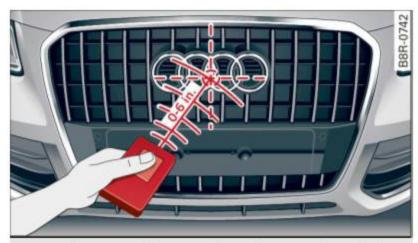
Fig. 150 Distance between the radiator grille and the hand transmitter
