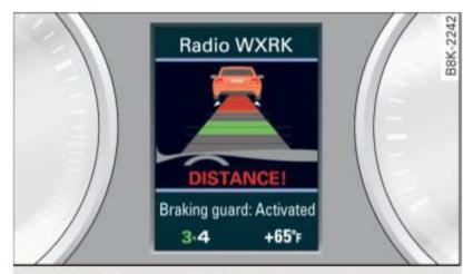
Fig. 124 Instrument cluster: approach warning
