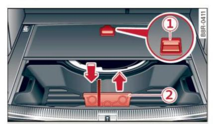
Fig. 75 Luggage compartment: cargo floor folded together with protective tray
