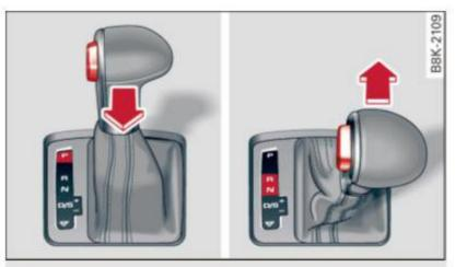
Fig. 133 Shift gate: selector lever lock positions and release button highlighted
