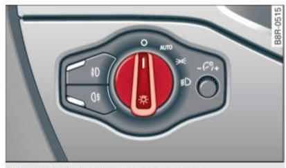
Fig. 43 Instrument panel: light switch
