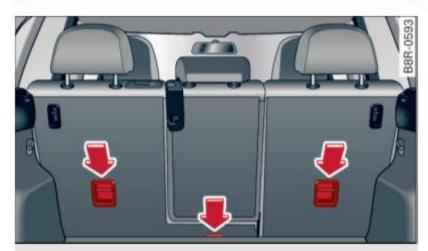
Fig. 183 Tether anchors: attachment hook locations behind the rear seatbacks
