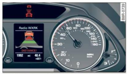
Fig. 123 Instrument cluster: request for driver intervention
