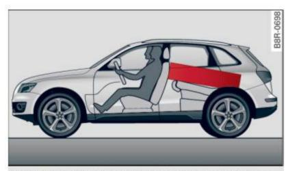
**Fig. 154** Safe load positioning: place heavy objects as low and as far forward as possible.
