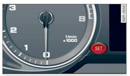
Fig. 105 SET button in the instrument cluster
