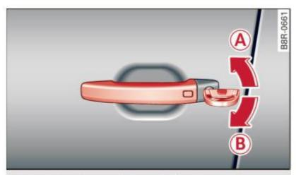
Fig. 41 Key turns for opening and closing
