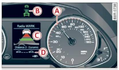
Fig. 119 Instrument cluster: adaptive cruise control
