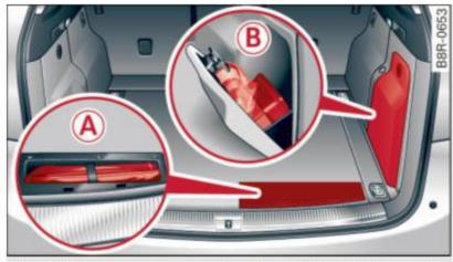
Fig. 113 Luggage compartment: vehicle tool bag and tire repair set
