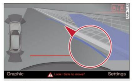
Fig. 148 MMI display: Blue curve on the curb
