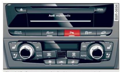
Fig. 143 Center console: Parking system switch
