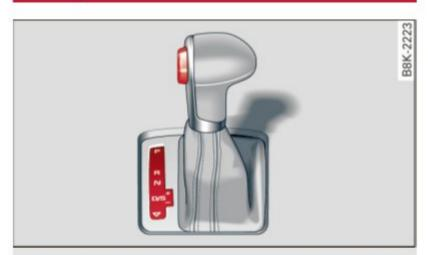
**Fig. 134** Shift gate on the center console: selector lever with release button
