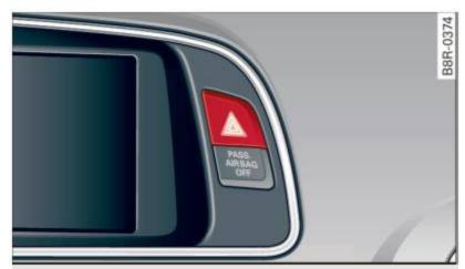
Fig. 47 Emergency flasher switch
