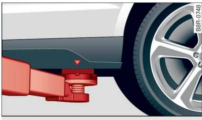
Fig. 235 Rear lifting point
