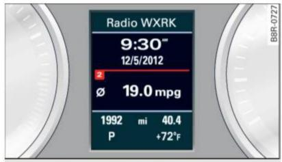
Fig. 9 Instrument cluster: center display
