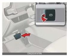
Releasing the parking brake with EPB switch.
