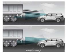
If the vehicle in front of you has cargo that extends rearward from the cab, or when the vehicle in front of you has higher ground clearance, additional special attention is required. Forward Collision-Avoidance Assist may not be able to detect the cargo extending from the vehicle. In these instances, you must maintain a safe braking distance from the rearmost object, and if necessary, steer your vehicle and depress the brake pedal to reduce your driving speed in order to maintain distance.
