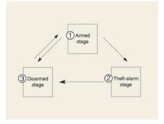
If triggered, the system provides an audible alarm with blinking of the hazard warning lights.
