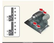
Depress the brake pedal and the unlock button when shifting.
