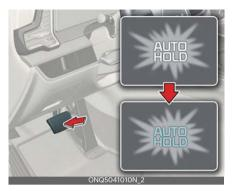
When coming to a complete stop by pressing the brake pedal, the AUTO HOLD indicator changes from white to green indicating the AUTO HOLD is engaged. The vehicle will remain at a standstill even if you release the brake pedal.
