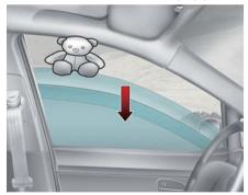
If the upward movement of the window is blocked by an object or part of the body, the window will detect the resistance and will stop upward movement. The window will then lower approximately 11.8 inches (30 cm) to allow the object to be cleared.
