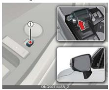
The position of the outside rear view mirror switch (1) determines whether or not the mirrors will move:
