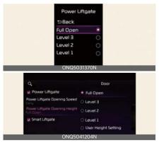
The liftgate opening height can be adjusted within the instrument cluster settings or the infotainment system.
