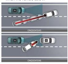
[A]: Your vehicle, [B]: Front vehicle If a vehicle cuts in front of your vehicle, Leading Departure Alert may not operate properly.
