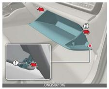
2. With the glove box open, pull the support strap.
