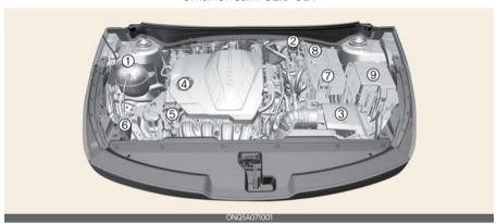
\* The actual engine room in the vehicle may differ from the illustration. 1. Engine coolant reservoir 7-16 2. Brake fluid reservoir 7-19 3. Air cleaner 7-12 4. Engine oil filler cap 7-14 5. Engine oil dipstick 7-14 6. Windshield washer fluid reservoir 7-20 7. Positive battery terminal 6-5, 7-24 6-5, 7-24 8. Negative battery terminal
