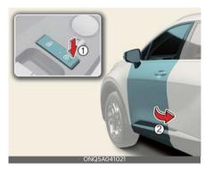
If you lock the door with the central door lock button (1), all vehicle doors will lock automatically.
