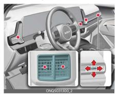
You can adjust the direction of air delivery from these vents using the vent control lever as shown.
