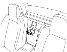
To open the fuel-filler lid, pull on the remote fuel-filler lid release.
