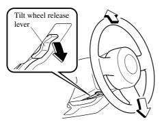
After adjusting, push the wheel up and down to be certain it's locked before driving.
