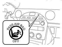
If the passenger weight sensors are normal, the indicator light illuminates when the ignition switch is turned to the ON position. After about 6 seconds it goes out.
