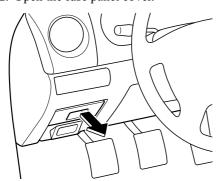
3. Pull the fuse straight out with the fuse puller provided on the fuse panel.
