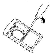
4. Put in the new battery (CR1620 or equivalent) with the positive pole (+) facing down.
