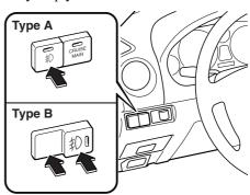
To turn on the fog lights, first turn the headlight switch to the ﷺ position. Then press the fog light switch. To turn the fog lights off:
