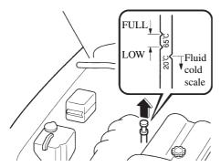
The proper fluid level is marked on the dipstick as follows.
