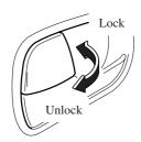
To lock any door with the door-lock knob from the outside, push the door-lock knob to the lock position and close the door. This does not operate the other door locks.
