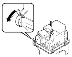
3. Lift off the air filter cover and remove the filter.
