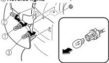
4. Install the new bulb in the reverse order of removal.
