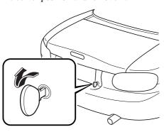
To activate the remote release, insert the key, turn it clockwise and open the trunk lid at the same time.
