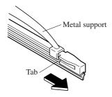
Remove the metal stiffeners from the blade rubber and install them in new blades.
