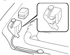
If it's at or near LOW, add enough coolant to the coolant reservoir to provide freezing and corrosion protection and to bring the level to FULL.
