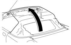
After securely hooking the top latches onto the windshield header, push each latch up with the palm of your hand until the lock buttons click and the latches are locked.
