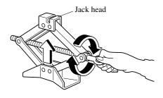
4. Place the jack under the jack-up position closest to the tire being changed with the jack head squarely under the jack-up point.
