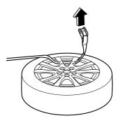
11. Thread the belt through the buckle, then pull the belt end to secure the flat tire.
