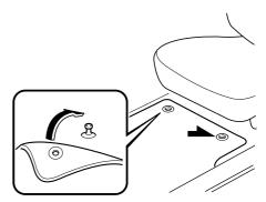
When setting a floor mat, position the floor mat so that its grommets are inserted over the pointed end of the retention posts.
