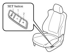
The driving position can be programmed or operated using the buttons on the side of the seat or the key.
