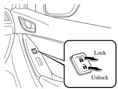
To lock all the doors from an open front door, press the lock side of the door lock switch and then close the door.
