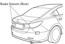
The radar sensors (rear) are installed inside the rear bumper, one each on the left and right sides.
