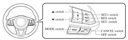
When the MODE switch is pressed, the Mazda Radar Cruise Control (MRCC) main indication (white) turns on and the vehicle speed and the distance between vehicles while in headway control can be set.
