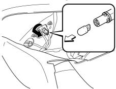
8. Install the new bulb in the reverse order of the removal procedure.
