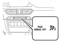
If the front passenger occupant classification sensor is normal, the indicator light turns on when the ignition is switched ON. The light turns off after a few seconds. Then, the indicator light turns on or is off under the following conditions:
