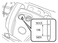
5. Pull it out again and examine the level. The level is normal if it is between the MIN and MAX marks. If it is near or below MIN, add enough oil to bring the level to MAX.
