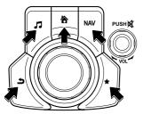
The following operations can be done by pressing the switches around the commander knob.
