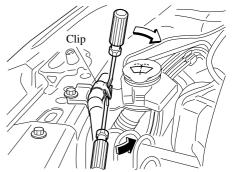
4. Remove the windshield washer fluid reservoir and bolts
