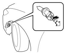
Turn the socket and bulb assembly to remove it. Carefully remove the bulb from its socket in the reflector by gently pulling it straight out of the socket
