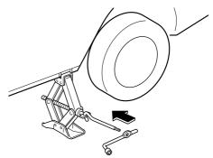
7. Turn the jack handle clockwise and raise the vehicle high enough so that the spare tire can be installed. Before removing the lug nuts, make sure your Mazda is firmly in position and that it cannot slip or move.
