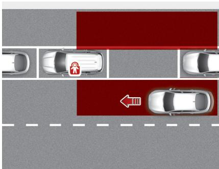
After the vehicle stops, when an approaching vehicle from the rear area is detected as soon as a passenger opens a door, Safe Exit Assist will warn the driver with a warning message and an audible warning to help prevent a collision.
