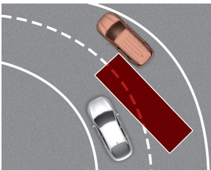
Blind-Spot Collision-Avoidance Assist may not operate properly when driving on a curved road. The function may not detect the vehicle in the next lane. Always pay attention to road and driving conditions while driving.
