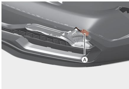
5. Remove the socket (A) from the assembly by turning the socket counterclockwise until the tabs on the socket align with the slots on the assembly.
