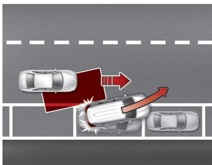
When you are driving forward out of a parking space, if Blind-Spot Collision-Avoidance Assist judges that there is a collision risk with an approaching vehicle in the blind spot,
