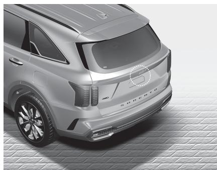
The rear view camera is used as a detecting sensor to detect pedestrians. If the camera lens is covered with foreign material, such as snow or rain, it may adversely affect camera performance and Reverse Parking Collision-Avoidance Assist may not operate normally. Always keep the camera lens clean.
