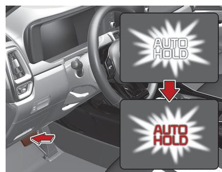
When coming to a complete stop by pressing the brake pedal, the AUTO HOLD indicator changes from white to green indicating the AUTO HOLD
