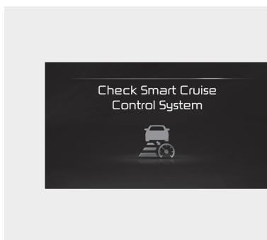
When Smart Cruise Control is not working properly, the 'Check Smart Cruise Control system' warning message will appear, and the (⚠) warning light will illuminate on the cluster. Have the function inspected by an authorized Kia dealer.
