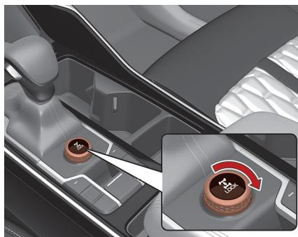
You can switch from DRIVE MODE to SNOW mode by turning the knob. If you turn the DRIVE/SNOW mode button again, the vehicle will go back to DRIVE MODE.
