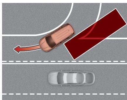
Blind-Spot Collision-Avoidance Assist may not operate properly when driving where the road merges or divides. The function may not detect the vehicle in the next lane. Always pay attention to road and driving conditions while driving.
