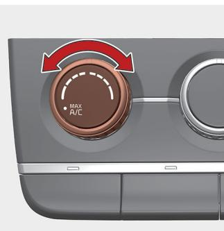
To change the air temperature in the passenger compartment, turn the knob to the right for warm and hot air or to the left for cooler air.
