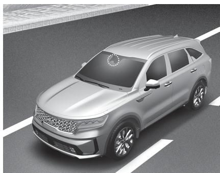
The front view camera is used as a detecting sensor to detect driving patterns and front vehicle departure while vehicle is being driven.
