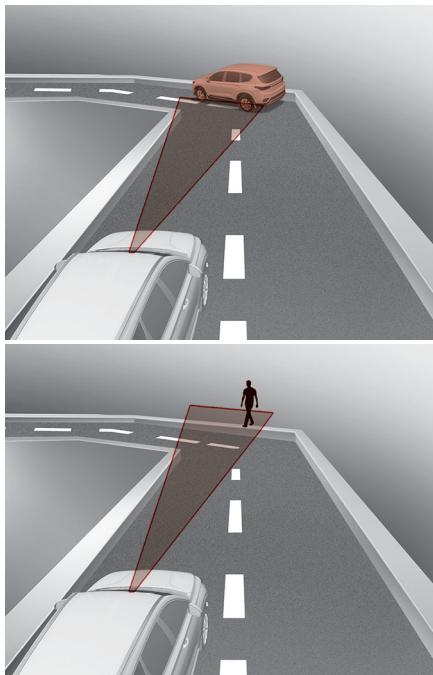
Forward Collision-Avoidance Assist may detect a vehicle, pedestrian in the next lane or outside the lane when driving on a curved road.
