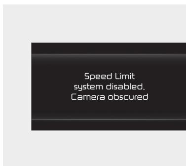
When the front windshield where the front view camera is located is covered with foreign material, such
