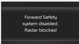
When the front windshield where the front view camera is located, front radar cover, sensor is covered with foreign material, such as snow or rain, it can reduce the detecting performance and temporarily limit or disable Forward Collision-Avoidance Assist.
