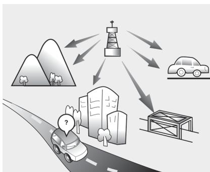
FM broadcasts are transmitted at high frequencies and do not bend to follow the earth's surface. Because of this, FM broadcasts generally
