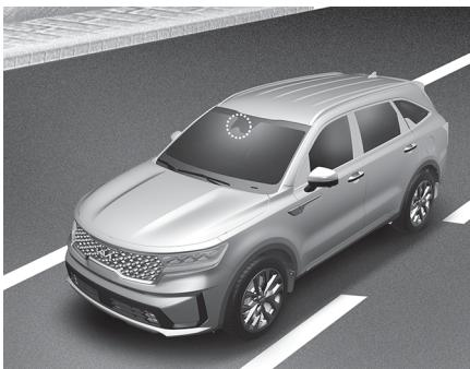
The front view camera is used as a detecting sensor to detect ambient light and brightness while driving.
