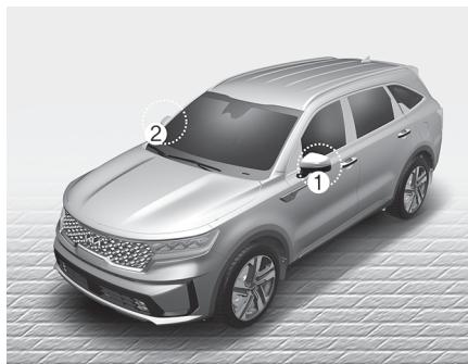
(camera located at bottom of the mirror)
