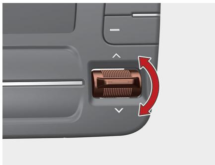
The temperature will increase to the maximum (HI) by moving the switch upwards.
