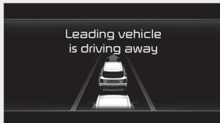
When the front vehicle departs from a stop, Leading Vehicle Departure Alert will inform the driver by displaying the 'Leading vehicle is driving away' message on the cluster and an audible warning will sound.
