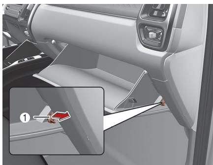
3. Remove the climate control air filter cover by pulling out both sides of the cover.
