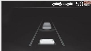
If temporary deceleration is required in the standby state and Navigation-based Smart Cruise Control is operating, the green (AUTO) symbol will illuminate on the cluster.
