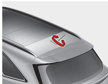
1. Shark fin antenna (Type A, if equipped)
