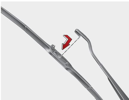
4. Make sure that both blade assemblies are installed firmly by trying to pull it slightly.
