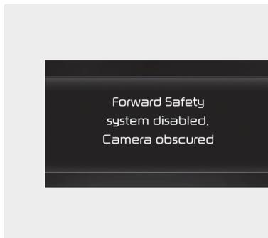
When the front windshield where the front view camera is located, is covered with foreign material, such as snow or rain, it can reduce the detecting performance and temporarily limit or disable Forward Collision-Avoidance Assist.
