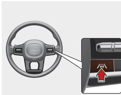
With the ENGINE START/STOP button in the ON position, shortly press the Lane Driving Assist button located on the steering wheel to turn on Lane Following Assist. The white or green (Ⓐ) indicator light will illuminate on the cluster.
