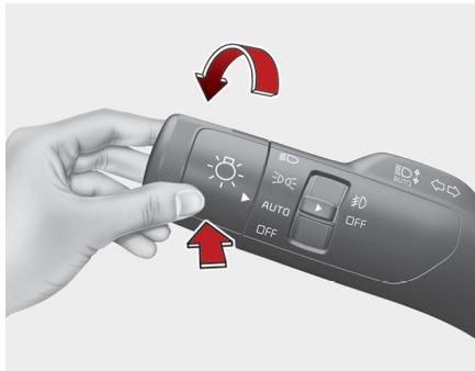
High Beam Assist is a function that automatically adjusts the headlamp range (switches between high beam and low beam) depending on the brightness of detected vehicles and certain road conditions.
