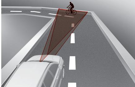
Forward Collision-Avoidance Assist may detect a vehicle, pedestrian or cyclist in the next lane or outside the lane when driving on a curved road. If this occurs, the function may unnecessarily warn the driver and control the brake. Always check
