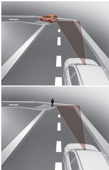
Forward Collision-Avoidance Assist may not detect other vehicles, pedestrians in front of you on curved roads adversely affecting the performance of the sensors. This may result in no warning, braking assist or steering assist when necessary.
