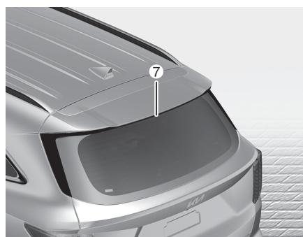
If the high mounted stop lamp (LED) (1) does not operate, have your vehicle checked by an authorized Kia dealer.
