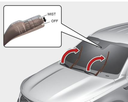
For your convenience and to prevent hood paint damage, you must move the windshield wiper blades to the service position as follows.
