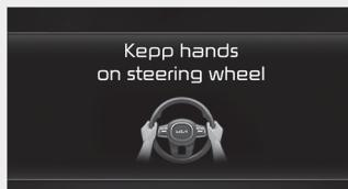
If the driver takes their hands off the steering wheel for several seconds, the 'Keep hands on the steering wheel' warning message will appear and an audible warning will sound in stages.
