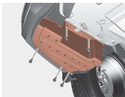
3. Loosen the plastic retaining screws and remove the under panel cover.
