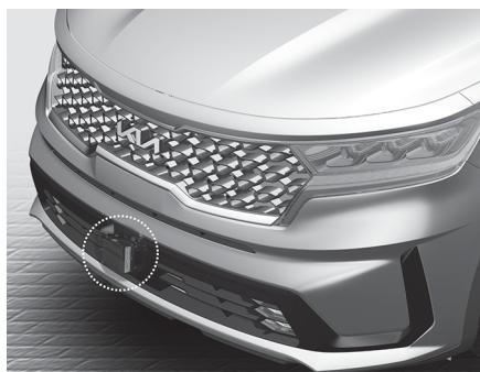
The front view camera and front radar are used as a detecting sensor to detect front vehicles.
