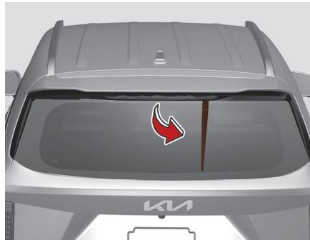
1. Within 20 seconds after the vehicle ignition is OFF, move the wiper lever to MIST position for over 2 seconds until the wiper moves down to the bottom middle part.
