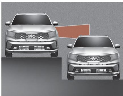
Blind-Spot Collision-Avoidance Assist may not operate properly when driving where the heights of the lanes are different. The function may not detect the vehicle on a road with different lane heights
