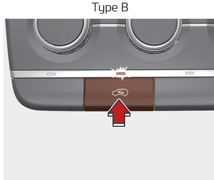
To change the air intake control position. Push the control button.
