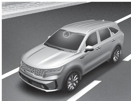
The front view camera is used as a detecting sensor to detect lane markings (or road edges).
