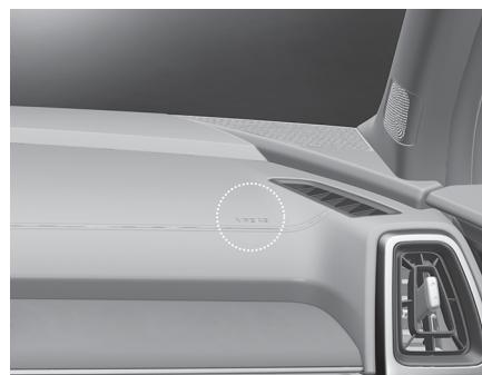
The indication of the function's presence are the letters "AIR BAG" located on the air bag pad cover on
