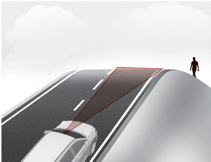
Forward Collision-Avoidance Assist may not detect other vehicles, pedestrians in front of you while driving uphill or downhill adversely affecting the performance of the sensors. This may result in unnecessary warning, braking assist or steering assist or no warning, braking assist or steering assist when necessary.
