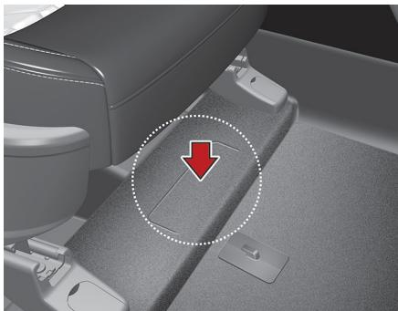
The number is punched on the floor under the front right side seat. To check the number, open the cover.
