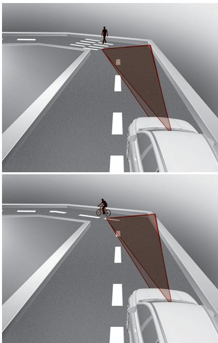
Forward Collision-Avoidance Assist may not detect other vehicles, pedestrians or cyclists in front of you on curved roads adversely affecting the performance of the sensors. This may result in no warning, and braking assist when necessary. When driving on a curve, you must maintain a safe braking distance, and if necessary, steer the vehicle and depress the brake pedal to reduce your driving speed in order to maintain a safe distance.
