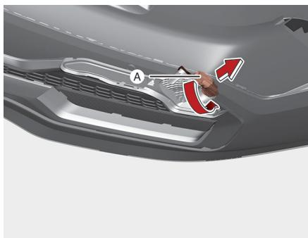
6. Remove the bulb from the socket by pressing it in and rotating it counterclockwise until the tabs on the bulb align with the slots in the socket. Pull the bulb out of the socket.
