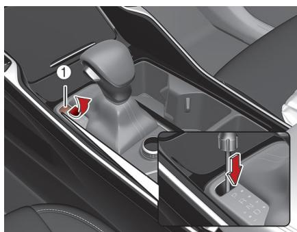
If the shift lever cannot be moved from the P (Park) position into R (Reverse) position with the brake pedal depressed, continue depressing the brake, then do the following:
