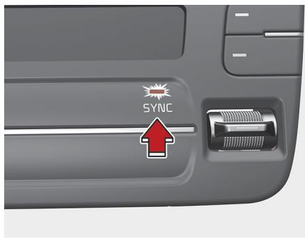
1. Press the "SYNC" button to adjust the driver and passenger side temperature equally.
