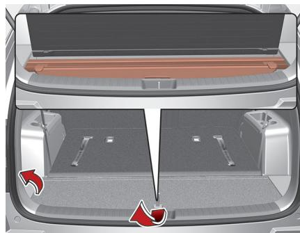
2. Push the guide pin in the direction as shown in the picture below.
