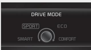
SPORT mode manages the driving dynamics by automatically adjusting the steering effort, the engine and transmission control logic for enhanced driver performance.
