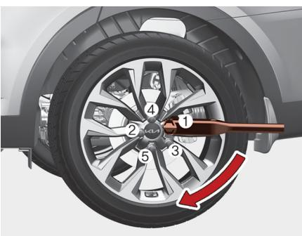
Then position the wrench as shown in the drawing and tighten the wheel nuts. Be sure the socket is seated completely over the nut. Do not stand on the wrench handle or use an extension pipe over the wrench handle. Go around the wheel tightening every other nut until they are all tight. Then double-check each nut for tightness. After changing wheels, have the system checked by a professional workshop. Kia recommends to visit an authorized Kia dealer.
