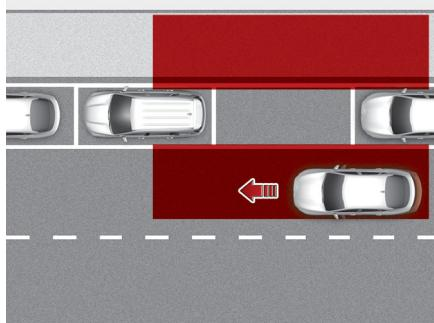
After the vehicle stops, when an approaching vehicle from the rear area is detected as soon as a passenger opens a door, Safe Exit Warning will warn the driver with a warning message and an audible warning to help prevent a collision.
