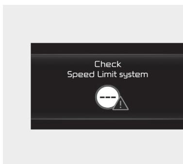
When Intelligent Speed Limit Assist is not working properly, the warning message will appear on the cluster for several seconds. If this occurs, have the function checked by an authorized Kia dealer.
