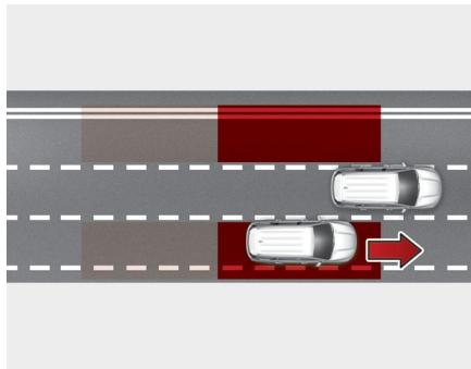
Blind-Spot Collision-Avoidance Assist will help detect and inform the driver that a vehicle is in the blind spot.
