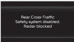
When the rear bumper around the rear corner radar or rear sensor is covered with foreign material, such as snow or rain, or installing a trailer or carrier, it can reduce the detect-
