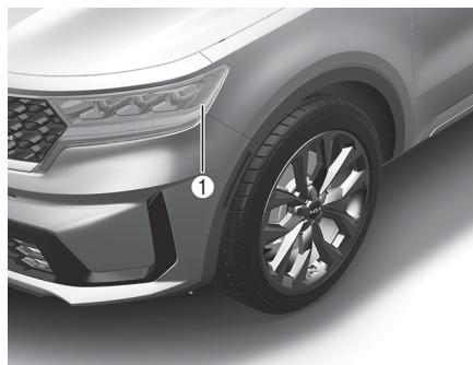
If the front side marker lamp LED (1) does not operate, have the vehicle checked by an authorized Kia dealer.
