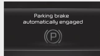
When the conversion from Auto Hold to EPB is not working properly a warning will sound and a message will appear.
