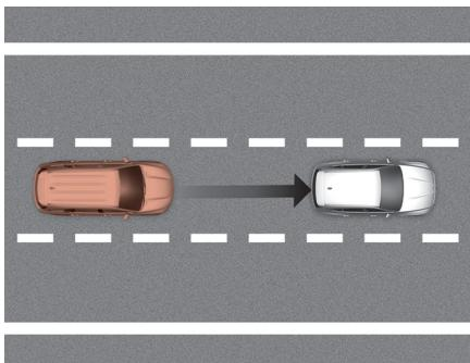
Highway Driving Assist is designed to help detect vehicles and lanes ahead, and help maintain distance from the vehicle ahead, maintain the set speed, and keep the vehicle between lanes while driving on the highway (or motorway).
