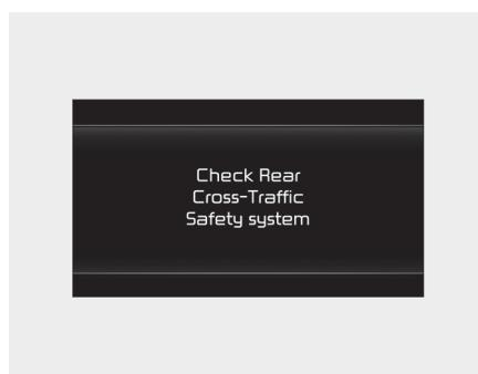
When Rear Cross-Traffic Collision-Avoidance Assist is not working properly, the 'Check Rear Cross-Traffic Safety system' warning message will appear on the cluster, and the function will turn off automatically or the function will be lim-
