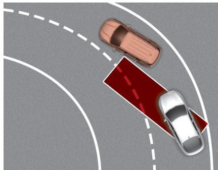
Blind-Spot Collision-Avoidance Assist may not operate properly when driving on a curved road. The function may recognize a vehicle in the same lane. Always pay attention to road and driving conditions while driving.
