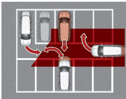
Rear Cross-Traffic Collision-Avoidance Assist may detect vehicles which are parking or pulling out near your vehicle (for example: a vehicle leaving beside your vehicle, a vehicle parking or pulling out in the rear area, a vehicle approaching your vehicle making a turn, etc.). If this occurs, the function may unnecessarily warn the driver and control the brake. Always check your surroundings while backing up.
