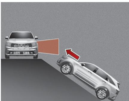
Rear Cross-Traffic Collision-Avoidance Assist may be limited when the vehicle is on a uphill or downhill slope, or near it, and may not detect the vehicle approaching from the left or right. If this occurs, the function may not warn the driver or control the brakes when necessary. Always check your surroundings while backing up.
