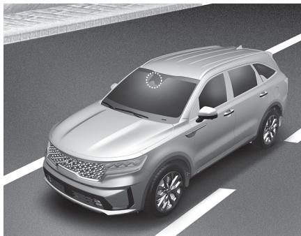
The front view camera is used as a detecting sensor to detect lane markings and front vehicles.
