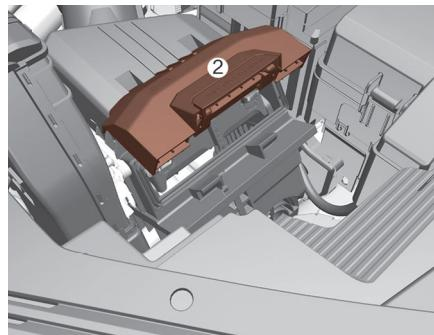
3. Rotate the fixed lever on the filter and loosen the lock.
