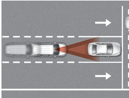
Forward Collision-Avoidance Assist is designed to help detect and monitor the vehicle ahead or help detect a pedestrian or cyclist in the roadway and warn the driver that a collision is imminent with a warning message and an audible warning, and if necessary, apply emergency braking.
