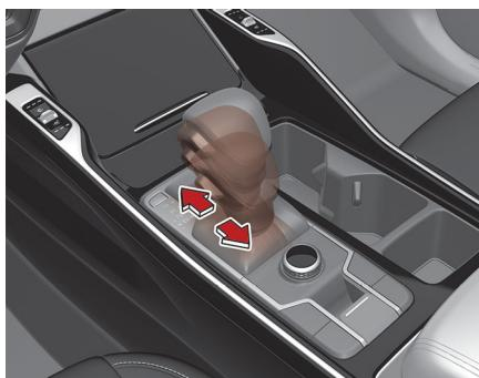
Whether the vehicle is stationary or in motion, manual mode is selected by pushing the shift lever from the D (Drive) position into the manual gate. To return to D (Drive) range operation, push the shift lever back into the main gate.
