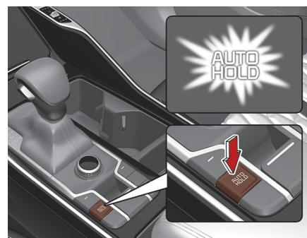
Before the Auto Hold will engage, the driver's door and engine hood must be closed.
