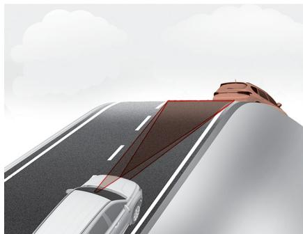
During uphill or downhill driving, the Smart Cruise Control may not detect a moving vehicle in your lane, and cause your vehicle to accelerate to the set speed. Also, vehicle speed will rapidly decrease when the vehicle ahead is detected suddenly.
