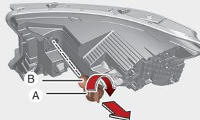
3. Remove the bulb (B) from the socket (A) by pressing it in and rotating it counterclockwise until the tabs on the bulb align with the slots in the socket. Pull the bulb out of the socket.
