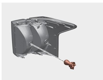
8. Remove the bulb from the socket by pressing it in and rotating it counterclockwise until the tabs on the bulb align with the slots in the socket. Pull the bulb out of the socket.
