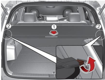
1. Pull the cargo security screen towards the rear of the vehicle by the handle (1).
