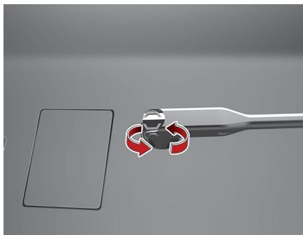
4. Use the wheel lug nut wrench to loosen the bolt enough to lower the spare tire.
