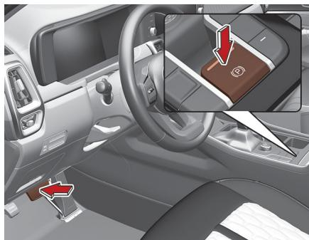
Releasing the parking brake with EPB switch,
