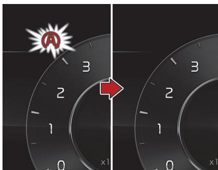
The engine will start and the green AUTO STOP indicator (A) on the instrument cluster will go out.
