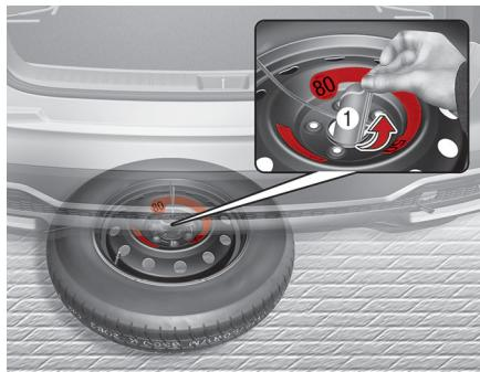
5. After the spare tire reaches the ground, continue to turn the wrench counterclockwise, and draw the spare tire outside. Never rotate the wrench excessively, otherwise the spare tire carrier may be damaged.
