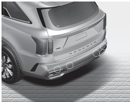
The rear ultrasonic sensors are located inside the rear bumper to detect objects in the rear area. If the sensors are covered with foreign material, such as snow or rain, it may adversely affect sensor performance and Reverse Parking Collision-Avoidance Assist may not operate normally. Always keep the rear bumper clean.
