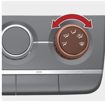
Air can be directed to the floor, dashboard outlets, or windshield. Five symbols are used to represent Face, Bi-Level, Floor, Floor-Defrost and Defrost air position.
