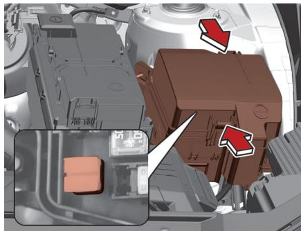
4. Check the removed fuse; replace it if it is blown.
