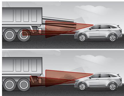
If the vehicle in front of you has cargo that extends rearward from the cab, or when the vehicle in front of you has higher ground clearance, additional special attention is required. Forward Collision-Avoidance Assist may not be able to detect the cargo extending from the vehicle. In these instances, you must maintain a safe braking distance from the rearmost object, and if necessary, steer your vehicle and depress the brake pedal to reduce your driving speed in order to maintain distance.
