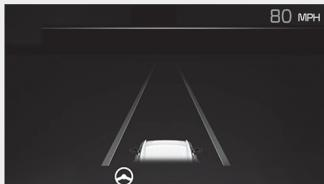
If the vehicle ahead and/or both lane markings are detected and your vehicle speed is above 60 km/h (40 mph) and below 200 km/h (120 mph), the green (Ⓐ) indicator light will illuminate on the cluster, and the function will help the vehicle stay in lane by assisting the steering wheel.
