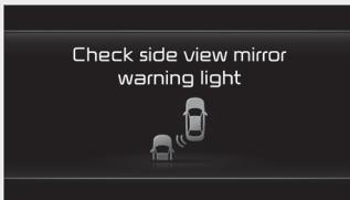
When the side view mirror warning light is not working properly, the 'Check side view mirror warning light' warning message will appear on the cluster. Have the function inspected by an authorized Kia dealer.
