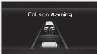
While Smart Cruise Control is operating, when the collision risk with the vehicle ahead is high, the 'Collision Warning' warning message will appear on the cluster, and an audible warning will sound to warn the driver. Always have your eyes on the road while driving, and if necessary, depress the brake pedal to reduce your driving speed in order to maintain a safe distance.
