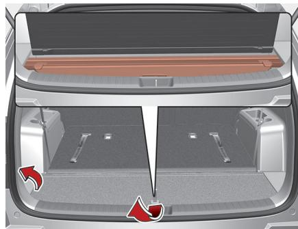
3. While pushing the guide pin, pull out the cargo security screen.
