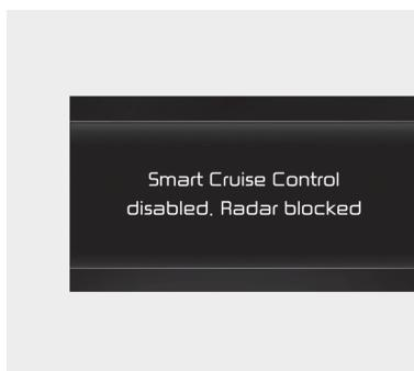
When the front radar cover or sensor is covered with snow, rain, or foreign material, it can reduce the detecting performance and temporarily limit or disable Smart Cruise Control.
