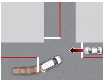
Junction Turning function will help avoid a collision with an oncoming vehicle in an adjacent lane when turning left at a crossroad with the turn signal on by applying emergency braking.
