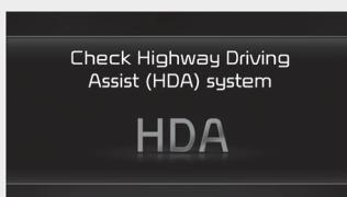
When Highway Driving Assist is not working properly, the 'Check Highway Driving Assist (HDA) system' warning message will appear, and the (⚠) warning light will illuminate on the cluster. Have the function inspected by an authorized Kia dealer.
