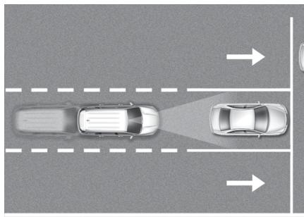
Forward Collision-Avoidance Assist is designed to help detect and monitor the vehicle ahead or help detect a pedestrian in the roadway and warn the driver that a collision is imminent with a warning message and an audible warning, and if necessary, apply emergency braking.
