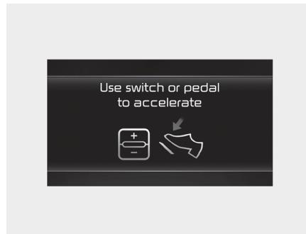
When Highway Driving Assist is operating, your vehicle will stop if the vehicle ahead of you stops. Also, if the vehicle ahead of you starts moving approximately within 30 seconds after the stop, your vehicle will start as well. In addition, after the vehicle has stopped and approximately 30 seconds have passed, the 'Use switch or pedal to accelerate' message will appear on the cluster. Depress the accelerator pedal or push the + switch, - switch or (II) switch to start driving.
