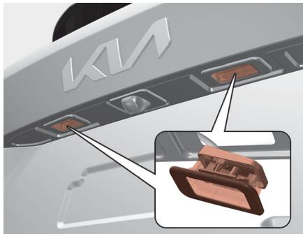
If the license plate lamp does not operate, have your vehicle checked by an authorized Kia dealer. The LED lamp cannot be replaced as a single unit because it is an integrated unit. The LED lamp has to be replaced with the unit. A skilled technician should check or repair the map lamp (LED), for it may damage related parts of the vehicle.
