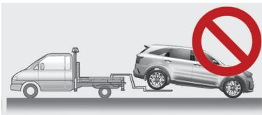
The AWD vehicle should never be towed with the wheels on the ground. Your vehicle must be towed with a wheel lift and dollies or flatbed equipment with all the wheels off the ground.
