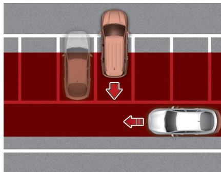
Rear Cross-Traffic Collision-Avoidance Assist may detect vehicles passing by behind you when parking backwards into a parking space. If this occurs, the function may unnecessarily warn the driver and control the brake. Always check your surroundings while backing up.
