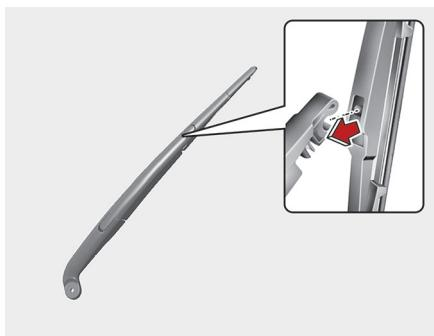
5. Make sure the blade assembly is installed firmly by trying to pull it slightly.
