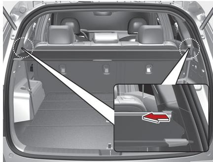
2. While pushing the guide pin, pull out the cargo security screen.
