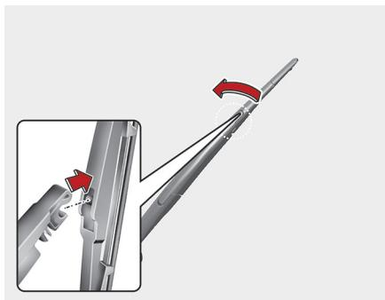
4. Install the new blade assembly by inserting the center part into the slot in the wiper arm until it clicks into place.
