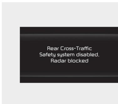
When the rear bumper around the rear corner radar or sensor is covered with foreign material, such as snow or rain, or installing a trailer or carrier, it can reduce the detecting performance and temporarily limit or disable Blind-Spot Collision-Avoidance Assist.
