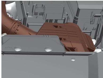
You can clean the filter when inspecting the air cleaner compartment. Clean the filter by using compressed air.
