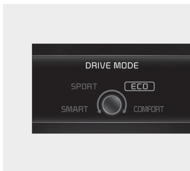
When the Drive Mode is set to ECO mode, the engine and transmission control logic are changed to maximize fuel efficiency.
