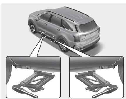
8. Insert the jack handle into the jack and turn it clockwise, raising the vehicle until the tire just clears the ground. This measurement is approximately 1.2 inches (30 mm). Before removing the wheel lug nuts, make sure the vehicle is stable and that there is no chance for movement or slippage.
