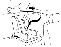
4. Push the child-restraint system firmly into the vehicle seat. Be sure the belt retracts as snugly as possible. A clicking noise from the retractor will be heard during retraction if the system is in the automatic locking mode. If the belt does not lock the seat down tight, repeat this step.
