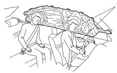
The side and curtain air bags will deploy only on the side the vehicle receives the force of the impact.
