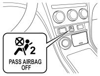
If the front passenger weight sensors are normal, the indicator light illuminates when the ignition switch is turned to the ON position. For a specified of time it goes out.
