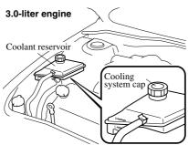
If you find no problems, the engine is cool, and no leaks are obvious, carefully add coolant as required (page 8-13).
