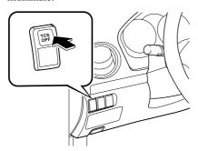
Press the switch again to turn the TCS back on. The TCS OFF indicator light will go out.
