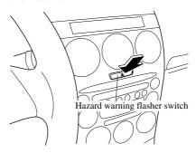
Depress the hazard warning switch and all four turn signals will flash at once.
