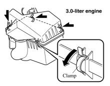
2. Tilt or lift the air filter cover and remove the filter.
