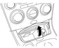
2. Press the lighter in and release it. When ready for use, it automatically pops out.
