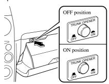
With the switch in the ON position, the remote trunk lid release can be operated.
