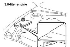
If it's at or near LOW or L, add enough coolant to the coolant reservoir to provide freezing and corrosion protection and to bring the level to FULL or F.
