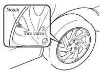
Damage could occur during installation if the wheel cover is not properly aligned.
