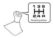
The shift pattern of the transaxle is conventional, as shown.
