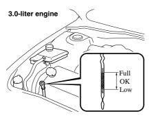
Pull it out again and examine the level. It's OK between MIN and MAX. But if it's near or below MIN, add enough oil to bring the level to MAX.
