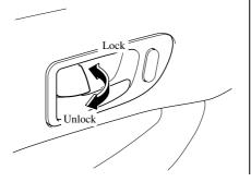
To lock any door with the door-lock button from the outside, push its doorlock button and close the door. This does not operate the other door lock.
