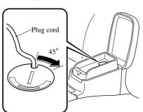
7. Set the plug cord into the slit of the tray mat and replace the tray mat.
