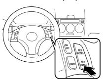
Your vehicle has a tap-down feature that allows you to decrease your current speed in decrements of 1.6 km/h (1 mph) by a momentary tap of the SET/COAST button. Multiple taps will decrease your vehicle speed 1.6 km/h (1 mph) for each tap.
