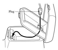
6. Make sure the plug cord is running through the cap slot; reinstall the cap and turn it clockwise (about 45° to the opened position).
