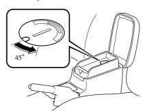
4. Open the tray by pulling the lower release catch.
