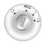
The ignition switch has four different positions.
