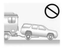
Notice: Towing the vehicle from the rear could damage it. Also, repairs would not be covered by the vehicle warranty. Never have the vehicle towed from the rear.
