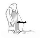
On vehicles with this feature, the handle is located on the inboard side of the seatback.
