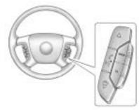
△ *I* ▽: Press to change favorite radio stations, select tracks on a CD/DVD, or to navigate tracks or folders on an iPod® or USB device.
