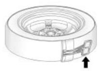
Remove the plastic spare tire heat shield by pulling the rubber latch. Store the plastic spare tire heat shield. See "Storing a Flat or Spare Tire and Tools" later in this section for more information.
