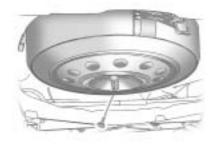
If the spare tire will not lower, the secondary latch could be engaged.
