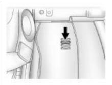
The interior temperature sensor located on the instrument panel to the right of the steering column, measures the temperature of the air inside the vehicle.
