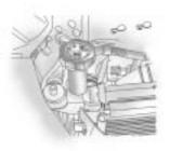
Start the engine and let it run until the upper radiator hose feels warm. Any time during this procedure, watch out for the engine cooling fan(s).  If the coolant level inside the radiator filler neck is low, add more of the proper DEX-COOL coolant mixture through the filler neck until the level is back up to the base of the filler neck. Replace the pressure cap. Be sure to secure it tightly.
