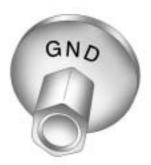
Connect the other end of the negative (-) cable at least 18 inches (45 cm) away from the dead battery, but not near engine parts that move.
