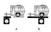
If a weight-carrying hitch or a weight-distributing hitch is being used, the trailer tongue (A) should weigh 10-15 percent of the total loaded trailer weight (B).
