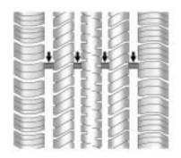
One way to tell when it is time for new tires is to check the treadwear indicators, which appear when the tires have only 1.6 mm (1/16 inch) or less of tread remaining.
