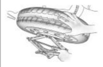
Disconnect the lug wrench from the jack and carefully remove the jack. Use one hand to push against the spare tire while firmly pulling the jack out from under the spare tire with the other hand.
