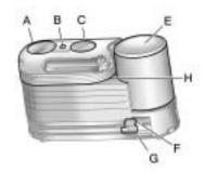
When using the tire sealant and compressor kit during cold temperatures, warm the kit in a heated environment for 5 minutes. This will help to inflate the tire faster.
