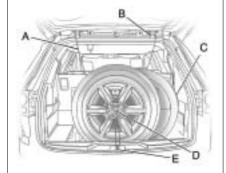
Pull the cable (A) through the door striker (E), the center of the wheel (D), and the plastic spare tire heat shield (C), as shown.
