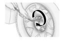
Loosen the wheel nuts — but do not remove them — using the lug wrench. For wheels with a wheel lock key, use the wheel lock key between the lock nut and lug wrench. The key is supplied in the front passenger door pocket.
