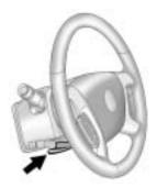
Pull the lever down to move the steering wheel up or down and in or out. Pull the lever up to lock the steering wheel in place.
