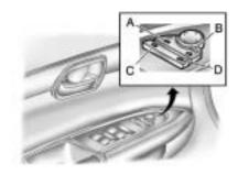
The controls for power foldaway mirrors are located on the driver door armrest.
