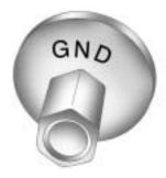
Connect the other end of the negative (-) cable at least 18 inches (45 cm) away from the dead battery, but not near engine parts that move.
