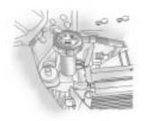
Start the engine and let it run until the upper radiator hose feels warm. Any time during this procedure, watch out for the engine cooling fan(s).  If the coolant level inside the radiator filler neck is low, add more of the proper DEX-COOL coolant mixture through the filler neck until the level is back up to the base of the filler neck. Replace the pressure cap. Be sure to secure it tightly.
