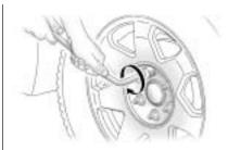
3. Loosen the wheel nuts — but do not remove them — using the lug wrench. For wheels with a wheel lock key, use the wheel lock key between the lock nut and lug wrench. The key is supplied in the front passenger door pocket.
