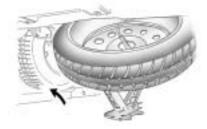
Lower the jack by turning the lug wrench counterclockwise.
