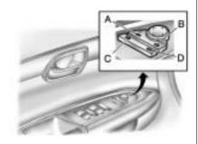
The vehicle may have outside power foldaway mirrors. The controls are located on the driver door armrest.
