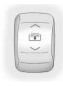
**Vent:** From the closed position, press and hold the front of the driver side switch to vent the sunroof. Press and hold the rear of the driver side switch to close the sunroof.
