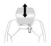
Pull the head restraint up to raise it. To lower the head restraint, press the release button, located on the head restraint post on the top of the seatback, while you push the head restraint down.
