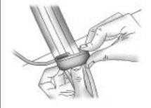
Place the guide over the belt and insert the two edges of the belt into the slots of the guide.
