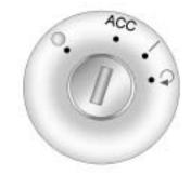
The ignition switch has four different positions.
