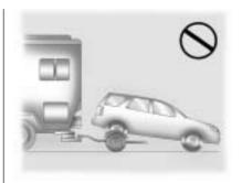
Notice: Towing the vehicle from the rear could damage it. Also, repairs would not be covered by the warranty. Never have the vehicle towed from the rear.
