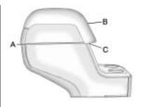
To access the upper storage area, press the upper button (B) and lift up. To access the lower storage area, press the lower button (C) and lift up. The top of the console can be folded forward for increased storage area. Lift up on handle on the rear of the console (A) and pull forward.
