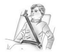
Buckle, position, and release the safety belt as described previously in this section. Make sure that the shoulder belt crosses the shoulder. To remove and store the comfort guide, squeeze the belt edges together so that the safety belt can be removed from the guide.
