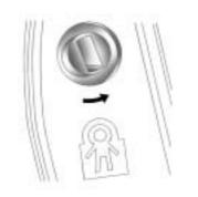
Open the rear doors to access the security locks on the inside edge of each door.
