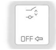
To change the liftgate to manual operation, press the switch on the center console to the OFF position.
