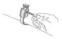
2. Disconnect the rear safety belt mini-latch, using a key in the slot on the mini-buckle, let the belt retract into the headliner. Stow the mini-latch in the holder located in the headliner.
