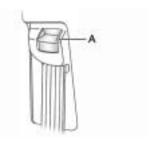
To move it down, push down on the button (A) and move the height adjuster to the desired position. You can move the height adjuster up by pushing up on the shoulder belt quide.
