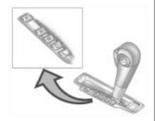
**P** (Park): This position locks the front wheels. It is the best position to use when starting the engine because the vehicle cannot move easily.
