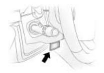
The adjustment lever is located on the left side of the steering column.
