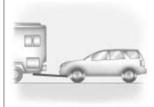
If the vehicle is front-wheel-drive, it can be dinghy towed from the front.
