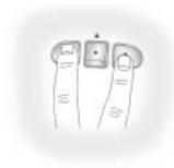
From inside the vehicle, press and hold down the two outside buttons at the same time, releasing only when the Universal Home Remote indicator light begins to flash, after 20 seconds. This step will erase the factory settings or all previously programmed buttons.
