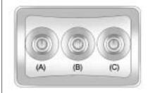
The A/V jacks, located on the rear of the floor console, allow audio or video signals to be connected from an auxiliary device such as a camcorder or a video game unit to the RSE system. Adapter connectors or cables (not supplied) might be required to connect the auxiliary device to the A/V jacks. Refer to the manufacturer's instructions for proper usage.
