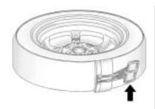
Remove the plastic spare tire heat shield by pulling the rubber latch. Store the plastic spare tire heat shield. See Storing a Flat or Spare Tire and Tools on page 5-78 for more information
