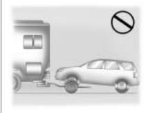
All-wheel-drive vehicles must not be towed with two wheels on the ground. To properly tow these vehicles, they should be placed on a platform trailer with all four wheels off of the ground or dinghy towed from the front.
