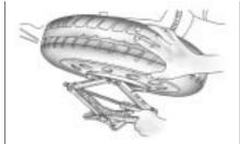
Disconnect the lug wrench from the jack and carefully remove the jack. Use one hand to push against the spare tire while firmly pulling the jack out from under the spare tire with the other hand.
