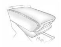
Pull up on the lever, located on the front of the center console armrest, to slide it forward and backward. To open the armrest storage area, press the button located on the front of the armrest. There is additional storage under the armrest, move the armrest all the way to the rear position, slide the cover back and remove the tray.
