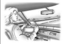
An emergency like this requires close attention and a quick decision. If holding the steering wheel at the recommended 9 and 3 o'clock positions, it can be turned a full 180 degrees very quickly without removing either hand.
