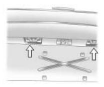
2. Turn and pull the license plate lamp forward through the lift gate trim opening.
