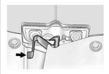
Go to the front of the vehicle to find the secondary hood release handle. The handle is under the front edge of the hood near the center. Push the handle to the right and at the same time raise the hood.
