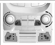
If available, the buttons are near the climate controls. To operate, the ignition must be in ON/RUN.
