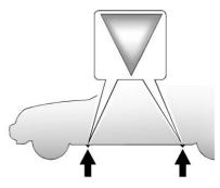
Position the jack lift head at the jack location nearest the flat tire. The location is indicated by a mark on the bottom edge of the front and rear door plastic molding. The jack must not be used in any other position. Place the jack notch under the frame rail seam.
