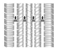
Treadwear indicators are one way to tell when it is time for new tires. Treadwear indicators appear when the tires have only 1.6 mm (1/16 in) or less of tread remaining. See *Tire Inspection* ⇒ 248 and *Tire Rotation* ⇒ 248.
