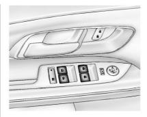
The power windows work when the ignition is in ON/RUN or ACC/ACCESSORY, or in Retained Accessory Power (RAP). See Retained Accessory Power (RAP) ⇒ 168.
