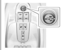
On vehicles with a power liftgate, the vehicle must be in P (Park) to use the power feature. The taillamps flash when the power liftgate moves.
