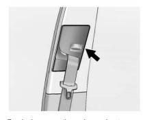
Push down on the release button and move the height adjuster to the desired position.
