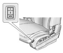
If available, the 1, 2, and MEM (Memory) buttons on the outboard side of the driver seat are used to manually store and recall the driver seat and outside mirror positions. These manually stored positions are referred to as Button Memory positions.
