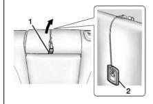
Stow the rear seat center armrest. Attach the retaining strap to the armrest loop (1) and to the center top tether anchor on the seatback (2). Make sure the retaining strap's clips are firmly attached.
