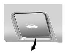
Pull the release handle located below the instrument panel to the left of the steering wheel.
