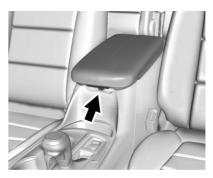
There is storage in the center console; lift the lever on the front to open.
