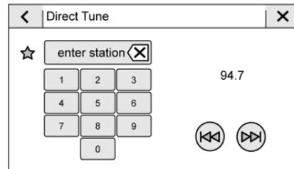
Access Direct Tune by touching the Tune icon on the infotainment display to bring up the keypad. Navigate through all frequencies using the arrows on the right side of the Direct Tune display. Directly enter a station or channel using the keypad. When a new station or channel is entered, the information about that station or channel displays on the right side. This information will update with each new valid frequency. Touch ☆ to save the station or channel as a favorite.
