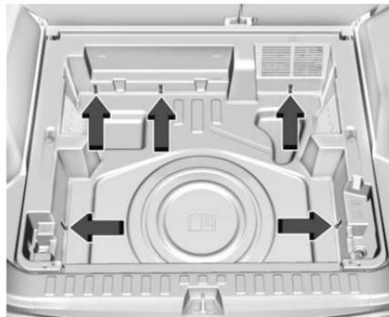
2. Reinstall the spare tire cover. To ensure proper engagement, press down firmly on the surface next to all five snap retainers.
