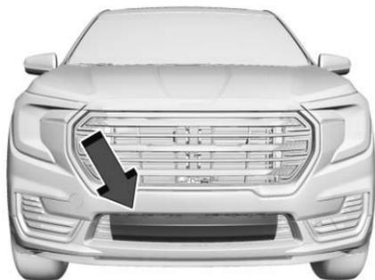
1. Center grille cover and make sure that it is positioned correctly.
