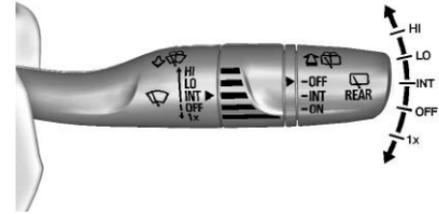
The windshield wiper/washer lever is on the side of the steering column. With the ignition on or in accessory mode, move the windshield wiper lever to select the wiper speed.
