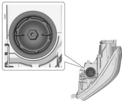
2. Remove the bulb access cap from the top of the headlamp assembly by turning it counterclockwise.
