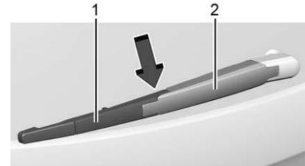
2. While holding the wiper arm, press down at the end of the wiper blade assembly (1) where it attaches to the wiper arm (2) to remove the wiper blade assembly from the wiper arm.
