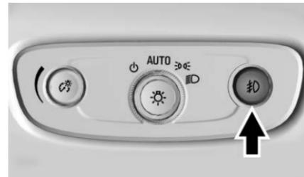
The ignition and parking lamps or headlamps must be on for the front fog lamps to work.
