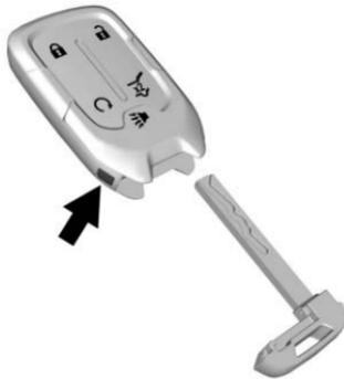
To remove the key, press the button near the bottom of the transmitter, and pull the key out. Never pull the key out without pressing the button.
