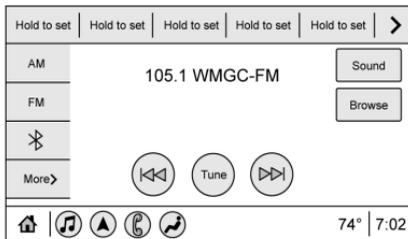
From the AM, FM, or SXM (if equipped) option, press ⇨ or ⇦ on the center stack to search for the previous or next strong station or channel.
