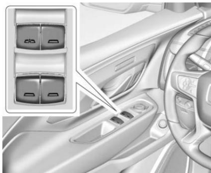
The power windows work when the ignition is on, in ACC/ACCESSORY, or in Retained Accessory Power (RAP). See *Retained Accessory Power (RAP)* ⇨ 215.
