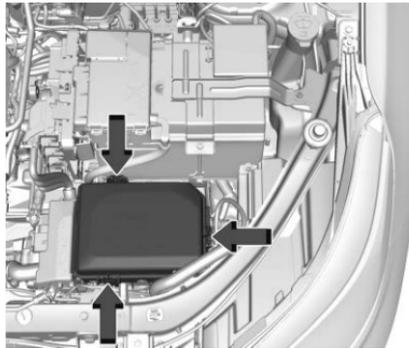
There are three clips on the side of the fuse block cover. See *Engine Compartment Overview* ⇨ 275.
