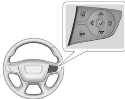
Press  $\triangleleft$  to access the cluster applications. Use  $\triangle$  or  $\nabla$  to scroll through the list of available applications.
