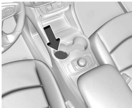
2. Place the two recognized transmitters in the cupholder.
