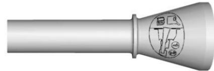
1. Locate the capless funnel adapter from under the spare tire.
