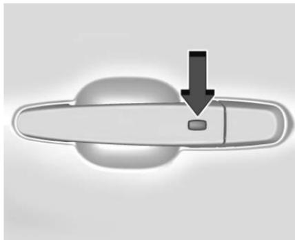
The RKE transmitter must be within 1 m (3 ft) of the liftgate or door being opened. Press the button on the door handle to open. See “Keyless Access Operation” in *Remote Keyless Entry (RKE) System Operation* ⇨ 7.
