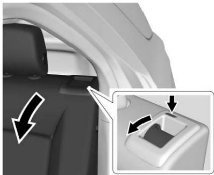
1. Pull the handle on top of the seatback to unlock it.
