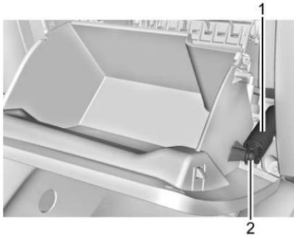
2. Disconnect the glove box door damper (1) from the glove box door assembly by squeezing the pivot (2) to release the damper ring.
