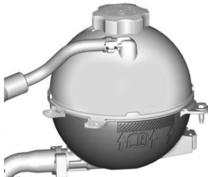
Check to see if coolant is visible in the coolant surge tank. If the coolant inside the coolant surge tank is boiling, do not do anything else until it cools down. If coolant is visible but the coolant level mark is not visible, add a 50/50 mixture of clean, drinkable water and DEX-COOL coolant at the coolant surge tank to the top rib on the middle of the tank, but be sure the cooling system is cool before this is done. See *Engine Overheating* ⇨ 284.
