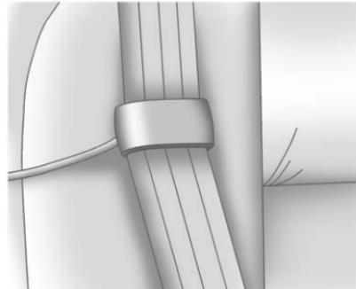
3. Be sure that the belt is not twisted and it lies flat. The elastic cord must be behind the belt with the plastic guide on the front.
