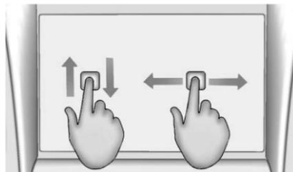
Drag is used to move applications on the Home Page, or to pan the map. To drag the item, it must be held and moved along the display to the new location. This can be
