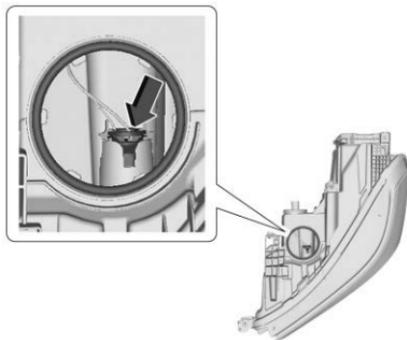
3. Remove the bulb from the bulb socket by pinching the tabs on either side of the bulb and pull straight out.
