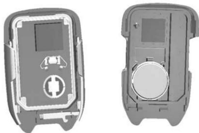
3. Lift the battery with a flat object.
