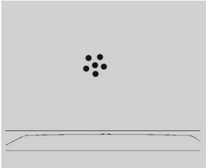
If Head-Up Display (HUD) is equipped and the screen is closed, when the vehicle approaches a pedestrian ahead too rapidly, the HUD with the integrated RLAD can display red spots reflected in the windshield.
