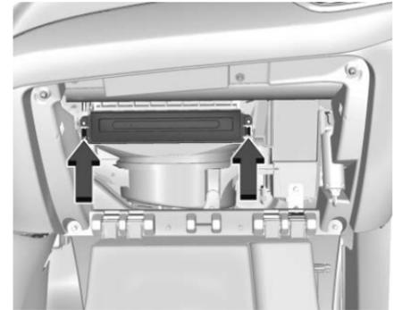
4. Remove the two screws securing the door.
