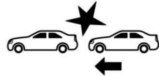
If Head-Up Display (HUD) is equipped and the screen is open, when your vehicle approaches another detected vehicle too rapidly, the HUD can display indicator on the screen as the FCA display.
