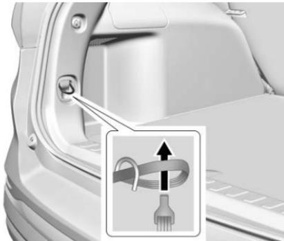
5. Route the loop end of the strap through one of the cargo tie-downs in the rear of the vehicle.
