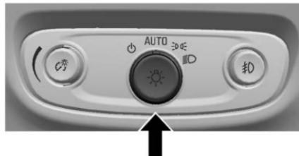
The exterior lamp control is on the instrument panel to the left of the steering column.
