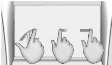
Fling or swipe is used to scroll through a list, pan the map, or change page views. Do this by placing a finger on the display then moving it rapidly up and down or right and left.
