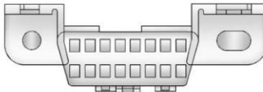
The DLC is under the instrument panel to the left of the steering wheel. Connecting devices that are not used to perform an Emissions Inspection/Maintenance test or to service the vehicle may affect vehicle
