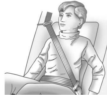
4. Buckle, position, and release the seat belt as described previously in this section. Make sure the shoulder belt crosses the shoulder. The belt should be close to, but not contacting, the neck.
