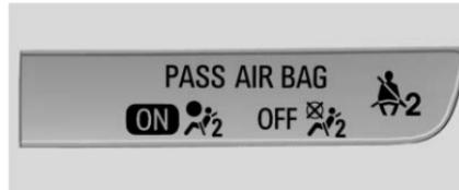
When the vehicle is started, the passenger airbag status indicator will light ON and OFF, and the symbols for on and off, for several seconds as a system check. Then, after several more seconds, the status indicator will light either ON or OFF, and either the on or off symbol, to let you know the status of the front outboard passenger frontal airbag.
