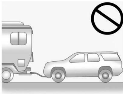
The vehicle was not designed to be towed with all four wheels on the ground. The vehicle may be towed using a platform trailer with all four wheels off the ground. Some vehicles may be dolly towed. See the following information on dolly towing.
