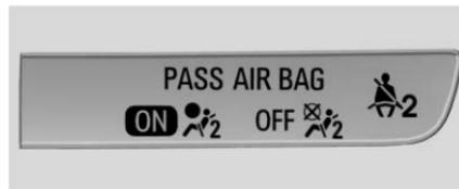
The words ON and OFF, and the symbols for on and off, will be visible during the system check. When the system check is complete, either the word ON or OFF, and the symbol for on or off, will be visible. See *Passenger Airbag Status Indicator* ⇨ 99.
