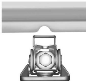
9. Position the jack lift head at the jack location nearest the flat tire. The location is indicated by a notch in the vertical bottom edge of the body side sheet metal.
