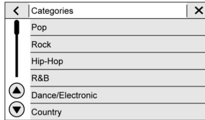
From the AM stations, if equipped with HD Radio, FM, or SXM (if equipped) display, touch Categories at the top of the Browse menu to access the categories list. The list contains names associated with the AM or FM stations, or SXM channels. Touch a category name to display a list of stations or channels for that category. Touching a station or channel from the list will tune the radio to that station or channel.
