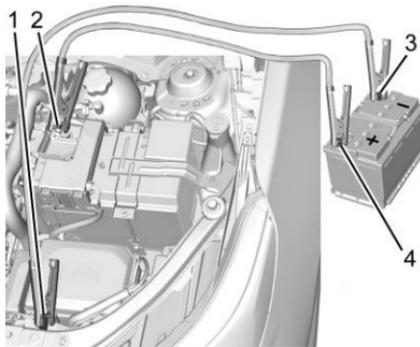
1. Discharged Battery Negative (-) Grounding Point
