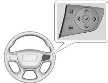
Press ◀ or ▶ to select VEHICLE menu, then use ▲ or ▼ to scroll through the menu items to select TCS/StabiliTrak/ESC.
