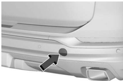
If equipped, carefully open the cover by using the small notch that conceals the rear tow eye socket.
