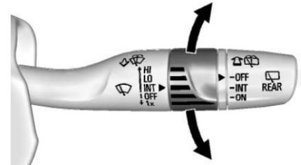
**INT** : Move the lever up to INT for intermittent wipes, then turn the band up for more frequent wipes or down for less frequent wipes.
