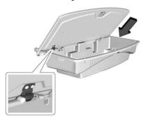
3. Angle the load floor approximately 70%, align the two hooks on the load floor above the rod, and push the load floor until the hooks engage the cargo bin rod.
