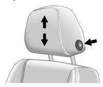
To raise or lower the head restraint, press the button located on the side of the head restraint, and pull up or push the head restraint down, and release the button. After releasing the button, ensure the head restraint locks in place and is unable to move up or down.
