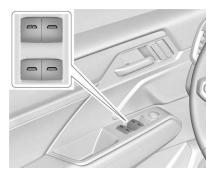
The power windows work when the vehicle is on, in accessory mode, or when Retained Accessory Power is active. See Retained Accessory Power (RAP) ⇒ 188.
