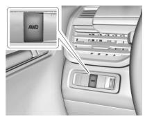
**All-Wheel Drive Mode:** All-Wheel Drive mode provides drive torque to all four wheels. Select All-Wheel Drive to improve traction and control on slippery road surfaces, such as gravel, sand, wet pavement, snow, and ice.
