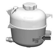
Check to see if coolant is visible in the coolant surge tank. If the coolant inside the coolant surge tank is boiling, do not do anything else until it cools down. If coolant is visible but the coolant level mark is not visible, add a 50/50 mixture of clean, drinkable water and DEX-COOL coolant at the coolant surge tank to the top rib on the middle of the tank, but be sure the cooling system is cool before this is done. See Engine Overheating ♀ 272.
