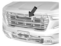
The vehicle may have a shutter system designed to help improve fuel economy. Keep the shutter system clear of debris, snow and ice. If the check engine light is activated, please check to see if the shutter system is clear of debris, snow or ice.
