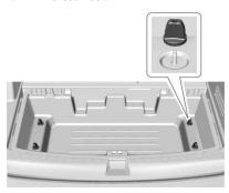
Remove the four wing nuts, then remove the cargo management system. See Cargo Management System \$ 87.
