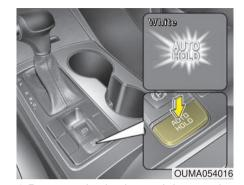
1.Depress the brake pedal, start the engine and then press the Auto Hold button. The white AUTO HOLD indicator will come on indicating the system is in standby. Before the Auto Hold will engage, the driver's door, engine hood and trunk must be closed and the driver's seat belt must be fastened.
