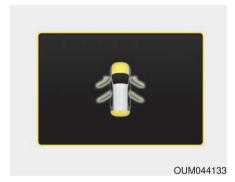
It means that any door, hood, or liftgate is open.
