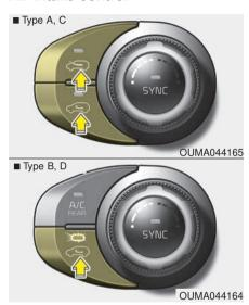
This is used to select the outside (fresh) air position or recirculated air position.
