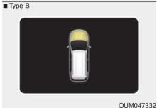
The warning message (for Type B cluster) will appear on the LCD display when hood is open.
