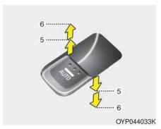
Pressing or pulling up the power window switch momentarily to the second detent position (6) completely lowers or raises the window even when the switch is released. To stop the window at the desired position while the window is in operation, pull up or press down and release the switch.
