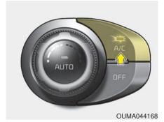
Press the A/C button to turn the air conditioning system on (indicator light will illuminate).
