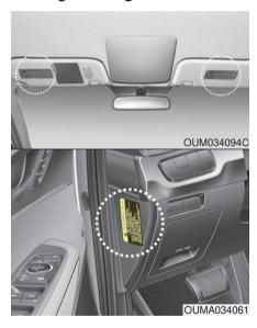
Air bag warning labels, some required by the Canada Motor Vehicle Safety Standards (CMVSS), are attached to the sunvisor to alert the driver and passengers of potential risks of the air bag system.
