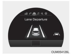
This mode displays the state of the Advanced Smart Cruise Control (ASCC) and Lane Departure Warning System (LDWS).
