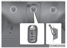
Child restraint hook holders are located on the back of the rear cushions.
