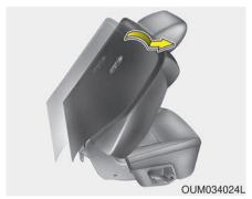
Fold the 2nd row seatback and push the seat to the farthest forward position.
