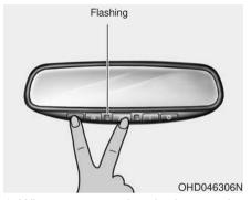
1. When programming the buttons for the first time, press and hold the left and center buttons (全 金) simultaneously until the indicator light begins to flash after approximately 20 seconds. (This procedure erases the factory-set default codes. Do not perform this step when programming the additional HomeLink buttons.)
