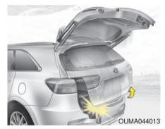
During power opening and closing if the power liftgate is blocked by an object or part of the body, the power liftgate will detect the resistance.
