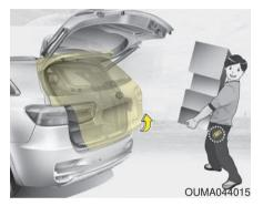
On a vehicle equipped with a smart key, the liftgate can be opened using the Smart Power Liftgate system.
