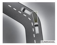
The ASCC may have limits to its ability to detect distance to the vehicle ahead due to road and traffic conditions.
