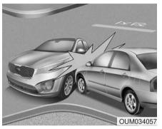
Front air bags may not inflate in side impact collisions, because occupants move to the direction of the collision, and thus in side impacts, frontal air bag deployment would not provide additional occupant protection.
