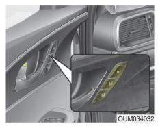
A driver position memory system is provided to store and recall the driver seat and outside rearview mirror position with a simple button operation. By saving the desired position into the system memory, different drivers can reposition the driver seat based upon their driving preference. If the battery is disconnected, the desired seat position memory will need to be re-saved.
