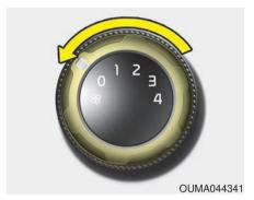
To turn off the blowers, turn the fan speed control knob to the "0" position.
