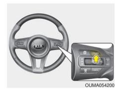
Press the CRUISE button. (the CRUISE indicator in the instrument cluster will go off).
