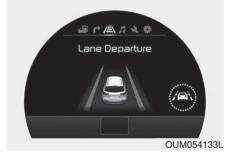
To activate/deactivate the LDWS: With the ignition switch in the ON position, press the LDWS button
