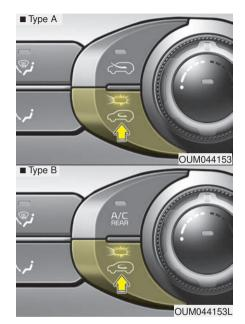
The air intake control is used to select the outside (fresh) air position or recirculated air position.
