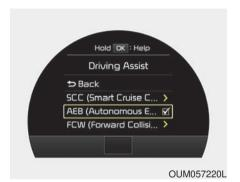
The driver can activate the AEB by placing the ignition switch to the ON position and by selecting 'User Settings', 'Driving Assist', and 'Assist Braking System'. The AEB deactivates, when the driver cancels the system setting.
