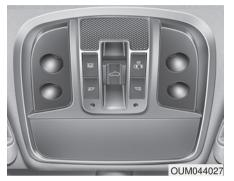
If your vehicle is equipped with a sunroof, you can slide or tilt your sunroof with the sunroof control lever located on the overhead console.
