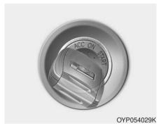
The steering wheel locks to protect against theft (if equipped). The ignition key can be removed only in the LOCK position.
