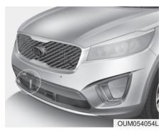
The sensor cannot maintain proper distance from the vehicle in front when the sensor lens is obscured by foreign substances, such as snow and rain, which will adversely affect performance. It may even temporarily cancel the AEB. Always keep the sensor clean.
