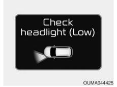
This warning message illuminates if there is a malfunction (burned-out bulb except LED lamp or circuit malfunction) with the headlamp. In this case, have your vehicle inspected by an authorized Kia dealer.
