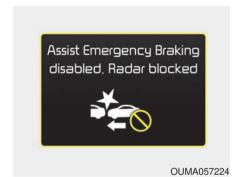
When the sensor is covered or the sensor lens is obscured by foreign substances, such as snow or rain, the AEB operation may temporarily stop. In this case, a warning message will appear to notify the driver.
