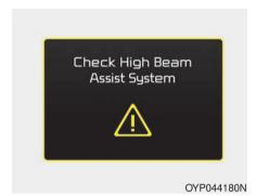
This warning message illuminates if there is a malfunction (burned-out bulb or circuit malfunction) with the headlamp. In this case, have your vehicle inspected by an authorized Kia dealer.
