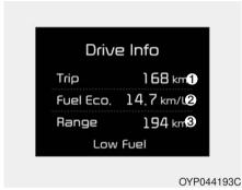
This display shows trip distance (1), average fuel economy (2) and the estimated distance that the vehicle can be driven with the remaining fuel (3).
