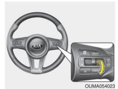
3.Move the lever down (to SET-), and release it at the desired speed. The SET indicator light in the instrument cluster will illuminate. Release the accelerator at the same time. The desired speed will automatically be maintained.
