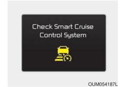
The message will appear when the vehicle to vehicle distance control system is not functioning normally.
