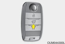
Press the power liftgate close button for approximately one second when the liftgate is opened.
