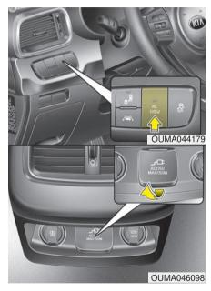
The AC inverter supplies 115V/150W electric power to operate electric accessories or equipment.
