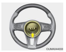
To sound the horn, press the horn symbols on your steering wheel. Check the horn regularly to be sure it operates properly.
