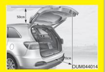
Make sure that there are no people or objects in the path of the power liftgate (or smart power liftgate) prior to use. Serious injury, damage to the vehicle or damage to surrounding objects may result if contact with the power liftgate (or smart power liftgate) occurs.
