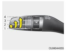
The light switch has a Headlight and a Parking light position.
