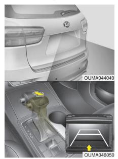
The rearview camera will activate with the ignition switch ON and the shift lever in the R (Reverse) position.
