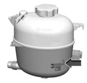
Check to see if coolant is visible in the coolant surge tank. If the coolant inside the coolant surge tank is boiling, do not do anything else until it cools down. If coolant is visible but the coolant level mark is not visible, add a 50/50 mixture of clean, drinkable water and DEX-COOL coolant at the coolant surge tank to the top rib on the middle of the tank, but be sure the cooling system is cool before this is done. See Engine Overheating \$\triangle\$ 276.
