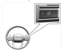
: If equipped, press to turn the heated steering wheel on or off. A light next to the button displays when the feature is turned on.
