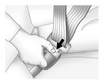
To unlatch the belt, push the pushbutton on the buckle. The belt should return to its stowed position.
