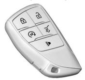
: Press to lock all doors. The turn signal indicators may flash and/or the horn may sound on the first press to indicate locking. To view available settings for this feature from the infotainment screen, touch Settings > Vehicle > Remote Lock, Unlock, Start.
