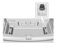
Remove the four wing nuts, then remove the cargo management system. See Cargo Management System \$ 86.
