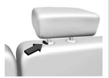
The height of the head restraint can be adjusted. Pull the head restraint up to raise it. Try to move the head restraint to make sure that it is locked in place.
