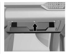
2. Push the rear center area of the glove box to lower beyond the stops.
