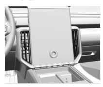
Use the air outlets in the center and on the side of the instrument panel to direct the airflow. move the center knobs on the air outlets to open or close off the airflow.
