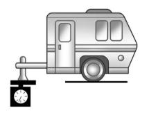
The trailer tongue weight contributes to the Gross Vehicle Weight (GVW). GVW includes the curb weight of your vehicle, any passengers, cargo, equipment, and the trailer tongue
