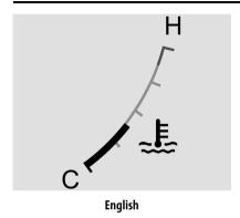
This gauge shows the engine coolant temperature.
