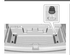
2. Remove the four wing nuts.
