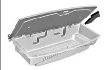
Remove the load floor. Open the load floor approximately 70% and pull upward and outward to release the two hooks from the rod affixed to the cargo management system.
