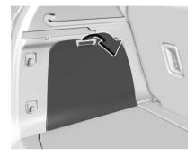
If equipped, there may be an outer panel that needs to be removed to get to the inner panel. Press the clip and pull the panel towards you to remove the panel.
