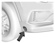
If equipped, the engine heater can provide easier starting and better fuel economy during engine warm-up in cold weather conditions at or below –18 °C (0 °F). Vehicles with an engine heater should be plugged in at least four hours before starting. An internal thermostat in the plug-end of the cord may exist, which will prevent engine heater operation at temperatures above –18 °C (0 °F).
