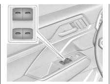
The power windows work when the vehicle is on, in accessory mode, or when *Retained Accessory Power (RAP)* ⇒ 187 is active. See Retained Accessory Power (RAP).
