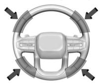
To begin steering manually, hold the steering wheel firmly with both hands using the highlighted regions. The Super Cruise light is lit red on the instrument cluster and a message displays in the DIC. In addition, beeps will sound, or the Safety Alert Seat will vibrate. To view Collision and Detection options from the infotainment screen, touch Settings > Vehicle > Collision/Detection Systems. After you begin steering manually, then Super Cruise will disengage.
