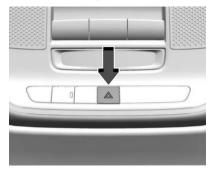
in Press this button on the overhead console to make the front and rear turn signal lamps flash on and off. This warns others that you are having trouble. Press again to turn the flashers off.
