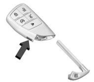
To remove the mechanical key, press the button on the side of the remote key, and pull the mechanical key out. Never pull the mechanical key out without pressing the button
