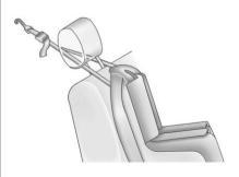
If the position you are using has an adjustable headrest or head restraint, adjust it accordingly to allow proper fitment. If you are using a dual tether, route the tether around the headrest or head restraint posts.
