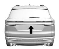
To open the liftgate, press the touch pad in the liftgate handle and lift up.
