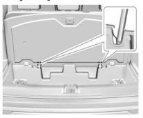
The hold open devices on the cargo bin allow the load floor to remain open without removal.
