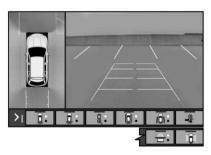
Touch the camera view buttons along the bottom of the infotainment display. Available views will differ depending on vehicle options.
