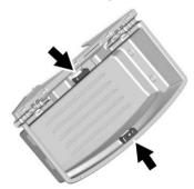
3. Lift up on the handles on both sides to remove the cargo management system to access the spare tire.
