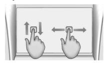
Drag is used to move applications on the infotainment home screen, or to pan the map. To drag the item, it must be held and moved along the display to the new location. This can be done up, down, right, or left. This feature is only available when vehicle is parked and not in motion.
