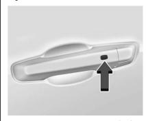
The remote key must be within 1 m (3 ft) of the liftgate or door being opened. Press the button on the door handle to open. See Remote Key Operation
