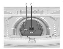
If the vehicle is equipped with a subwoofer (5), remove the center wing nut (6), then remove the subwoofer and set it aside. Do not disconnect the wiring harness.
