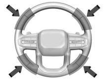
To begin steering manually, hold the steering wheel firmly with both hands using the highlighted regions. The Super Cruise light  $\widehat{\Theta}$  is lit red on the
