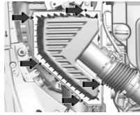
1. Remove the five screws and lift the cover out of the assembly.
