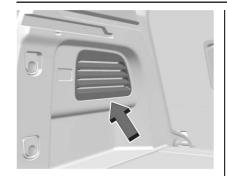
The inner panel is removed by prying along the top edge of the trim panel. Remove the trim panel to access the fuse block, or see your dealer.
