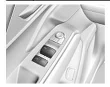
The power windows work when the vehicle is on, in accessory mode, or when Retained Accessory Power (RAP) is active. See Retained Accessory Power (RAP) ⇒ 179.
