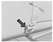
Disconnect the center seat belt mini-latch, using a key in the slot on the mini-buckle, and let the belt retract into the headliner.
