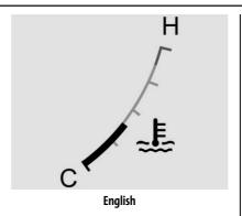
This gauge shows the engine coolant temperature.
