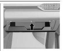
2. Push the rear center area of the glove box to lower beyond the stops.
