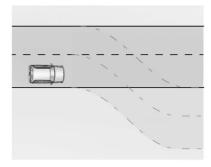
Super Cruise may occasionally provide an alert and/or steering that is considered unnecessary. It could respond to lane markings in different lanes, signs, guardrails, and other stationary objects when entering or exiting a curve. This is normal operation. The vehicle does not need service.
