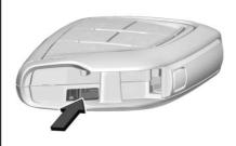
Separate the two halves of the remote key by using the blade of the mechanical key inserted into the bottom center of the remote key. Do not use the key slot.
