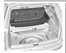
The load floor and storage bin can be placed on the lowered third row seats while accessing the spare tire.
