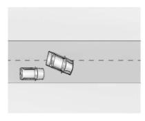
Super Cruise may not detect a vehicle that enters your lane or may not brake fast enough to avoid a crash. You must manually brake and steer the vehicle.
