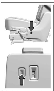
If equipped with power rear seats, the second row seat can also be moved for third row entry/exit by pressing the switch on the second row seat side or on the seatback of the second row seat.
