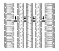
Treadwear indicators are one way to tell when it is time for new tires. Treadwear indicators appear when the tires have only 1.6 mm (1/16 in) or less of tread remaining. See *Tire Inspection* ⇒ 297 and *Tire Rotation* ⇒ 297.
