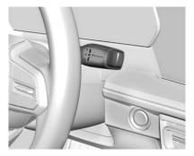
The shift pattern is displayed on the front of the shift lever. The selected gear position will illuminate red on the shift lever, while all others will be displayed in white. If the shift is not immediate, as in very cold conditions, the indicator on the shift switch may blink until it is fully engaged. P:
