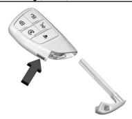
Press the button on the side of the remote key near the bottom and pull the mechanical key out. Never pull the mechanical key out without pressing the button.
