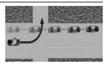
I-AEB can be set to Off, Alert, or Alert and Brake. To view available settings from the infotainment screen, touch Settings > Vehicle > Collision/Detection Systems.
