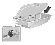
Angle the load floor approximately 70%, align the two hooks on the load floor above the rod, and push the load floor until the hooks engage the cargo bin rod.
