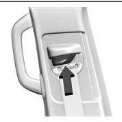
Press and hold the release button while raising or lowering the height adjuster to the desired position.
