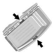
3. Lift up on the handles on both sides to remove the cargo management system to access the spare tire.
