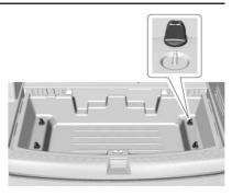
2. Remove the four wing nuts.
