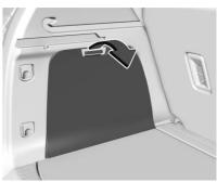
If equipped, there may be an outer panel that needs to be removed to get to the inner panel. Press the clip and pull the panel towards you to remove the panel.
