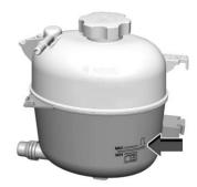
Check to see if coolant is visible in the coolant surge tank. If the coolant inside the coolant surge tank is boiling, do not do anything else until it cools down. If coolant is visible but the coolant level mark is not visible, add a 50/50 mixture of clean, drinkable water and DEX-COOL coolant at the coolant surge tank to the top rib on the middle of the tank, but be sure the cooling system is cool before this is done. See Engine Overheating \$\triangle\$ 270.
