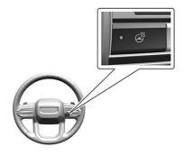
: If equipped, press to turn the heated steering wheel on or off. A light next to the button displays when the feature is turned on.
