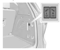
If equipped, press the switch on the side trim of the cargo area to fold the second row seatback. The left switch folds the left seatback, and the right switch folds the right seatback.
