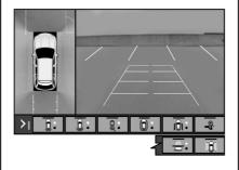
Touch the camera view buttons along the bottom of the infotainment display. Available views will differ depending on vehicle options.
