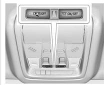
The dome lamp is in the overhead console. To operate, press the following buttons:
