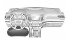
The driver knee airbag is below the steering column.
