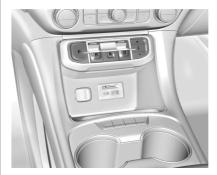
The shift switches are on the center stack. The selected gear position will illuminate red on the shift switch, while all others will be displayed in white. If the shift is not
