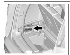
Remove the side bin, load floor, and foam. See Cargo Management System  $\Leftrightarrow$  85.
