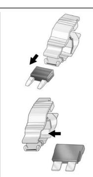
3. Use the fuse puller to remove the fuse from the top or side, as shown above.
