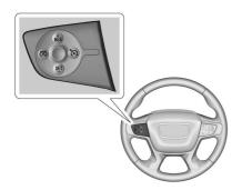
(S): Press to turn the system on and off. A white indicator appears in the instrument cluster when cruise is turned on.
