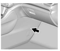
The instrument panel fuse block is inside the center console on the passenger side of the vehicle.
