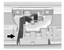
Go to the front of the vehicle and locate the secondary release lever under the front center of the hood. Push the secondary hood release lever to the right to release. After you have partially lifted the hood, the gas strut system will automatically lift the hood and hold it in the fully open position.
