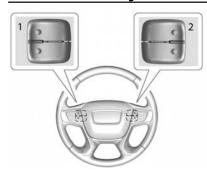
The favorites and volume switches are on the back of the steering wheel.
