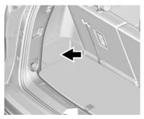
The rear compartment fuse block is behind a trim panel on the driver side of the rear storage compartment.
