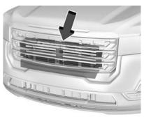
The vehicle may have a shutter system designed to help improve fuel economy. Keep the shutter system clear of debris,
