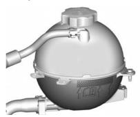
Check to see if coolant is visible in the coolant surge tank. If the coolant inside the coolant surge tank is boiling, do not do anything else until it cools down. See Engine
