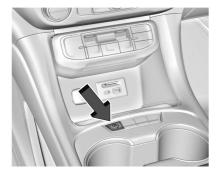
The automatic engine Stop/Start feature can be disabled and enabled by pressing (A). Auto Stop/Start is enabled each time you start the vehicle.
