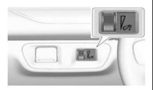
This feature adjusts the brightness of all illuminated controls. This feature is on the left side of the instrument panel.
