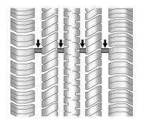
Treadwear indicators are one way to tell when it is time for new tires. Treadwear indicators appear when the tires have only 1.6 mm (1/16 in) or less of tread remaining. See *Tire Inspection* \$ 313 and *Tire Rotation* \$ 313 for additional information.
