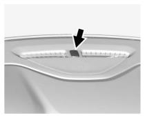
The solar sensor, located in the defrost grille in the middle of the instrument panel, monitors the solar heat. Do not cover the solar sensor or the system will not work properly.
