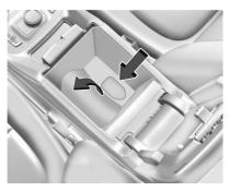
Place the new transmitter into the transmitter pocket. The transmitter pocket is under the liner on the bottom of the center console storage area. Lift up the liner and set it aside.
