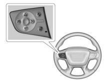
The Collision Alert control is on the steering wheel. Press to set the FCA timing to Far, Medium, or Near, or on some vehicles, Off. The first button press shows the current
