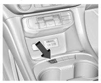
The automatic engine Stop/Start feature can be disabled and enabled by pressing (A). Auto Stop/Start is enabled each time you start the vehicle.
