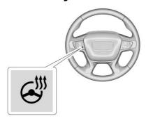
: If equipped, press to turn it on or off. An indicator light next to the button displays when the feature is turned on.
