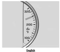
This gauge shows the engine oil temperature.
