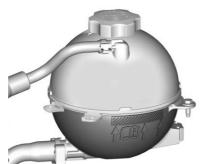
The coolant surge tank is located in the engine compartment on the driver side of the vehicle. See *Engine Compartment*Overview
