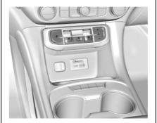
The shift switches are on the center stack. The selected gear position will illuminate red on the shift switch, while all others will be displayed in white. If the shift is not immediate, as in very cold conditions, the indicator on the shift switch may flash until it is fully engaged.
