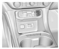
ERS or manual mode allows for the selection of the range of gear positions. Use this mode when driving downhill or towing a trailer to limit the top gear and vehicle
