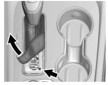
2. Remove the shift lever boot by pulling up on the rear of the trim plate.
