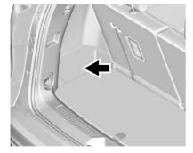
The rear compartment fuse block is behind a trim panel on the driver side of the rear storage compartment.
