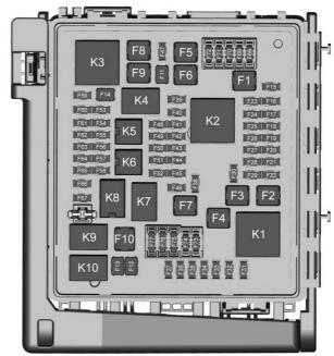
**Engine Compartment Fuse Block**
