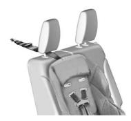
If the position you are using has a fixed headrest or head restraint and you are using a single tether, route the tether under the headrest or head restraint.
