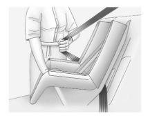
Pull the shoulder belt all the way out of the retractor to set the lock. When the retractor lock is set, the shoulder belt can be tightened but not pulled out of the retractor.
