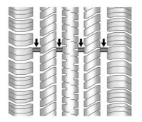
Treadwear indicators are one way to tell when it is time for new tires. Treadwear indicators appear when the tires have only 1.6 mm (1/16 in) or less of tread remaining. See *Tire Inspection* ♀ 329 and *Tire Rotation* ♀ 329.
