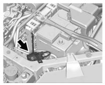
Open the hood and unwrap the electrical cord. The bundled cord is on the driver side of the engine compartment, in front of the battery. See Engine Compartment Overview
