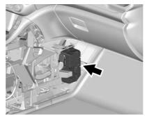
To reinstall the door, push the door back into its original location.
