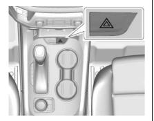
⚠: Press this button to make the front and rear turn signal lamps flash on and off. This warns others that you are having trouble. Press again to turn the flashers off.
