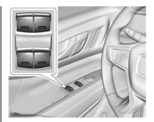
The windows work when the vehicle is in ON/RUN, ACC/ACCESSORY, or Retained Accessory Power (RAP). See Retained Accessory Power (RAP) ⇒ 230.
