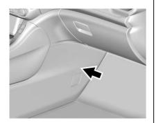
The instrument panel fuse block is inside the center console on the passenger side of the vehicle.
