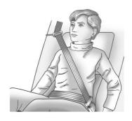
4. Buckle, position, and release the safety belt as described previously in this section. Make sure the shoulder portion of the belt is on the shoulder and not falling off of it. The belt should be close to, but not contacting, the neck To remove and store the comfort guide, squeeze the belt edges together so that the safety belt can be removed from the guide. Slide the guide back into its storage pocket on the side of the seatback.
