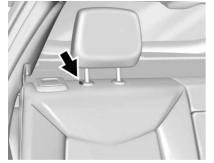
To lower the head restraint, press the button, located on the top of the seatback, and push the head restraint down. Try to move the head restraint after the button is released to make sure that it is locked in place.
