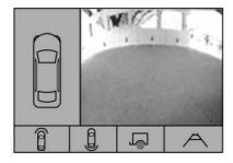
If equipped, a view of the area in front of the vehicle displays. The view displays after shifting from R (Reverse) to a forward gear, or by touching CAMERA in the infotainment display, and when the vehicle is moving forward slower than 8 km/h (5 mph). If equipped, the Front Vision Camera also displays when the Parking Assist system detects an object within 30 cm (12 in).
