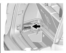
Remove the side bin, load floor and foam. See *Cargo Management System ⇒ 109*.
