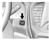
Vehicles with Keyless Access have pushbutton starting.
