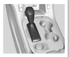
**P**: This position locks the front wheels. It is the best position to use when starting the engine because the vehicle cannot move easily.
