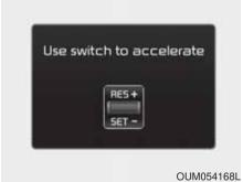
In traffic, your vehicle will stop if the vehicle ahead of you stops. Also, if the vehicle ahead of you starts moving, your vehicle will start as well. However, if the vehicle stops for more than 3 seconds, you must depress the accelerator pedal or move up/down the lever (to RES+ or SET-) to start driving.
