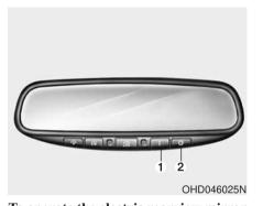
To operate the electric rearview mirror Press the I button (1) to turn the automatic- dimming function on. The mirror indicator light will illuminate. Press the O button (2) to turn the automatic- dimming function off. The mirror indicator light will turn off.
