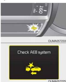
When the AEB is not working properly, the AEB warning light ( ) will illuminate and the warning message will appear for a few seconds. After the message disappears, the master warning light ( ) will illuminate. In this case, we recommend you to have the vehicle inspected by an authorized Kia dealer.
