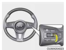
3.Move the lever down (to SET-), and release it at the desired speed. The SET indicator light in the instrument cluster will illuminate. Release the accelerator at the same time. The desired speed will
