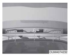
4. Loosen the retaining nuts and remove the spoiler.
