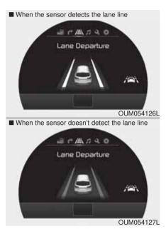
If the system detects that your vehicle is leaving the lane when the LDWS is operating and vehicle speed exceeds 64 km/h (40 mph), the warning operates as follows:
