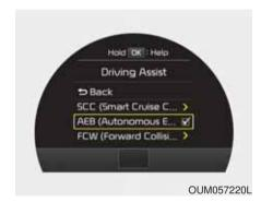
The driver can activate the AEB by placing the ignition switch to the ON position and by selecting 'User Settings', 'Driving Assist', and 'Assist Braking System'. The AEB deactivates, when the driver cancels the system setting.
