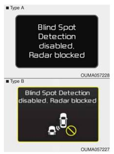
The message will appear to notify the driver if there are foreign substances on the rear bumper or it is hot near the rear bumper. The light on the switch and the system will turn off automatically. Remove the foreign substance on the rear bumper.
