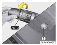
Adaptive front lighting system uses the steering angle and vehicle speed, to keep your field of vision wide by swiveling and leveling the headlamp.
