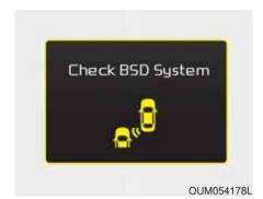
If the system does not work properly, a warning message will appear and the light on the switch will turn off. The system will turn off automaticallv.
