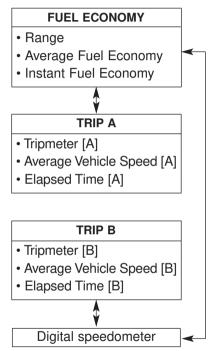
To change the trip mode, scroll the TRIP scroll switch  $(\triangle/\nabla)$  in the trip computer mode.
