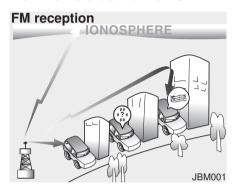
AM and FM radio signals are broadcast from transmitter towers located around your city. They are intercepted by the radio antenna on your vehicle. This signal is then processed by the radio and sent to your vehicle speakers.
