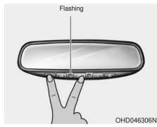
1. When programming the buttons for the first time, press and hold the left and center buttons (介介) simultaneously until the indicator light begins to flash after approximately 20 seconds. (This procedure erases the factory-set default codes. Do not perform this step when programming the additional HomeLink buttons.)
