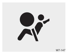
The purpose of air bag warning light in your instrument panel is to alert you of a potential problem with your air bag system, which could include your side and/or curtain air bags used for rollover protection.
