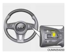
Press the CRUISE button. (the CRUISE indicator in the instrument cluster will go off).
