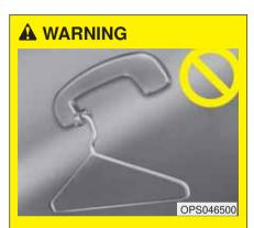
Do not hang other objects such as hangers or hard objects except clothes. Also, do not put heavy, sharp or breakable objects in the clothe pockets. In an accident or when the curtain air bag is inflated, it may cause vehicle damage or personal injury.
