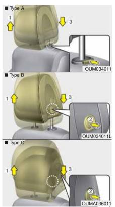
To raise the headrest, pull it up to the desired position (1). To lower the headrest, push and hold the release button (2) on the headrest support and lower the headrest to the desired position (3).
