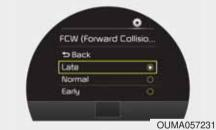
The driver can select the initial warning activation time in the User Settings in the instrument cluster LCD display. The options for the initial Forward Collision Warning include the following:
