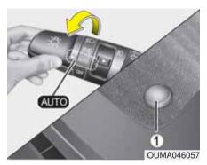
It will operate when the ignition is in "ON" or the engine is running.
