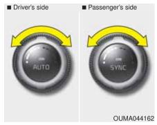
2. Turn the temperature control knob to the desired temperature.
