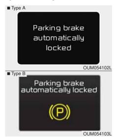
If the EPB is applied while Auto Hold is activated because of ESC (Electronic Stability Control) signal, a warning will sound and a message will appear.
