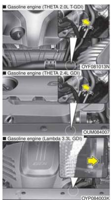
The engine number is stamped on the engine block as shown in the drawing.
