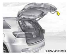
To close the liftgate, lower and push down the liftgate firmly. Make sure that the liftgate is securely latched. Make sure your hands, feet and other parts of your body are safely out of the way before closing the liftgate.
