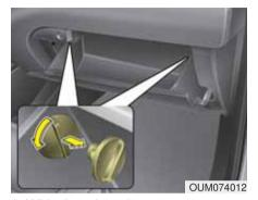
2. With the glove box open, remove the stoppers on both sides.
