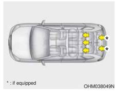
The rear seat(s) is equipped with headrests in all the seating positions for the occupant's safety and comfort. The headrests not only provide comfort for passengers, but also helps protect the head and neck in the event of a collision.
