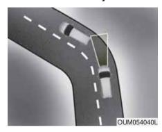
The ASCC may have limits to its ability to detect distance to the vehicle ahead due to road and traffic conditions.
