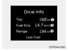
This display shows trip distance (1), average fuel economy (2) and the estimated distance that the vehicle can be driven with the remaining fuel (3).
