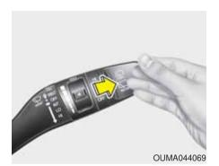
Push the lever away from you to spray rear washer fluid and to run the rear wipers 1~3 cycles. The spray and wiper operation will continue until vou release the lever.
