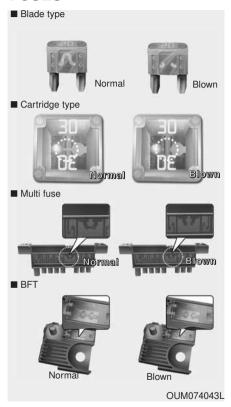
A vehicle's electrical system is protected from electrical overload damage by fuses.
