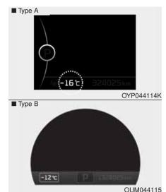
This gauge indicates the current outside air temperatures by 1°C (1°F).
