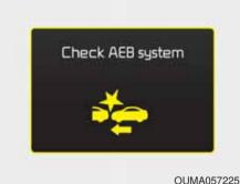
· This warning message illuminates if there is a malfunction with the Autonomous Emergency Braking (AEB) system. In this case, have your vehicle be inspected by an authorized Kia dealer.
