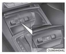
If your vehicle has an AUX and/or USB(universal serial bus) port, you can use the AUX port to connect audio devices and the USB port to plug in a USB device or iPod<sup>®</sup>.
