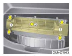
3. Remove the climate control air filter case by pulling out right side of the cover.
