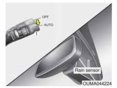
The rain sensor located on the upper end of the windshield glass senses the amount of rainfall and controls the wiping cycle for the proper interval. The more it rains, the faster the wiper operates. When the rain stops, the wipers stop. To vary the speed setting, turn the speed control knob (1).
