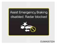
When the sensor is covered or the sensor lens is obscured by foreign substances, such as snow or rain, the AEB operation may temporarily stop. In this case, a warning message will appear to notify the driver.
