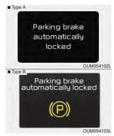
If the EPB is applied while Auto Hold is activated because of ESC (Electronic Stability Control) signal, a warning will sound and a message will appear.
