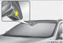
The message will appear when camera's field of view is covered by some objects. The system stops until the field of view is normal.
