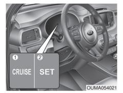
The cruise control system allows you to program the vehicle to maintain a constant speed without depressing the accelerator pedal.
