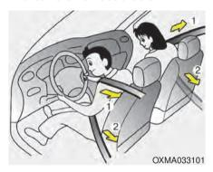
Your vehicle is equipped with driver's and front passenger's pre-tensioner seat belts (retractor pretensioner and EFD (Emergency Fastening Device)). The pre-tensioner seat belts may be activated, when a frontal collision is severe enough, together with the air bags.
