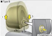
To raise the headrest, pull it up to the desired position (1). To lower the headrest, push and hold the release button (2) on the headrest support and lower the headrest to the desired position (3).
