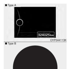
The odometer Indicates the total distance that the vehicle has been driven and should be used to determine when periodic maintenance should be performed.
