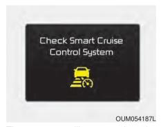
The message will appear when the vehicle to vehicle distance control system is not functioning normally.
