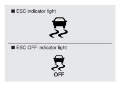
When ignition switch is turned to ON, the indicator light illuminates, then goes off if the ESC system is operating normally.
