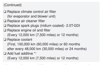
\* Inspect : Inspect and if necessary, adjust, correct, clean or replace.
