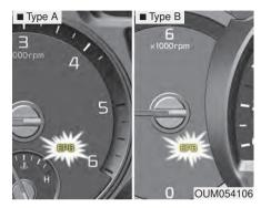
This warning light illuminates if the engine start/stop button is changed to the ON position and goes off in approximately 3 seconds if the system is operation normally.
