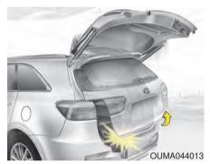
During power opening and closing if the power liftgate (tailgate) is blocked by an object or part of the body, the power liftgate (tailgate) will detect the resistance.
