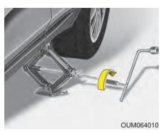
Insert the wheel lug nut wrench into the jack and turn it clockwise, raising the vehicle until the tire just clears the ground. This measurement is approximately 30 mm (1 in.).
