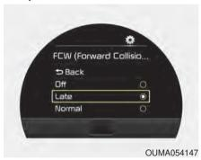
Go to the User Settings Mode (Driving Assist) and select FCW (Forward Collision Warning) on the LCD display.
