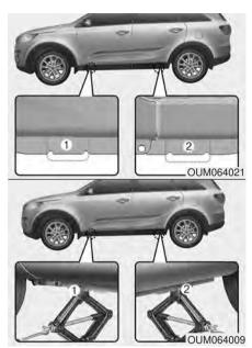
7. Place the jack at the front (1) or rear (2) jacking position closest to the tire you are changing. Place the jack at the designated locations under the frame. The jacking positions are plates welded to the frame with two tabs and a raised dot to index with the jack.
