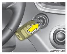
If the battery is weak or the smart key does not work correctly, you can start the engine by pressing the engine start/stop button with the smart key.
