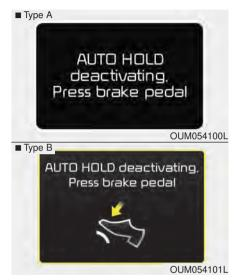
When the conversion from Auto Hold to EPB is not working properly a warning will sound and a message will appear.
