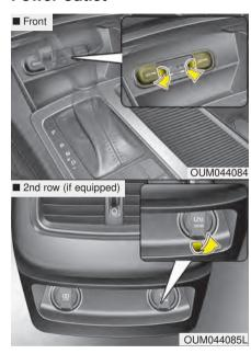
The power outlet is designed to provide power for mobile telephones or other devices designed to operate with vehicle electrical systems. The devices should draw less than 10 amps with the engine running.
