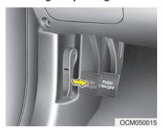
Check whether the stroke is within specification when the parking brake pedal is depressed with 30 kg (66 lb, 294 N) of force. Also, the parking brake alone should securely hold the vehicle on a fairly steep grade. If the stroke is more or less than specified, have the parking brake adjusted by an authorized Kia dealer.
