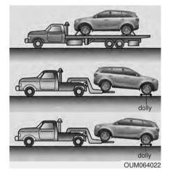
If emergency towing is necessary, we recommend having it done by an authorized Kia dealer or a commercial tow-truck service. Proper lifting and towing procedures are necessary to prevent damage to the vehi-
