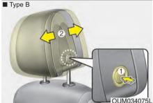
The headrest may be adjusted forward to 4 different positions by pulling the headrest forward to the desired detent. To adjust the headrest to it's full rearward position.
