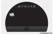
When the LDWS is not working properly, the warning light will illuminate and the warning message will come on for a few second. After the message disappears, the master warning light will illuminate.
