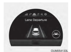
To operate the LDWS, press the button with the engine start/stop button in the ON position. The indicator illuminates on the cluster. To cancel the LDWS, press the button again.
