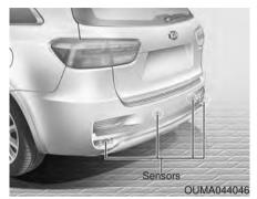
The rear parking assist system assists the driver during backward movement of the vehicle by chiming if any object is sensed within a distance of 120 cm (47 in.) behind the vehicle.
