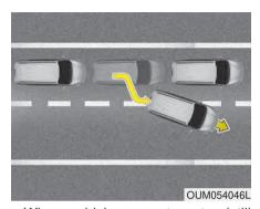
When vehicles are at a standstill and the vehicle in front of you changes to the next lane, be careful when your vehicle starts to move because it may not recognize the stopped vehicle in front of you.
