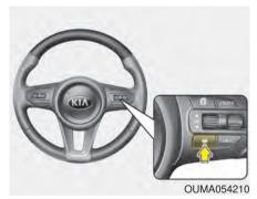
This function allows you to program the vehicle to maintain relative distance to the vehicle ahead without depressing the accelerator pedal or brake pedal. The vehicle to vehicle distance will automatically activate when the ASCC is on.
