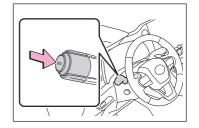
When the headlight switch lever is in the low beam position, the AHS system will be enabled and the AHS indicator will illuminate.
