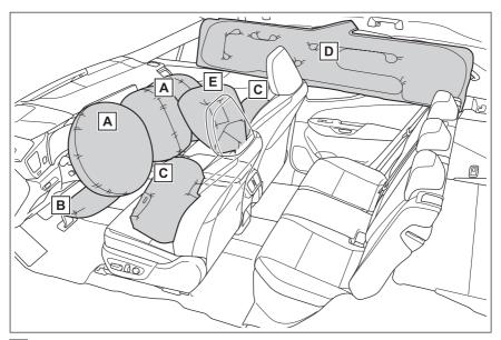
A SRS driver airbag/front passenger airbag
