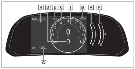
A Engine coolant temperature gauge
