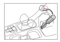
5 Press and hold the shift lock override button and then push the button on the shift knob.
