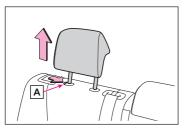
Pull the head restraint up while pressing the lock release button  $\boxed{\mathbf{A}}$ .
