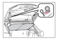
2 Pull the lever upwards and fold the deck board.
