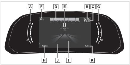
A Engine coolant temperature gauge
