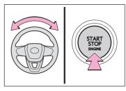
To prevent the steering lock motor from overheating, operation of the motor may be suspended if the engine is turned on and off repeatedly in a short period of time. In this case, refrain from running the engine. After about 10 seconds, the steering lock motor will resume functioning.
