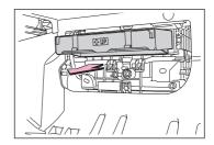
6 Remove the air conditioning filter from the filter case and replace it with a new one.
