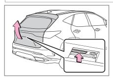
Lift the back door while pressing the back door opener switch.
