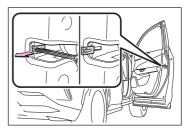
2 Insert the mechanical key into the opening.
