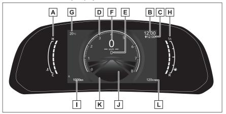
A Engine coolant temperature gauge
