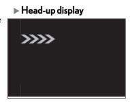
When the system determines that your vehicle may be about to enter an intersection even though a vehicle is approaching from the left or right in front of your vehicle, a buzzer will sound and a message will be displayed to urge you to depress the brake pedal.
