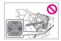
There is a label(s) on the passenger side sun visor, indicating it is forbidden to attach a rear-facing child restraint system to the front passenger seat.
