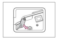
3 Using a screwdriver, push the lever.
