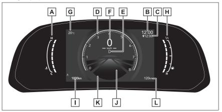
A Engine coolant temperature gauge
