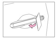
2 Using the mechanical key, turn the door lock to the lock side to disable the door.
