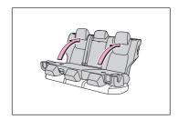
2 Check that the plate for each seat belt is on the front side of the seat.
