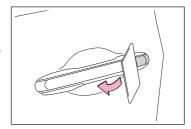
Using the mechanical key, turn the lock cylinder to the unlock side to enable the manual release handle.
