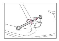
4 Tighten down the towing eyelet securely using a wheel bolt wrench or hard metal bar.
