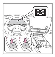
1 Pull the switch to set the parking brake.
