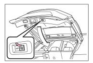
Perform the following procedure with no electronic keys for this vehicle inside the vehicle. When the power back door is closed, all of the doors will lock.
