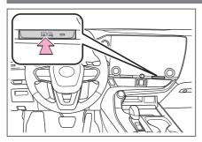
Press the rear windshield and outside rear view mirror defogger switch.
