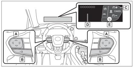
A The function of each switch differs depending on the conditions and settings.
