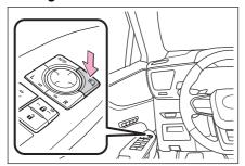
Press the switch to fold the mirrors.
