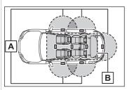
A When locking or unlocking the doors (vehicles with entry function)
