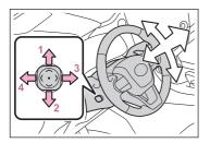
Operating the switch moves the steering wheel in the following directions:
