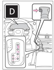
\*1: For the vehicle be able to be shifted from P, the brake pedal must be depressed before the shift release button is pushed. If the shift release button is pushed first, the shift lock will not be released.
