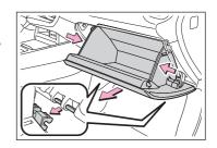
4 Unlock the filter cover (A), pull the filter cover out of the claws (B), and remove the filter cover.
