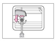
5 Using a screwdriver, push the lever.
