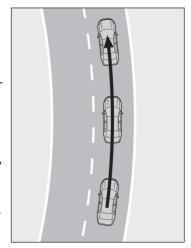
If the system determines that the steering wheel has not been operated for a certain amount of time or the steering wheel is not being firmly gripped, the driver will be alerted via a display and this function will be temporarily canceled.
