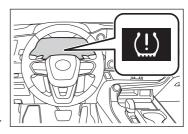
If the specified tire inflation pressure of the wheel set installed differs from that of the previous set, it will be necessary to perform the tire inflation pressure setting procedure of the tire pressure warning system.
