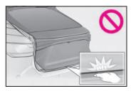
Use caution when using the back door closer as it still operates when the power back door system is disabled.
