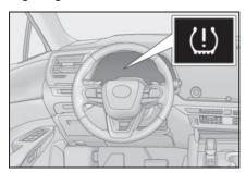
7 If the specified tire inflation pressure of the wheel set installed differs from that of the previous set, it will be necessary to perform the tire inflation pressure setting procedure of the tire pressure warning system. (→P.460)
