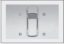
When "Adjust Pressure" is displayed on the multi-information display (Normal Warning)
