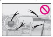
Do not attach anything to areas such as the doors, windshield, side windows, front or rear pillars, roof side rails and assist grips.
